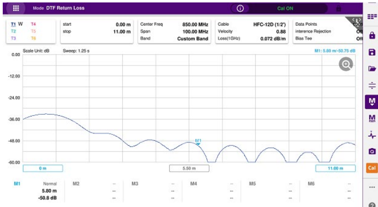
Reflection VSWR & DTF return loss measurement screen (horizontal layout)
