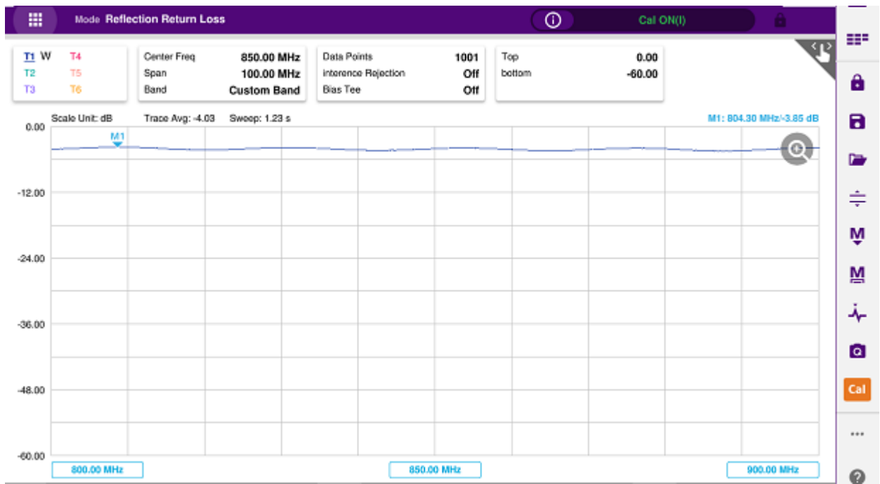
Reflection return loss measurement screen (zoom zones)
