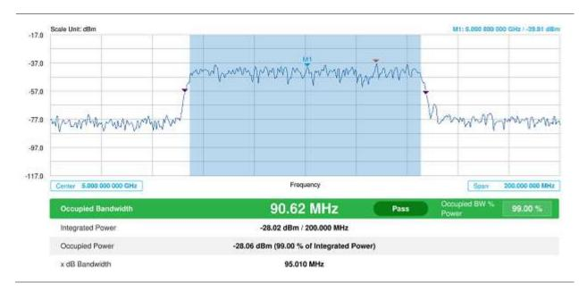
The Occupied Bandwidth measurement shows both of power across the band and power bandwidth in a user specified percentage to determine the amount of spectrum used by a modulated signal. Occupied bandwidth is typically calculated as the bandwidth containing 99% of the transmitted power.
