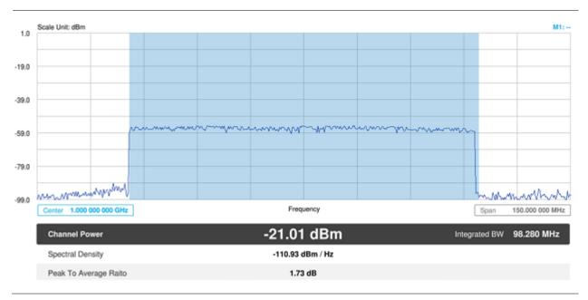
Channel power measurement result shows channel power and spectrum density in a user specified channel bandwidth. The peak to average ratio (PAR) is shown at the bottom of the screen as well. The shaded area on the display indicates the channel bandwidth.
