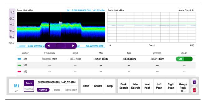
You can go to Menu > Limit to analyze your measurements with the display line, multi-segment line, and channel limit. See "Setting limit" for more details. Once you tap the vertical move bar and move it up and down, the reference line value changes.
