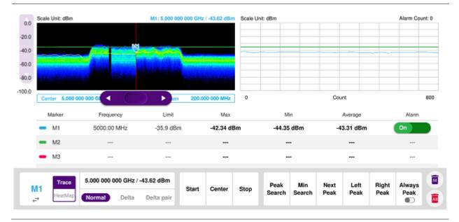
You can go to Menu > Limit to analyze your measurements with the display line, multi-segment line, and channel limit. See "<u>Setting limit</u>" for more details. Once you tap the vertical move bar and move it up and down, the reference line value changes.
