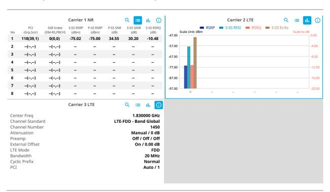
NSA analyzer measurement with sweep normal (tapped the Magnifier icon)
