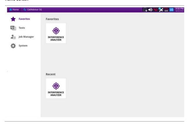
The Home screen provides access to the **Tests**, **Job Manager**, and **System** pages. You can return to the **Home** screen at any time by clicking the **Home** button in the top left corner of the screen.
