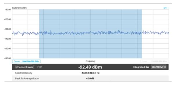
Channel power measurement result shows channel power and spectrum density in a user specified channel bandwidth. The peak to average ratio (PAR) is shown at the bottom of the screen as well. The shaded area on the display indicates the channel bandwidth.
