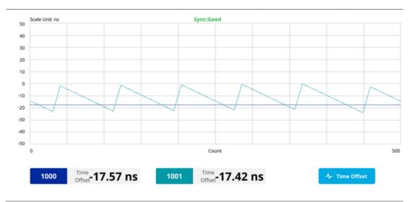
MIMO time alignment error with time offset chart with 5G TM
