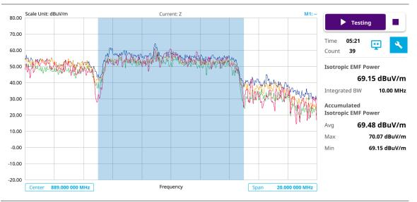
EMF Spectrum (level recorder) measurement
