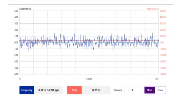
You can tap the Distance box and input the value that you want to compensate for distance. When distance is entered, the time will show the value with distance correction. Make sure the default value for Distance is 0.
