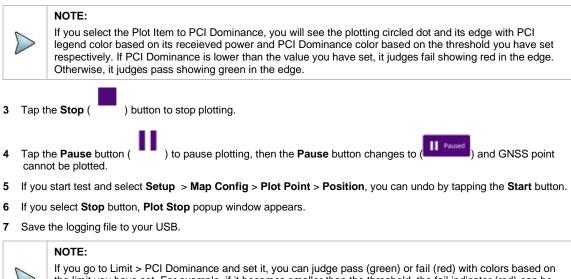
If you go to Limit > PCI Dominance and set it, you can judge pass (green) or fail (red) with colors based on the limit you have set. For example, if it becomes smaller than the threshold, the fail indicator (red) can be identified in the PCI column of the Information window and the top right corner of the instrument at the same time.
