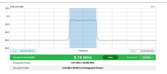
The Occupied Bandwidth measurement shows both of power across the band and power bandwidth in a user specified percentage to determine the amount of spectrum used by a modulated signal. Occupied bandwidth is typically calculated as the bandwidth containing 99% of the transmitted power.
