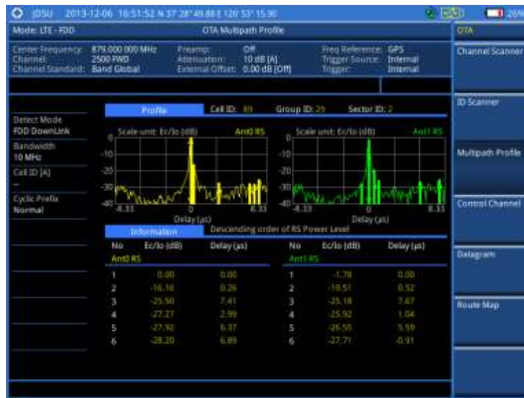
Figure 119 Multipath profile measurement with LTE-FDD OTA signal analyzer
