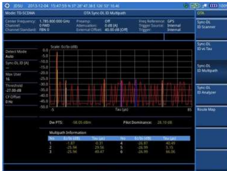
Figure 245 Sync-DL ID multipath measurement with TD-SCDMA OTA signal analyzer
