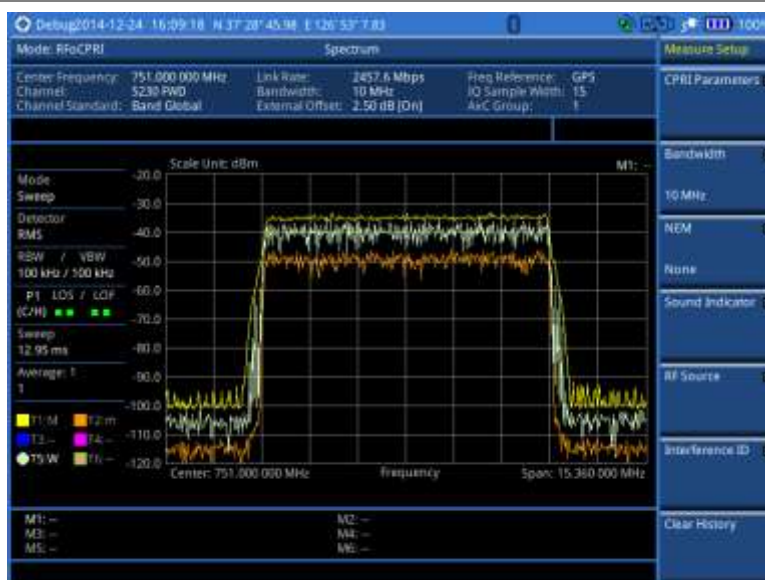
Figure 299 RFoCPRI spectrum analysis on LTE Uplink 10 MHz, antenna 2
