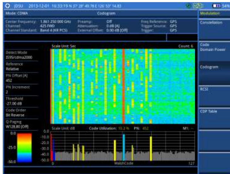
Figure 189 Codogram in full view with CDMA signal analyzer
