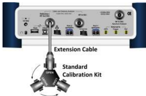
Figure 269 1-port calibration connection with mechanical Y-Cal kit
