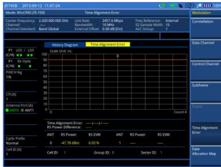
Figure 333 Time alignment error measurement with RFoCPRI LTE-TDD signal analyzer
