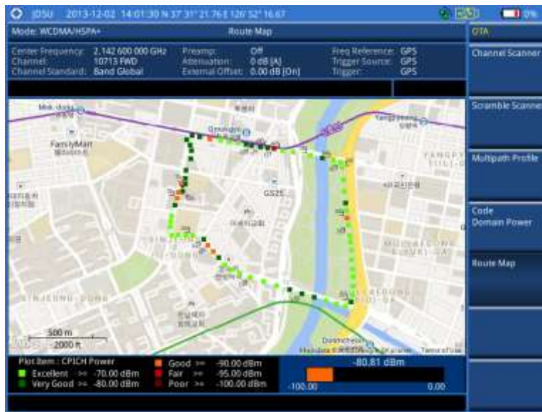
Figure 84 Route map measurement ( CPICH Ec/Io ) with WCDMA/HSPA+ OTA signal analyzer
