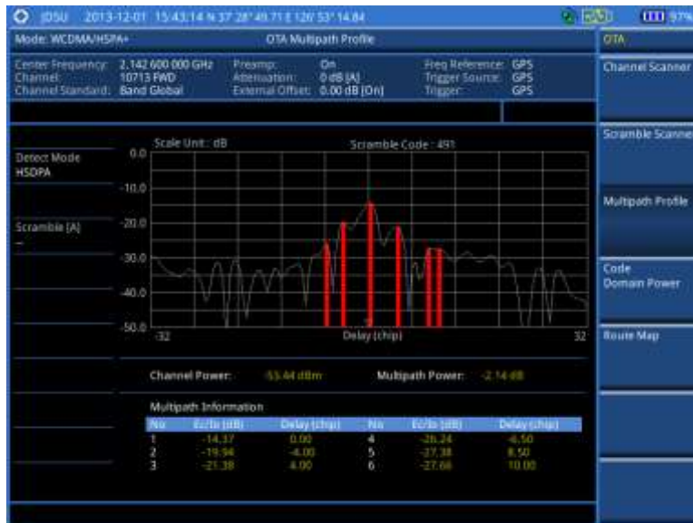
Figure 81 Multipath profile measurement with WCDMA/HSPA+ OTA signal analyzer
