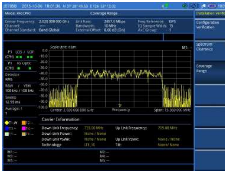
Figure 352 Example of coverage range in BBU emulation
