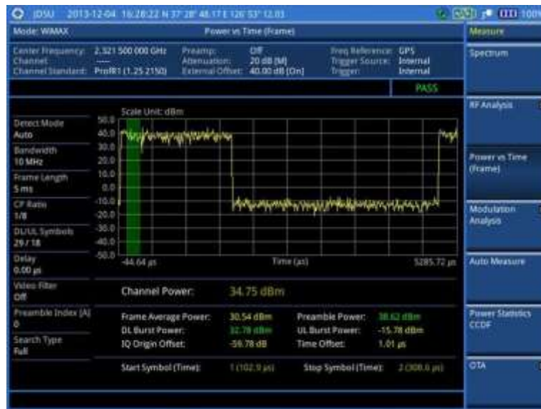
Figure 258 Power vs. time (frame) measurement with Mobile WiMAX signal analyzer
