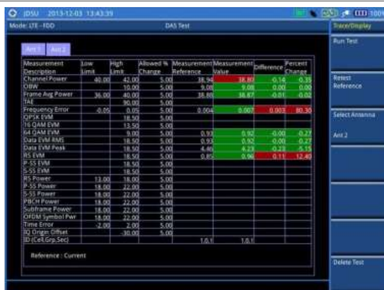
Figure 113 DAS measurement with LTE-FDD signal analyzer
