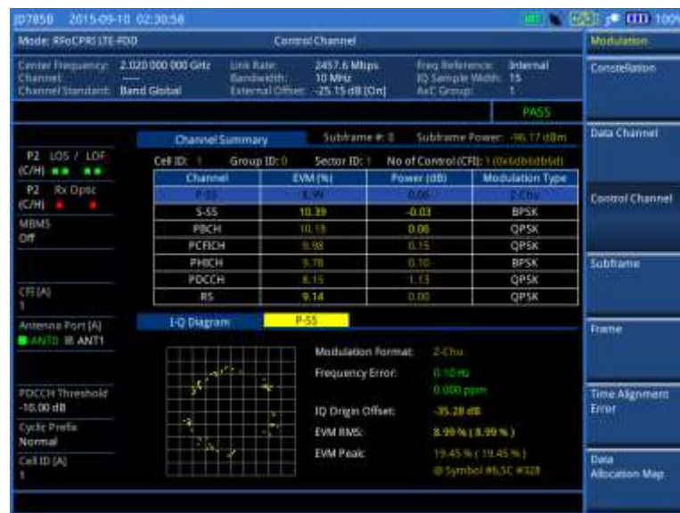
Figure 318 Control channel measurement with RFoCPRI LTE-FDD signal analyzer
