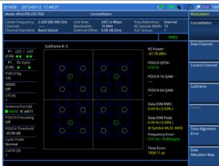
Figure 329 Constellation measurement with RFoCPRI LTE-TDD signal analyzer
