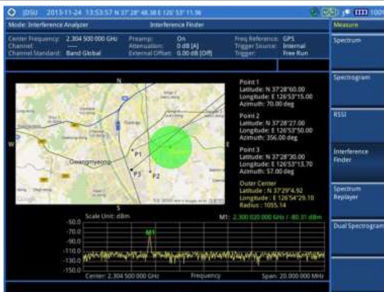
Figure 37 Interference finder measurement in map view
