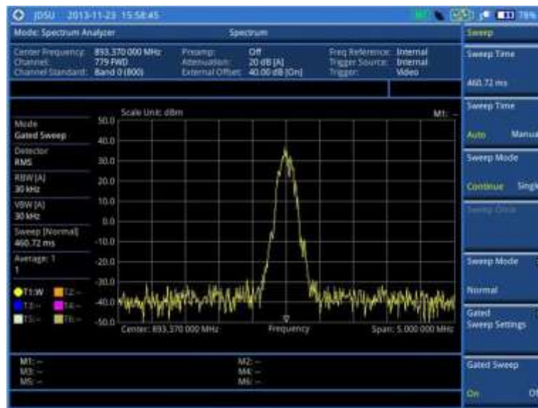
Figure 15 Gate sweep measurement with spectrum analyzer
