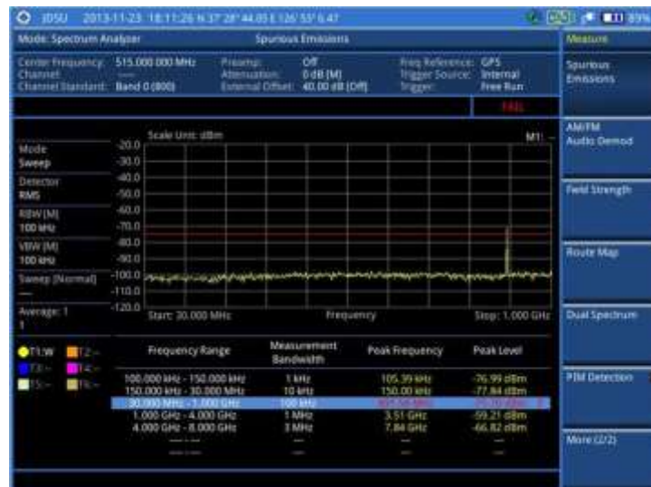
Figure 21 Spurious emissions measurement with spectrum analyzer
