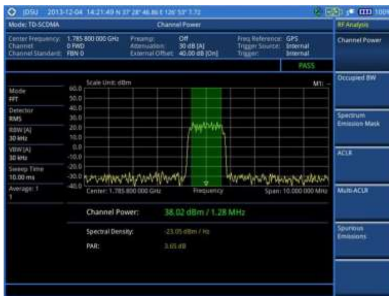
Figure 229 Channel power measurement with TD-SCDMA signal analyzer
