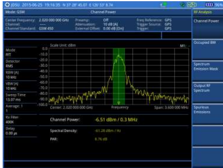
Figure 46 Channel power measurement with GSM signal analyzer
