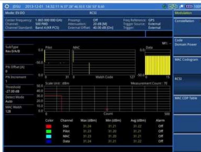
Figure 215 RCSI measurement with EV-DO signal analyzer
