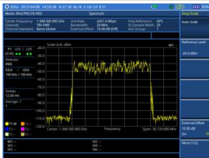
Figure 312 Spectrum measurement with RFoCPRI LTE-FDD signal analyzer
