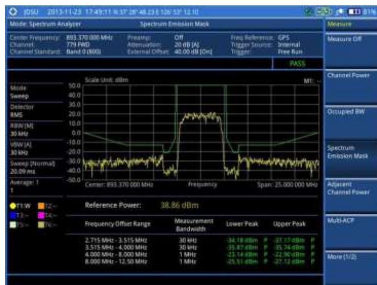
Figure 18 Spectrum emission mask measurement with spectrum analyzer
