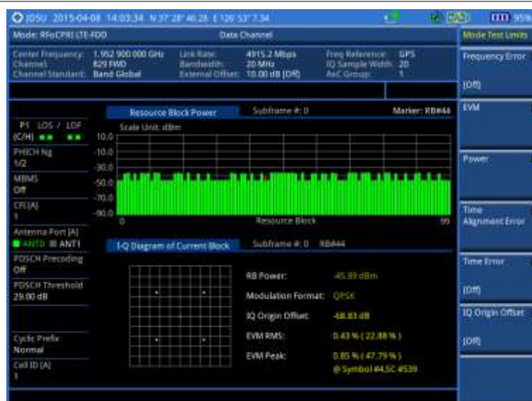
Figure 317 Data channel measurement with RFoCPRI LTE-FDD signal analyzer
