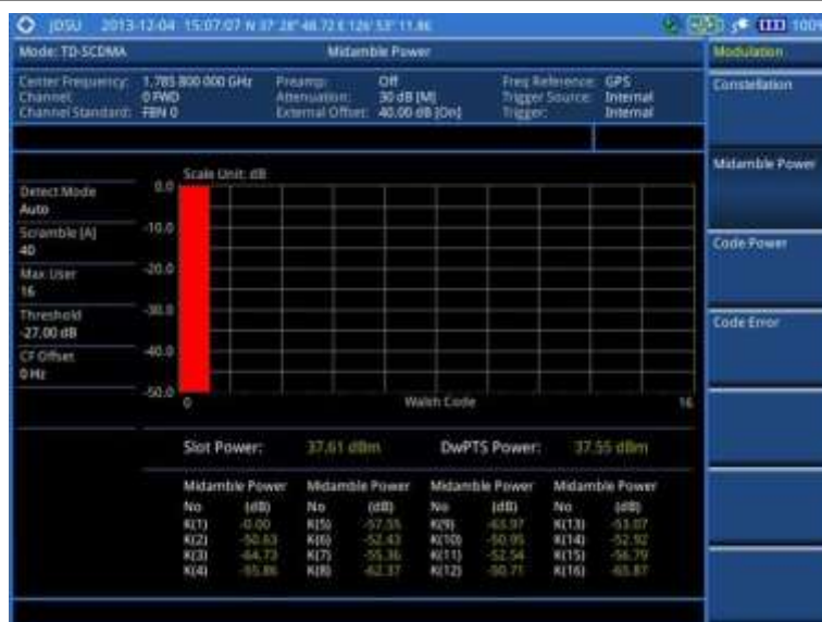
Figure 240 Midamble measurement with TD-SCDMA signal analyzer
