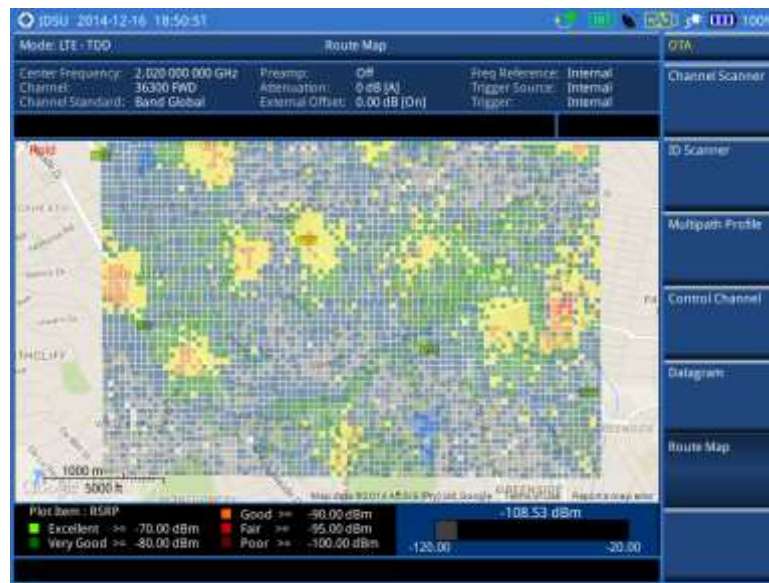
Figure 173 Raster image overlaid on the base map with LTE-TDD OTA signal analyzer
