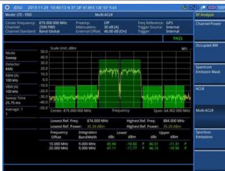
Figure 96 Multi-ACLR measurement with LTE-FDD signal analyzer
