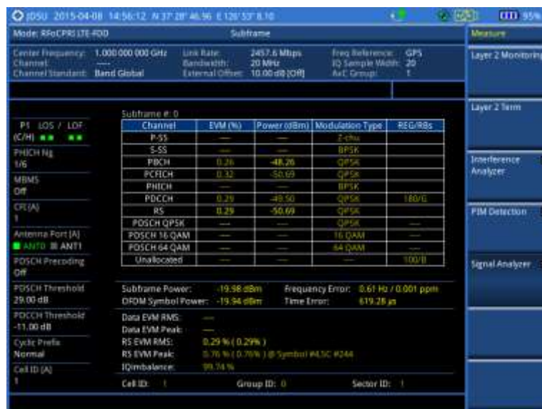
Figure 319 Subframe measurement (regular view) with RFoCPRI LTE-FDD signal analyzer
