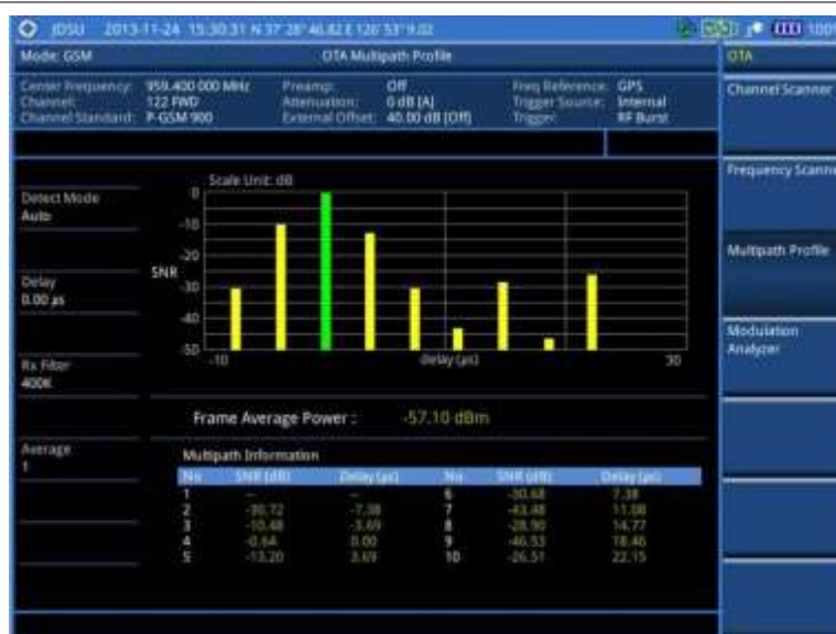
Figure 58 Multipath profile measurement with GSM OTA signal analyzer
