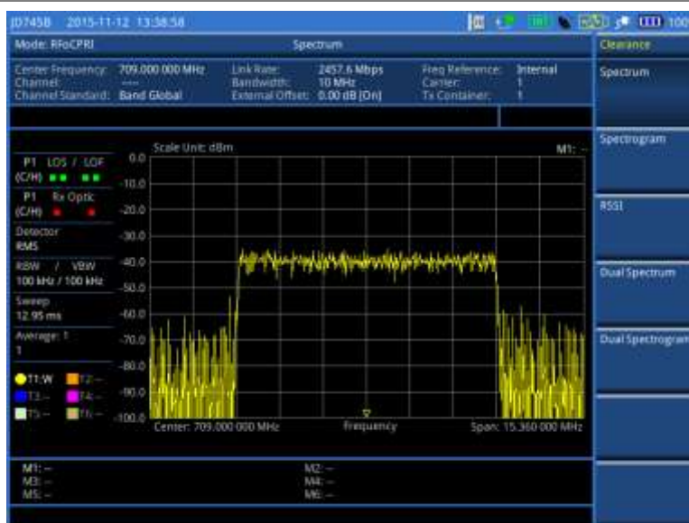
Figure 347 Example of spectrum measurement in BBU emulation
