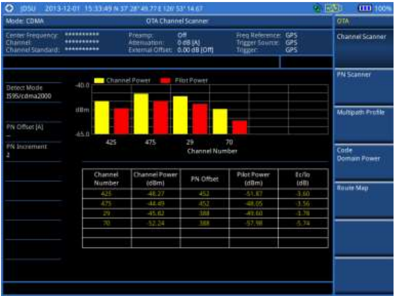
Figure 193 Channel scanner measurement with CDMA OTA signal analyzer
