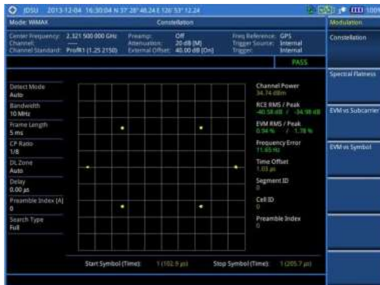
Figure 259 Constellation measurement with Mobile WiMAX signal analyzer
