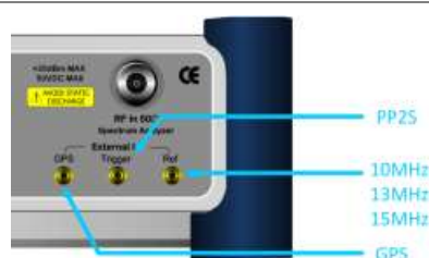
Figure 135 Connection ports for external reference clock
