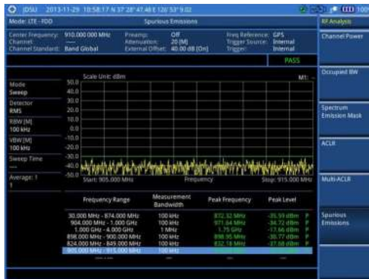
Figure 97 Spurious emissions measurement with LTE-FDD signal analyzer
