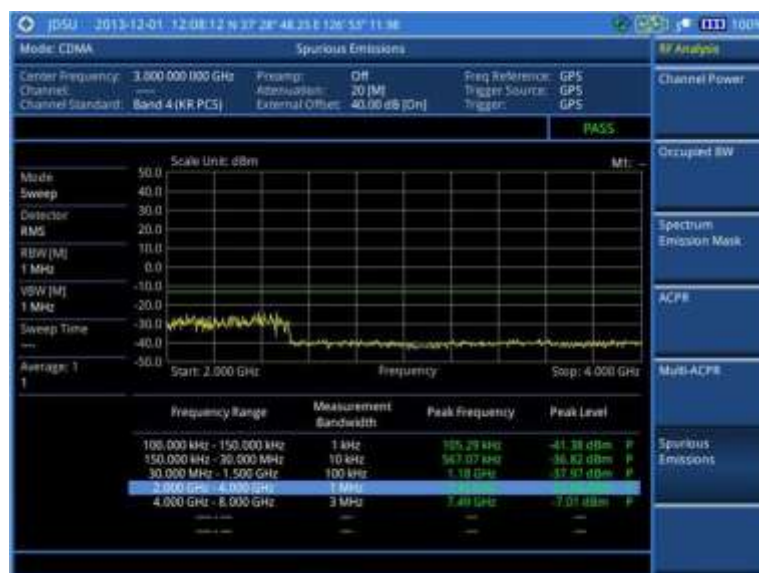
Figure 186 Spurious emissions measurement with CDMA signal analyzer
