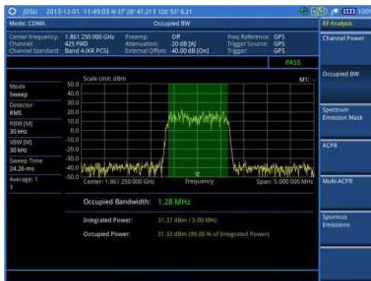
Figure 182 Occupied bandwidth measurement with CDMA signal analyzer
