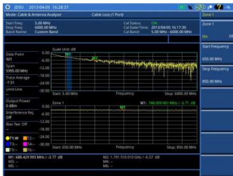
Figure 283 Cable loss (1 port) measurement with the zone enabled
