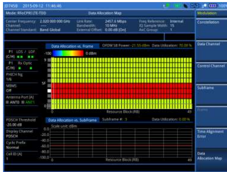
Figure 334 Data allocation map measurement with RFoCPRI LTE-TDD signal analyzer
