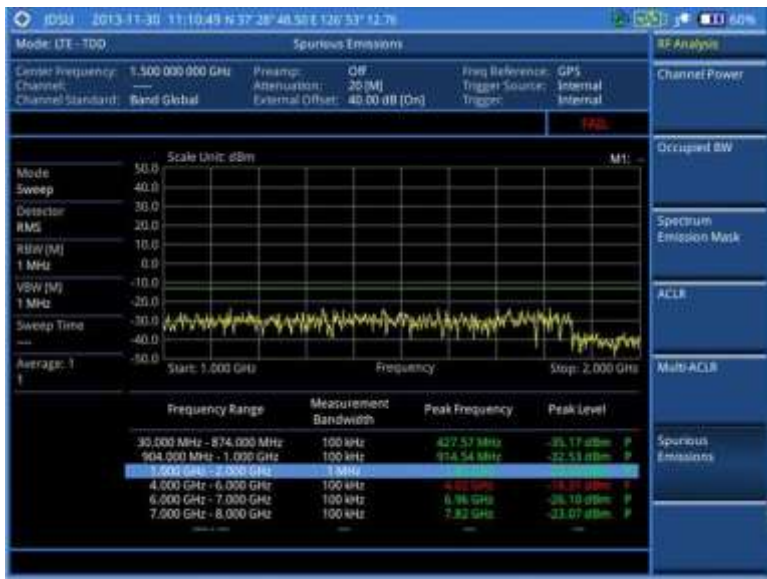
Figure 142 Spurious emissions measurement with LTE-TDD signal analyzer
