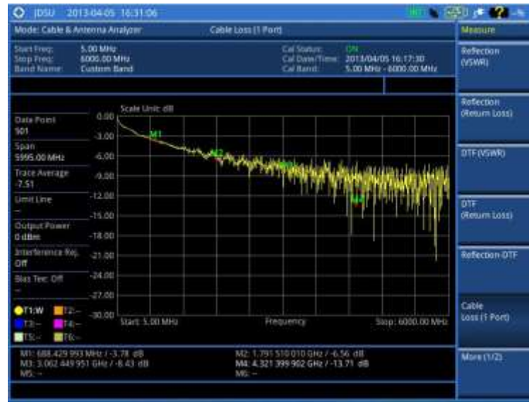
Figure 282 Cable loss (1 port) measurement
