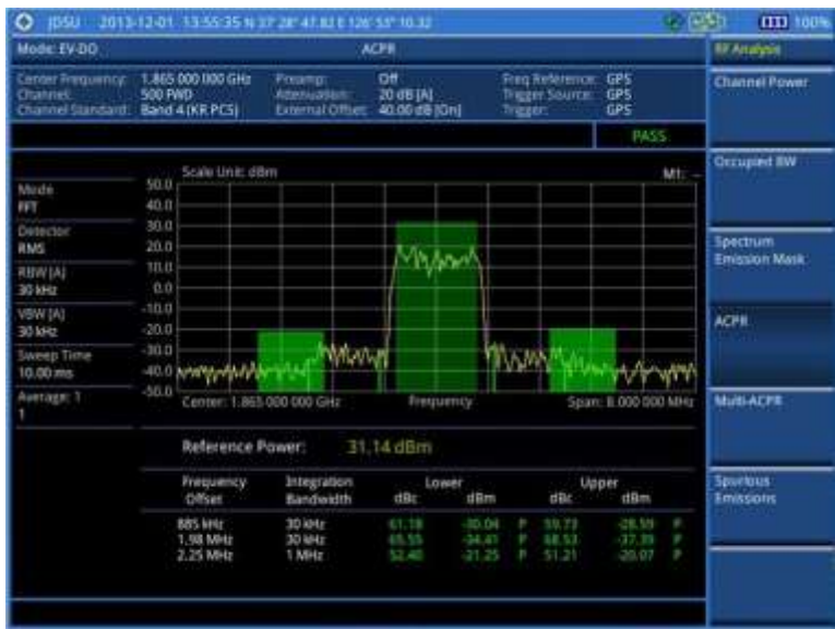
Figure 207 ACPR measurement with EV-DO signal analyzer
