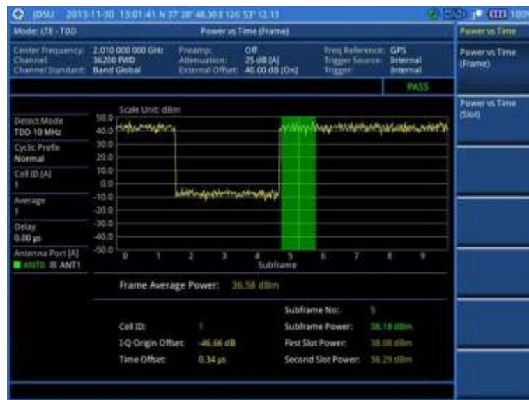
Figure 144 Power vs. time (frame) measurement with LTE – TDD signal analyzer
