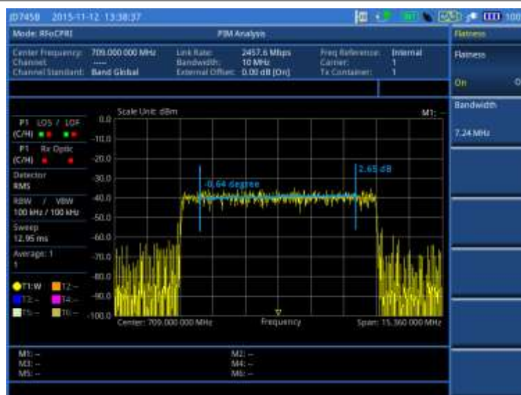
Figure 353 Example of PIM analysis in BBU emulation
