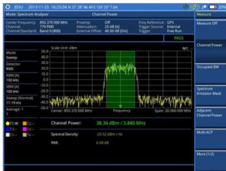
Figure 16 Channel power measurement with spectrum analyzer
