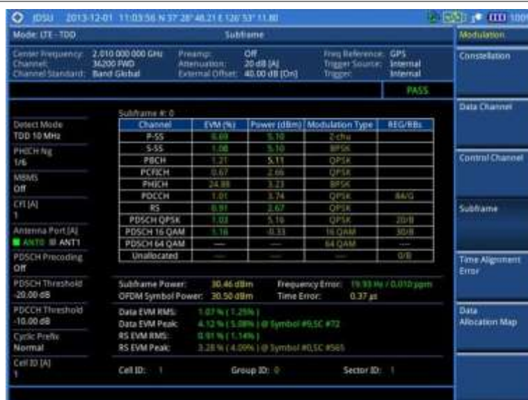
Figure 151 Subframe measurement with LTE-TDD signal analyzer
