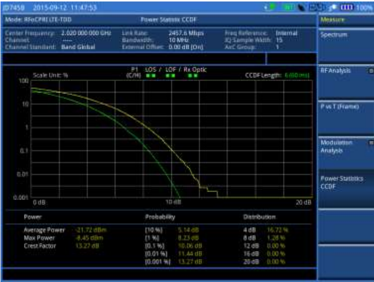
Figure 335 CCDF measurement with RFoCPRI LTE-TDD signal analyzer
