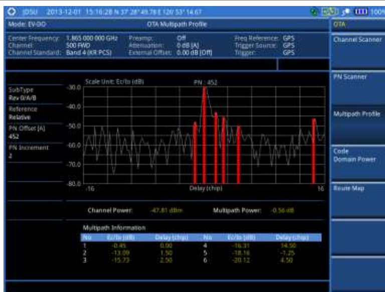
Figure 220 Multipath profile measurement with EV-DO OTA signal analyzer
