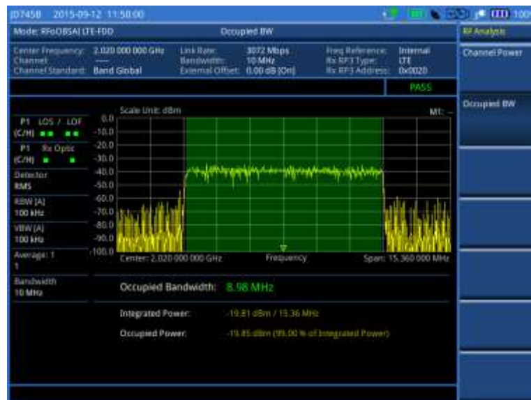
Figure 370 Occupied bandwidth measurement with RFoBSAI LTE-FDD signal analyzer
