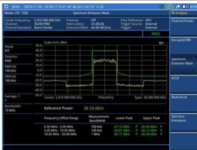
Figure 139 SEM measurement with LTE-TDD signal analyzer
