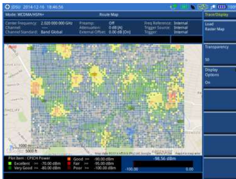
Figure 85 Raster image overlaid on the base map in WCDMA/HSPA+ OTA signal analyzer
