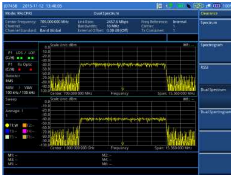
Figure 348 Example of dual spectrum analysis in BBU emulation
