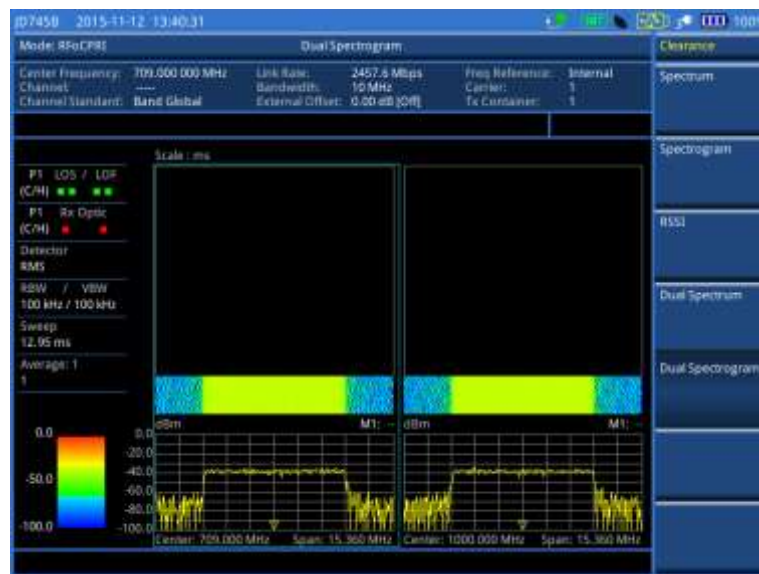
Figure 350 Example of dual spectrogram analysis in BBU emulation
