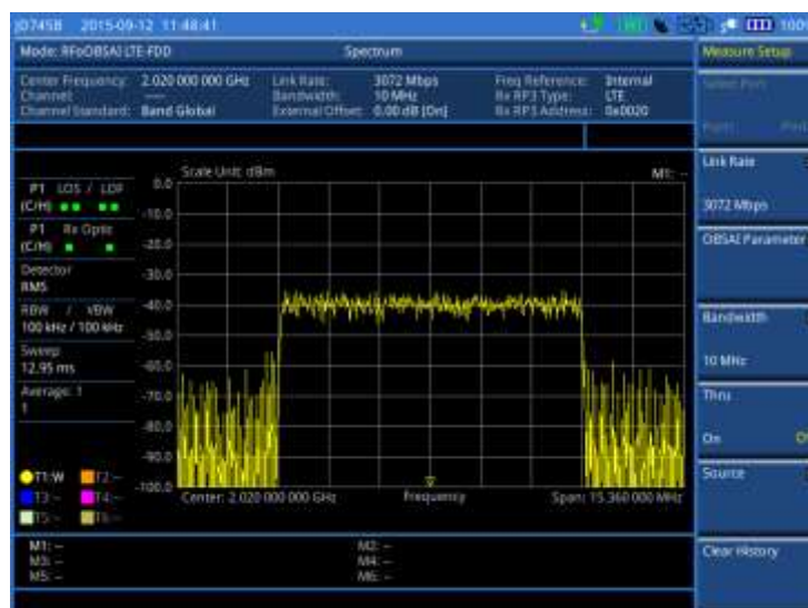
Figure 368 Spectrum measurement with RFoBSAI LTE-FDD signal analyzer
