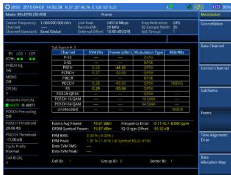
Figure 320 Frame measurement with RFoCPRI LTE-FDD signal analyzer
