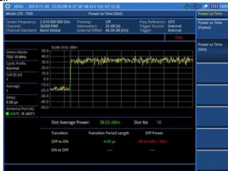
Figure 143 Power vs. time (slot) measurement with LTE – TDD signal analyzer
