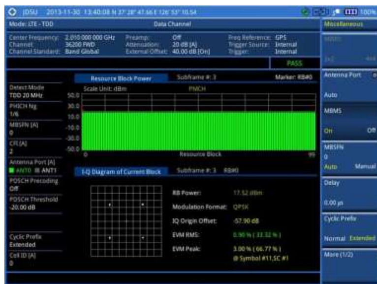
Figure 148 Data channel measurement with LTE-TDD signal analyzer (MBMS On)
