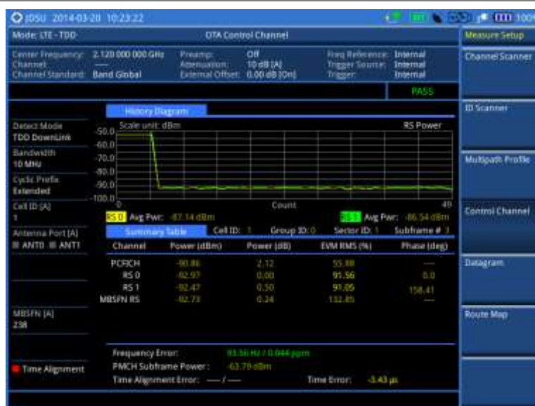
Figure 164 Control channel measurement with LTE-TDD OTA signal analyzer
