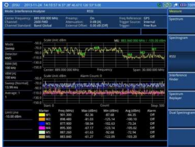
Figure 36 Interference measurement in RSSI
