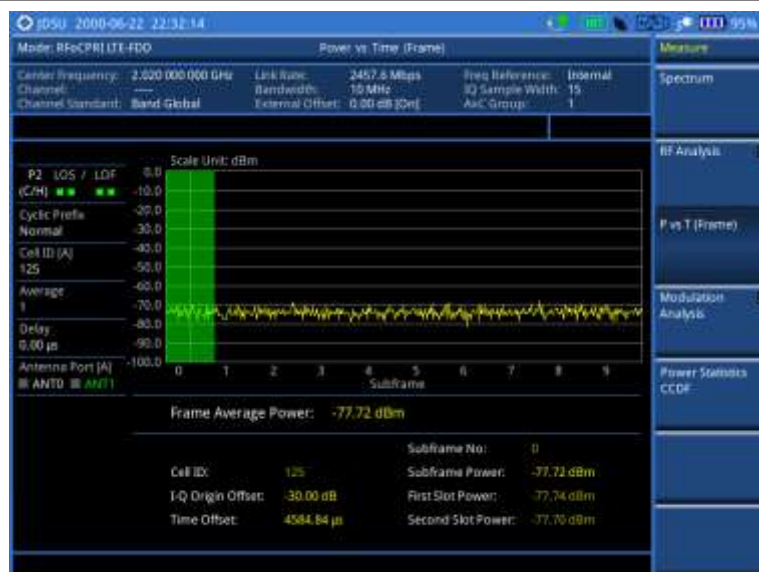
Figure 315 Power vs. time (frame) measurement with RFoCPRI LTE-FDD signal analyzer
