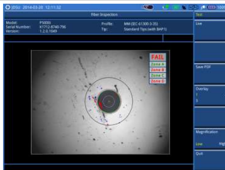
Figure 397 Analyzed fiber image and fiber inspection result
