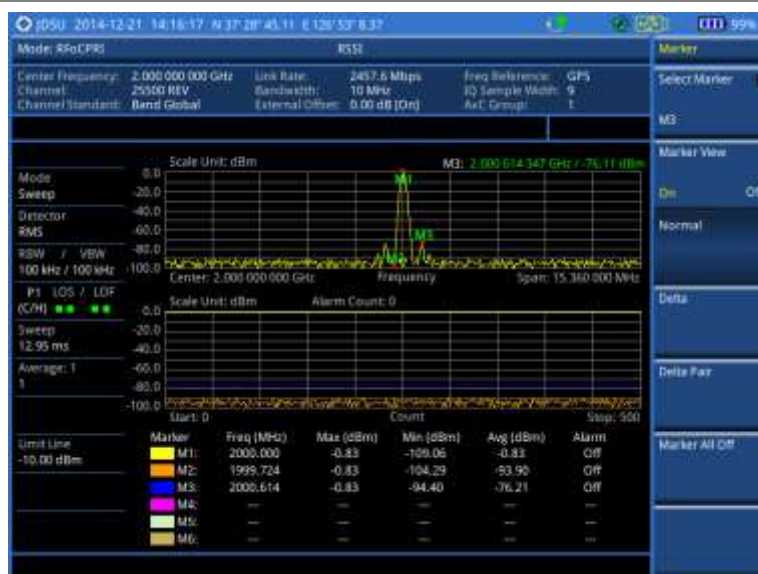
Figure 305 RFoCPRI interference measurement in RSSI
