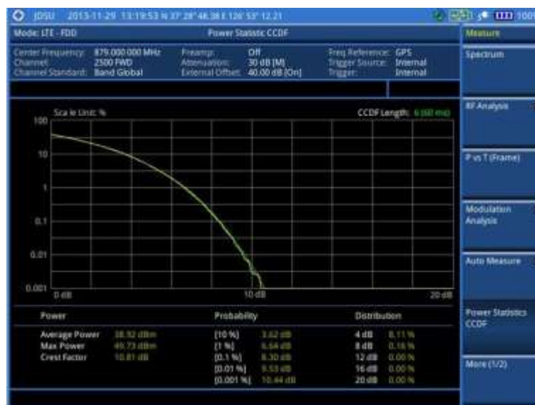
Figure 114 CCDF measurement with LTE-FDD signal analyzer
