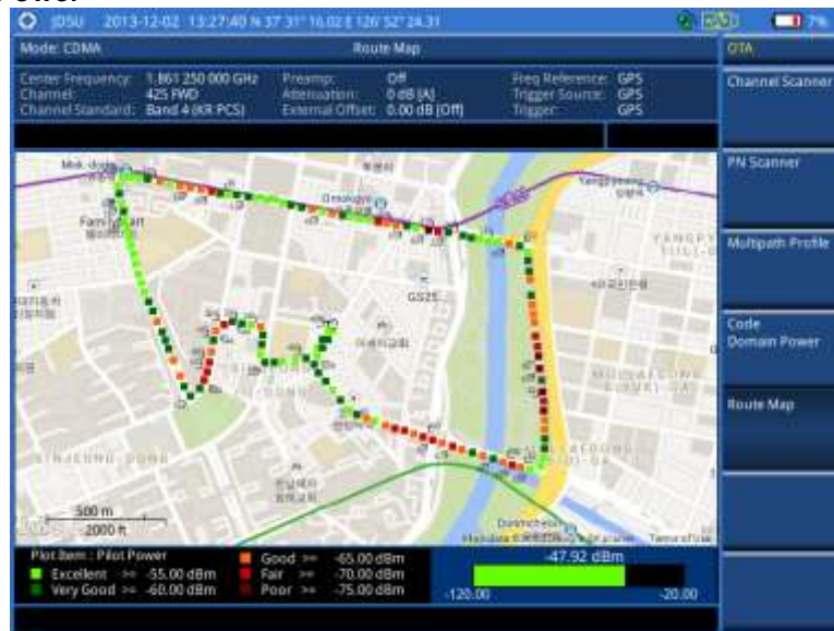
Figure 197 Route map measurement with CDMA OTA signal analyzer
