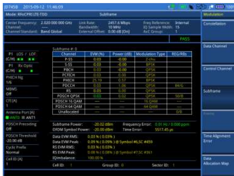
Figure 332 Subframe measurement (regular view) with RFoCPRI LTE-TDD signal analyzer
