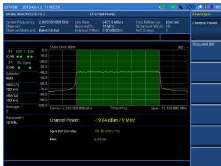
Figure 326 Channel power measurement with RFoCPRI LTE-TDD signal analyzer
