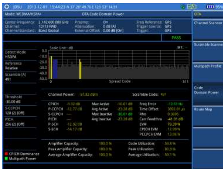
Figure 82 Code domain power measurement with WCDMA/HSPA+ OTA signal analyzer
