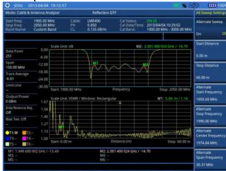
Figure 281 Reflection-DTF dual measurement
