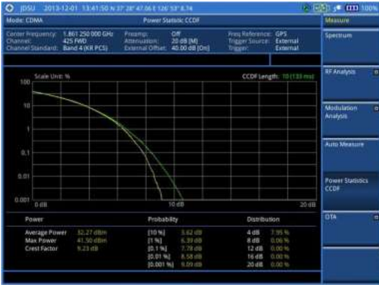
Figure 192 CCDF measurement with CDMA signal analyzer
