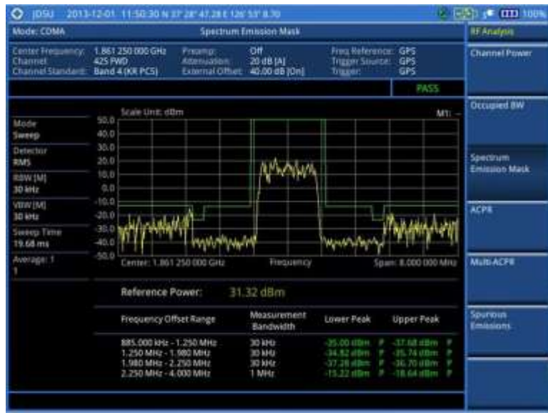
Figure 183 SEM measurement with CDMA signal analyzer
