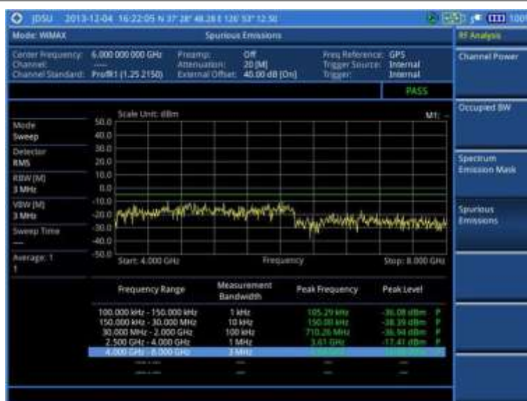
Figure 257 Spurious emissions measurement with Mobile WiMAX signal analyzer
