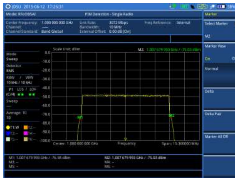
Figure 366 PIM detection of single radio
