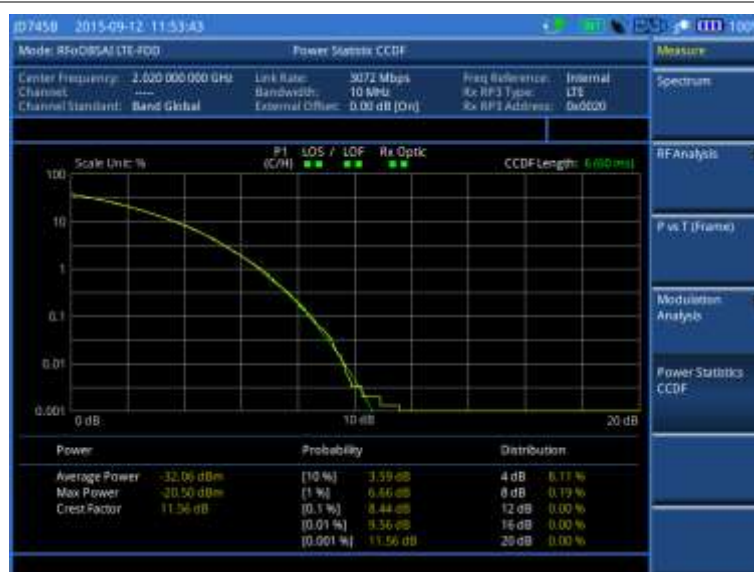
Figure 379 CCDF measurement with RFoBSAI LTE-FDD signal analyzer
