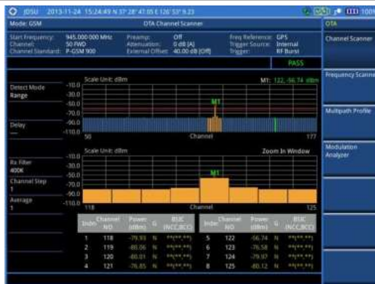
Figure 56 Channel scanner measurement with GSM OTA signal analyzer
