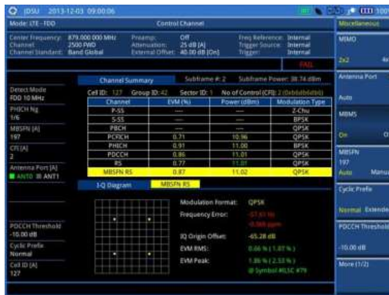
Figure 104 Control channel measurement with LTE-FDD signal analyzer (MBMS On)
