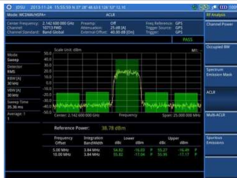
Figure 69 ACLR measurement with WCDMA/HSPA+ signal analyzer
