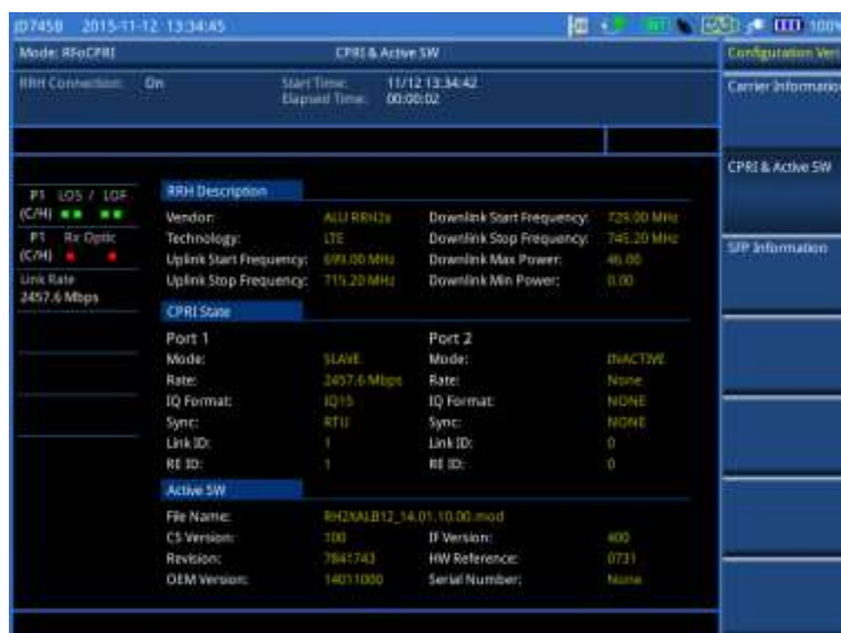
Figure 343 Example of verification of CPRI state and active software
