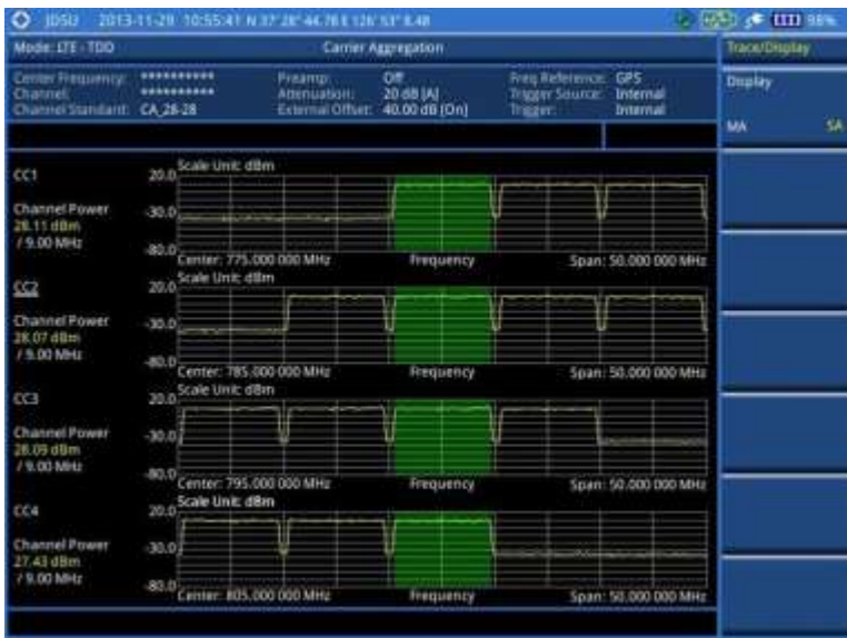
Figure 160 Carrier aggregation measurement with LTE-TDD signal analyzer (SA)
