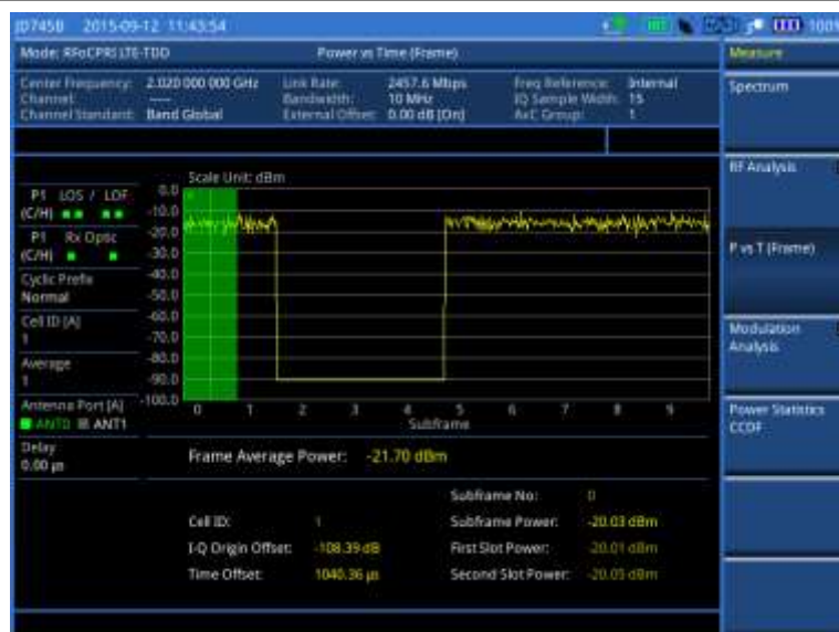
Figure 328 Power vs. time (frame) measurement with RFoCPRI LTE-TDD signal analyzer
