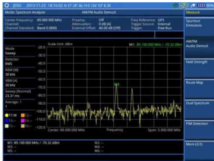
Figure 22 AM/FM audio demodulation with spectrum analyzer
