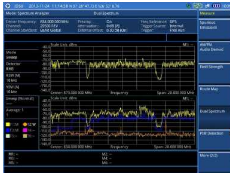
Figure 26 Dual spectrum measurement with spectrum analyzer
