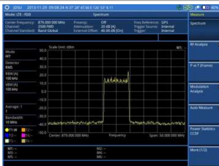
Figure 91 Spectrum measurement screen with LTE-FDD signal analyzer
