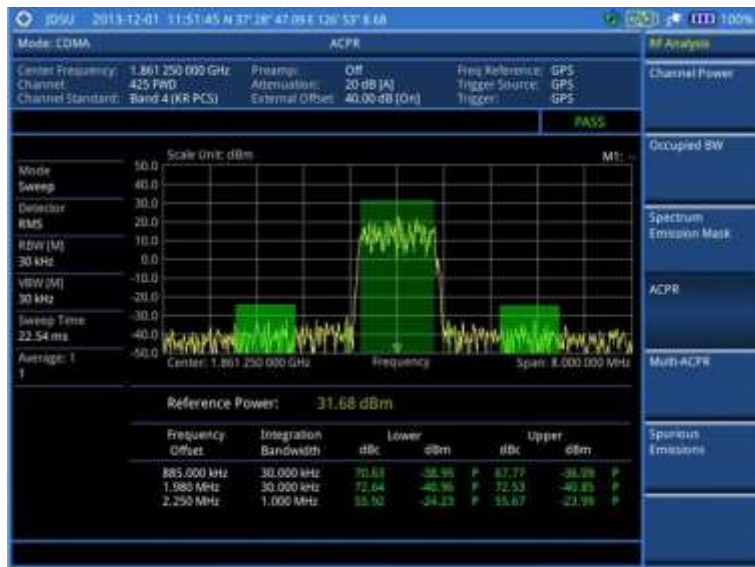
Figure 184 ACPR measurement with CDMA signal analyzer
