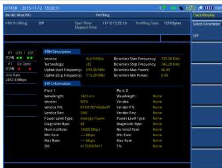
Figure 340 Example of RRH profiling results with SFP information
