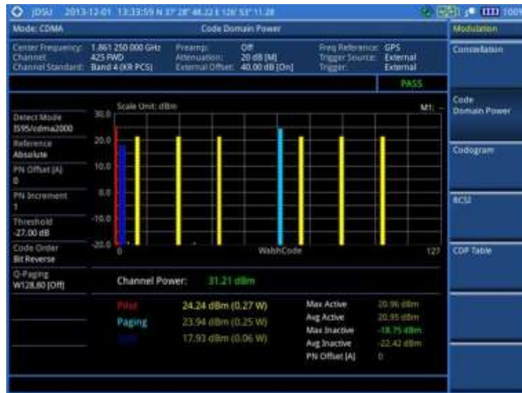
Figure 188 Code domain power measurement with CDMA signal analyzer
