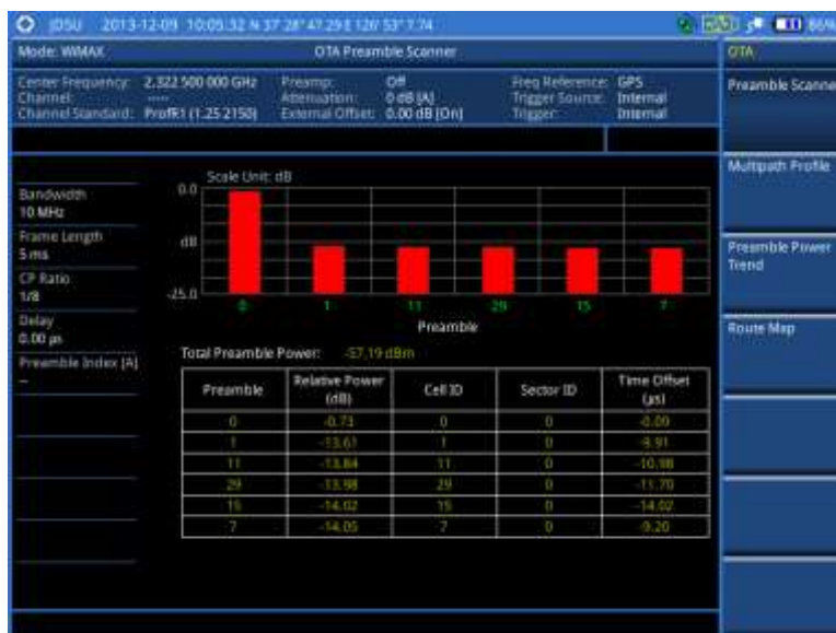
Figure 264 Preamble scanner measurement with Mobile WiMAX OTA signal analyzer
