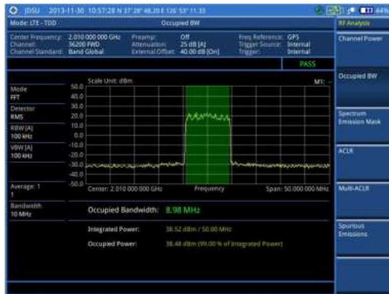
Figure 138 Occupied bandwidth measurement with LTE-TDD signal analyzer
