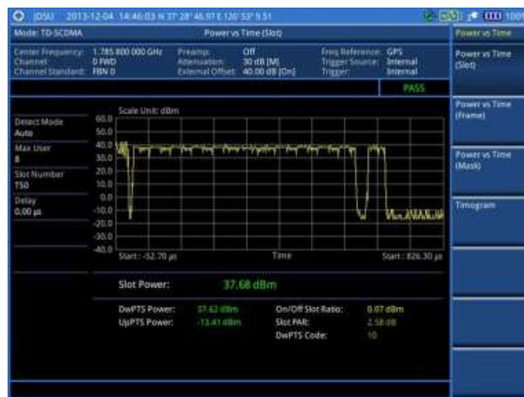
Figure 235 Power vs. time (slot) measurement with TD-SCDMA signal analyzer
