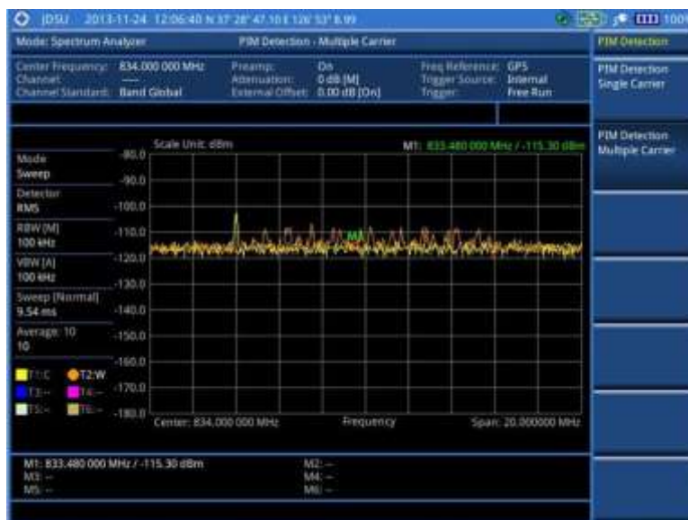
Figure 28 PIM detection for multiple carriers
