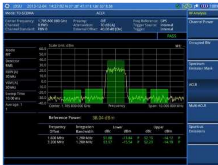
Figure 232 ACLR measurement with TD-SCDMA signal analyzer
