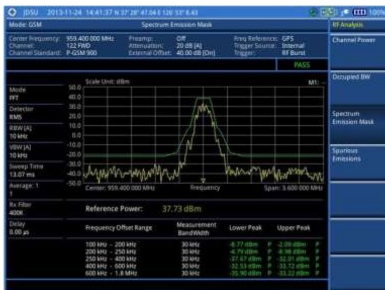
Figure 48 SEM measurement with GSM signal analyzer
