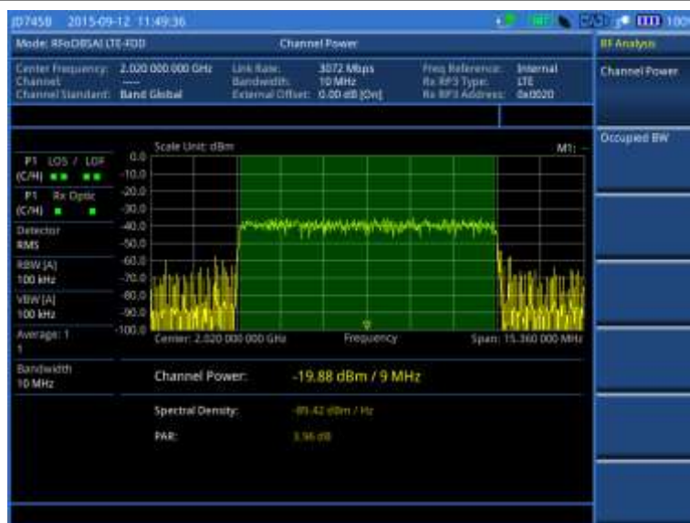
Figure 369 Channel power measurement with RFoBSAI LTE-FDD signal analyzer
