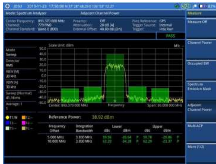
Figure 19 Adjacent channel power measurement with spectrum analyzer
