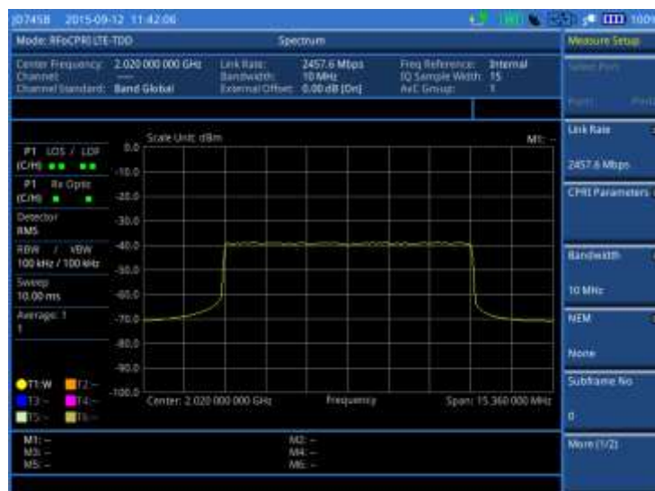
Figure 325 Spectrum measurement with RFoCPRI LTE-TDD signal analyzer
