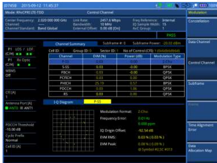
Figure 331 Control channel measurement with RFoCPRI LTE-TDD signal analyzer
