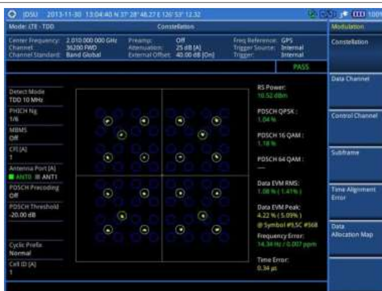
Figure 145 Constellation measurement with LTE-TDD signal analyzer
