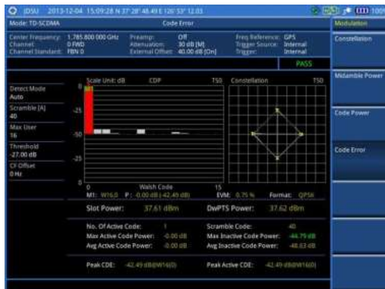
Figure 242 Code error measurement with TD-SCDMA signal analyzer
