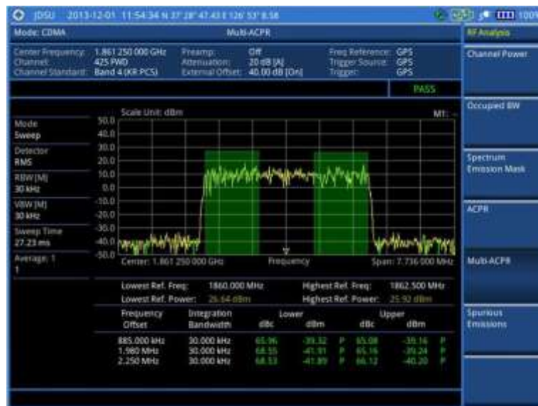
Figure 185 Multi-ACPR measurement with CDMA signal analyzer
