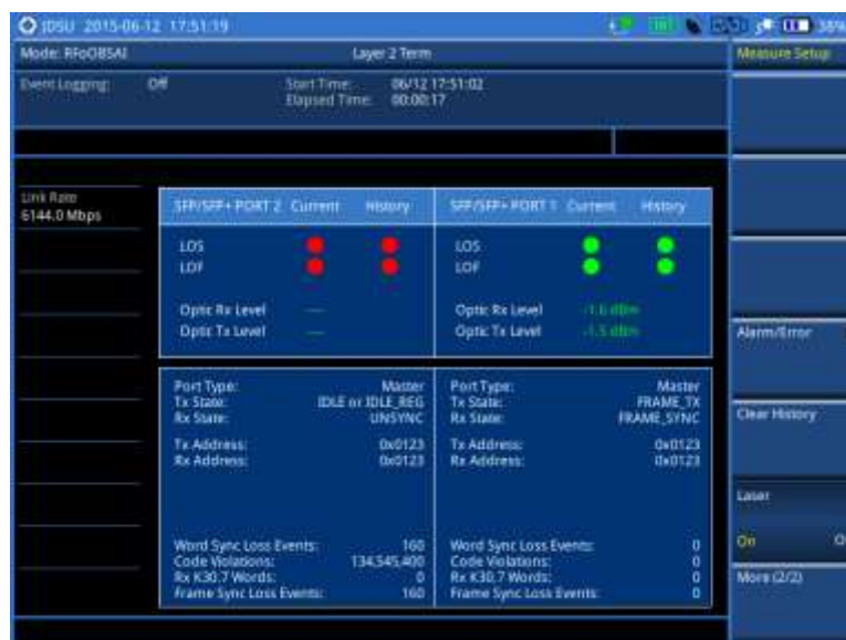
Figure 359 OBSAI layer 2 term test
