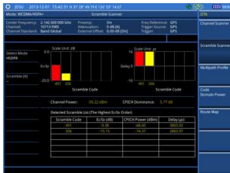
Figure 80 Scramble scanner measurement with WCDMA/HSPA+ OTA signal analyzer
