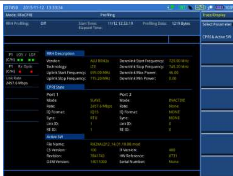
Figure 339 Example of RRH profiling results with CPRI state and activated SW
