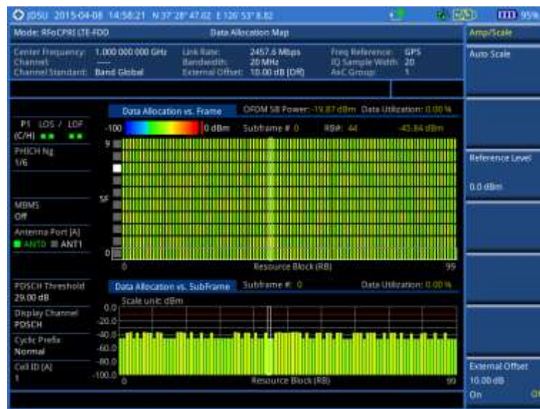
Figure 322 Data allocation map measurement with RFoCPRI LTE-FDD signal analyzer
