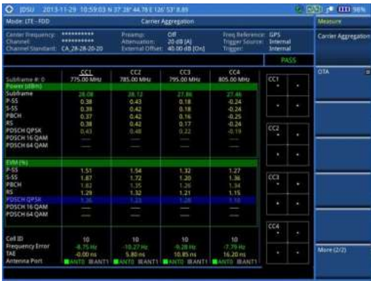
Figure 116 Carrier aggregation measurement with LTE-FDD signal analyzer (SA)
