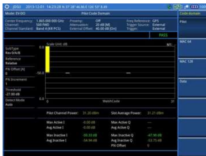
Figure 213 Code domain power measurement with EV-DO signal analyzer
