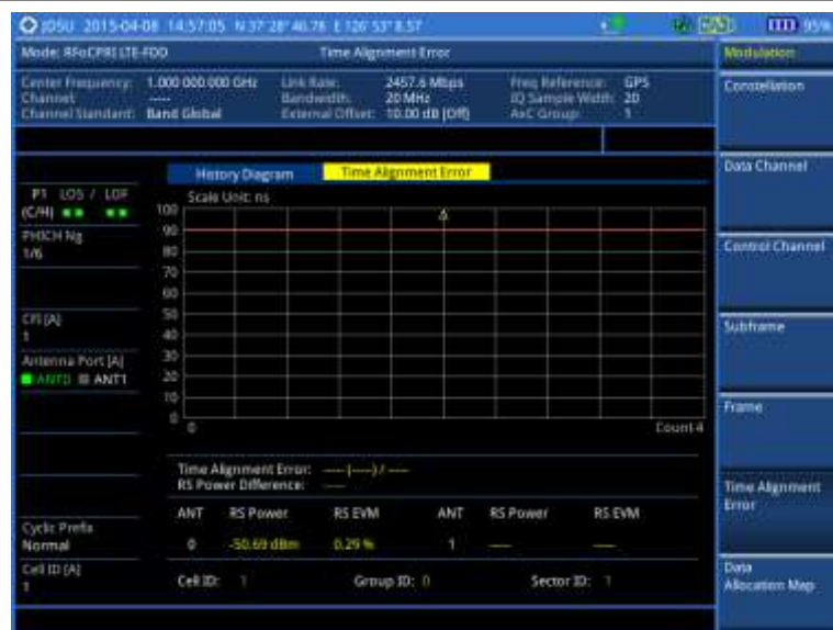
Figure 321 Time alignment error measurement with RFoCPRI LTE-FDD signal analyzer
