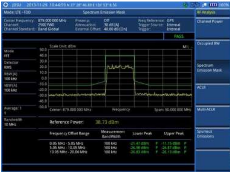
Figure 94 SEM measurement with LTE-FDD signal analyzer
