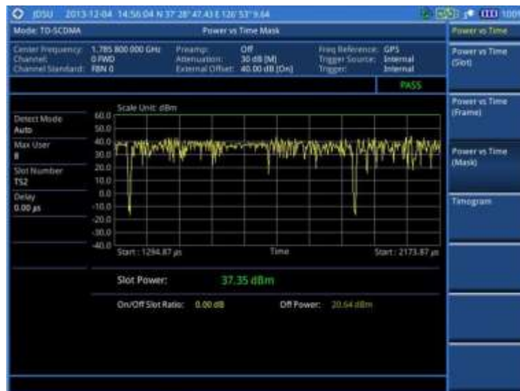
Figure 237 Power vs. time (mask) measurement with TD-SCDMA signal analyzer
