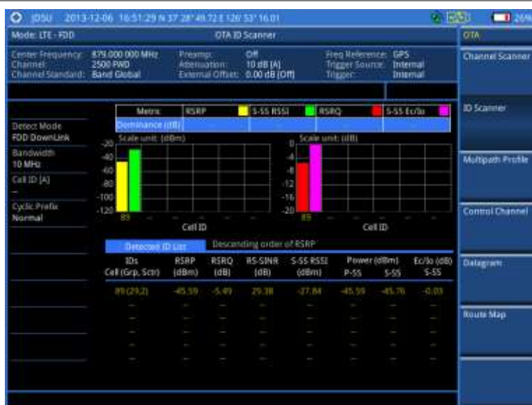
Figure 118 ID scanner measurement with LTE-FDD OTA signal analyzer
