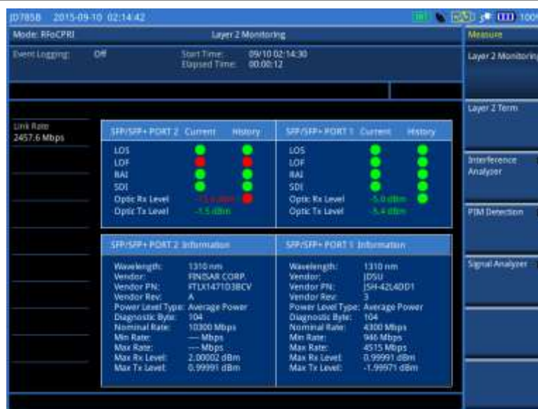
Figure 291 CPRI layer 2 monitoring
