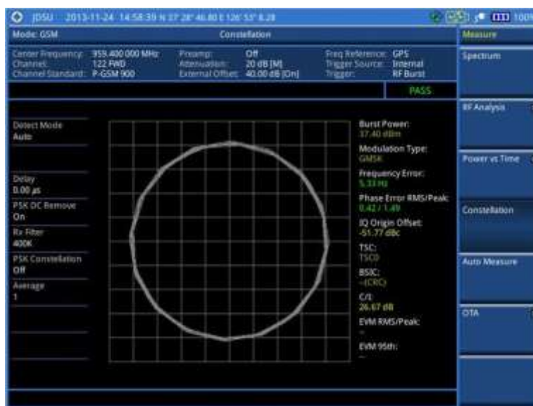
Figure 55 Constellation measurement (PSK on) with GSM signal analyzer
