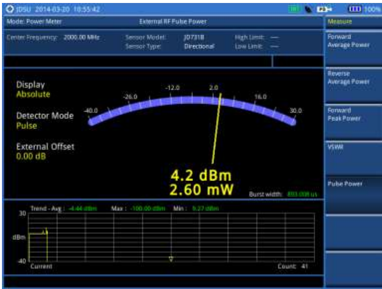
Figure 392 External power measurement of pulse power
