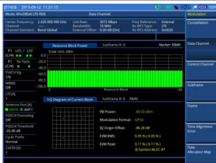
Figure 373 Data channel measurement with RFoBSAI LTE-FDD signal analyzer
