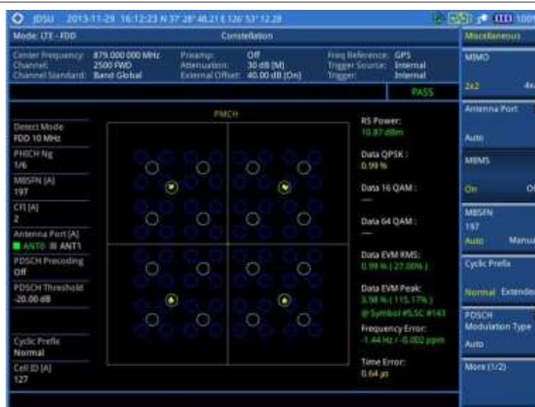
Figure 100 Constellation measurement with LTE-FDD signal analyzer (MBMS On)
