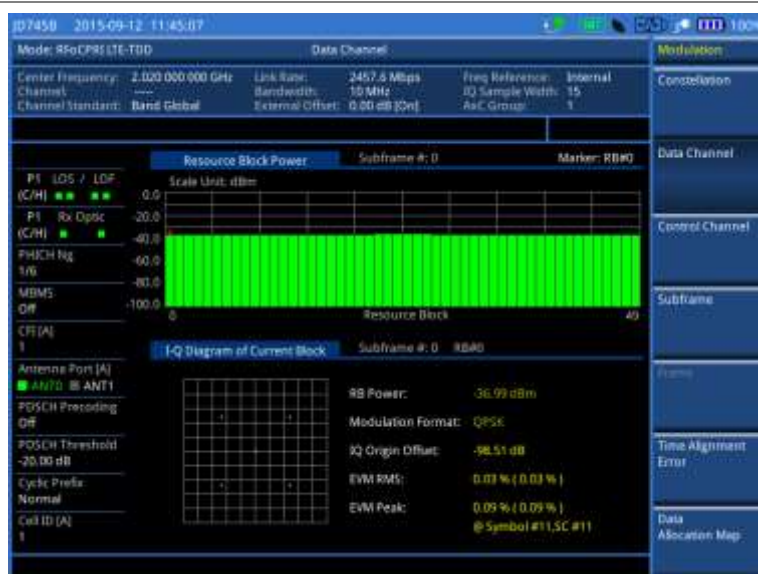
Figure 330 Data channel measurement with RFoCPRI LTE-FDD signal analyzer
