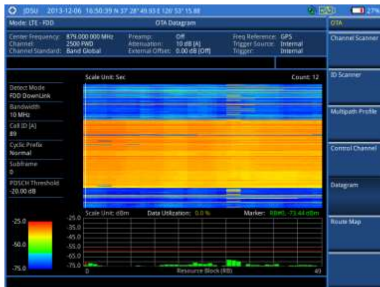
Figure 121 Datagram measurement with LTE-FDD signal analyzer
