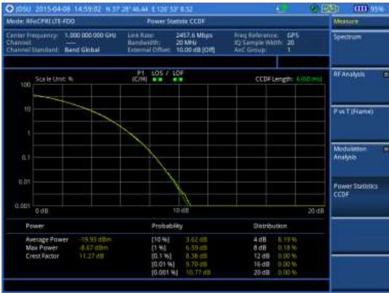
Figure 323 CCDF measurement with RFoCPRI LTE-FDD signal analyzer
