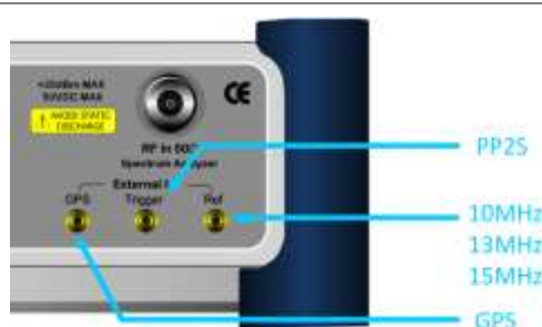
Figure 64 Connection ports for external reference clock
