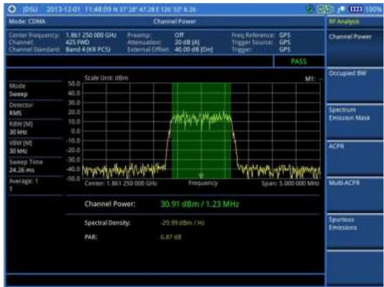
Figure 181 Channel power measurement with CDMA signal analyzer
