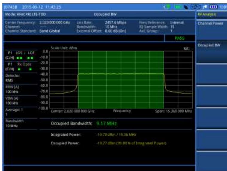
Figure 327 Occupied bandwidth measurement with RFoCPRI LTE-TDD signal analyzer
