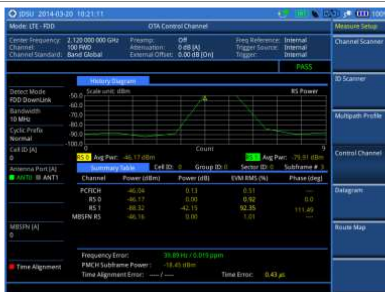
Figure 120 Control channel measurement with LTE-FDD OTA signal analyzer
