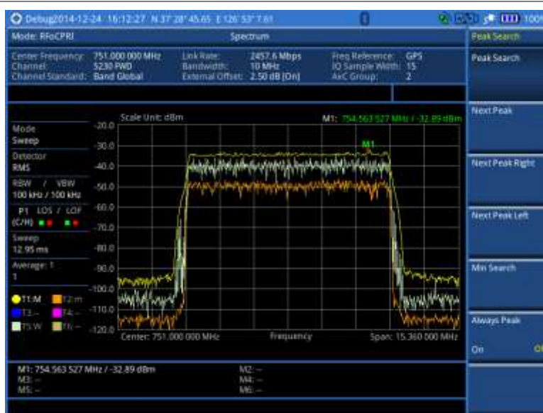
Figure 299 RFoCPRI spectrum analysis on LTE Uplink 10 MHz, antenna 2
