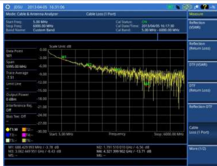
Figure 284 Cable loss (1 port) measurement
