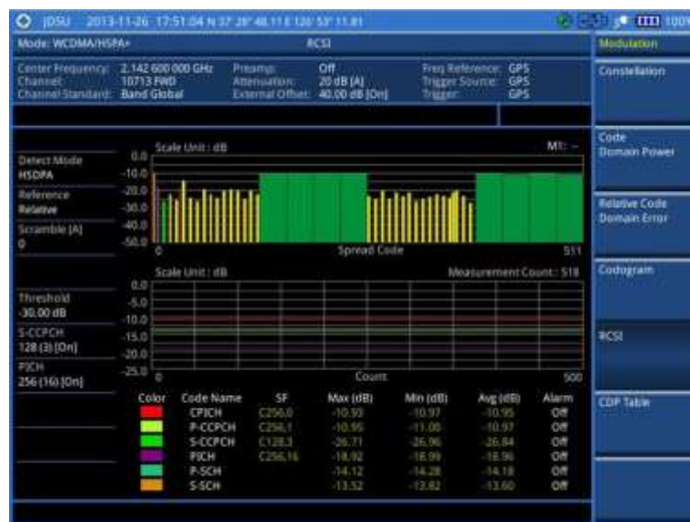
Figure 76 RCSI measurement with WCDMA/HSPA+ signal analyzer
