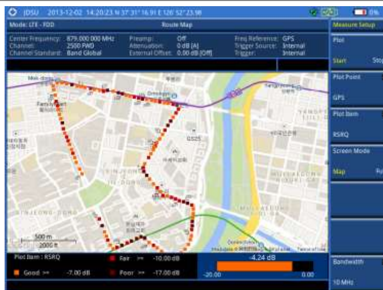
Figure 124 Route map measurement (RS-SINR) with LTE-FDD OTA signal analyzer
