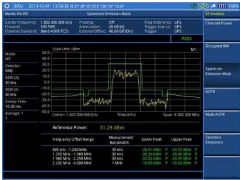
Figure 206 SEM measurement with EV-DO signal analyzer
