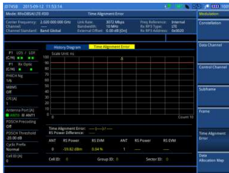
Figure 377 Time alignment error measurement with RFoBSAI LTE-FDD signal analyzer
