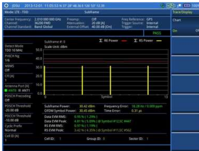
Figure 152 Subframe measurement with LTE-TDD signal analyzer (Chart On)
