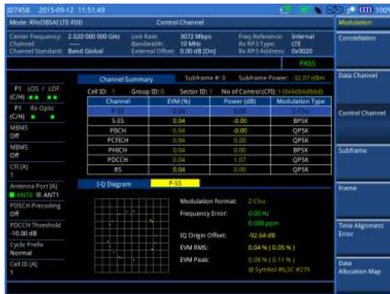
Figure 374 Control channel measurement with RFoBSAI LTE-FDD signal analyzer
