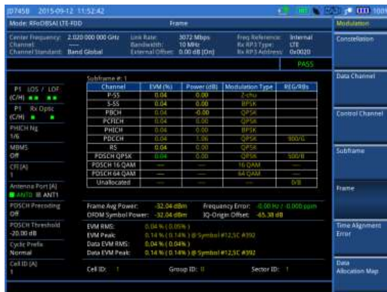
Figure 376 Frame measurement with RFoBSAI LTE-FDD signal analyzer
