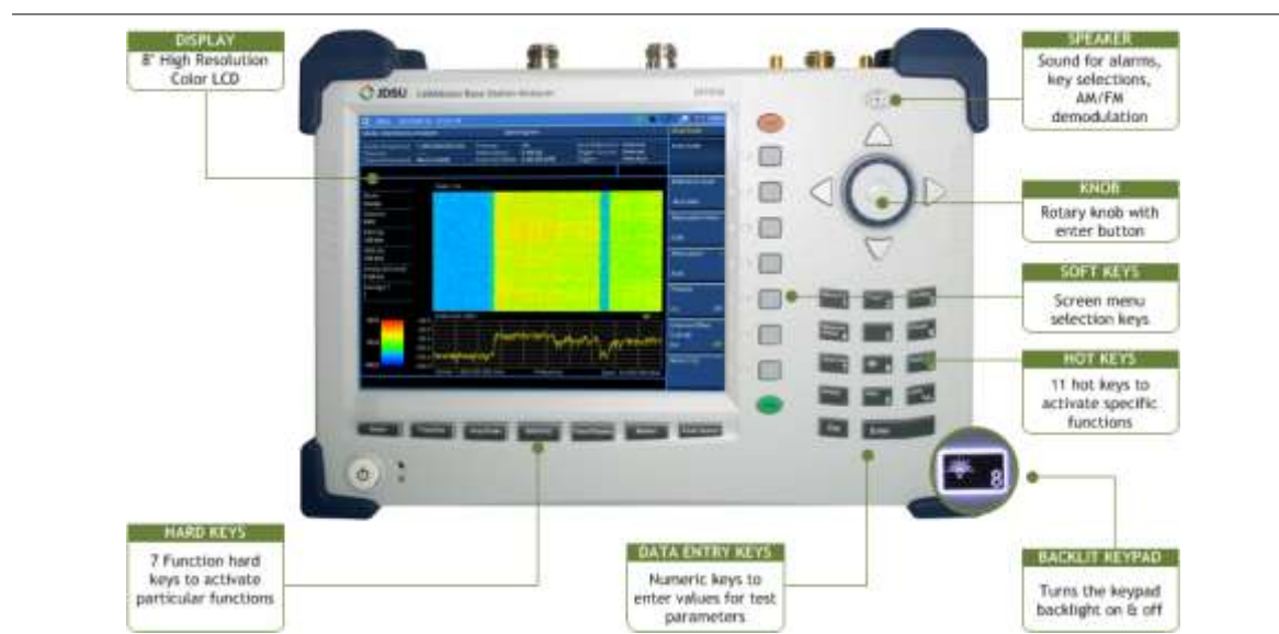
Figure 1 JD785B front panel view
