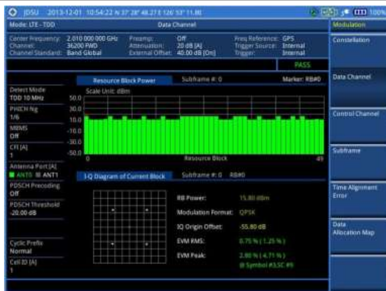
Figure 148 Data channel measurement with LTE-TDD signal analyzer (MBMS On)
