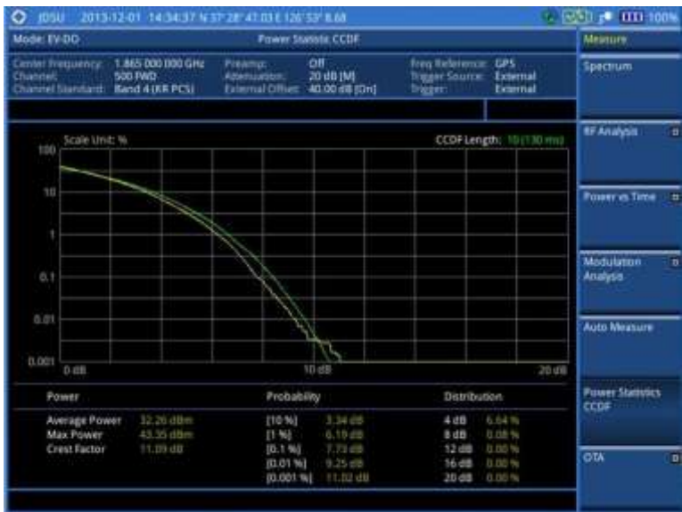
Figure 217 CCDF measurement with EV-DO signal analyzer
