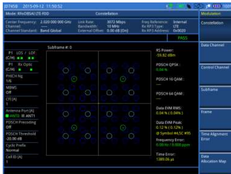
Figure 372 Constellation measurement with RFoBSAI LTE-FDD signal analyzer
