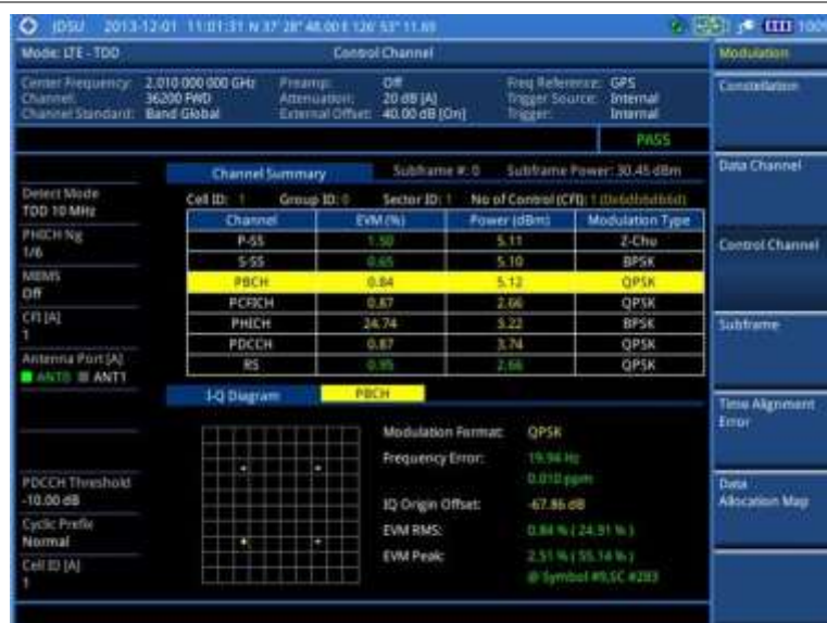
Figure 149 Control channel measurement with LTE-TDD signal analyzer
