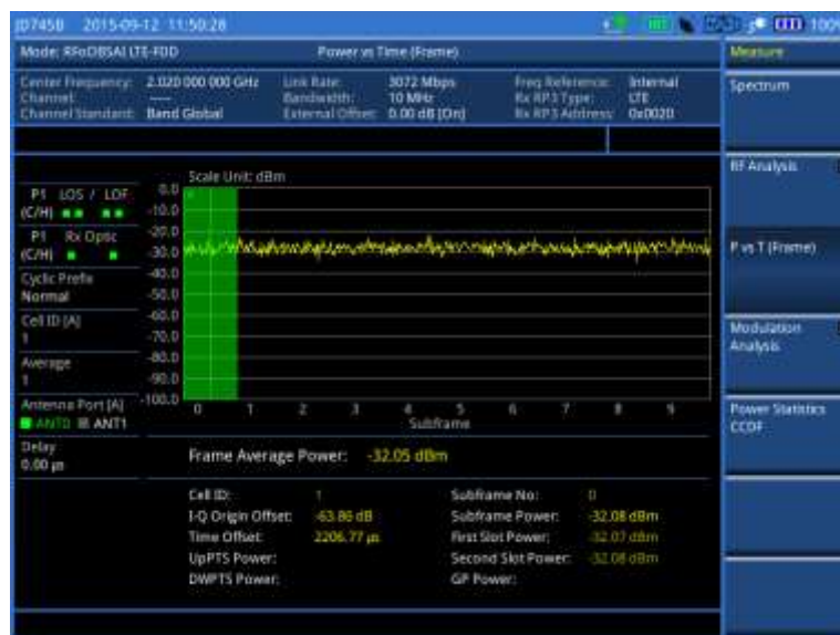
Figure 371 Power vs. time (frame) measurement with RFoOBSAI LTE-FDD signal analyzer
