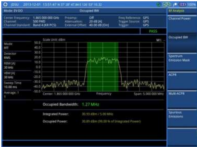
Figure 205 Occupied bandwidth measurement with EV-DO signal analyzer
