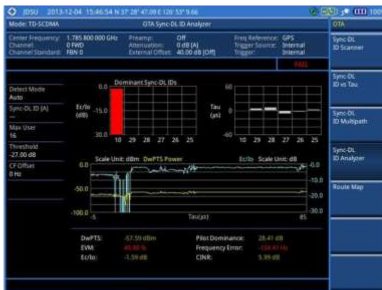
Figure 246 Sync-DL ID analyzer measurement with TD-SCDMA OTA signal analyzer
