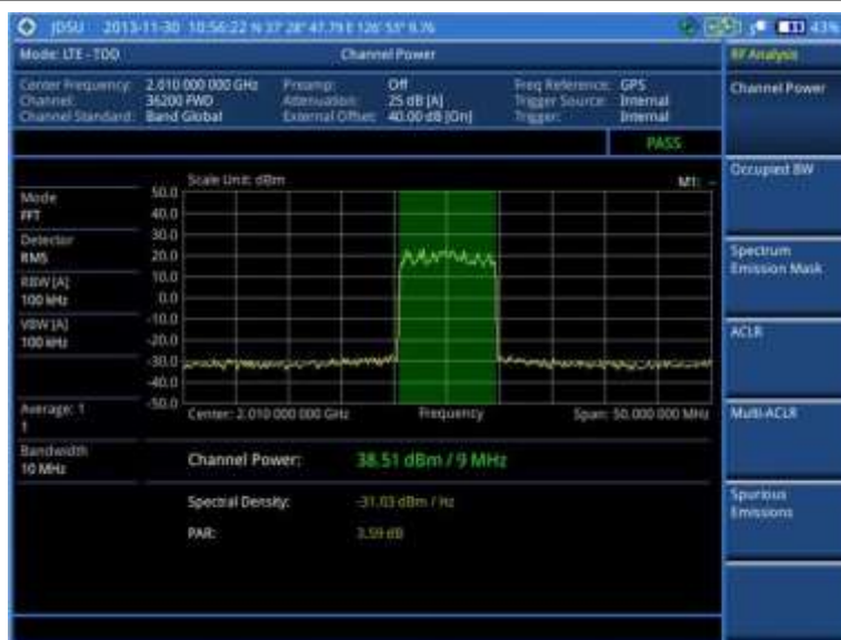
Figure 137 Channel power measurement with LTE-TDD signal analyzer
