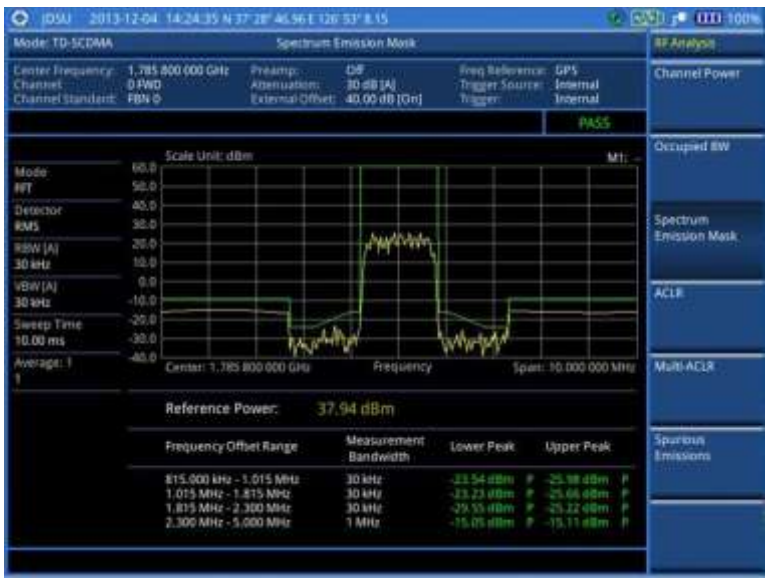
Figure 231 SEM measurement with TD-SCDMA signal analyzer
