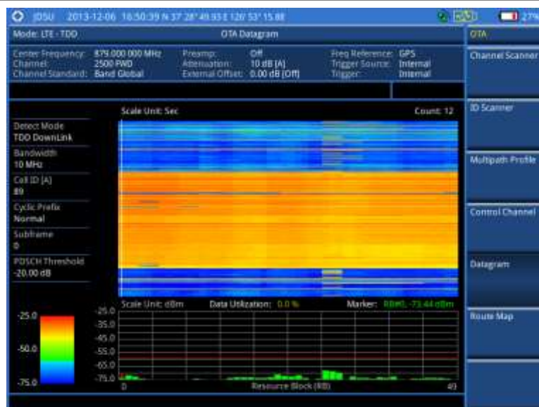
Figure 165 Datagram measurement with LTE-TDD signal analyzer
