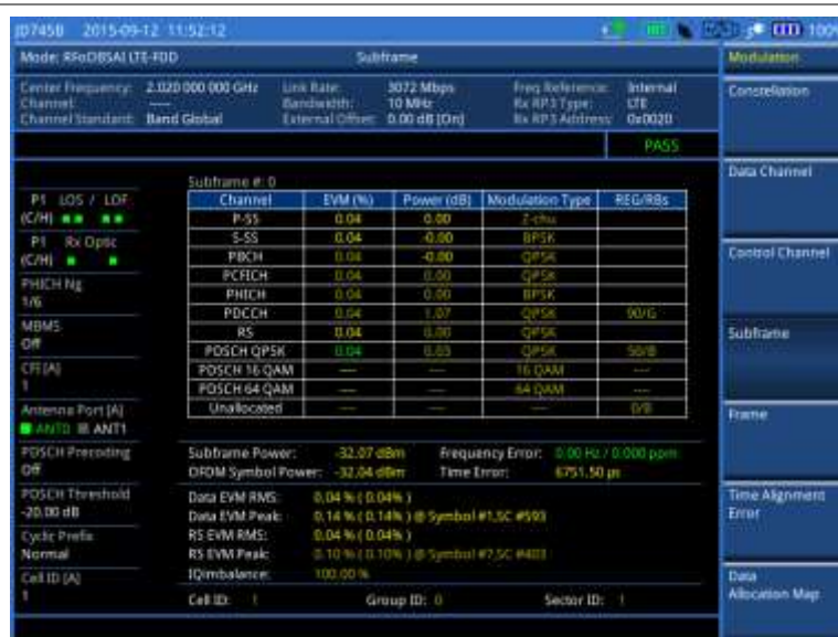
Figure 375 Subframe measurement with RFoBSAI LTE-FDD signal analyzer
