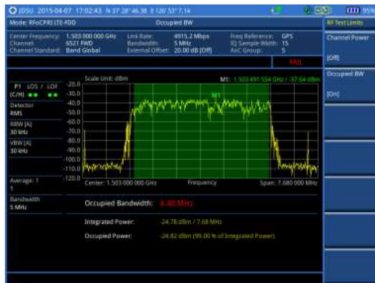
Figure 314 Occupied bandwidth measurement with RFoCPRI LTE-FDD signal analyzer
