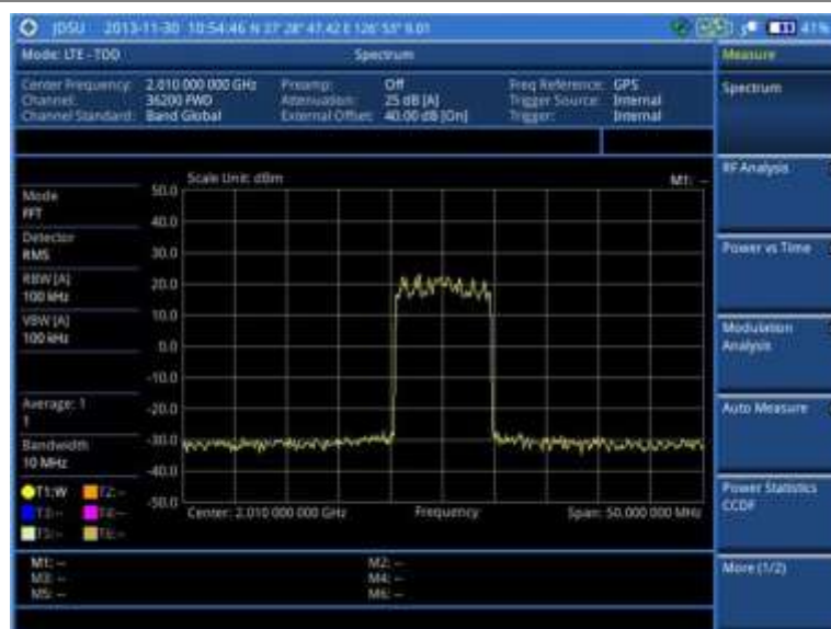
Figure 136 Spectrum measurement screen with LTE-TDD signal analyzer
