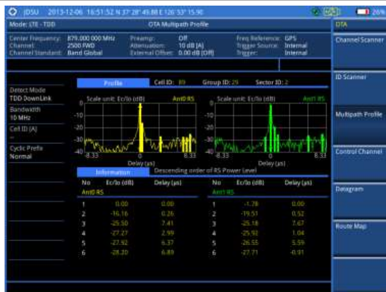
Figure 163 Multipath profile measurement with LTE-TDD OTA signal analyzer
