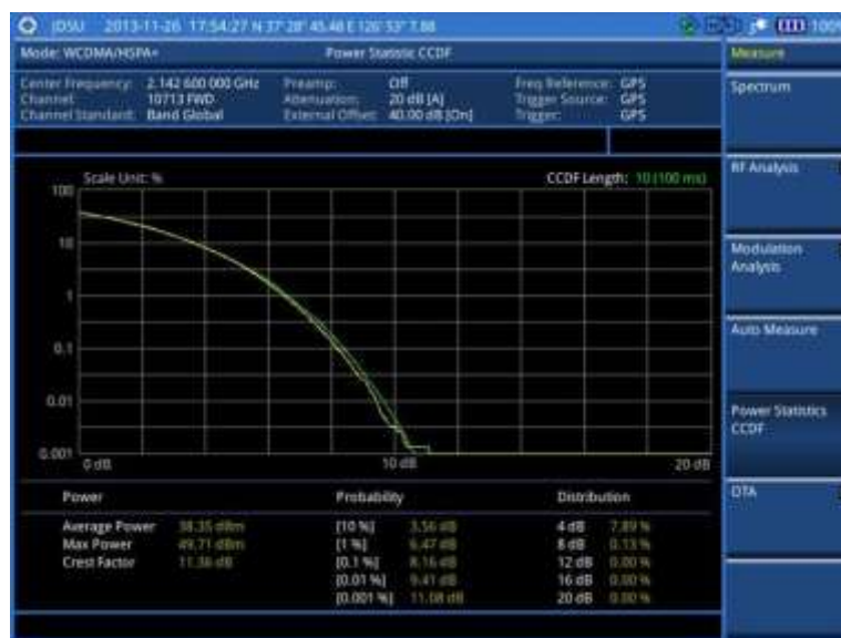
Figure 78 CCDF measurement with WCDMA/HSPA+ signal analyzer
