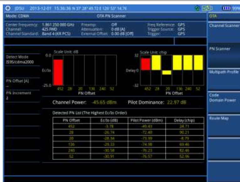
Figure 194 PN scanner measurement with CDMA OTA signal analyzer
