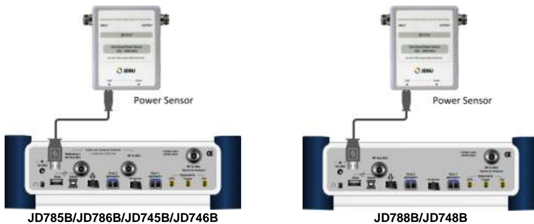
Figure 391 Directional power sensor connection
