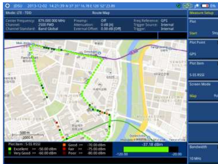
Figure 169 Route map measurement (S-SS RSSI) with LTE-TDD OTA signal analyzer
