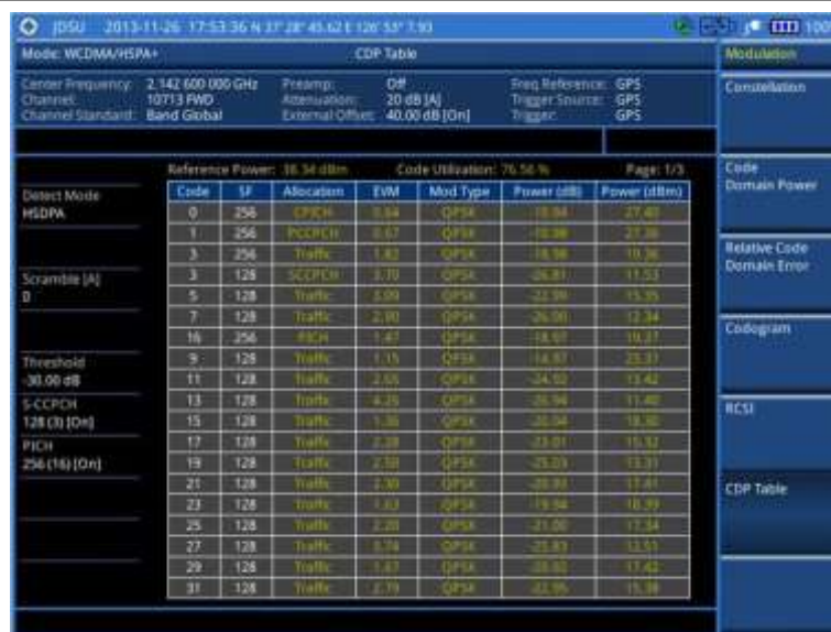
Figure 77 CDP Table measurement with WCDMA/HSPA+ signal analyzer
