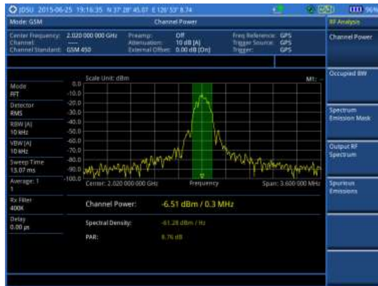
Figure 48 Channel power measurement with GSM signal analyzer
