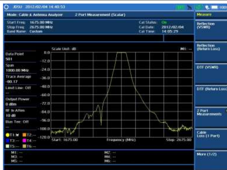
Figure 310 2-port scalar measurement
