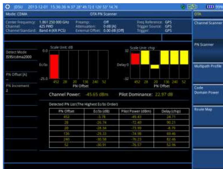
Figure 200 PN scanner measurement with CDMA OTA signal analyzer
