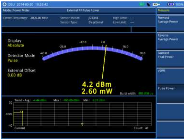
Figure 420 External power measurement of pulse power
