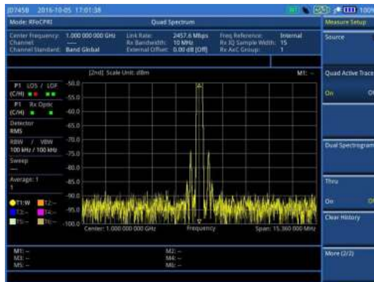
Figure 328 RFoCPRI quad spectrum with quad active trace off
