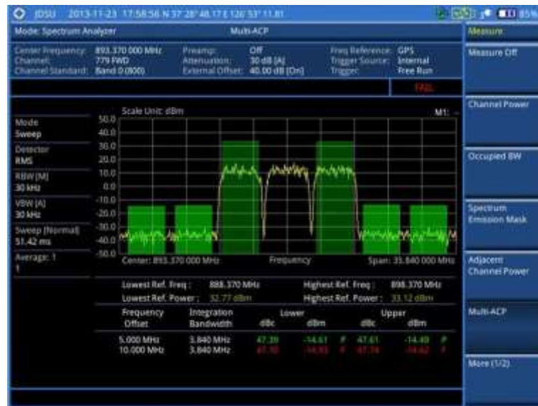
Figure 22 Multi-ACP measurement with spectrum analyzer
