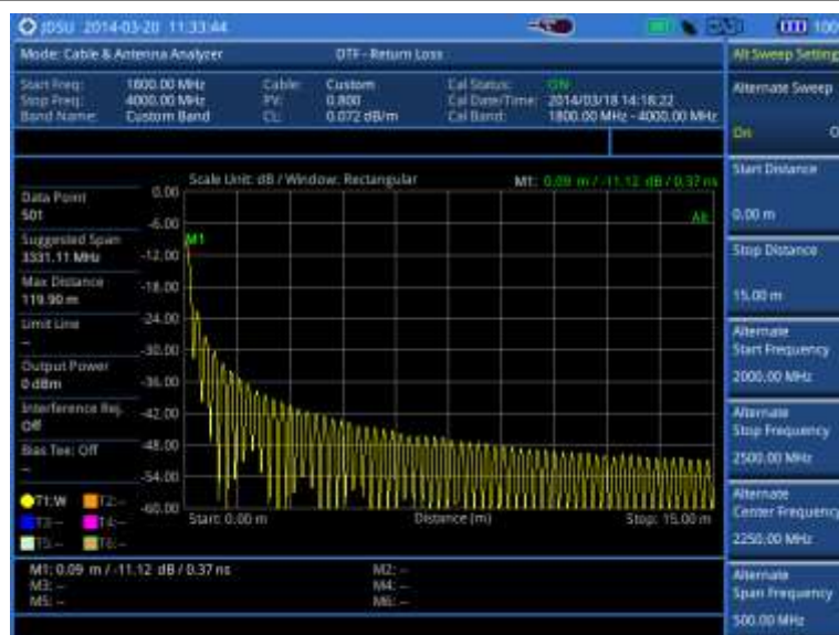
Figure 302 DTF measurement with the alternate sweep on
