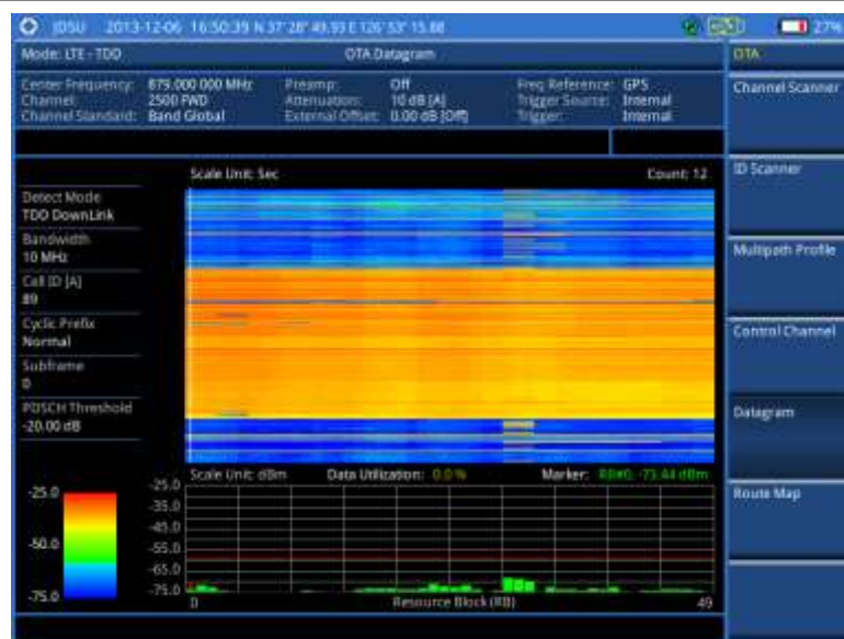
Figure 171 Datagram measurement with LTE-TDD signal analyzer
