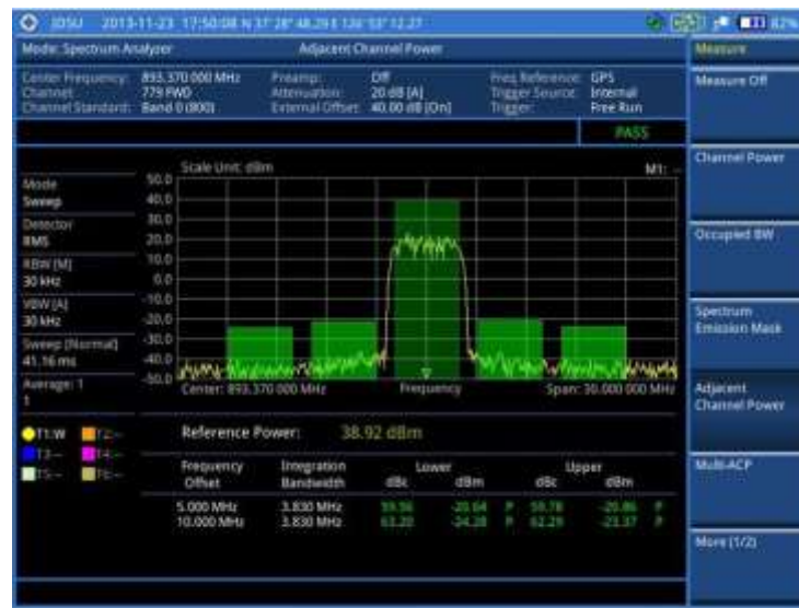
Figure 21 Adjacent channel power measurement with spectrum analyzer
