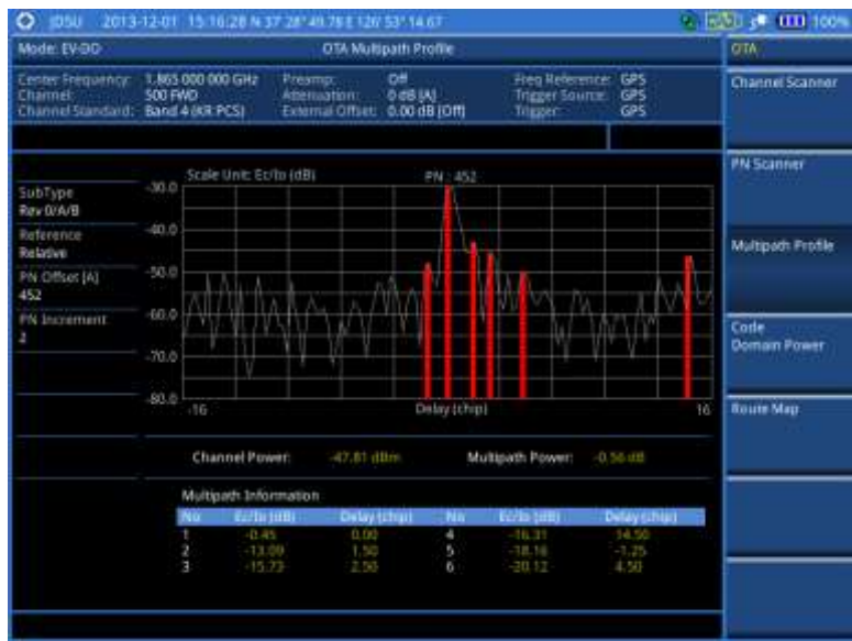
Figure 226 Multipath profile measurement with EV-DO OTA signal analyzer
