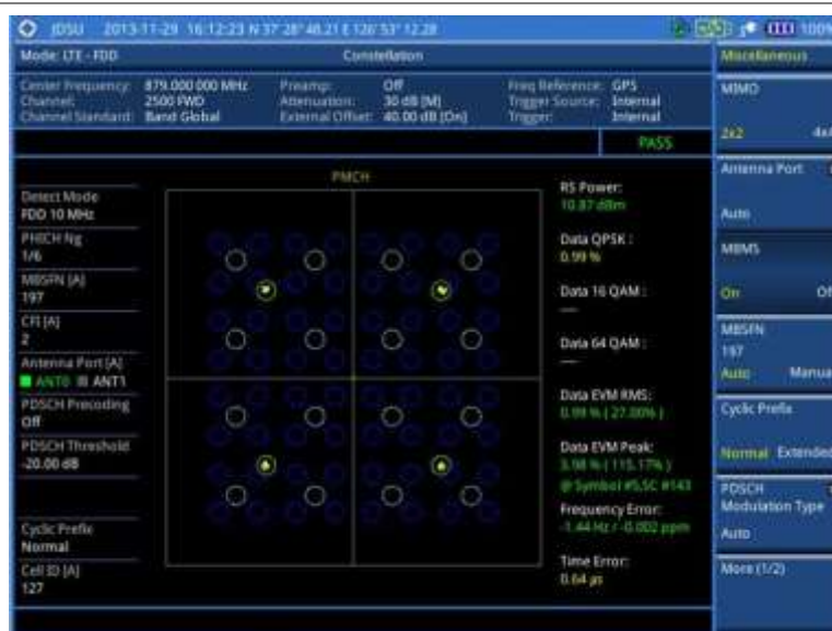
Figure 102 Constellation measurement with LTE-FDD signal analyzer (MBMS On)
