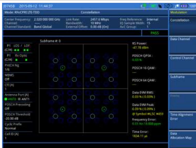
Figure 356 Constellation measurement with RFoCPRI LTE-TDD signal analyzer
