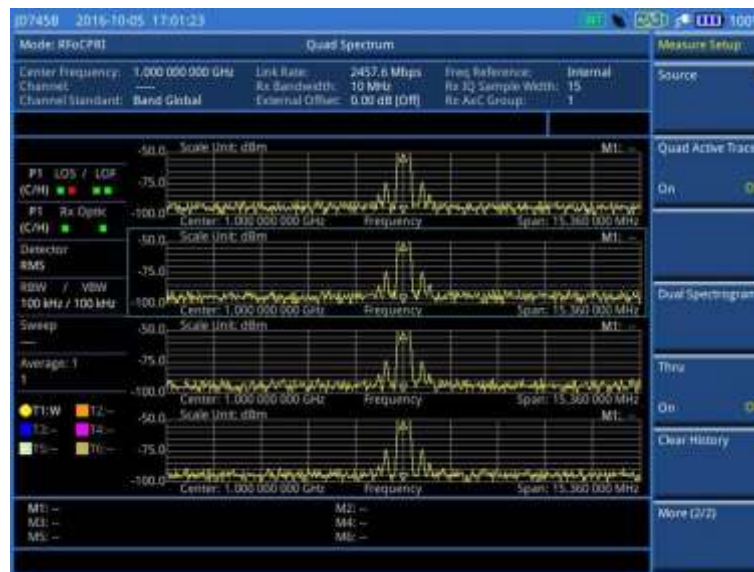
Figure 329 RFoCPRI quad spectrum with quad active trace on
