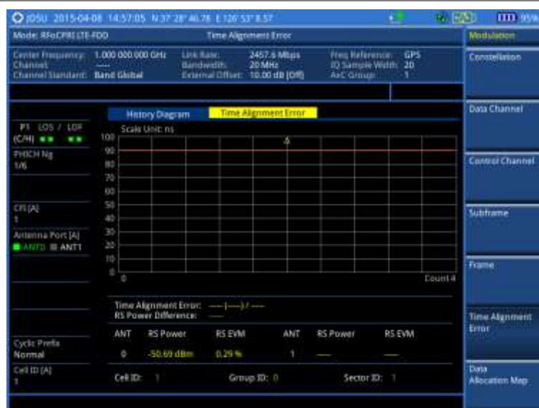
Figure 348 Time alignment error measurement with RFoCPRI LTE-FDD signal analyzer
