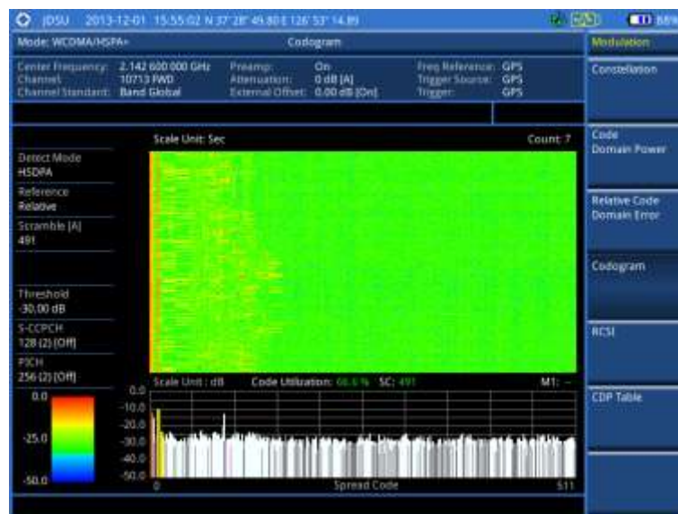
Figure 77 Codogram in full view with WCDMA/HSPA+ signal analyzer
