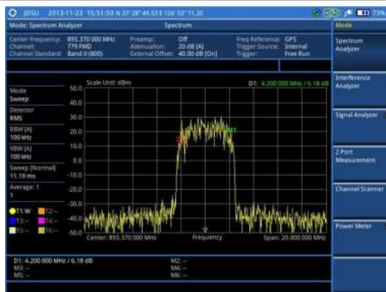
Figure 14 Spectrum measurement with spectrum analyzer
