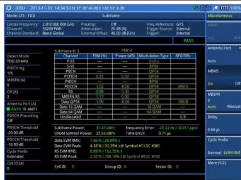
Figure 159 Subframe measurement with LTE-TDD signal analyzer (MBMS On)
