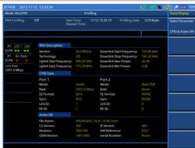
Figure 366 Example of RRH profiling results with CPRI state and activated SW
