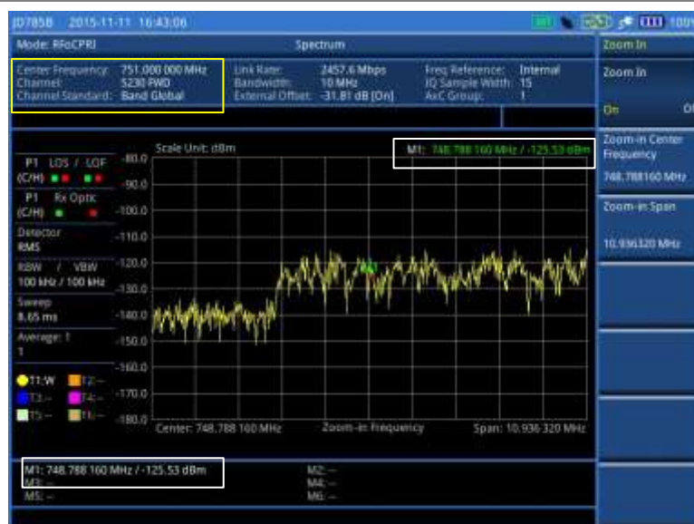
Figure 333 Zoomed-in spectrum view in RFoCPRI interference analyzer
