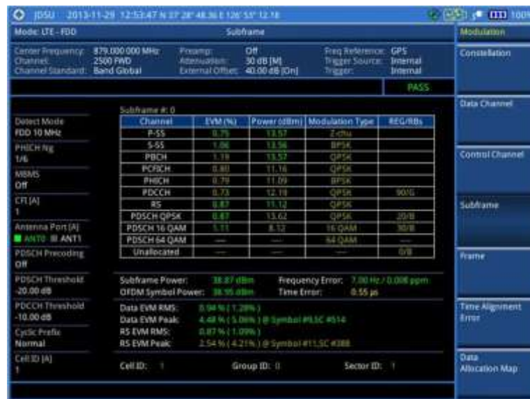
Figure 109 Subframe measurement with LTE-FDD signal analyzer (Chart On)
