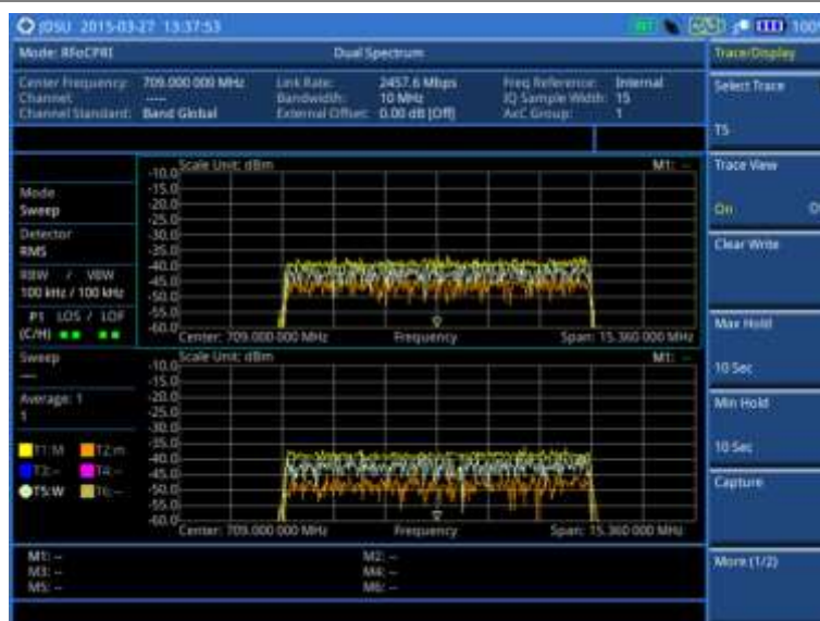
Figure 325 RFoCPRI dual spectrum analysis
