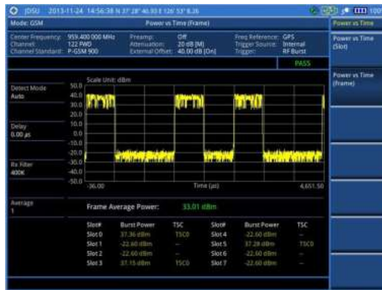
Figure 55 Power vs. time (frame) measurement with GSM signal analyzer
