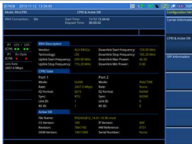
Figure 370 Example of verification of CPRI state and active software
