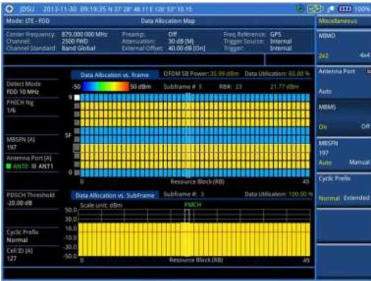
Figure 115 Data allocation map measurement with LTE-FDD signal analyzer (MBMS On)
