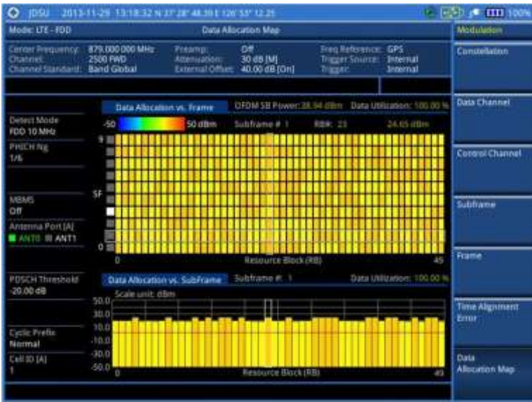
Figure 115 Data allocation map measurement with LTE-FDD signal analyzer (MBMS On)
