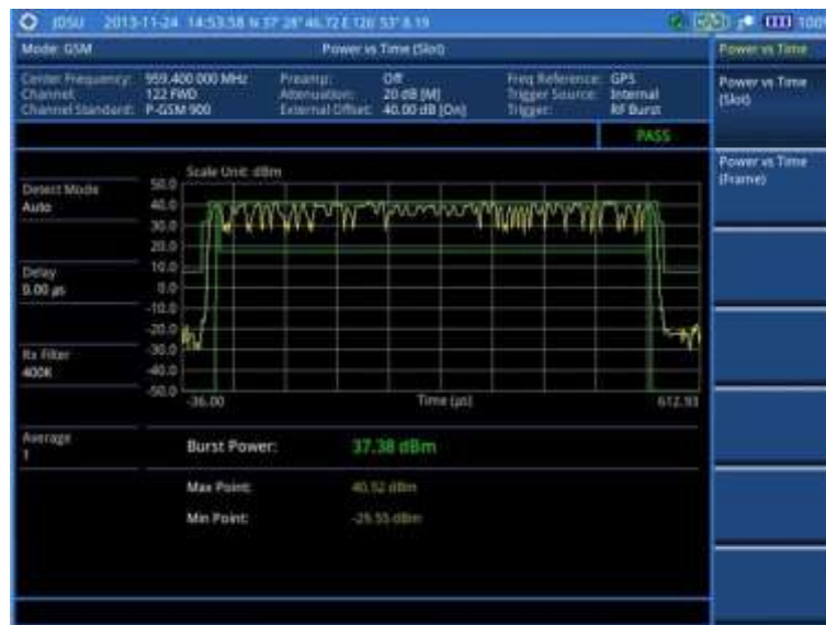
Figure 54 Power vs. time (slot) measurement with GSM signal analyzer
