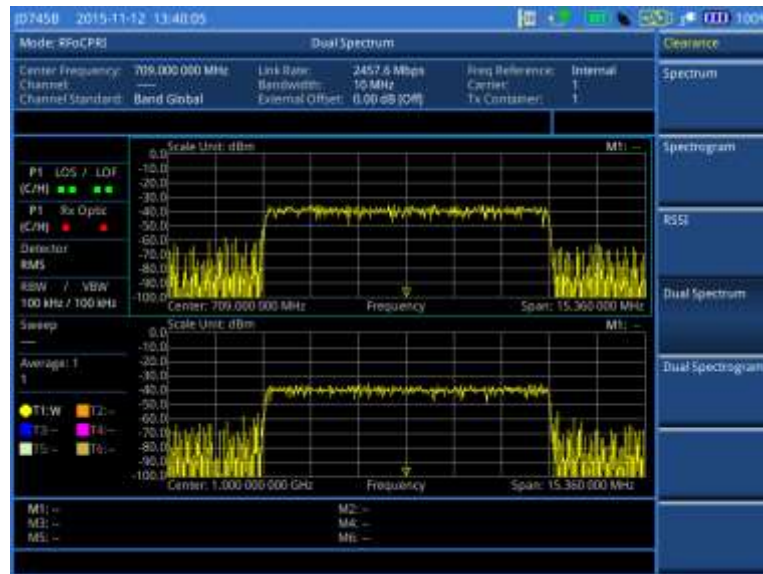
Figure 375 Example of dual spectrum analysis in BBU emulation
