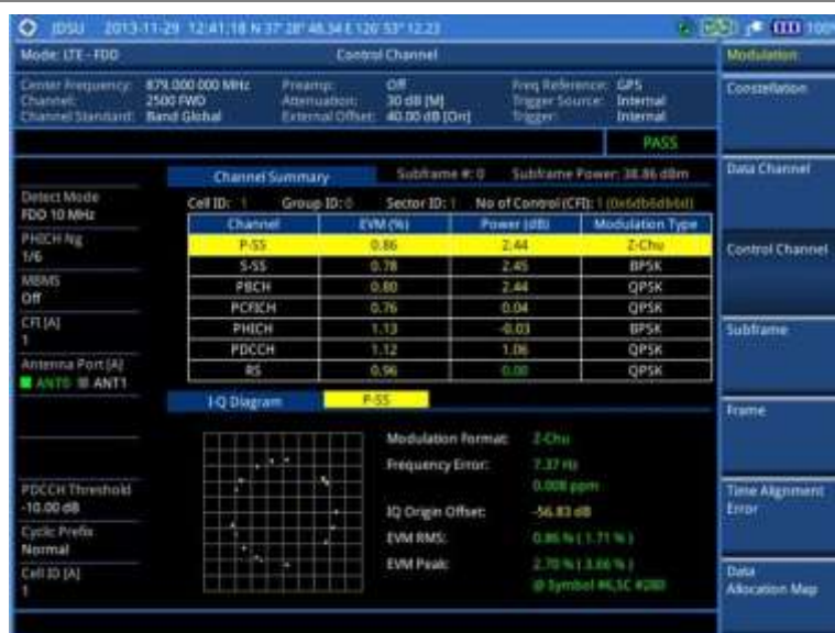
Figure 106 Control channel measurement with LTE-FDD signal analyzer
