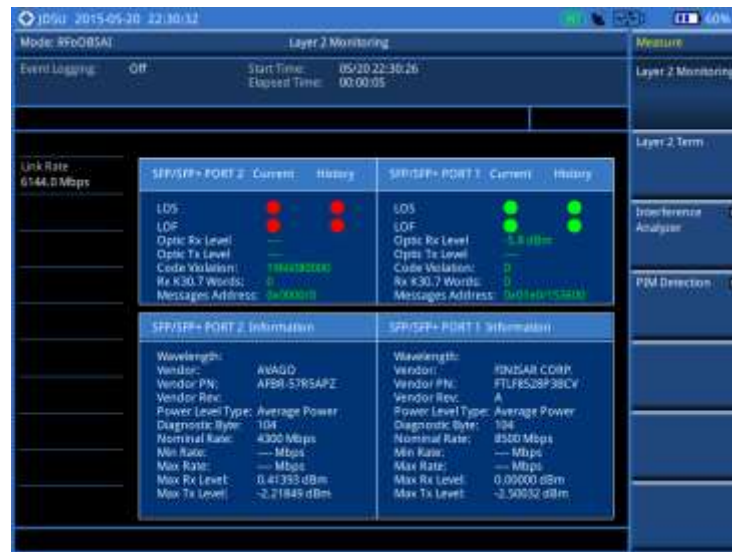
Figure 385 OBSAI RP3 layer 2 monitoring
