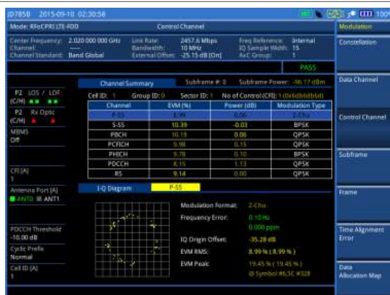
Figure 345 Control channel measurement with RFoCPRI LTE-FDD signal analyzer
