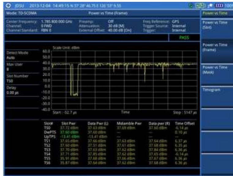
Figure 242 Power vs. time (frame) measurement with TD-SCDMA signal analyzer
