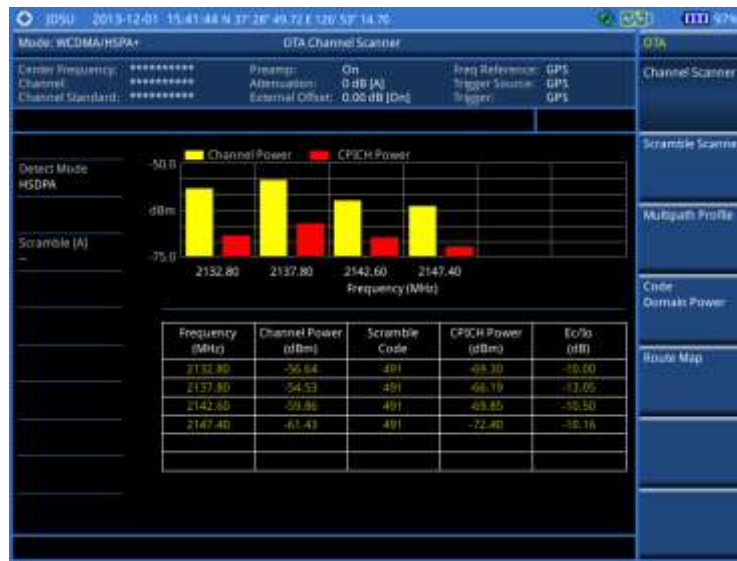
Figure 81 Channel scanner measurement with WCDMA/HSPA+ OTA signal analyzer
