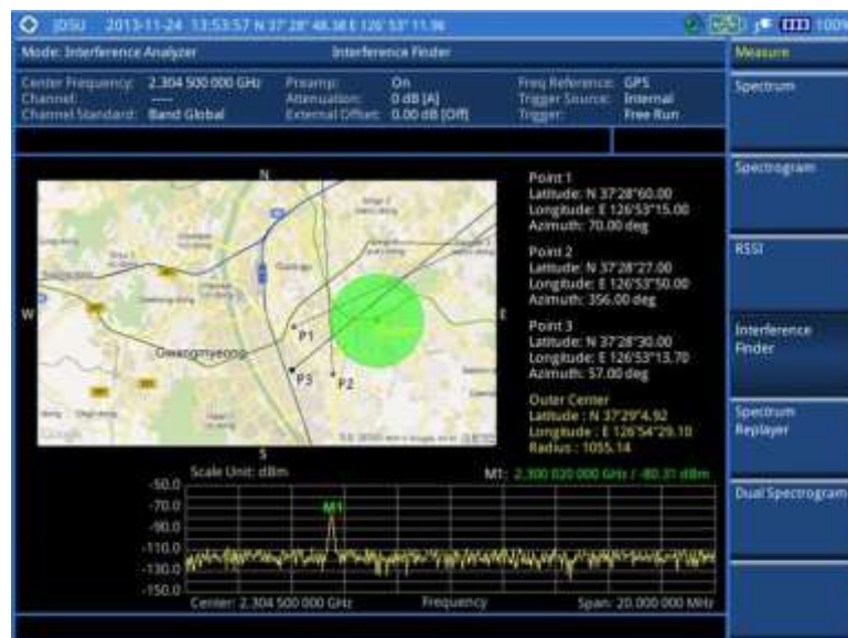
Figure 39 Interference finder measurement in map view
