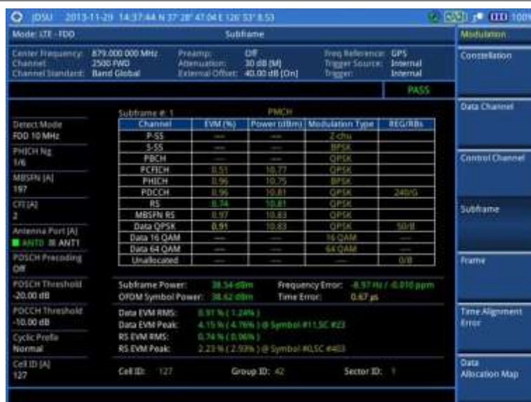
Figure 110 Subframe measurement with LTE-FDD signal analyzer (MBMS On)
