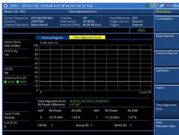
Figure 113 Time alignment error measurement with LTE-FDD signal analyzer
