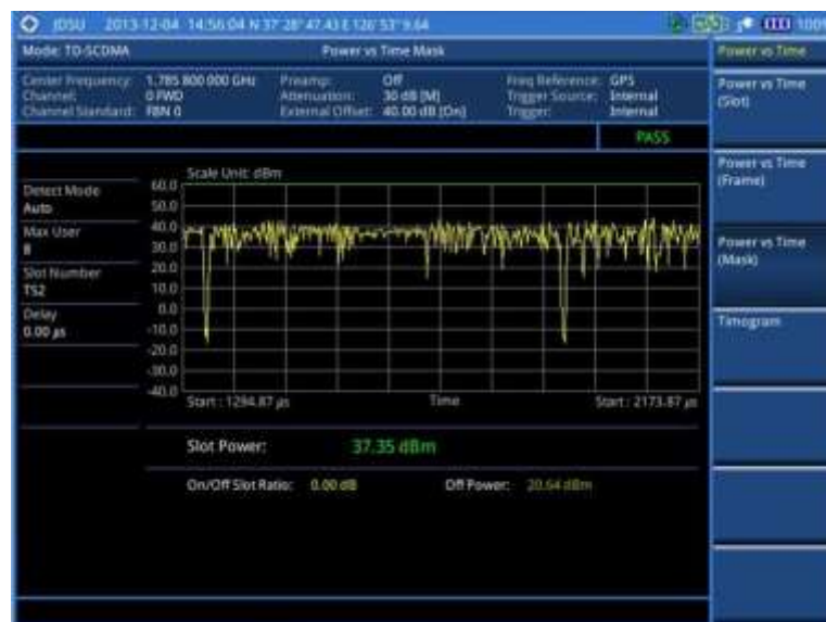
Figure 243 Power vs. time (mask) measurement with TD-SCDMA signal analyzer
