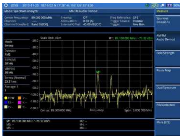
Figure 24 AM/FM audio demodulation with spectrum analyzer
