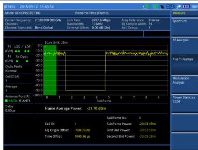
Figure 355 Power vs. time (frame) measurement with RFoCPRI LTE-TDD signal analyzer
