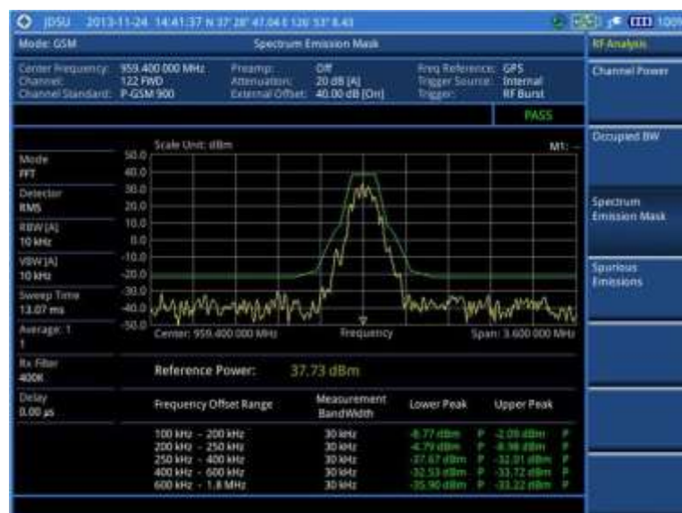
Figure 50 SEM measurement with GSM signal analyzer
