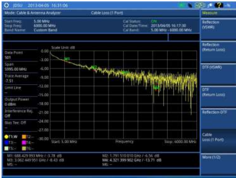
Figure 304 Cable loss (1 port) measurement
