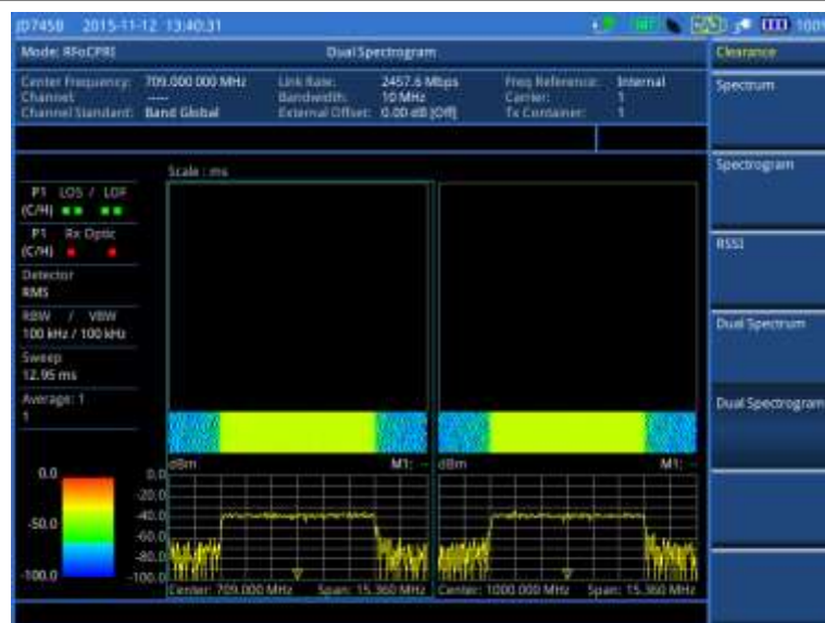
Figure 377 Example of dual spectrogram analysis in BBU emulation
