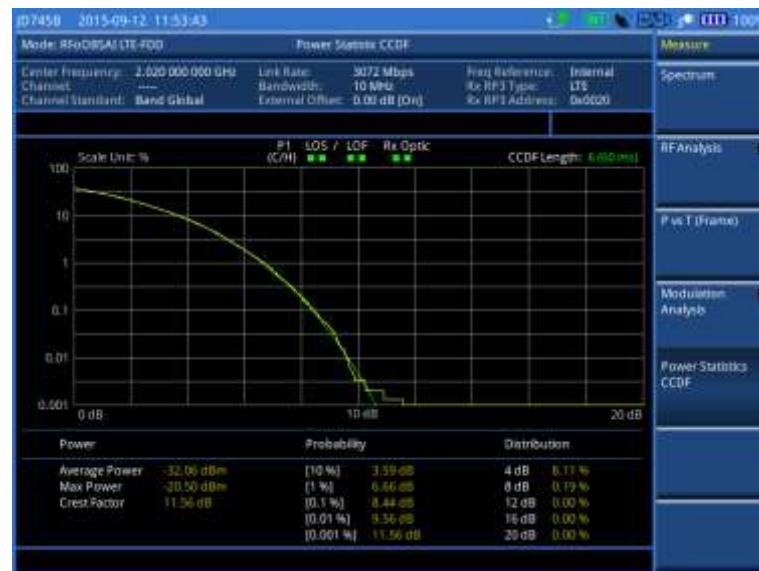
Figure 407 CCDF measurement with RFoBSAI LTE-FDD signal analyzer
