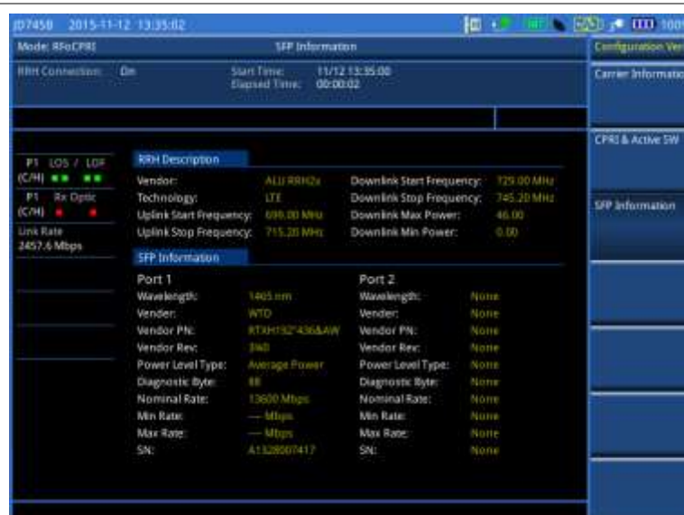
Figure 371 Example of verification of SFP information
