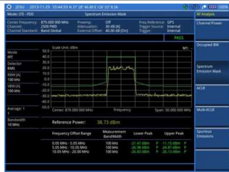
Figure 96 SEM measurement with LTE-FDD signal analyzer
