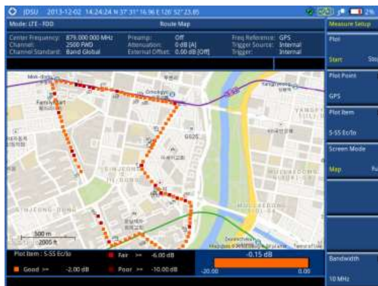
Figure 132 Route map measurement (S-SS Ec/Io) with LTE-FDD OTA signal analyzer
