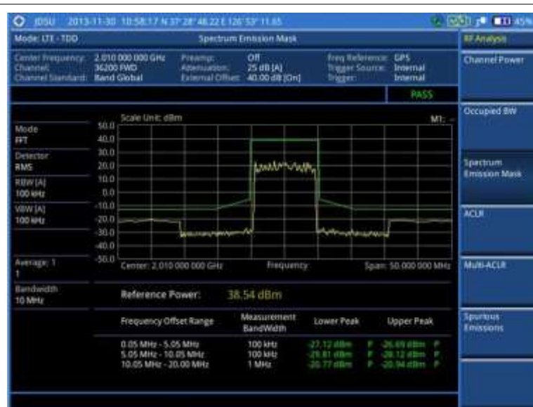
Figure 145 SEM measurement with LTE-TDD signal analyzer
