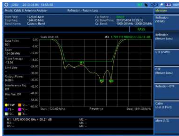
Figure 300 Reflection measurement in return loss scale
