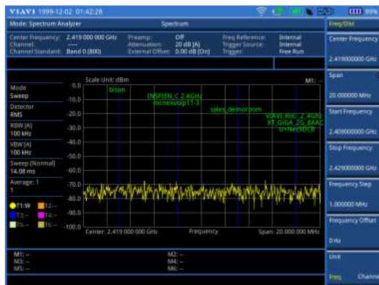
Figure 16 Wi-Fi SSID display with spectrum analyzer
