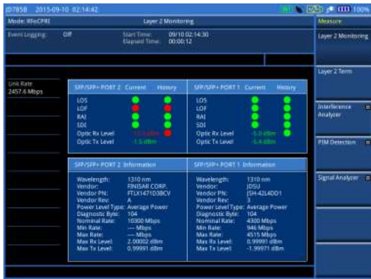
Figure 313 CPRI layer 2 monitoring
