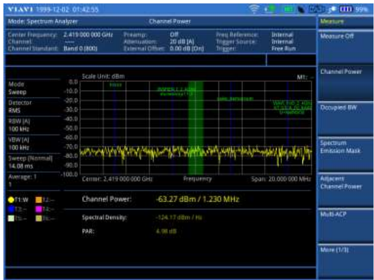
Figure 18 Wi-Fi SSID display in channel power measurement with spectrum analyzer
