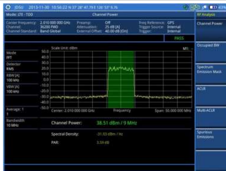
Figure 143 Channel power measurement with LTE-TDD signal analyzer
