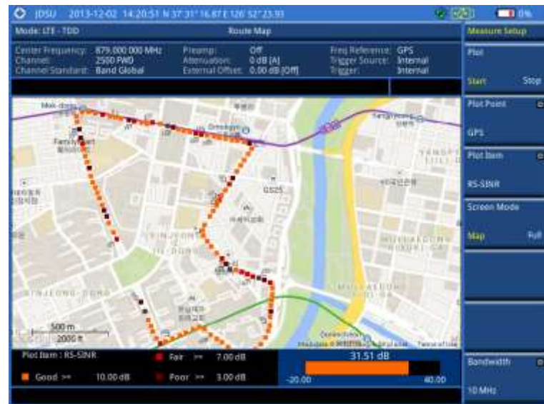
Figure 174 Route map measurement (RS-SINR) with LTE-TDD OTA signal analyzer
