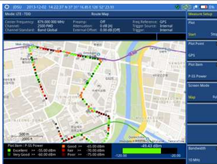
Figure 176 Route map measurement (P-SS Power) with LTE-TDD OTA signal analyzer
