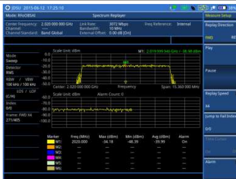
Figure 392 RFoBSAI spectrum replay
