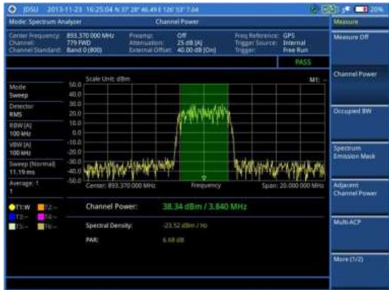
Figure 17 Channel power measurement with spectrum analyzer
