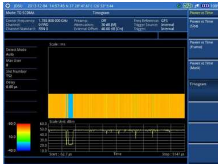
Figure 244 Timogram with TD-SCDMA signal analyzer
