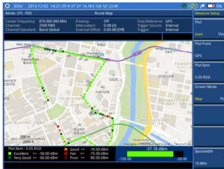
Figure 129 Route map measurement (S-SS RSSI) with LTE-FDD OTA signal analyzer
