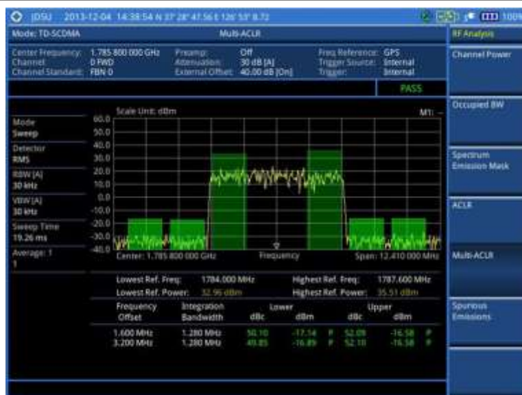
Figure 239 Multi-ACLR measurement with TD-SCDMA signal analyzer
