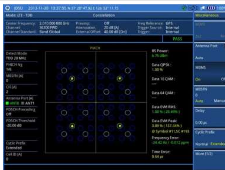
Figure 152 Constellation measurement with LTE-TDD signal analyzer (MBMS On)
