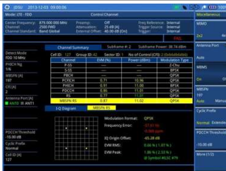
Figure 107 Control channel measurement with LTE-FDD signal analyzer (MBMS On)
