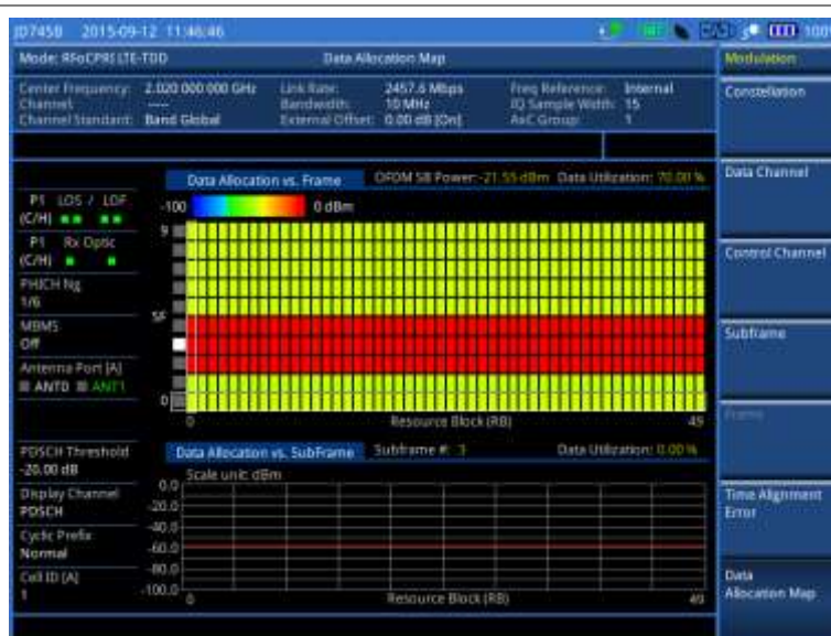
Figure 361 Data allocation map measurement with RFoCPRI LTE-TDD signal analyzer
