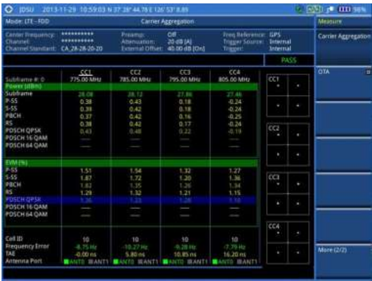
Figure 120 Carrier aggregation measurement with LTE-FDD signal analyzer (SA)
