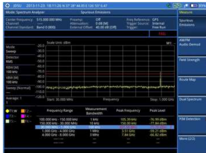
Figure 23 Spurious emissions measurement with spectrum analyzer
