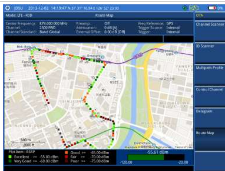
Figure 126 Route map measurement (RSRP) with LTE-FDD OTA signal analyzer
