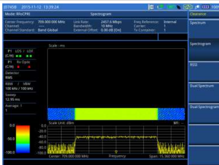
Figure 376 Example of spectrogram in BBU emulation
