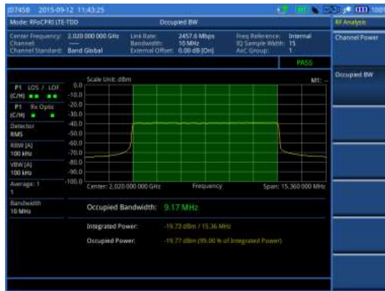
Figure 354 Occupied bandwidth measurement with RFoCPRI LTE-TDD signal analyzer
