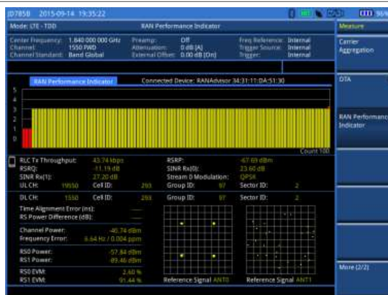
Figure 180 RAN performance indicator with LTE-TDD signal analyzer
