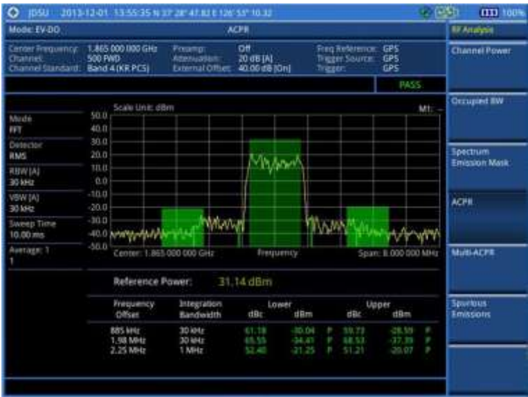
Figure 213 ACPR measurement with EV-DO signal analyzer
