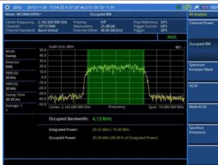
Figure 69 Occupied bandwidth measurement with WCDMA/HSPA+ signal analyzer
