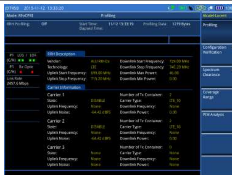
Figure 365 Example of RRH profiling results with carrier information
