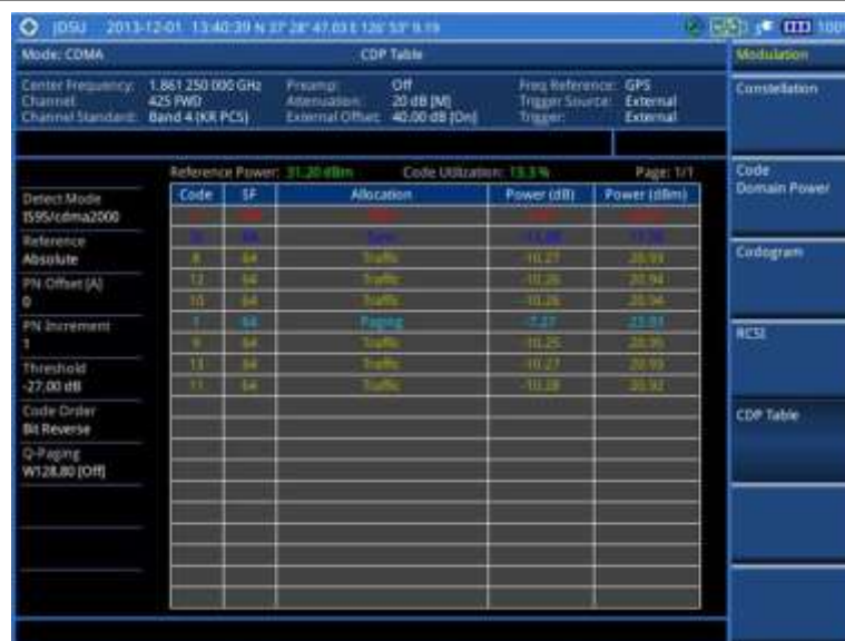
Figure 197 CDP Table measurement with CDMA signal analyzer
