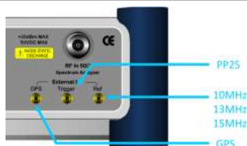
Figure 92 Connection ports for external reference clock
