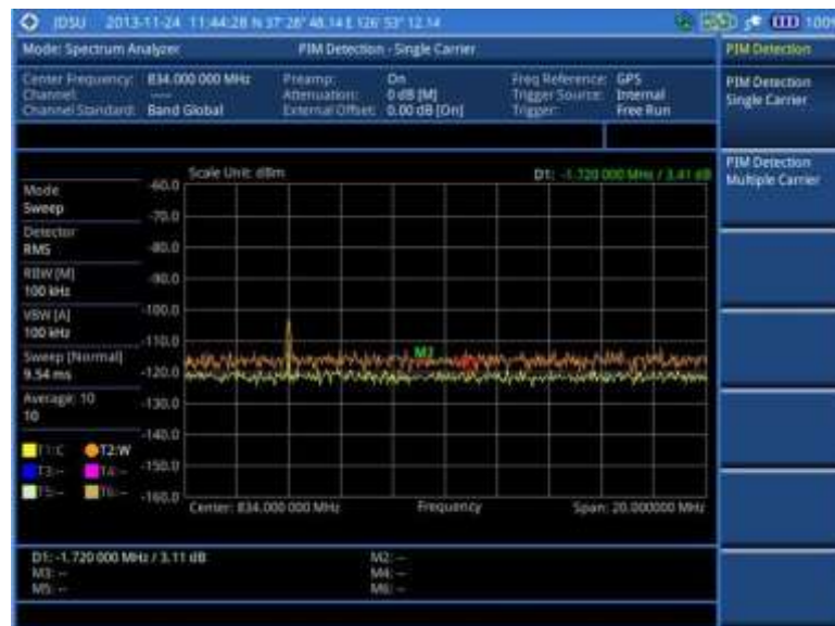
Figure 30 PIM detection for multiple carriers
