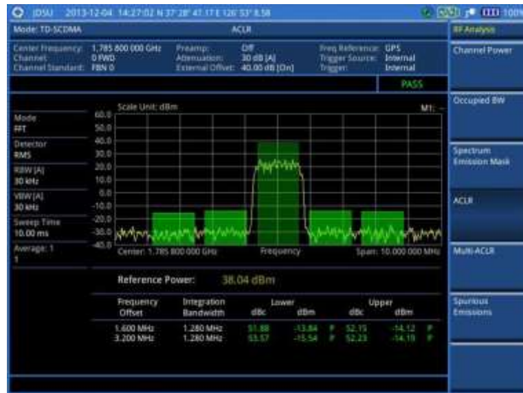
Figure 238 ACLR measurement with TD-SCDMA signal analyzer
