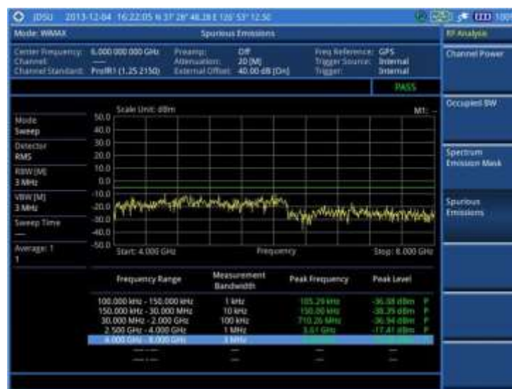
Figure 263 Spurious emissions measurement with Mobile WiMAX signal analyzer
