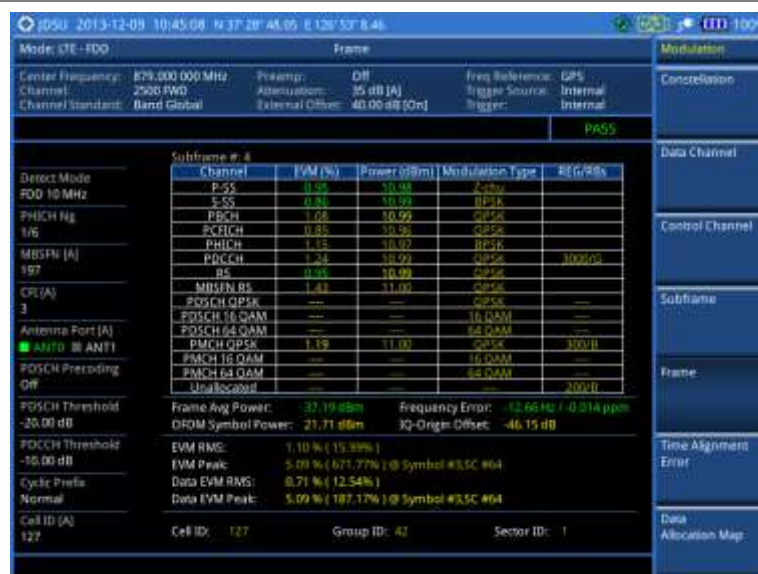
Figure 112 Frame measurement with LTE-FDD signal analyzer (MBMS On)
