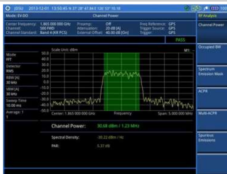
Figure 210 Channel power measurement with EV-DO signal analyzer
