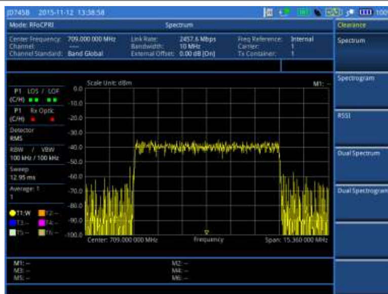
Figure 374 Example of spectrum measurement in BBU emulation
