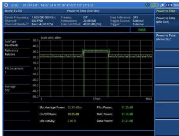
Figure 216 Power vs. time (idle slot) measurement with EV-DO signal analyzer
