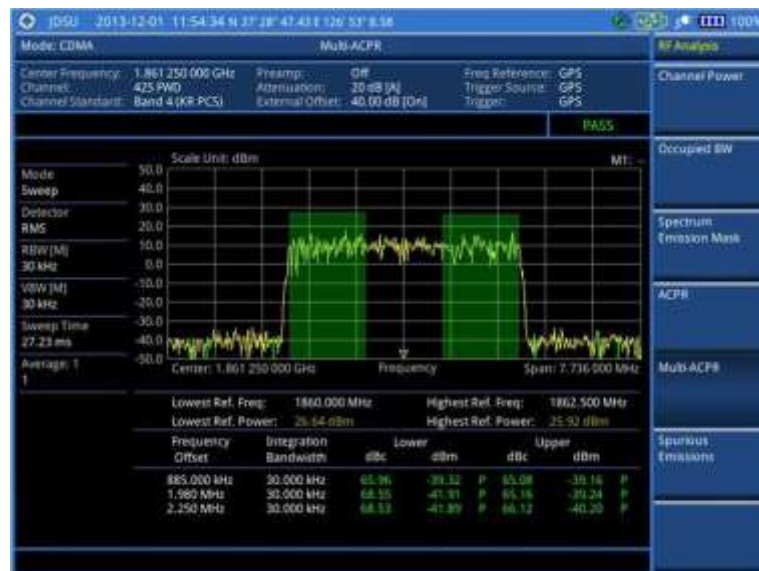
Figure 191 Multi-ACPR measurement with CDMA signal analyzer
