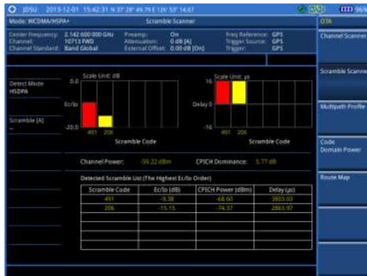
Figure 82 Scramble scanner measurement with WCDMA/HSPA+ OTA signal analyzer
