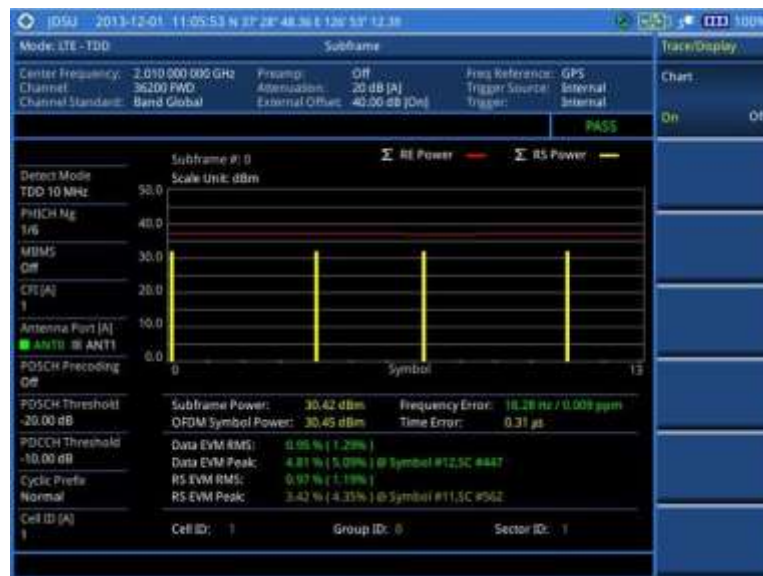
Figure 158 Subframe measurement with LTE-TDD signal analyzer (Chart On)
