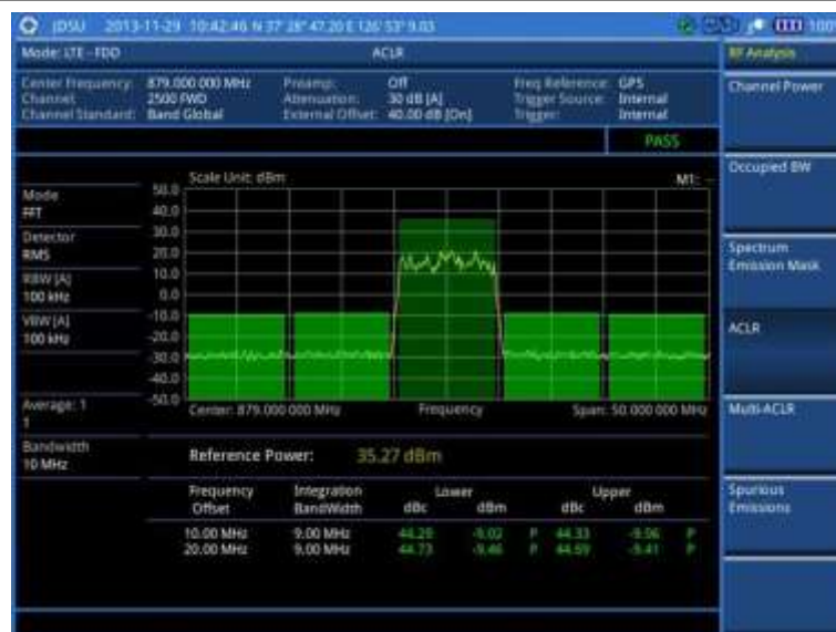
Figure 97 ACLR measurement with LTE-FDD signal analyzer
