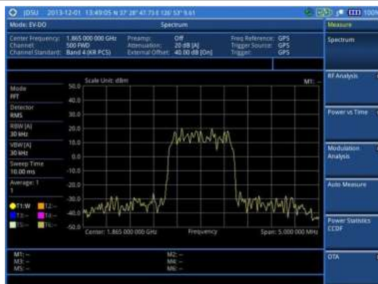
Figure 209 Spectrum measurement screen with EV-DO signal analyzer
