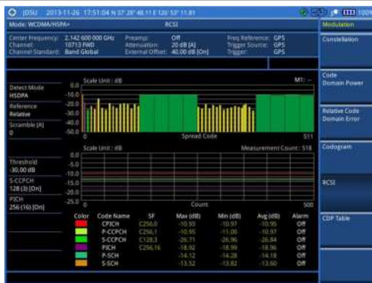
Figure 78 RCSI measurement with WCDMA/HSPA+ signal analyzer
