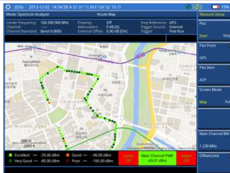
Figure 26 Route map measurement screen with GPS
