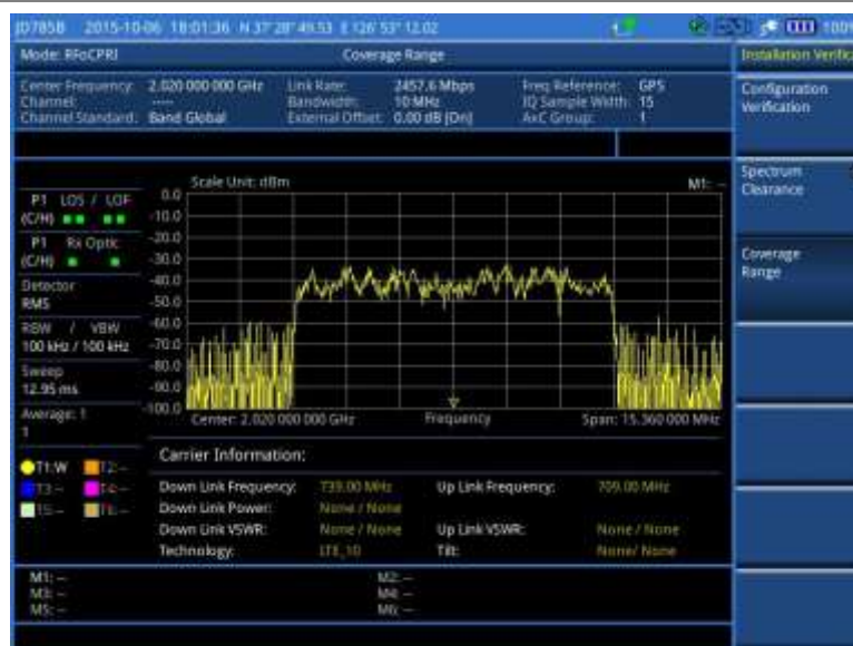
Figure 379 Example of coverage range in BBU emulation
