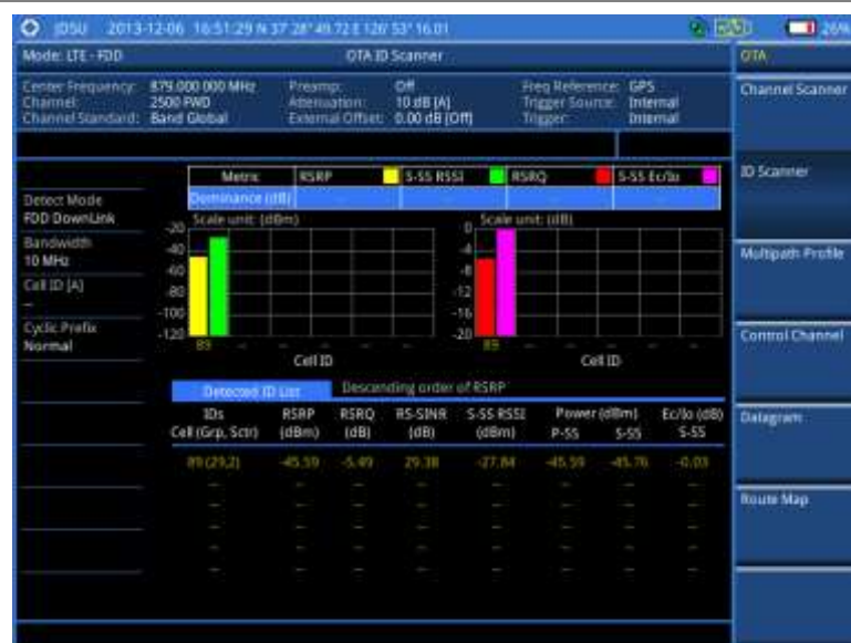
Figure 122 ID scanner measurement with LTE-FDD OTA signal analyzer
