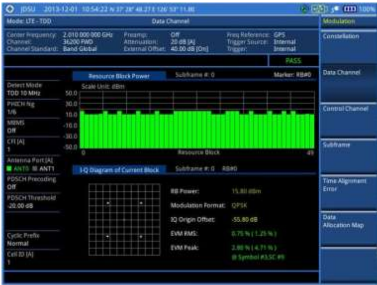
Figure 154 Data channel measurement with LTE-TDD signal analyzer (MBMS On)
