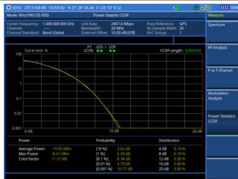
Figure 350 CCDF measurement with RFoCPRI LTE-FDD signal analyzer
