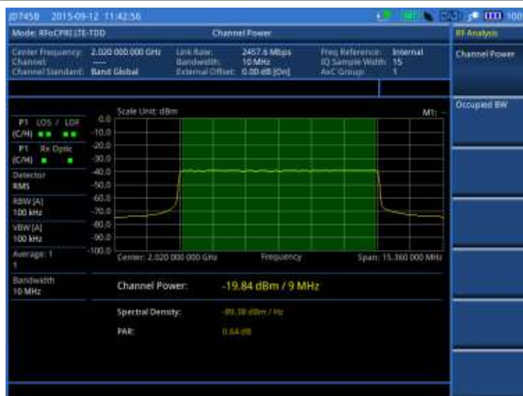
Figure 353 Channel power measurement with RFoCPRI LTE-TDD signal analyzer
