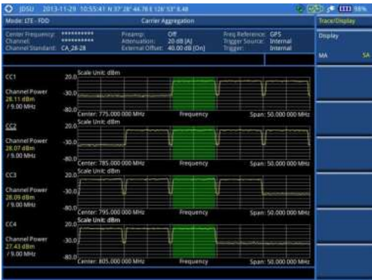
Figure 120 Carrier aggregation measurement with LTE-FDD signal analyzer (SA)
