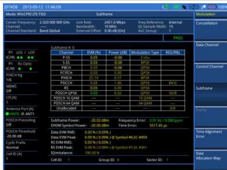
Figure 359 Subframe measurement (regular view) with RFoCPRI LTE-TDD signal analyzer
