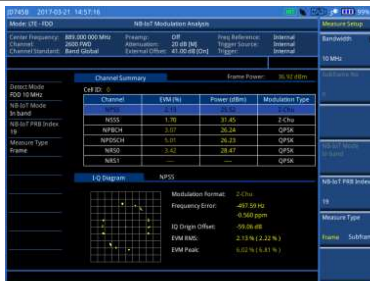
Figure 136 NB-IoT modulation measurement with LTE-FDD signal analyzer (Subframe 2)
