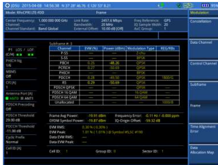
Figure 347 Frame measurement with RFoCPRI LTE-FDD signal analyzer
