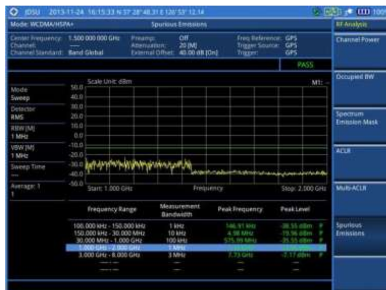
Figure 73 Spurious emissions measurement with WCDMA/HSPA+ signal analyzer
