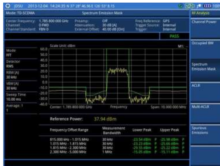
Figure 237 SEM measurement with TD-SCDMA signal analyzer
