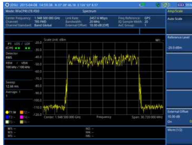
Figure 339 Spectrum measurement with RFoCPRI LTE-FDD signal analyzer
