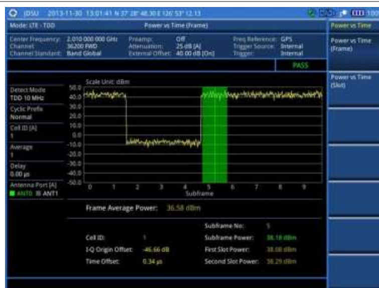
Figure 150 Power vs. time (frame) measurement with LTE – TDD signal analyzer
