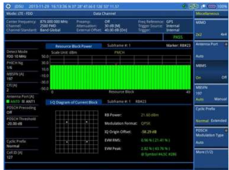
Figure 104 Data channel measurement with LTE-FDD signal analyzer (MBMS On)
