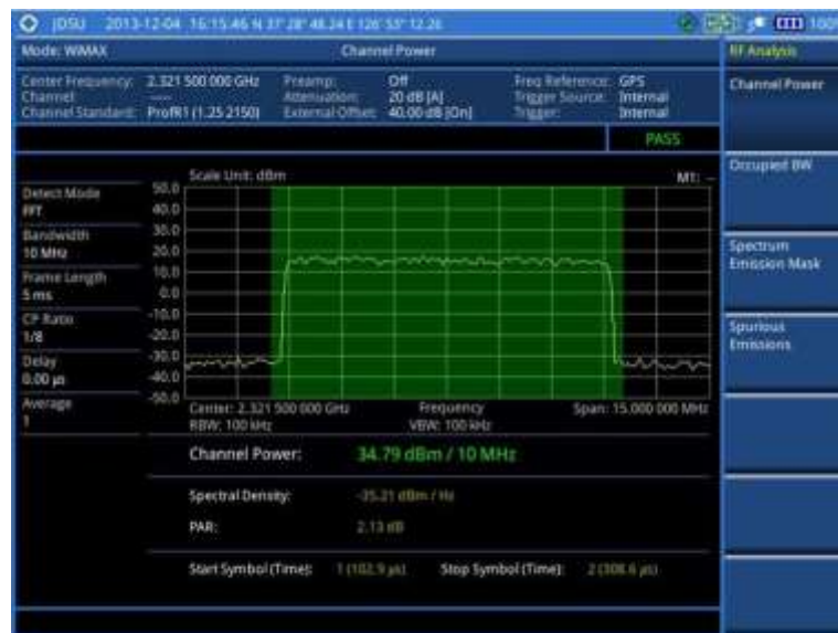
Figure 260 Channel power measurement with Mobile WiMAX signal analyzer
