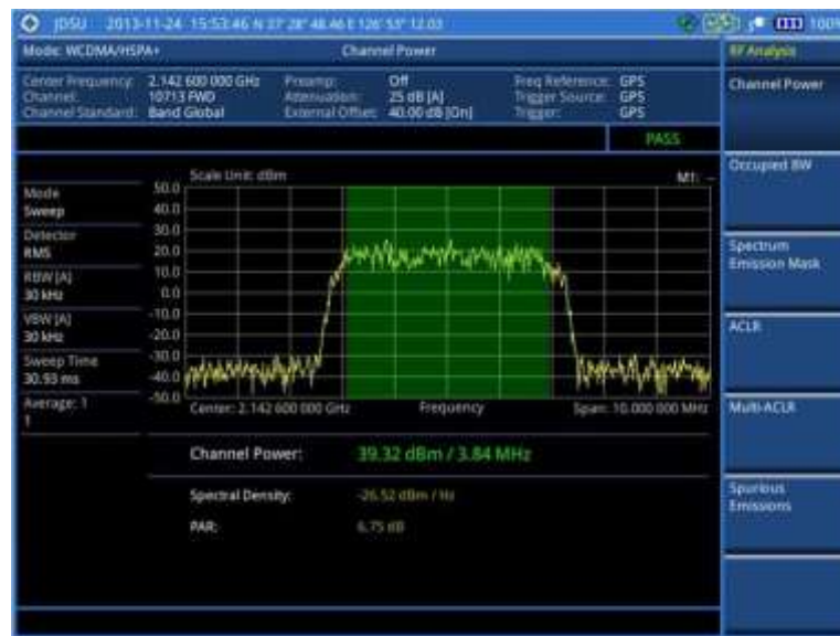
Figure 68 Channel power measurement with WCDMA/HSPA+ signal analyzer
