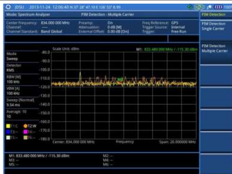
Figure 30 PIM detection for multiple carriers
