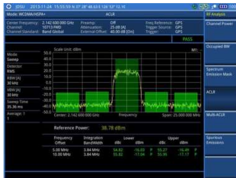
Figure 71 ACLR measurement with WCDMA/HSPA+ signal analyzer
