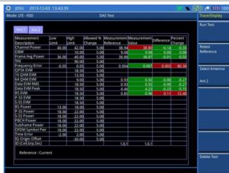
Figure 117 DAS measurement with LTE-FDD signal analyzer
