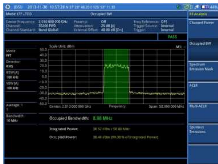
Figure 144 Occupied bandwidth measurement with LTE-TDD signal analyzer
