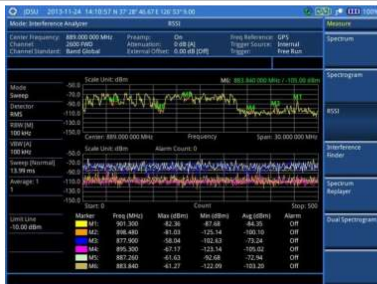
Figure 38 Interference measurement in RSSI
