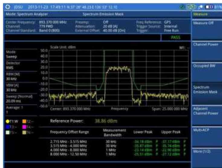
Figure 20 Spectrum emission mask measurement with spectrum analyzer
