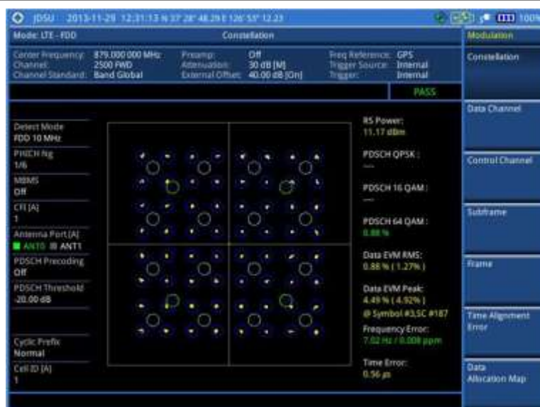
Figure 101 Constellation measurement with LTE-FDD signal analyzer
