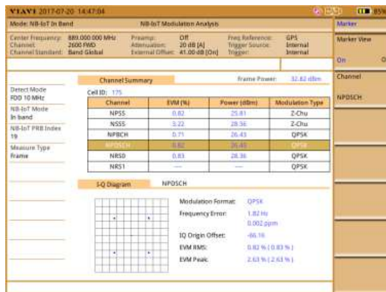
Figure 278 NB-IoT In Band Modulation Analysis measurement screen (Frame)
