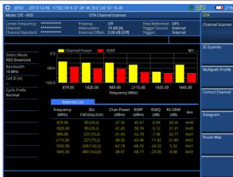
Figure 121 Channel scanner measurement with LTE-FDD OTA signal analyzer
