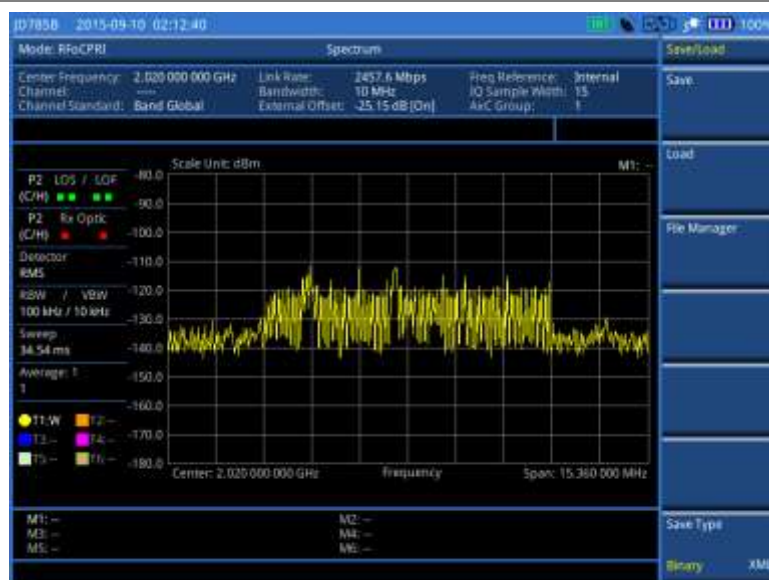
Figure 323 RFoCPRI spectrum analysis on LTE Uplink 10 MHz, antenna 1
