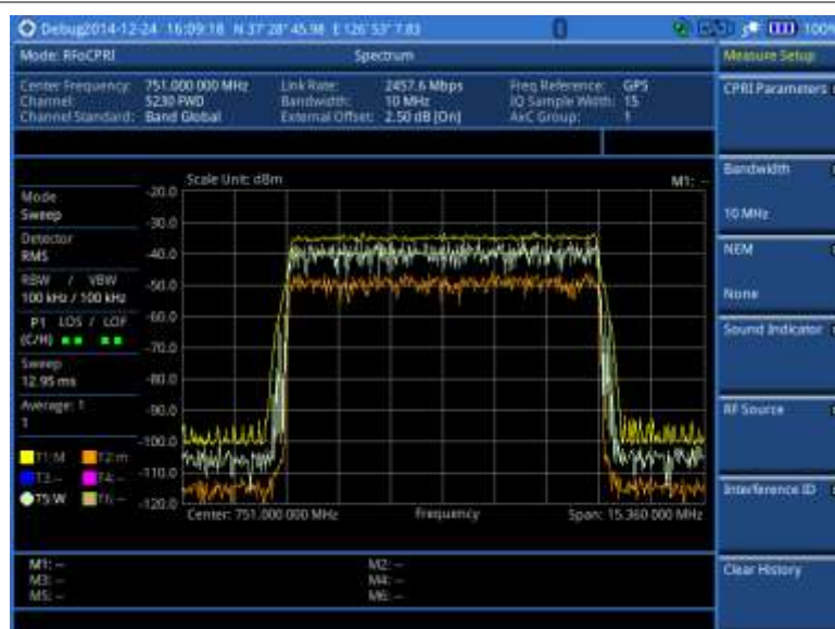
Figure 323 RFoCPRI spectrum analysis on LTE Uplink 10 MHz, antenna 1
