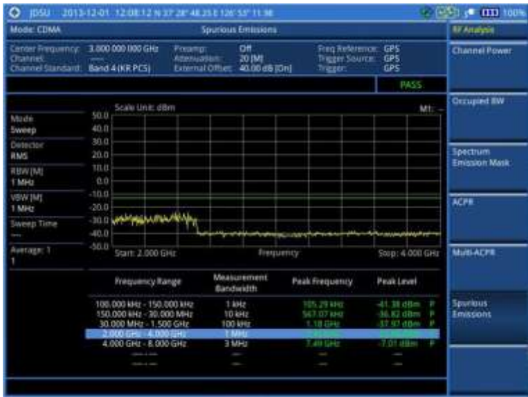
Figure 192 Spurious emissions measurement with CDMA signal analyzer
