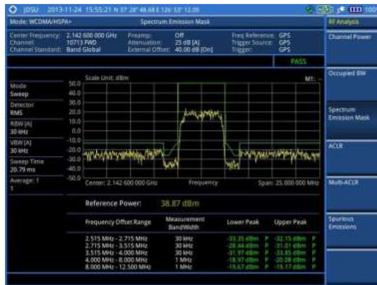
Figure 70 SEM measurement with WCDMA/HSPA+ signal analyzer
