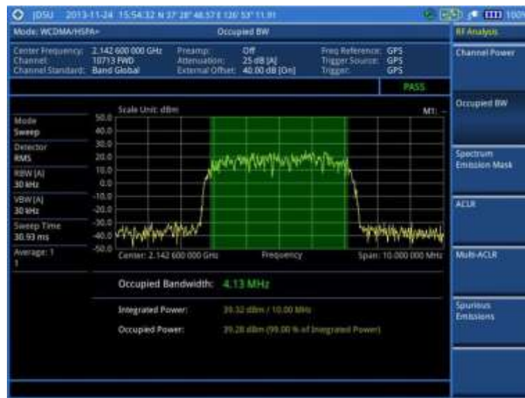
Figure 88 Occupied bandwidth measurement with WCDMA/HSPA+ signal analyzer
