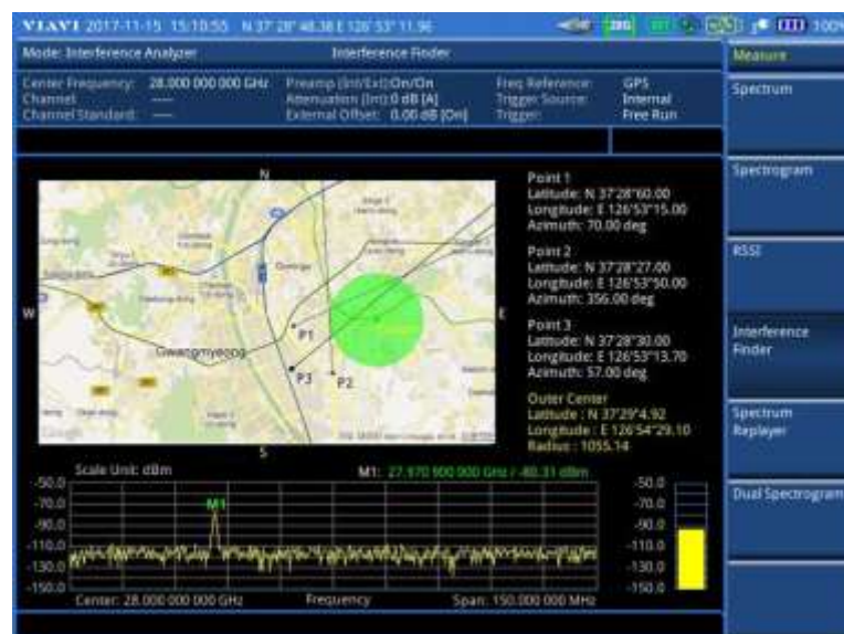
Figure 55 Interference finder measurement in map view (on 28 GHz downconverter)
