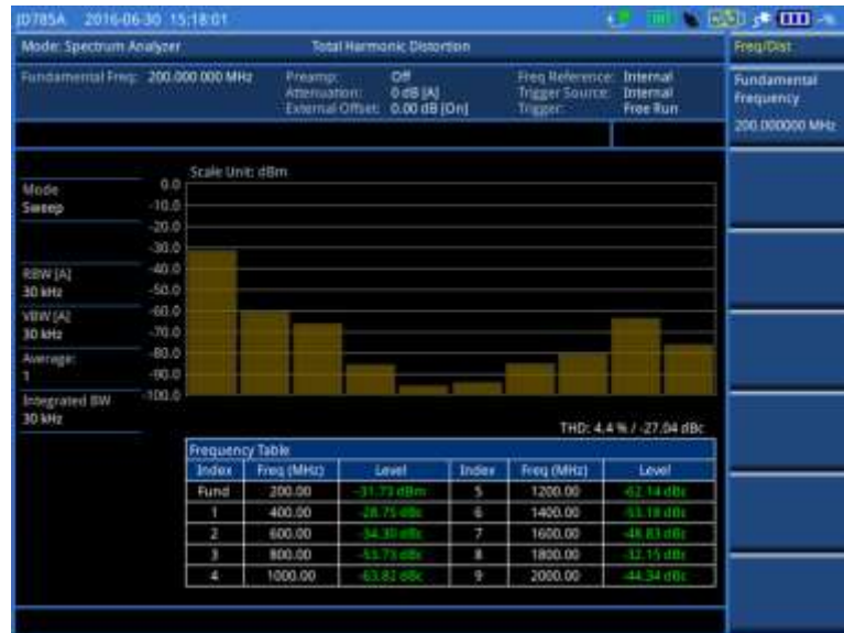
Figure 42 Total harmonic distortion screen
