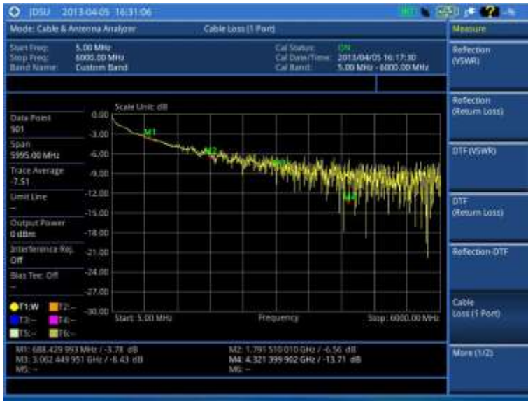
Figure 323 Cable loss (1 port) measurement
