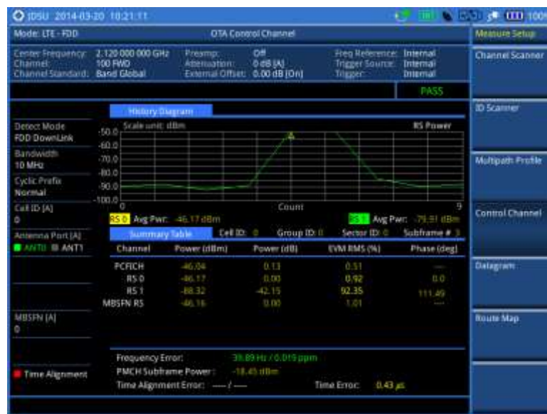
Figure 143 Control channel measurement with LTE-FDD OTA signal analyzer
