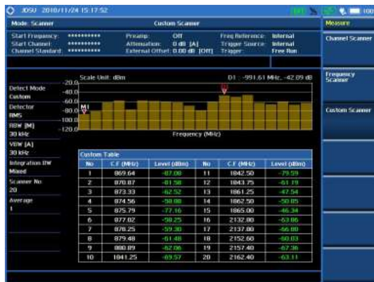
Figure 433 Custom scanner measurement
