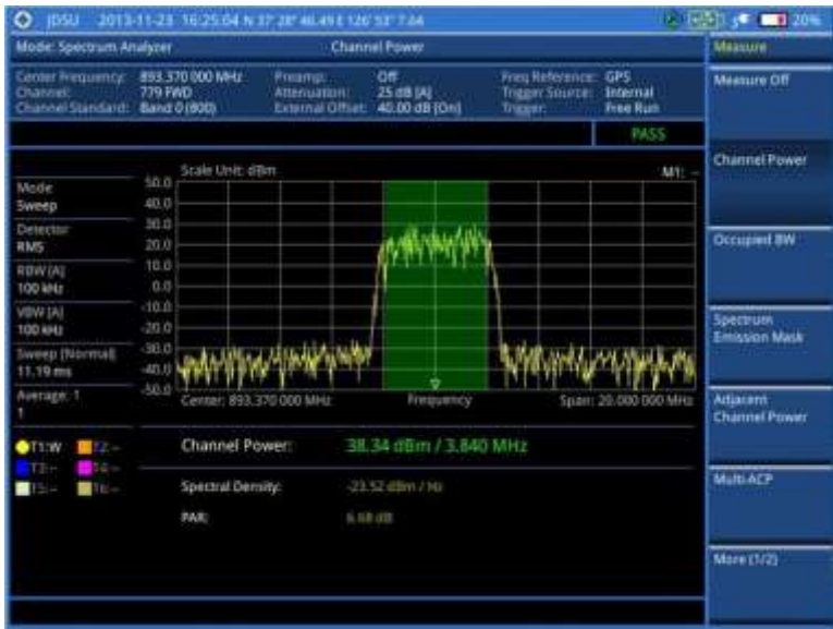
Figure 20 Channel power measurement with spectrum analyzer
