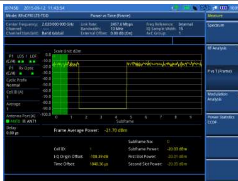
Figure 374 Power vs. time (frame) measurement with RFoCPRI LTE-TDD signal analyzer
