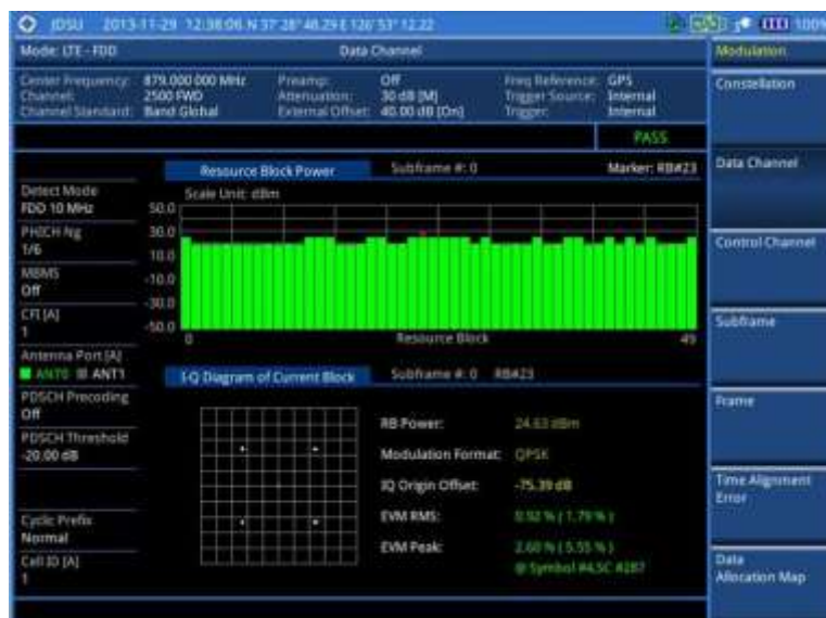
Figure 122 Data channel measurement with LTE-FDD signal analyzer
