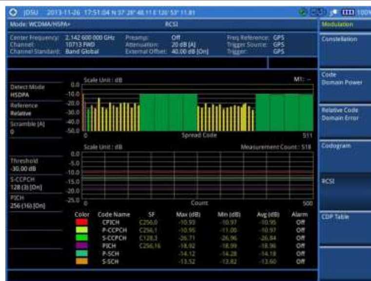
Figure 97 RCSI measurement with WCDMA/HSPA+ signal analyzer
