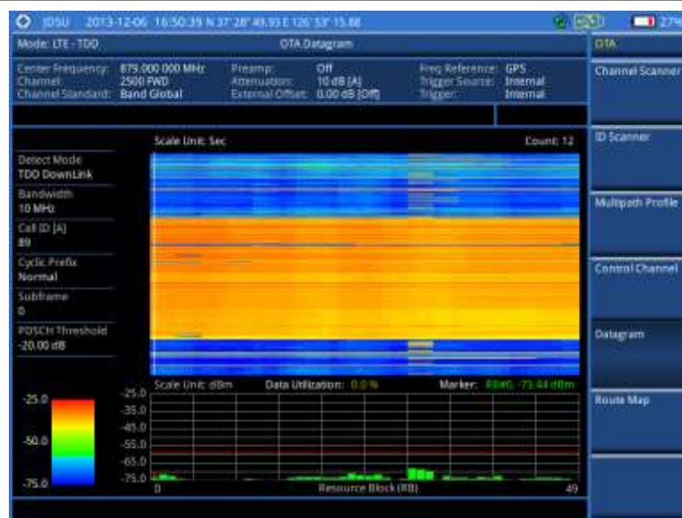
Figure 190 Datagram measurement with LTE-TDD signal analyzer
