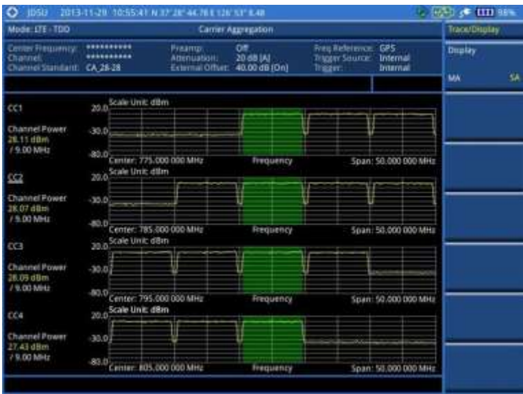
Figure 185 Carrier aggregation measurement with LTE-TDD signal analyzer (SA)
