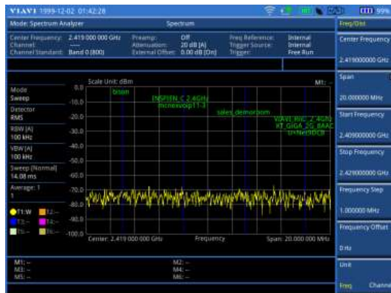
Figure 19 Wi-Fi SSID display with spectrum analyzer
