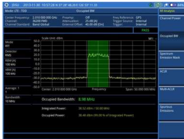
Figure 163 Occupied bandwidth measurement with LTE-TDD signal analyzer
