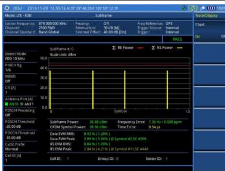
Figure 128 Subframe measurement with LTE-FDD signal analyzer (Chart On)
