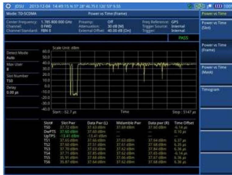
Figure 261 Power vs. time (frame) measurement with TD-SCDMA signal analyzer
