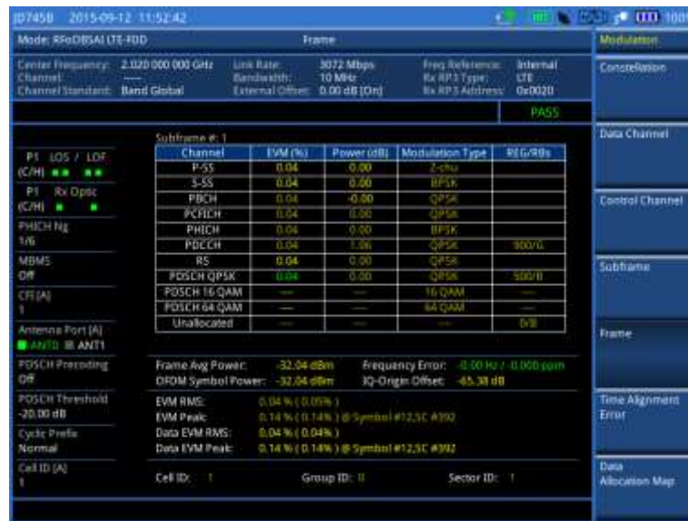
Figure 423 Frame measurement with RFoBSAI LTE-FDD signal analyzer
