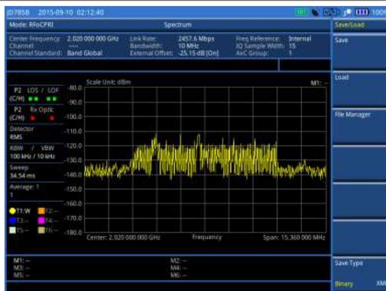
Figure 342 RFoCPRI spectrum analysis on LTE Uplink 10 MHz, antenna 1
