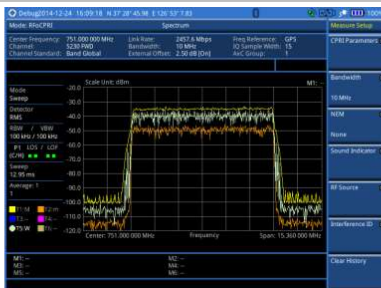
Figure 342 RFoCPRI spectrum analysis on LTE Uplink 10 MHz, antenna 1
