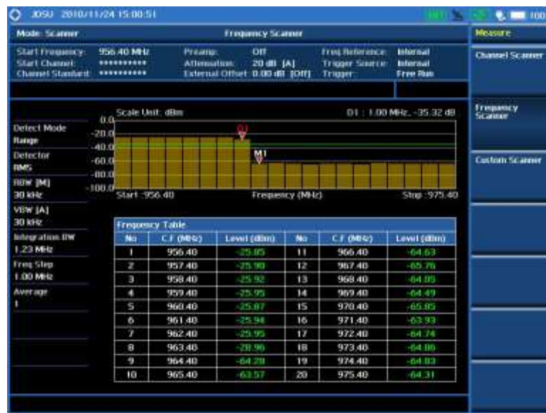
Figure 432 Frequency scanner measurement
