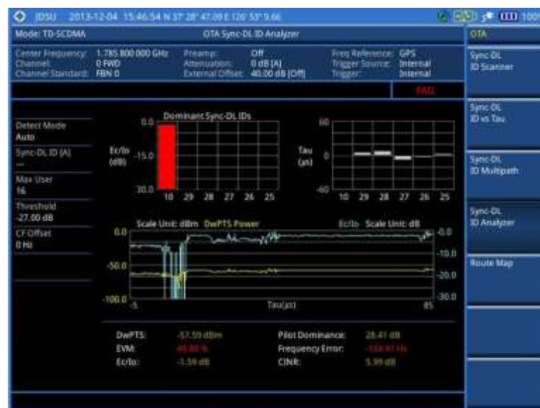
Figure 271 Sync-DL ID analyzer measurement with TD-SCDMA OTA signal analyzer
