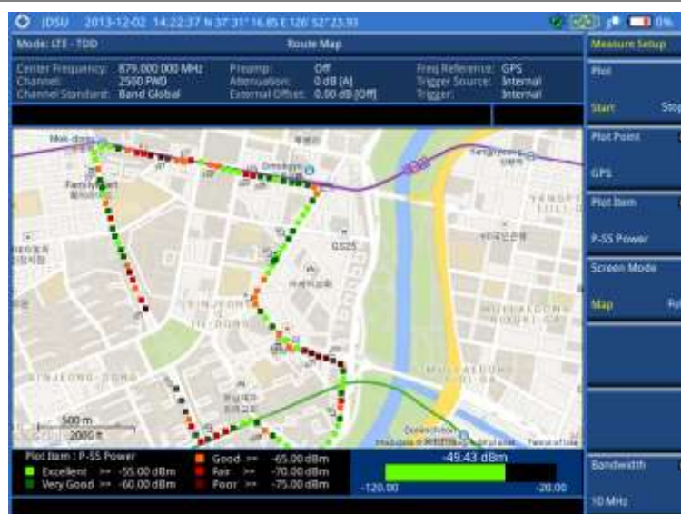
Figure 195 Route map measurement (P-SS Power) with LTE-TDD OTA signal analyzer
