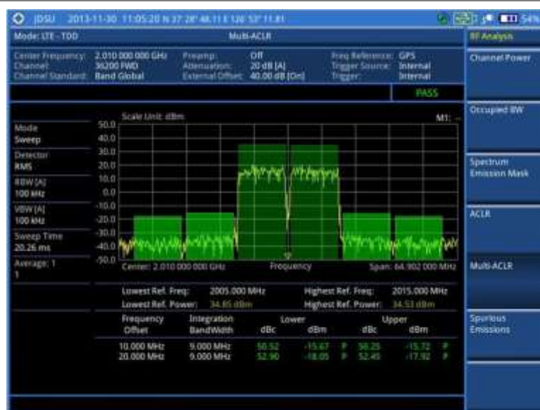
Figure 166 Multi-ACLR measurement with LTE-TDD signal analyzer
