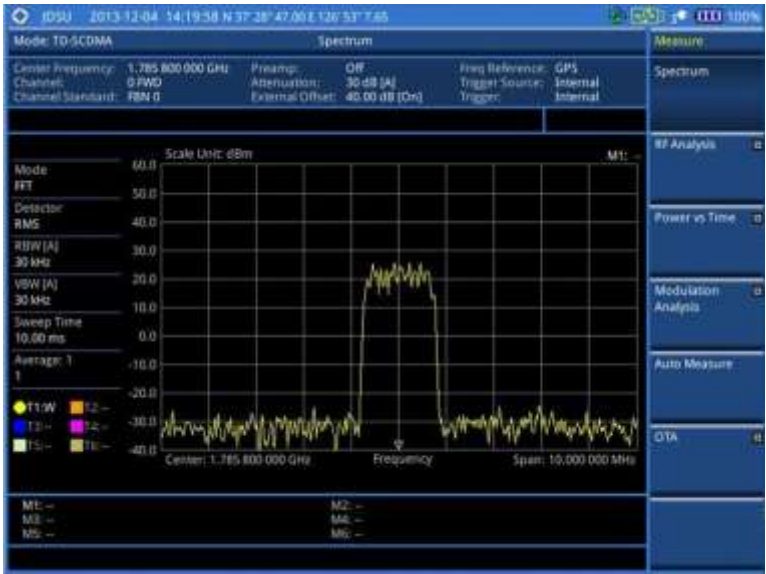
Figure 253 Spectrum measurement screen with TD-SCDMA signal analyzer
