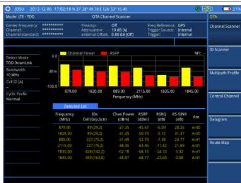
Figure 186 Channel scanner measurement with LTE-TDD OTA signal analyzer
