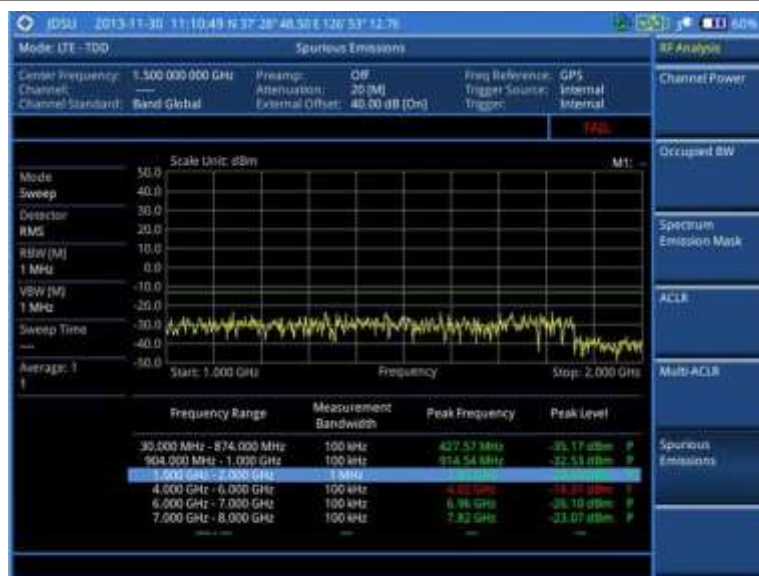
Figure 167 Spurious emissions measurement with LTE-TDD signal analyzer
