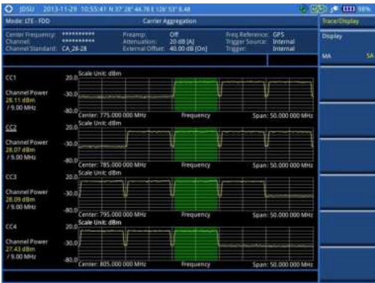
Figure 139 Carrier aggregation measurement with LTE-FDD signal analyzer (SA)
