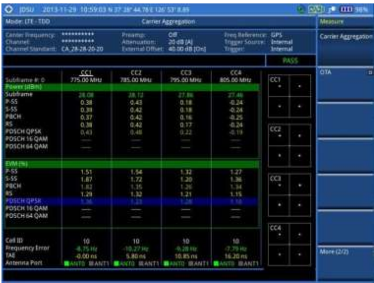
Figure 185 Carrier aggregation measurement with LTE-TDD signal analyzer (SA)
