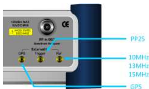
Figure 204 Connection ports for external reference clock
