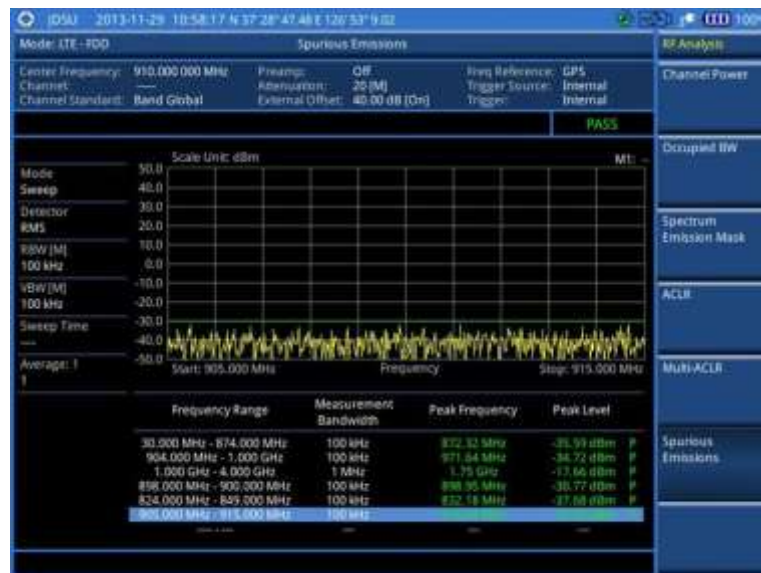
Figure 118 Spurious emissions measurement with LTE-FDD signal analyzer
