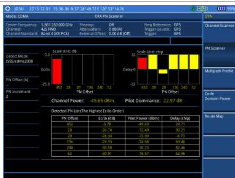
Figure 219 PN scanner measurement with CDMA OTA signal analyzer
