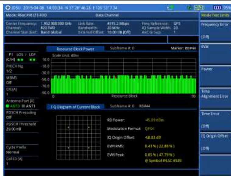
Figure 363 Data channel measurement with RFoCPRI LTE-FDD signal analyzer
