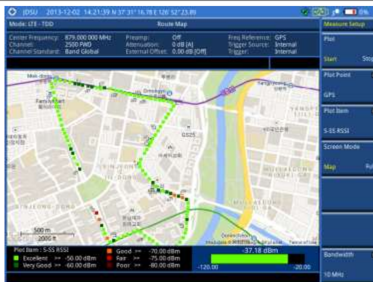
Figure 195 Route map measurement (P-SS Power) with LTE-TDD OTA signal analyzer
