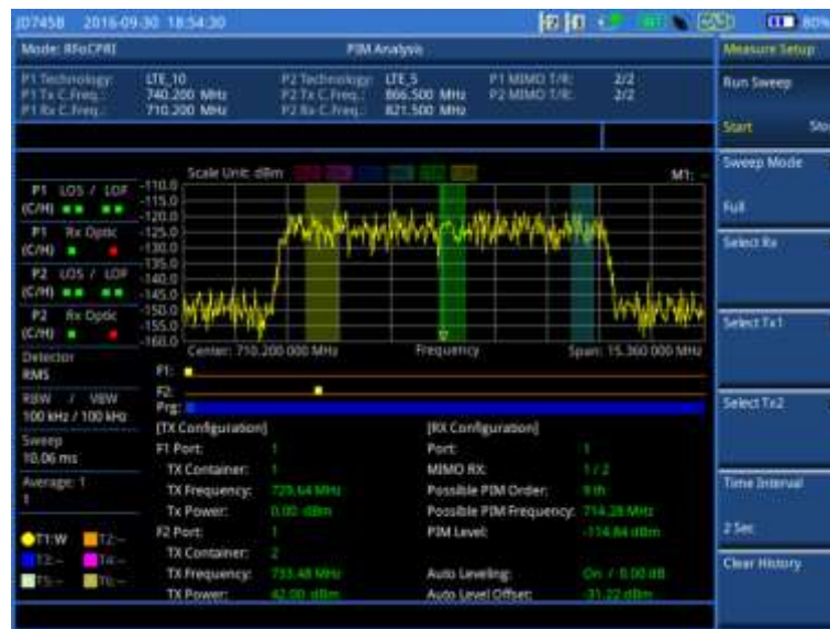
Figure 399 Example of Sweep mode PIM Analysis in BBU emulation
