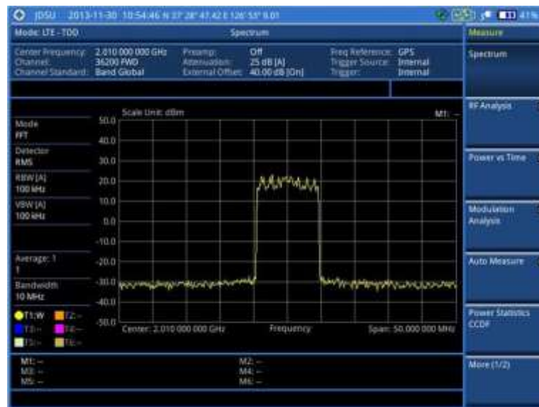
Figure 161 Spectrum measurement screen with LTE-TDD signal analyzer
