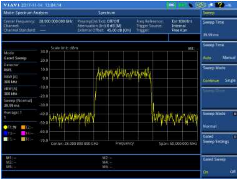
Figure 18 Gated sweep measurement with spectrum analyzer (on 28 GHz downconverter)
