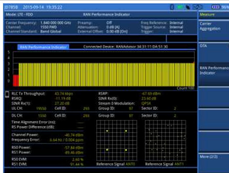
Figure 153 RAN performance indicator with LTE-FDD signal analyzer
