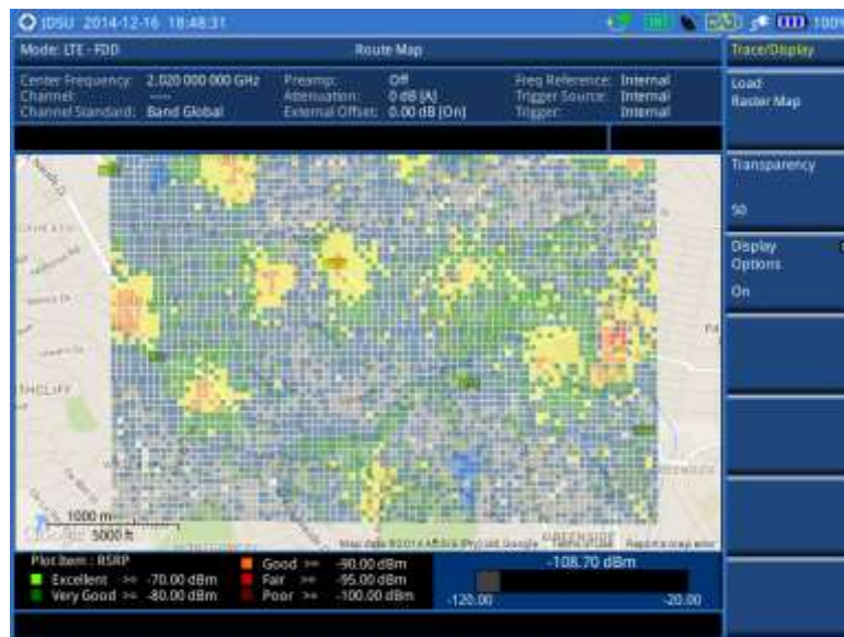
Figure 152 Raster image overlaid on the base map with LTE-FDD OTA signal analyzer
