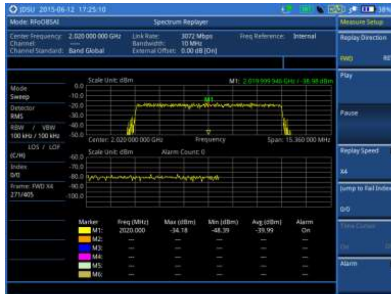
Figure 411 RFoBSAI spectrum replay
