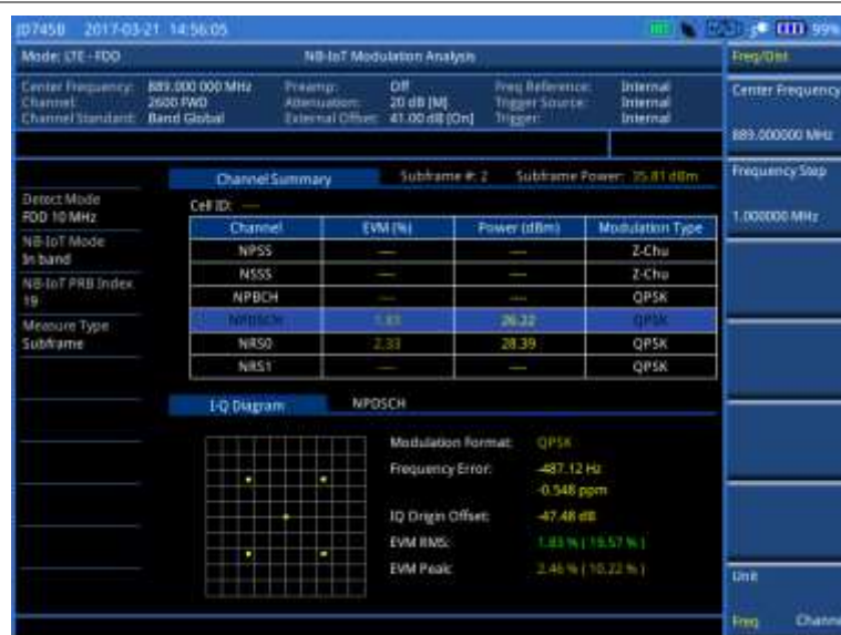
Figure 155 NB-IoT modulation measurement with LTE-FDD signal analyzer (Subframe 2)
