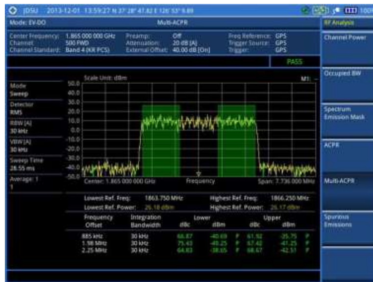
Figure 233 Multi-ACPR measurement with EV-DO signal analyzer
