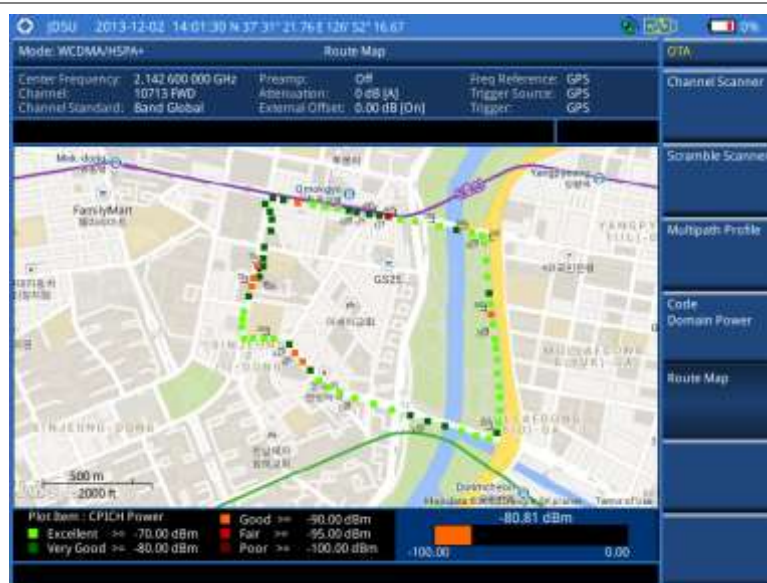
Figure 105 Route map measurement (CPICH Ec/Io) with WCDMA/HSPA+ OTA signal analyzer
