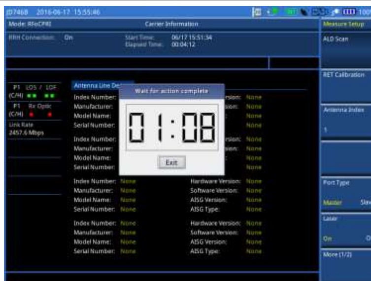
Figure 401 Example of ALD scanning in RET information
