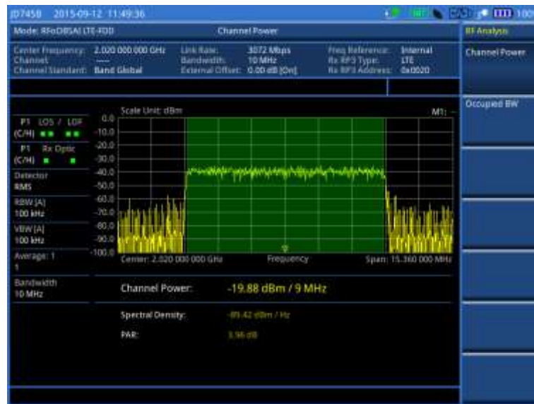
Figure 416 Channel power measurement with RFoBSAI LTE-FDD signal analyzer
