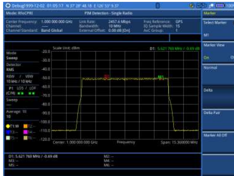
Figure 355 PIM detection of single radio
