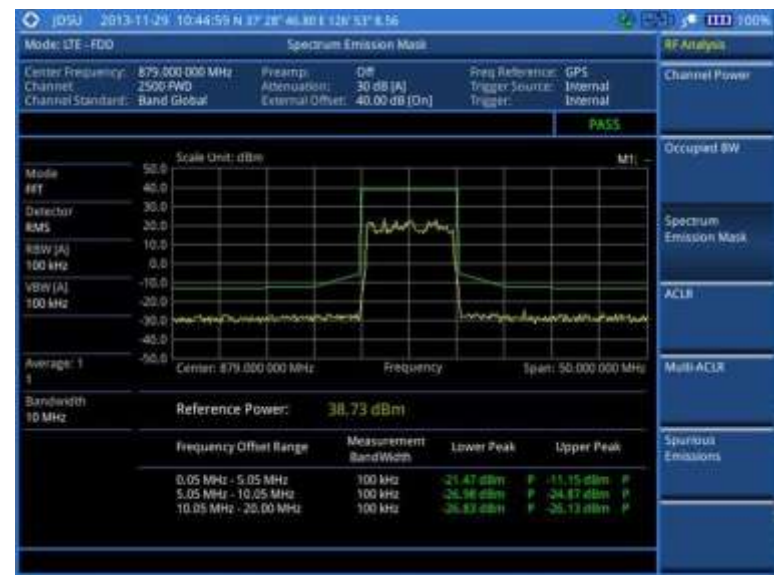
Figure 115 SEM measurement with LTE-FDD signal analyzer
