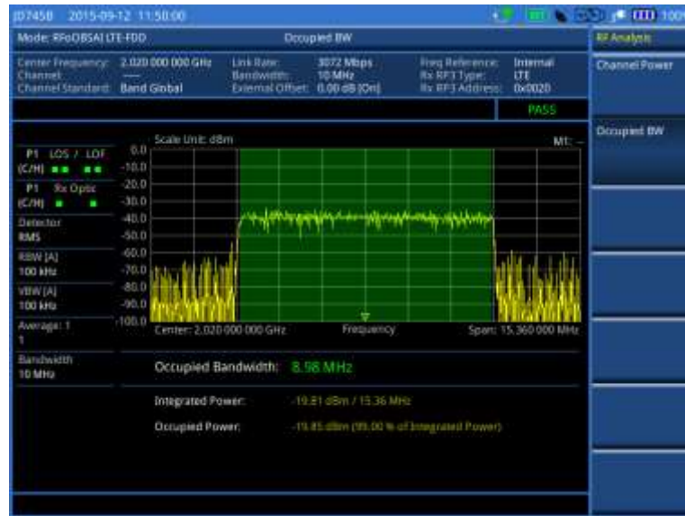
Figure 417 Occupied bandwidth measurement with RFoBSAI LTE-FDD signal analyzer
