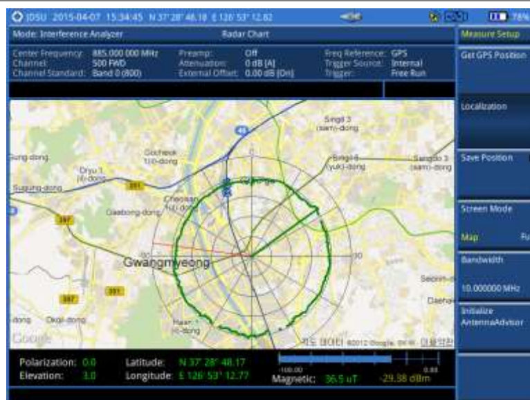
Figure 61 Localized RSSI data on the radar chart (on 28 GHz downconverter)
