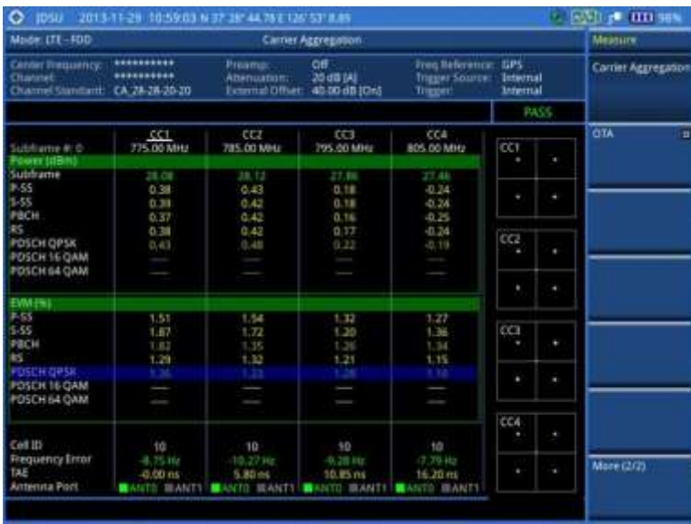
Figure 139 Carrier aggregation measurement with LTE-FDD signal analyzer (SA)
