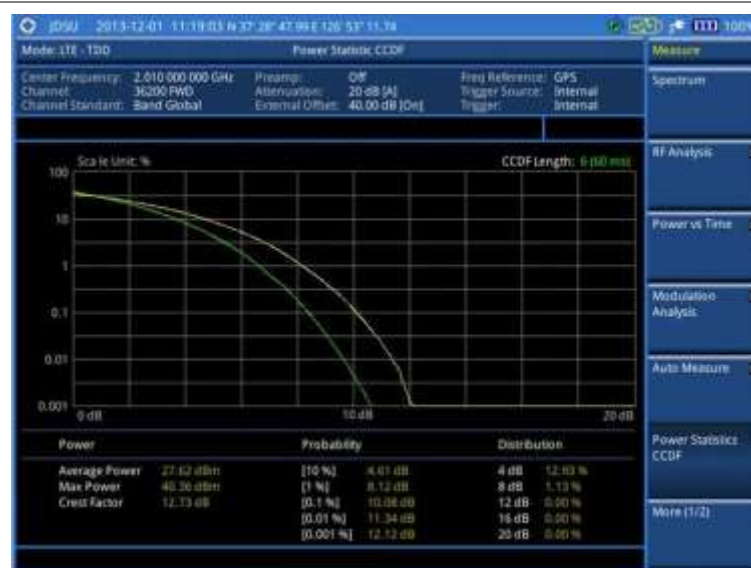
Figure 183 CCDF measurement with LTE-TDD signal analyzer
