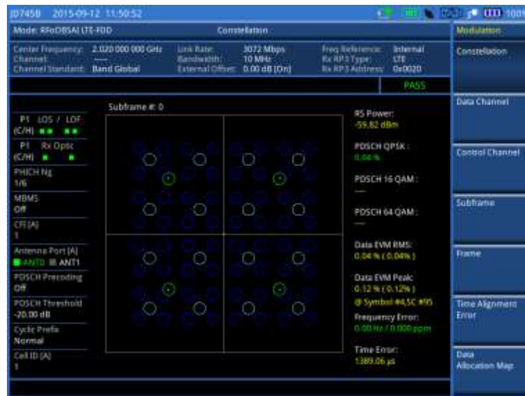
Figure 419 Constellation measurement with RFoBSAI LTE-FDD signal analyzer
