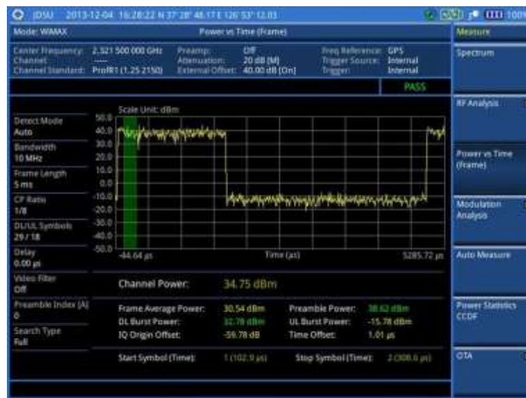
Figure 283 Power vs. time (frame) measurement with Mobile WiMAX signal analyzer
