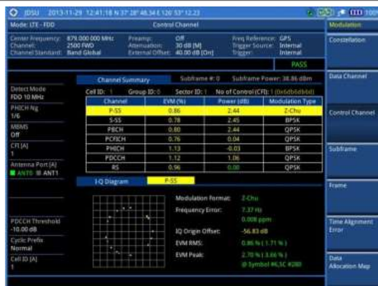
Figure 125 Control channel measurement with LTE-FDD signal analyzer
