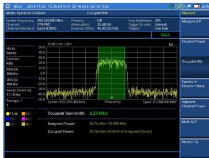
Figure 24 Occupied bandwidth measurement with spectrum analyzer (on 28 GHz downconverter)
