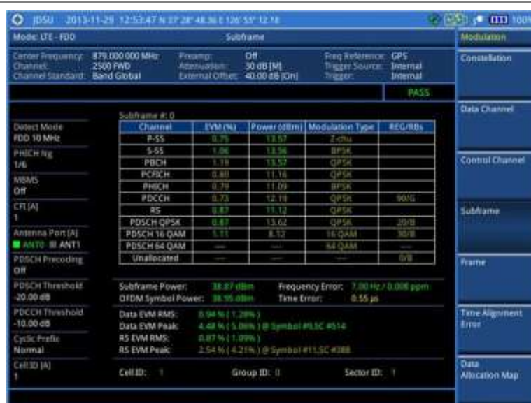
Figure 128 Subframe measurement with LTE-FDD signal analyzer (Chart On)
