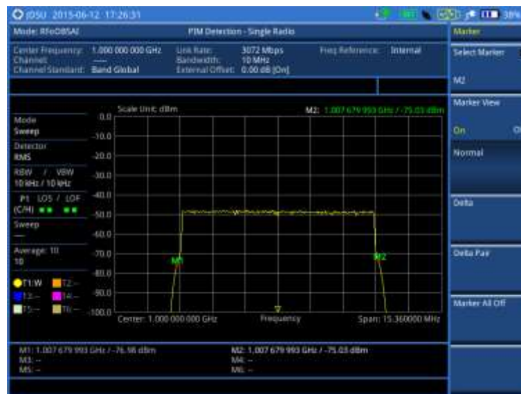
Figure 413 PIM detection of single radio
