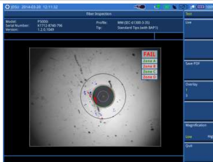
Figure 444 Analyzed fiber image and fiber inspection result
