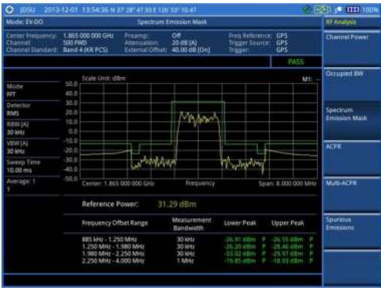
Figure 231 SEM measurement with EV-DO signal analyzer
