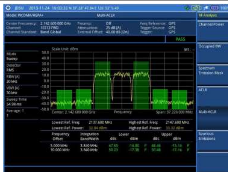
Figure 91 Multi-ACLR measurement with WCDMA/HSPA+ signal analyzer
