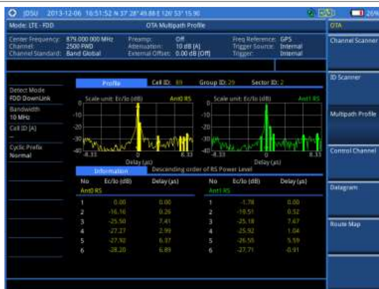
Figure 142 Multipath profile measurement with LTE-FDD OTA signal analyzer
