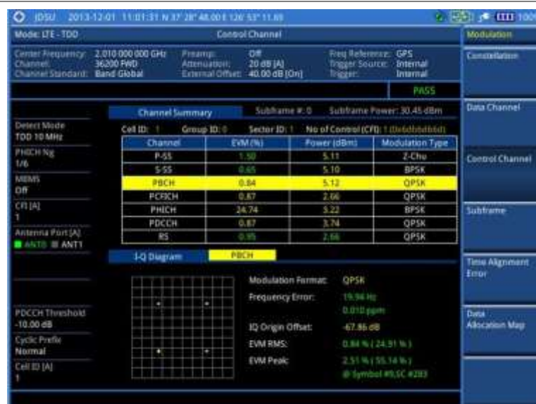
Figure 174 Control channel measurement with LTE-TDD signal analyzer
