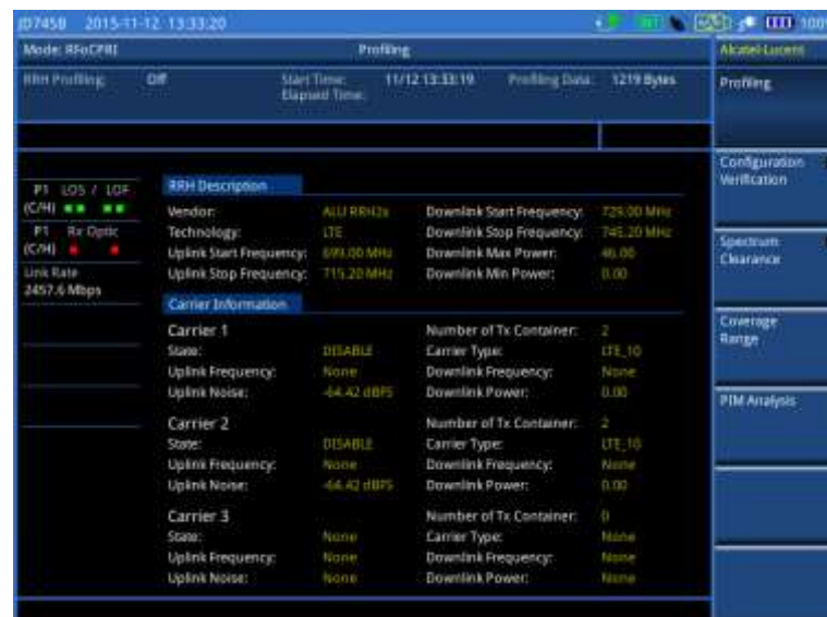
Figure 384 Example of RRH profiling results with carrier information
