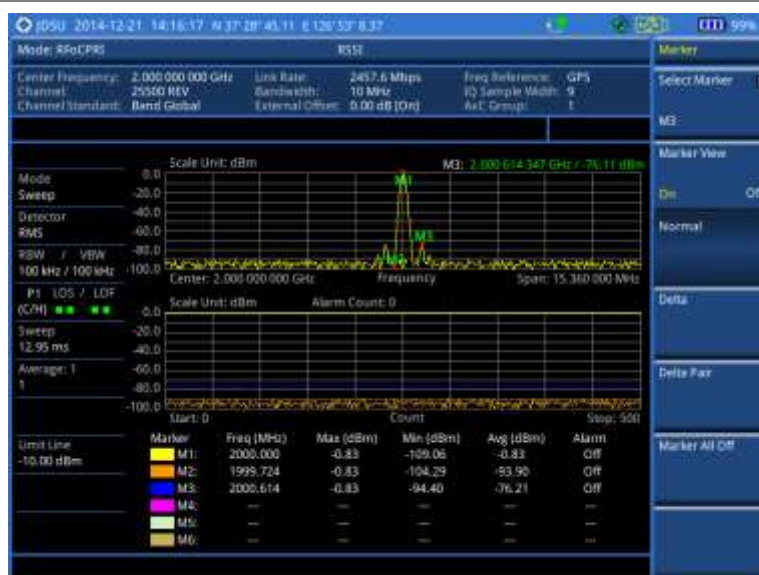
Figure 351 RFoCPRI interference measurement in RSSI
