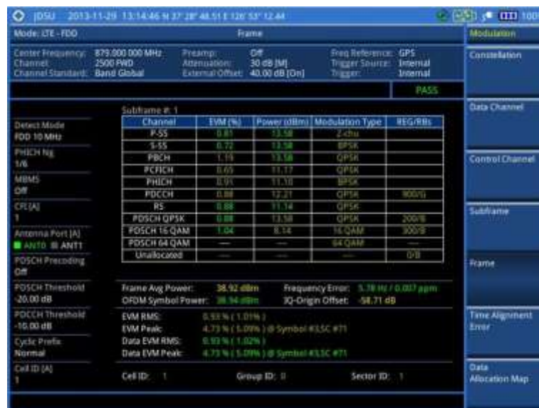
Figure 130 Frame measurement with LTE-FDD signal analyzer
