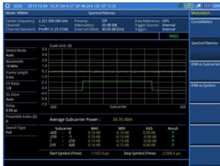
Figure 285 Spectral flatness measurement with Mobile WiMAX signal analyzer
