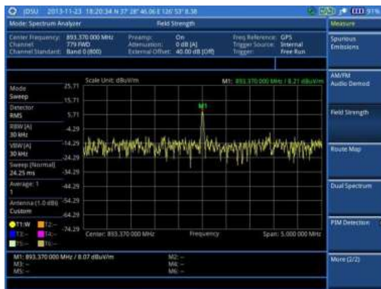
Figure 35 Field strength measurement with spectrum analyzer
