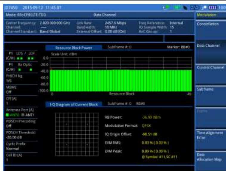
Figure 376 Data channel measurement with RFoCPRI LTE-FDD signal analyzer
