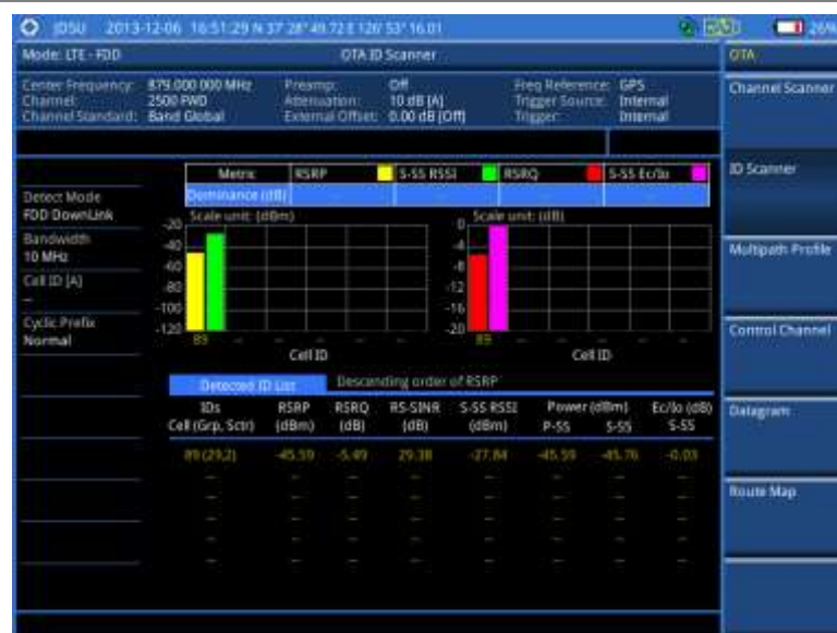
Figure 141 ID scanner measurement with LTE-FDD OTA signal analyzer
