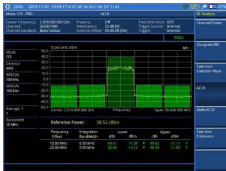
Figure 165 ACLR measurement with LTE-TDD signal analyzer
