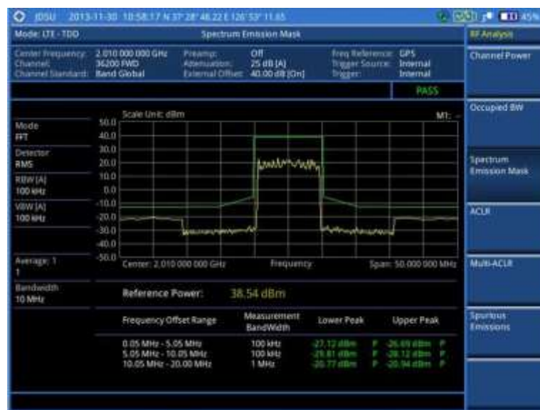
Figure 164 SEM measurement with LTE-TDD signal analyzer
