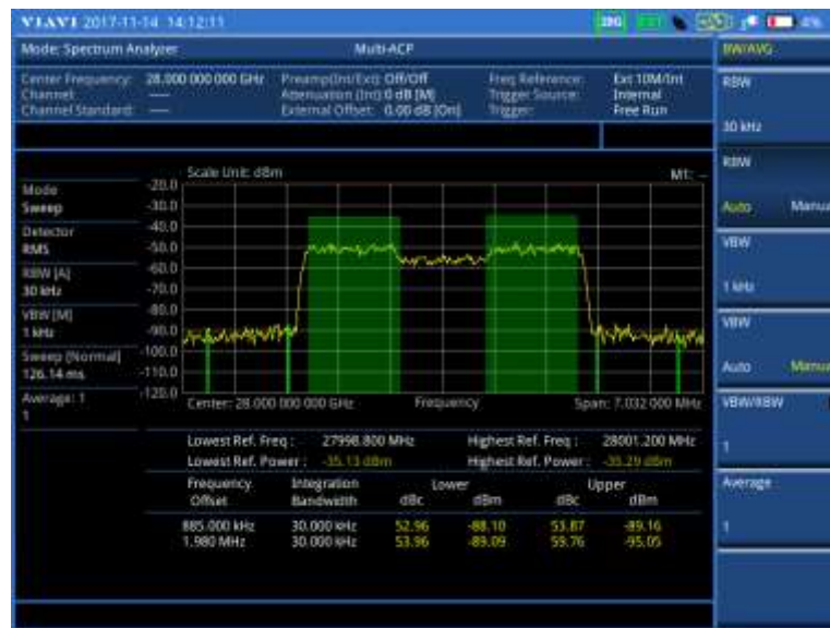
Figure 30 Multi-ACP measurement with spectrum analyzer (on 28 GHz downconverter)
