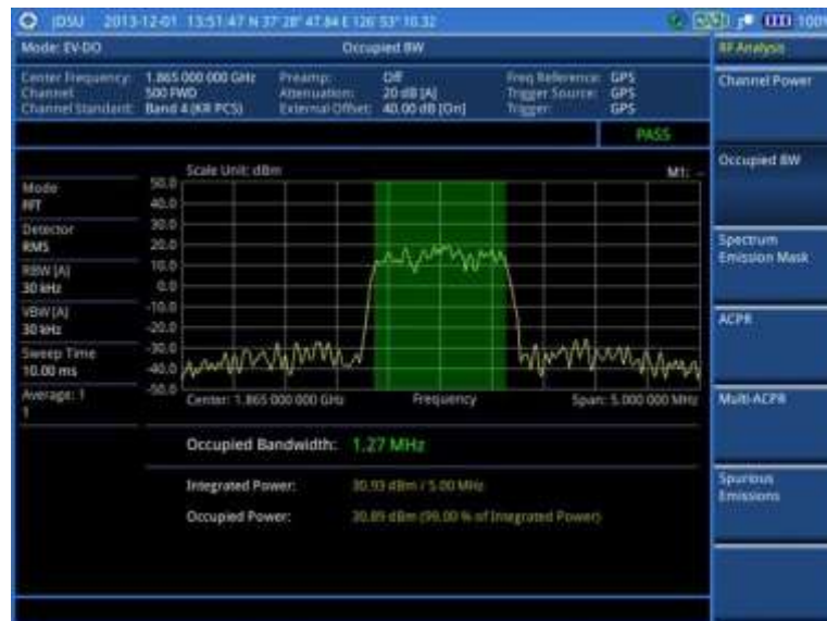
Figure 230 Occupied bandwidth measurement with EV-DO signal analyzer
