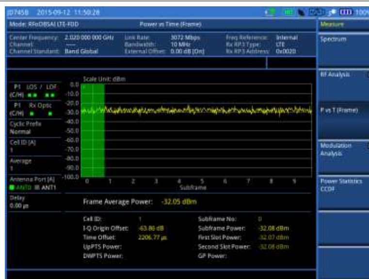
Figure 418 Power vs. time (frame) measurement with RFoBSAI LTE-FDD signal analyzer
