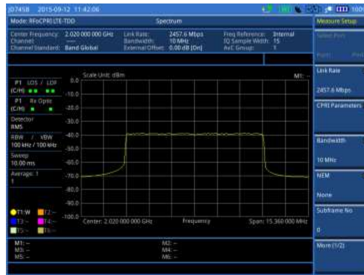
Figure 371 Spectrum measurement with RFoCPRI LTE-TDD signal analyzer
