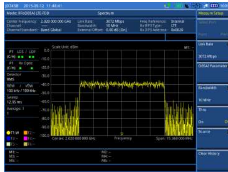
Figure 415 Spectrum measurement with RFoBSAI LTE-FDD signal analyzer
