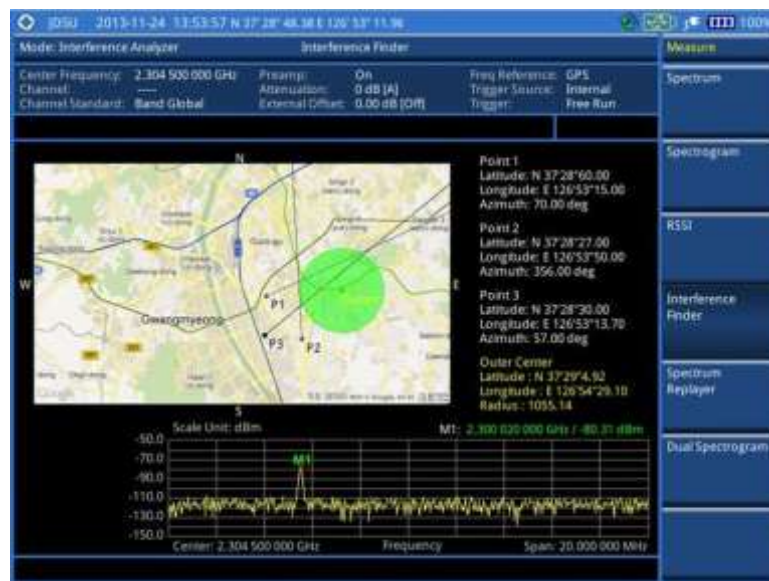
Figure 55 Interference finder measurement in map view (on 28 GHz downconverter)
