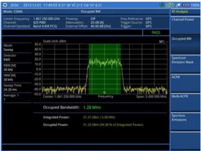
Figure 207 Occupied bandwidth measurement with CDMA signal analyzer
