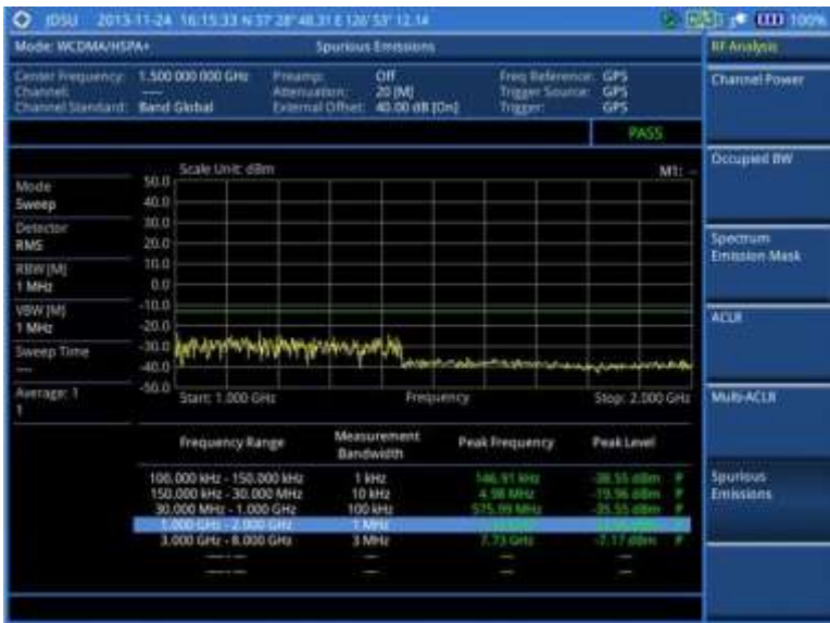
Figure 92 Spurious emissions measurement with WCDMA/HSPA+ signal analyzer
