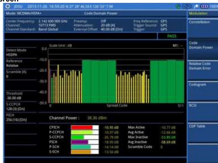
Figure 94 Code domain power measurement with WCDMA/HSPA+ signal analyzer
