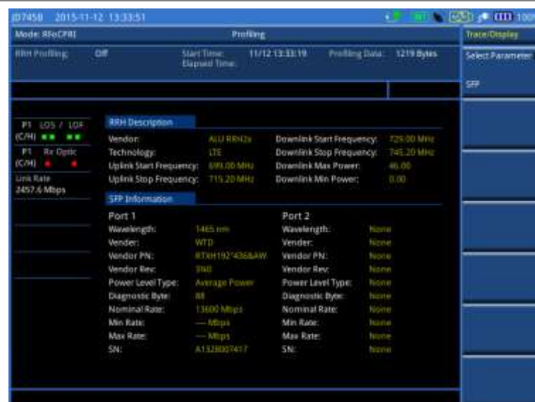
Figure 386 Example of RRH profiling results with SFP information
