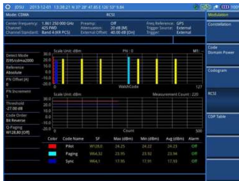
Figure 215 RCSI measurement with CDMA signal analyzer
