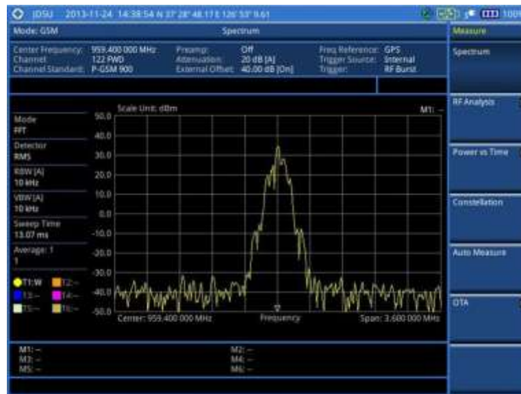
Figure 66 Spectrum measurement screen with GSM signal analyzer
