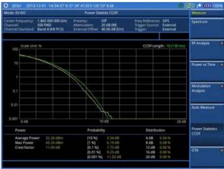
Figure 242 CCDF measurement with EV-DO signal analyzer
