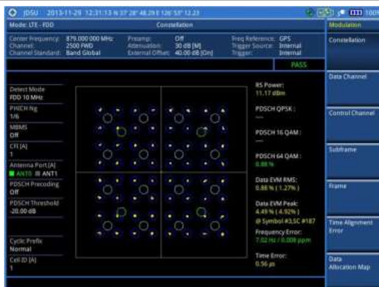
Figure 120 Constellation measurement with LTE-FDD signal analyzer
