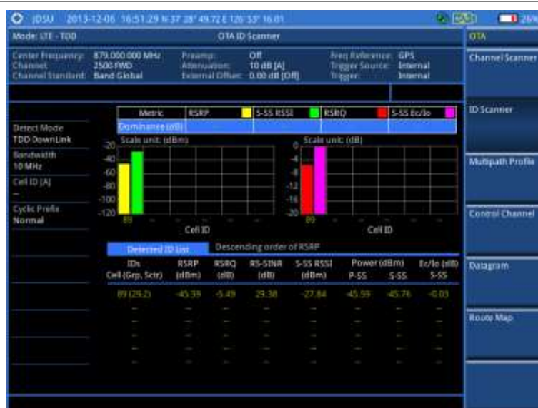
Figure 187 ID scanner measurement with LTE-TDD OTA signal analyzer
