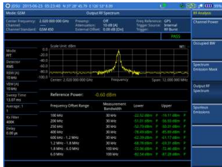
Figure 70 Output RF spectrum measurement with GSM signal analyzer
