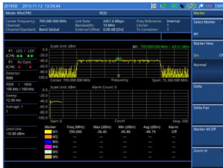
Figure 397 Example of RSSI in BBU emulation
