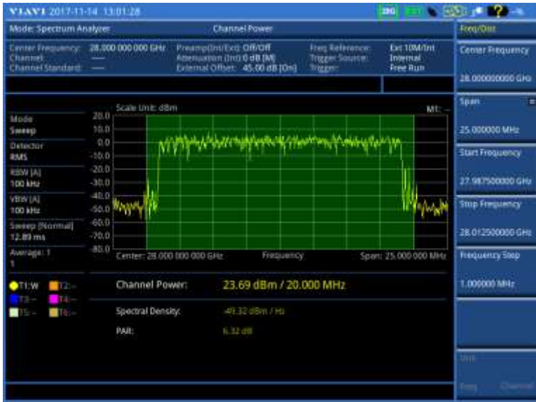
Figure 21 Channel power measurement with spectrum analyzer (on 28 GHz downconverter)
