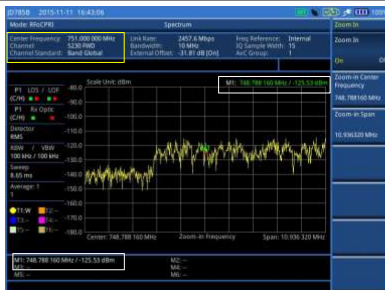
Figure 352 Zoomed-in spectrum view in RFoCPRI interference analyzer
