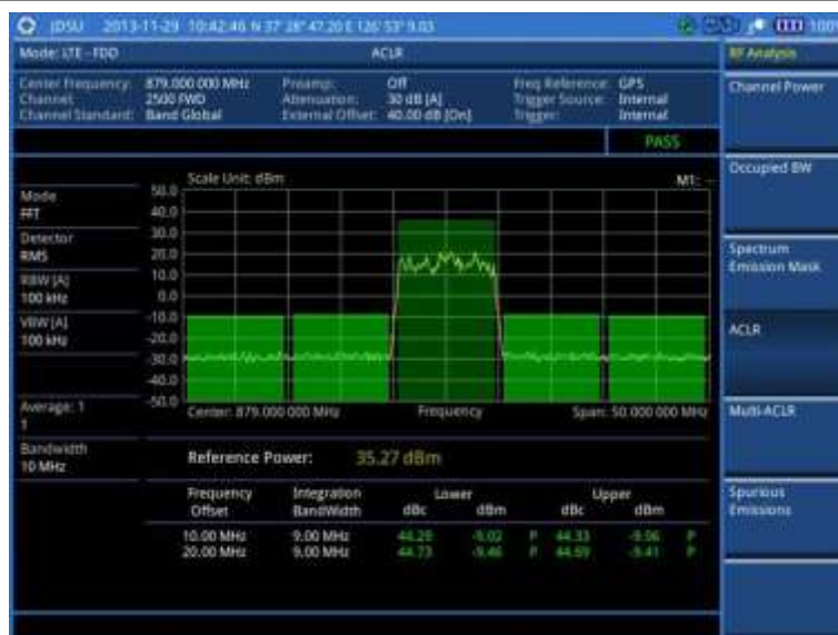
Figure 116 ACLR measurement with LTE-FDD signal analyzer
