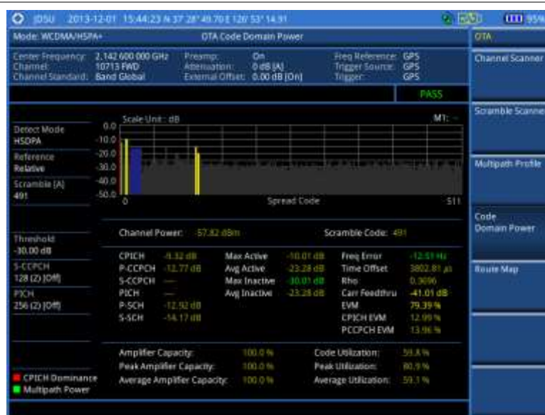
Figure 103 Code domain power measurement with WCDMA/HSPA+ OTA signal analyzer
