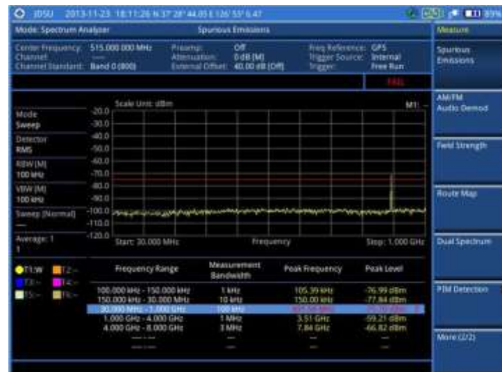
Figure 31 Spurious emissions measurement with spectrum analyzer
