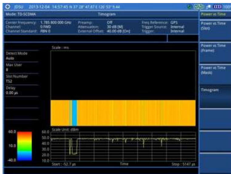
Figure 263 Timogram with TD-SCDMA signal analyzer
