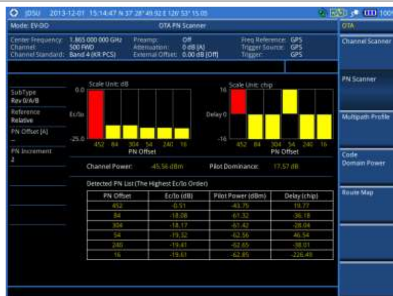
Figure 244 PN scanner measurement with EV-DO OTA signal analyzer
