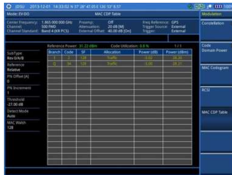
Figure 241 MAC CDP Table measurement with EV-DO signal analyzer
