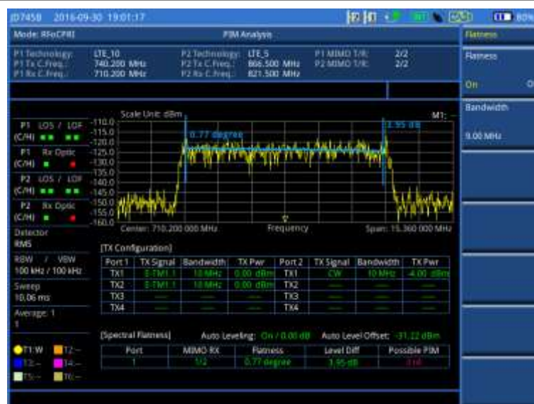
Figure 400 Example of Wideband Mode PIM analysis in BBU emulation
