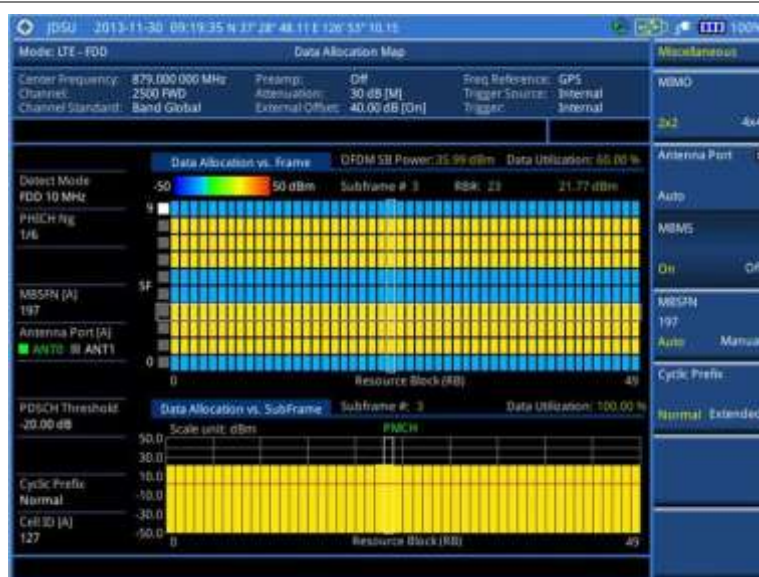
Figure 134 Data allocation map measurement with LTE-FDD signal analyzer (MBMS On)
