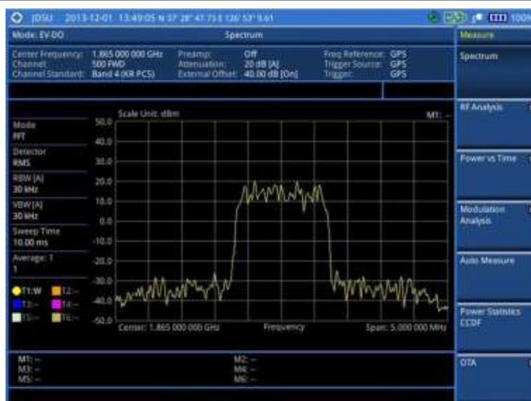
Figure 228 Spectrum measurement screen with EV-DO signal analyzer
