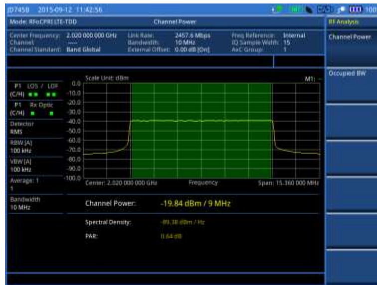
Figure 374 Channel power measurement with RFoCPRI LTE-TDD signal analyzer
