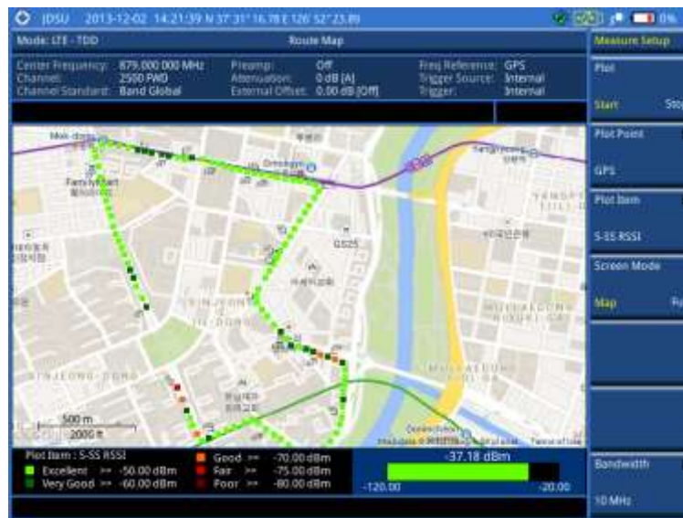
Figure 196 Route map measurement (S-SS RSSI) with LTE-TDD OTA signal analyzer
