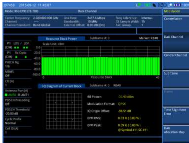
Figure 378 Data channel measurement with RFoCPRI LTE-FDD signal analyzer
