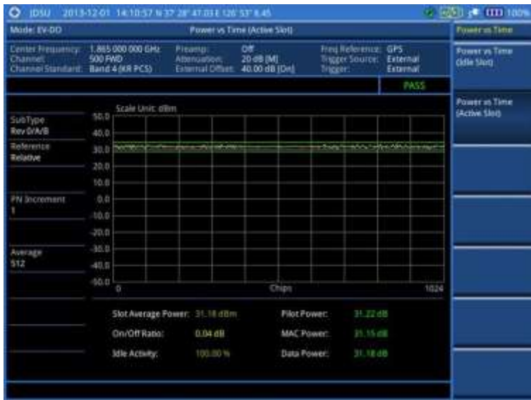
Figure 238 Power vs. time (active slot) measurement with EV-DO signal analyzer
