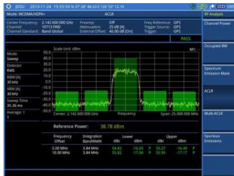
Figure 91 ACLR measurement with WCDMA/HSPA+ signal analyzer
