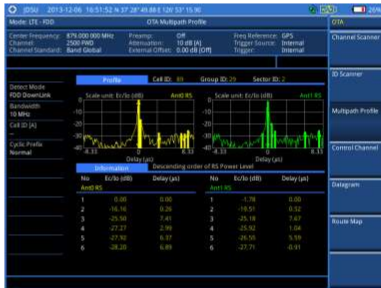
Figure 145 Multipath profile measurement with LTE-FDD OTA signal analyzer
