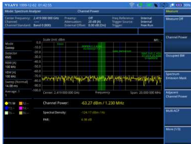
Figure 23 Wi-Fi SSID display in channel power measurement with spectrum analyzer
