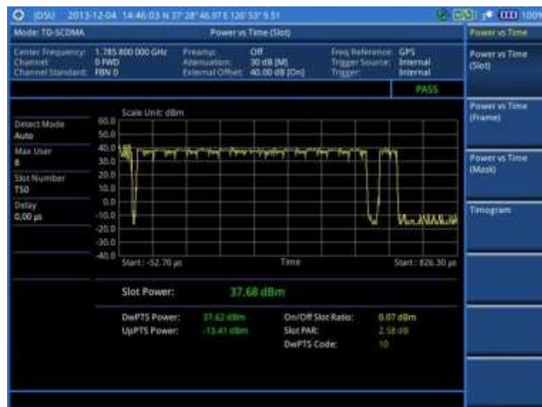
Figure 262 Power vs. time (slot) measurement with TD-SCDMA signal analyzer
