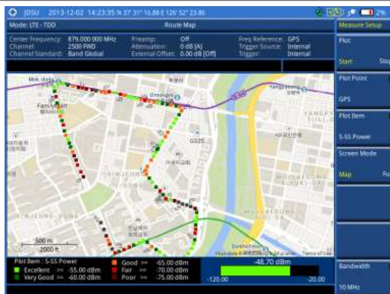
Figure 199 Route map measurement (S-SS Ec/Io) with LTE-TDD OTA signal analyzer
