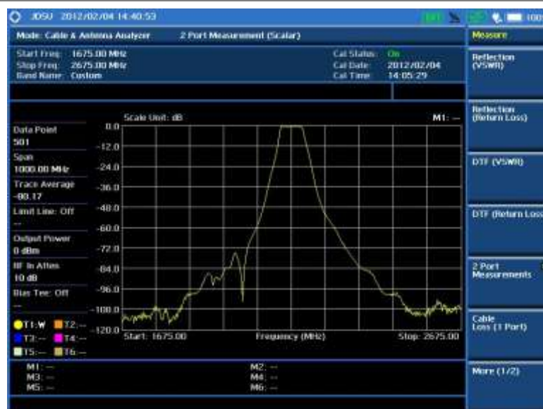
Figure 331 2-port scalar measurement
