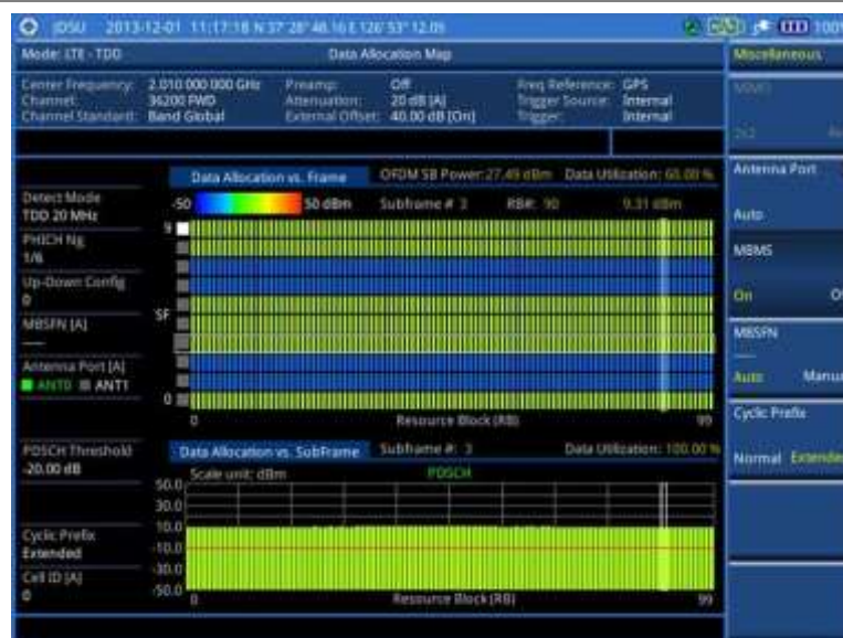
Figure 182 Data allocation map measurement with LTE-TDD signal analyzer (MBMS On)
