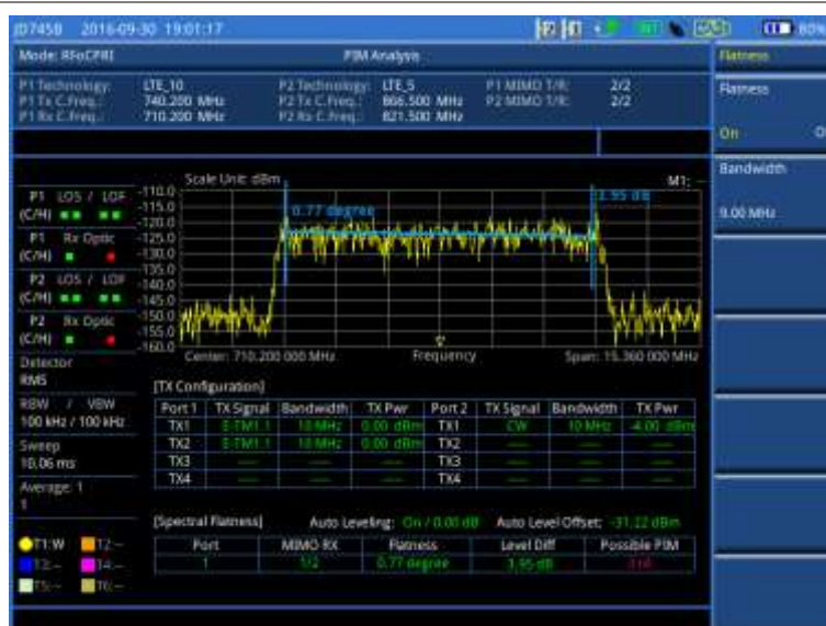
Figure 404 Example of Wideband Mode PIM analysis in BBU emulation
