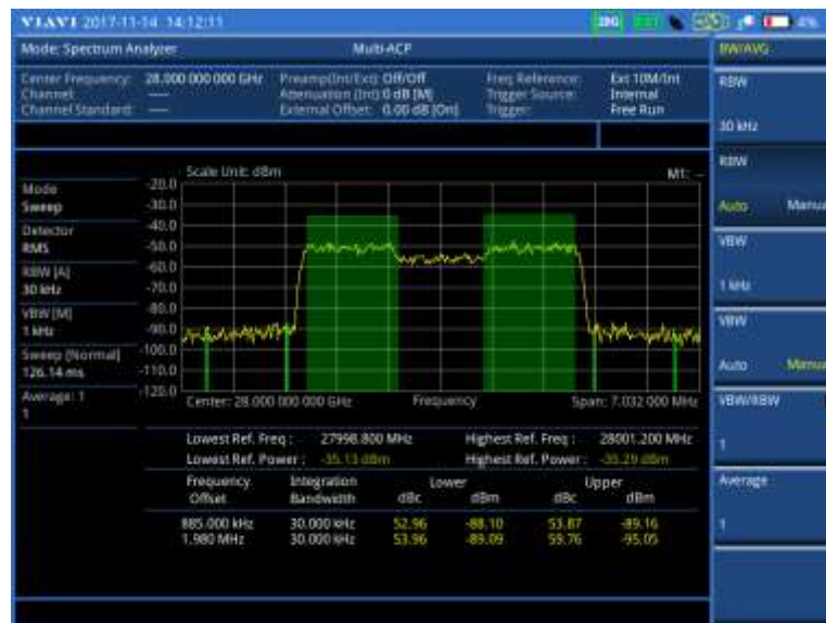
Figure 31 Multi-ACP measurement with spectrum analyzer (on 28 GHz downconverter)
