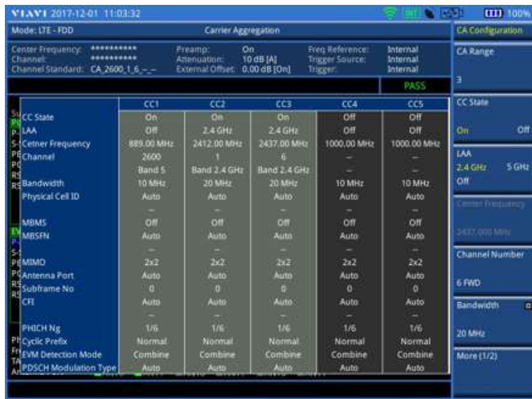
Figure 139 LAA (Licensed Assited Acss) measurement with LTE-FDD signal analyzer
