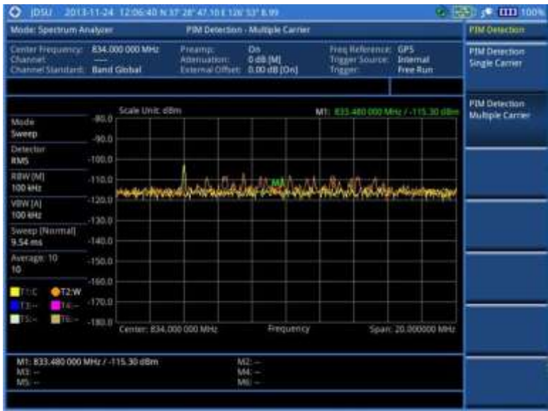
Figure 42 PIM detection for multiple carriers
