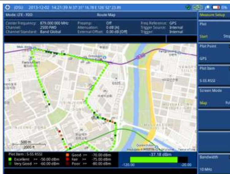
Figure 152 Route map measurement (P-SS Power) with LTE-FDD OTA signal analyzer
