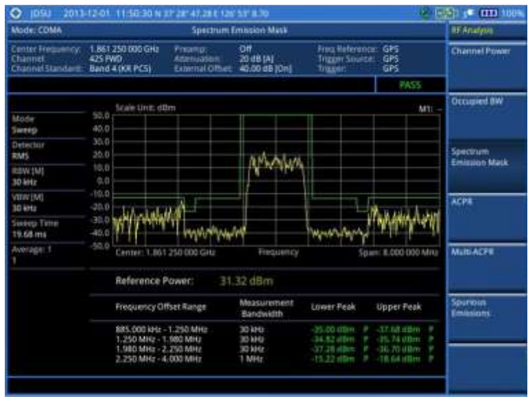
Figure 210 SEM measurement with CDMA signal analyzer
