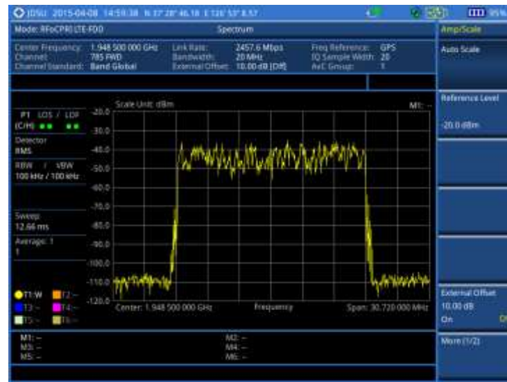
Figure 359 Spectrum measurement with RFoCPRI LTE-FDD signal analyzer
