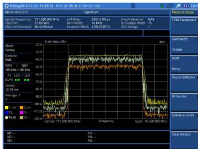
Figure 344 RFoCPRI spectrum analysis on LTE Uplink 10 MHz, antenna 1
