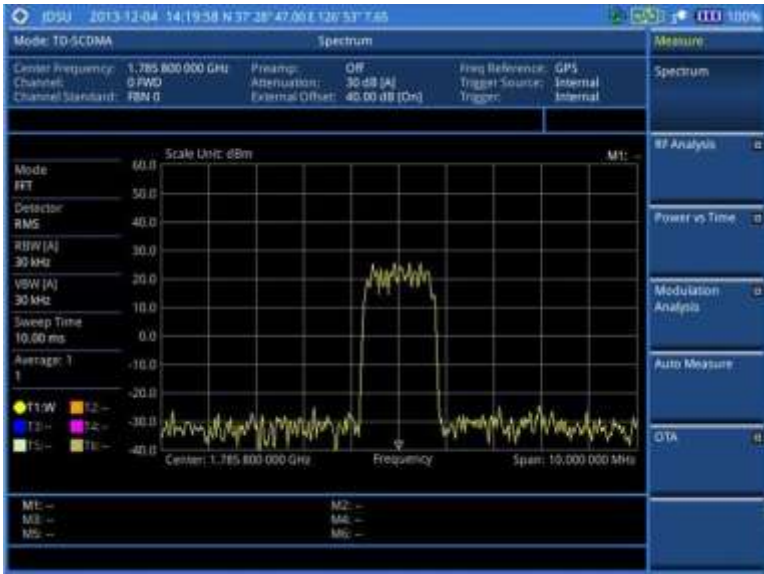
Figure 255 Spectrum measurement screen with TD-SCDMA signal analyzer
