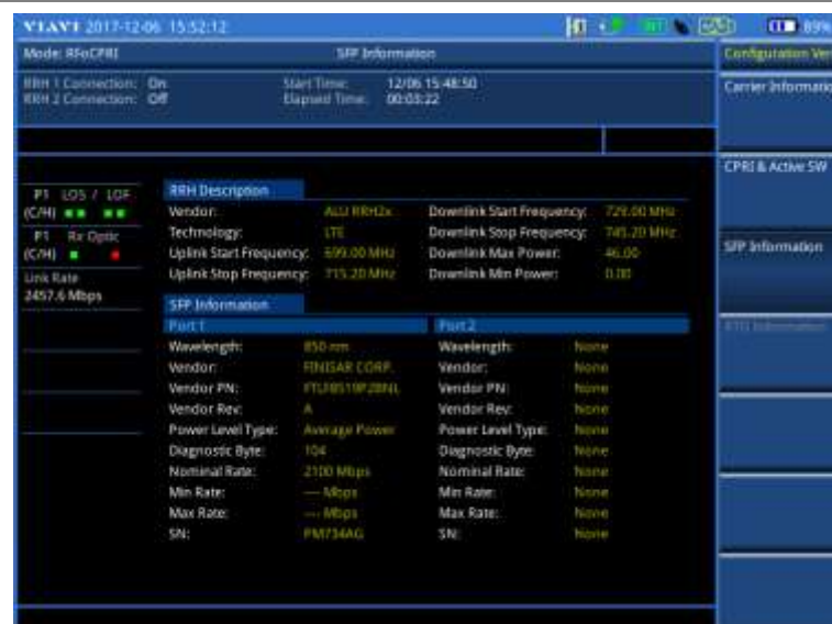
Figure 392 Example of verification of SFP information
