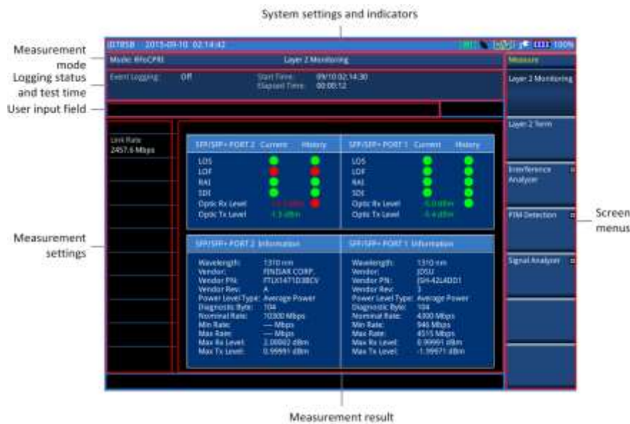
Figure 332 RFoCPRI analysis screen
