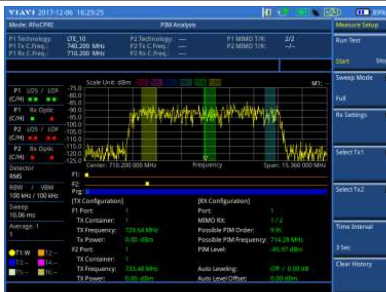
Figure 403 Example of multi port sweep mode PIM Analysis in BBU emulation
