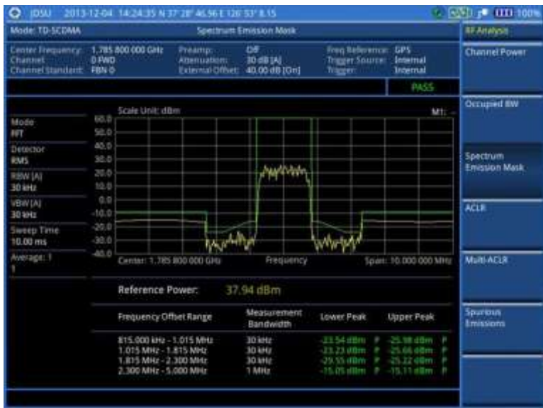
Figure 258 SEM measurement with TD-SCDMA signal analyzer
