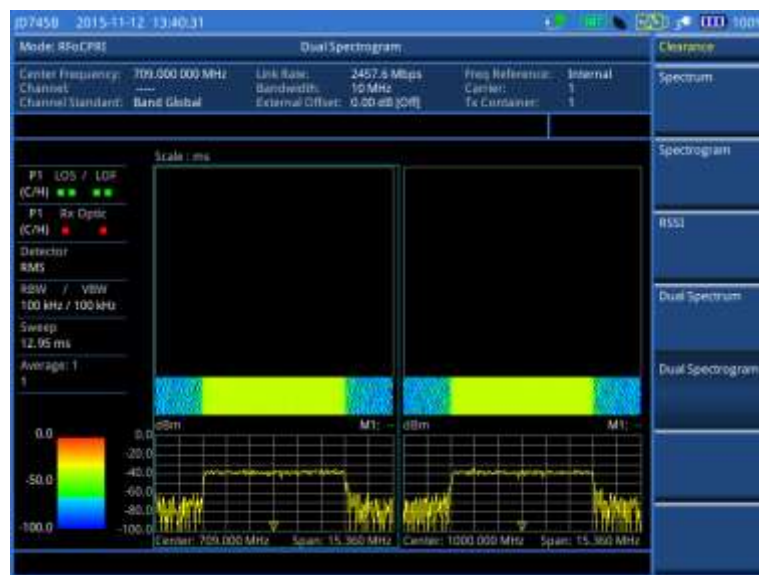
Figure 399 Example of dual spectrogram analysis in BBU emulation
