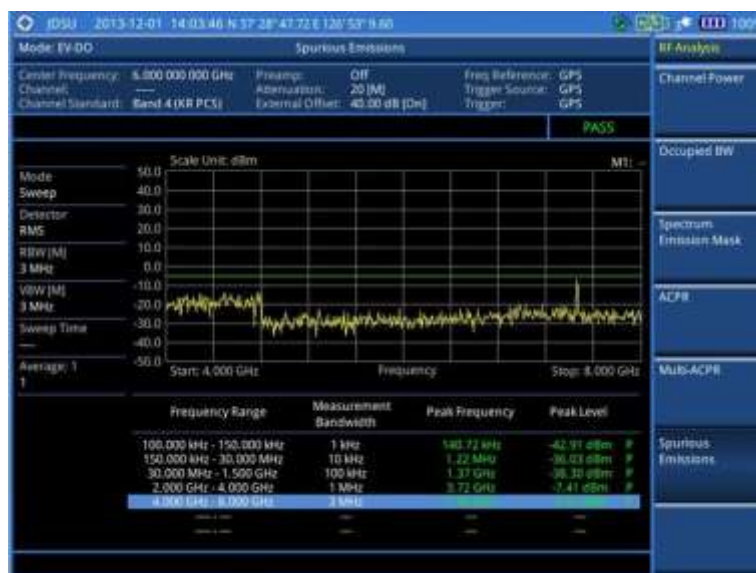
Figure 236 Spurious emissions measurement with EV-DO signal analyzer
