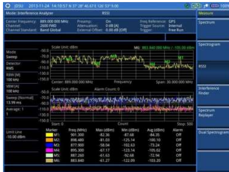
Figure 54 Interference measurement in RSSI (on 28 GHz downconverter)
