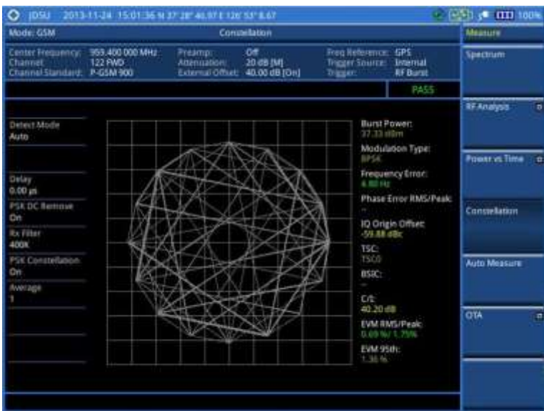
Figure 77 Constellation measurement (PSK on) with GSM signal analyzer
