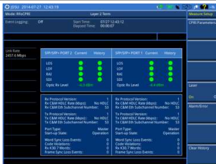
Figure 336 CPRI layer 2 term test
