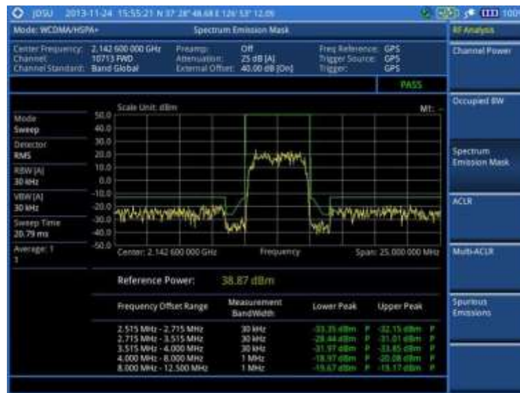
Figure 90 SEM measurement with WCDMA/HSPA+ signal analyzer
