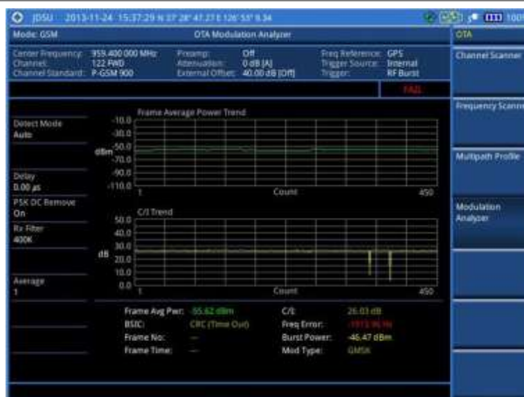
Figure 81 Modulation analyzer measurement with GSM OTA signal analyzer
