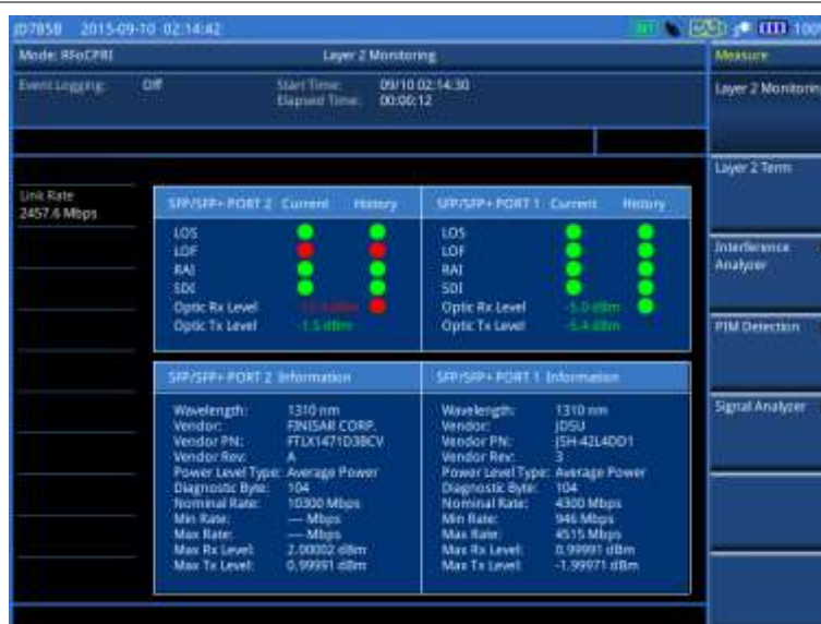
Figure 334 CPRI layer 2 monitoring
