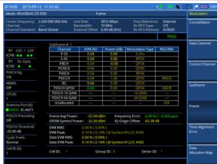
Figure 431 Frame measurement with RFoBSAI LTE-FDD signal analyzer
