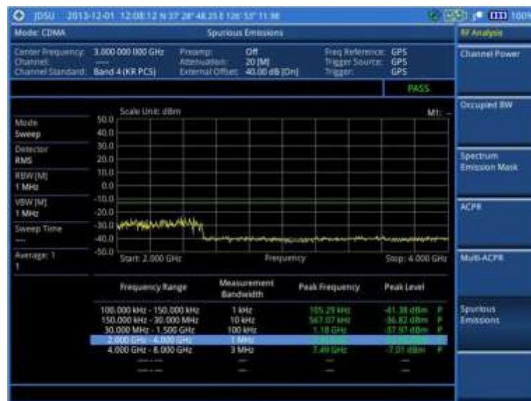
Figure 213 Spurious emissions measurement with CDMA signal analyzer
