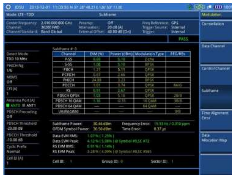
Figure 177 Subframe measurement with LTE-TDD signal analyzer
