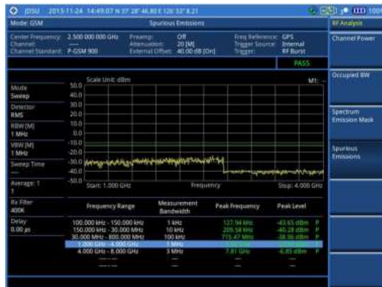
Figure 72 Spurious emissions measurement with GSM signal analyzer
