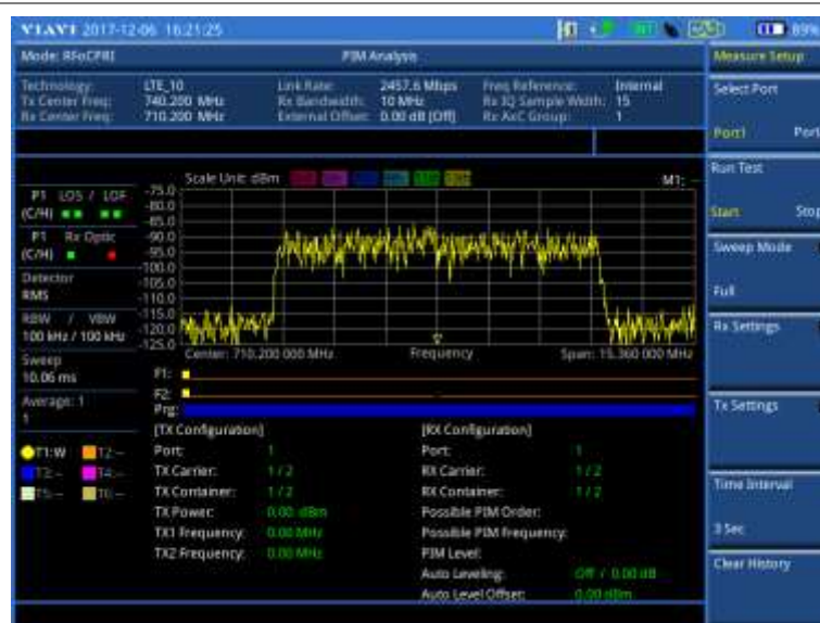
Figure 402 Example of single port sweep mode PIM Analysis in BBU emulation
