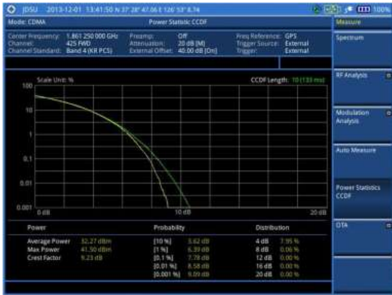
Figure 219 CCDF measurement with CDMA signal analyzer
