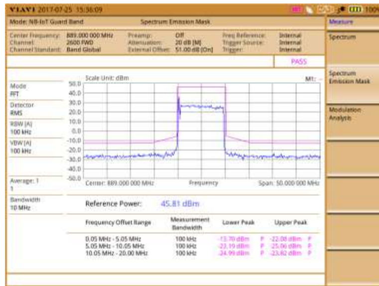
Figure 301 Spectrum Emission Mask measurement screen
