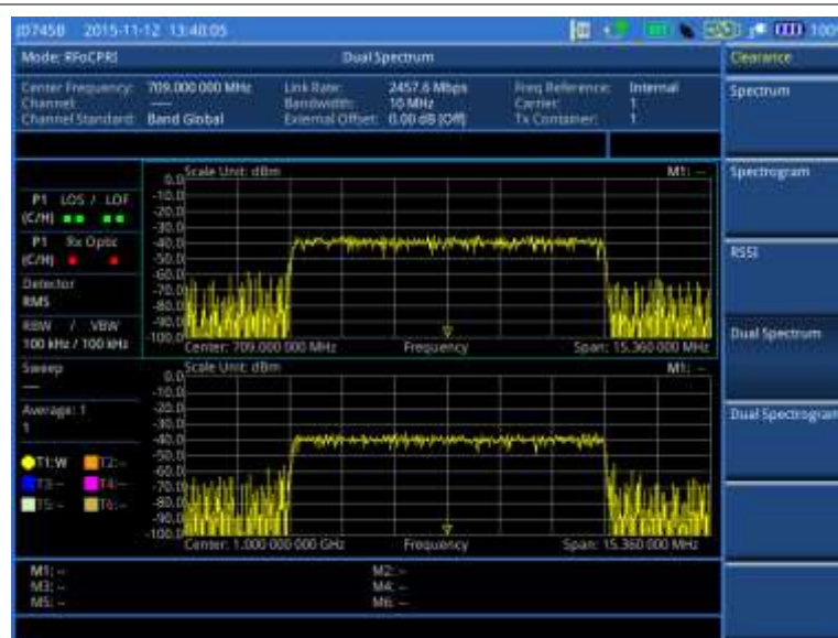
Figure 397 Example of dual spectrum analysis in BBU emulation
