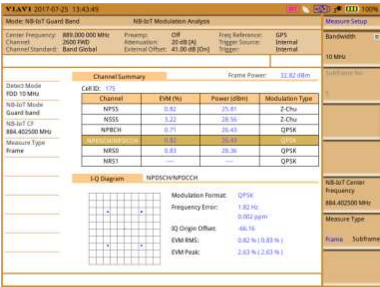
Figure 303 NB-IoT Guard Band Modulation Analysis measurement screen (Subframe 0- NPBCH)
