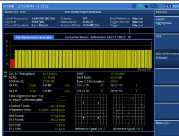
Figure 156 RAN performance indicator with LTE-FDD signal analyzer
