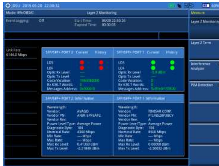
Figure 412 OBSAI RP3 layer 2 monitoring
