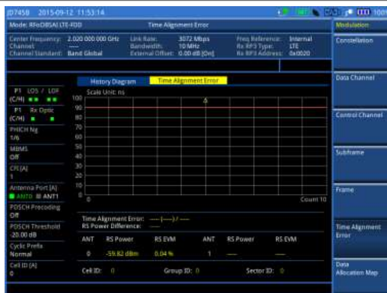
Figure 432 Time alignment error measurement with RFoBSAI LTE-FDD signal analyzer
