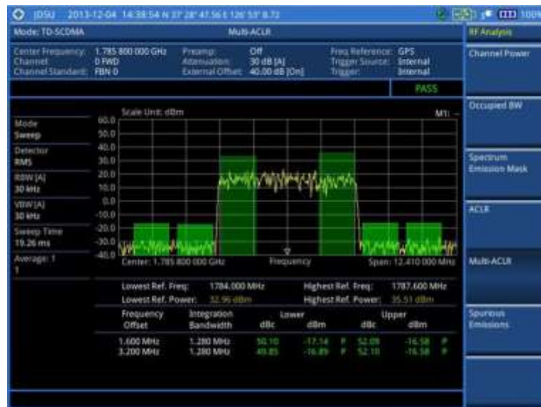
Figure 260 Multi-ACLR measurement with TD-SCDMA signal analyzer
