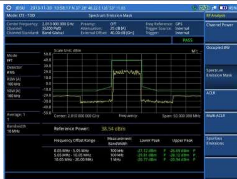
Figure 165 SEM measurement with LTE-TDD signal analyzer
