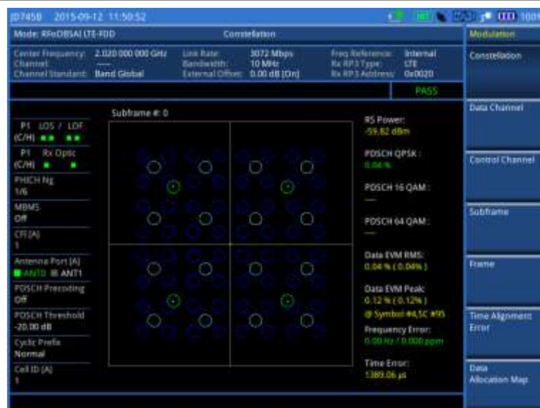
Figure 427 Constellation measurement with RFoBSAI LTE-FDD signal analyzer
