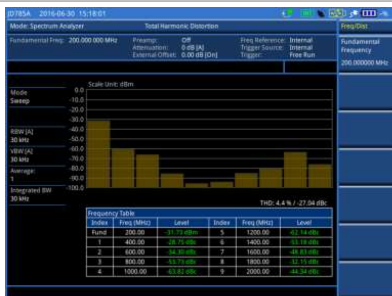
Figure 43 Total harmonic distortion screen
