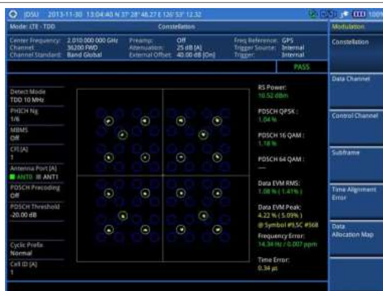
Figure 171 Constellation measurement with LTE-TDD signal analyzer
