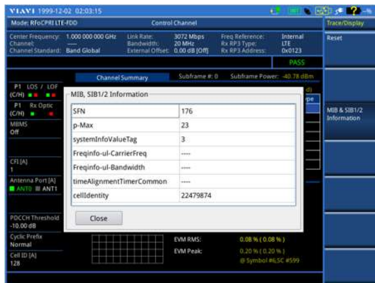
Figure 366 Decoded MIB & SIB1/2 information in RFoCPRI LTE-FDD signal analyzer
