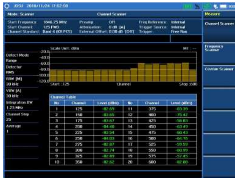
Figure 439 Channel scanner measurement
