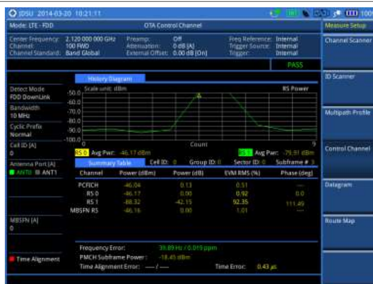
Figure 146 Control channel measurement with LTE-FDD OTA signal analyzer
