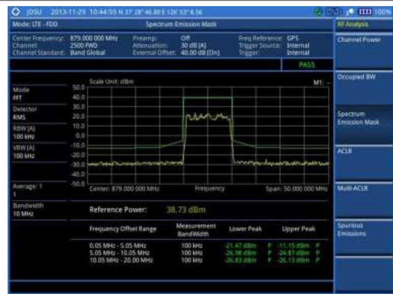
Figure 116 SEM measurement with LTE-FDD signal analyzer
