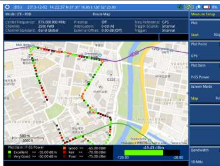
Figure 152 Route map measurement (P-SS Power) with LTE-FDD OTA signal analyzer
