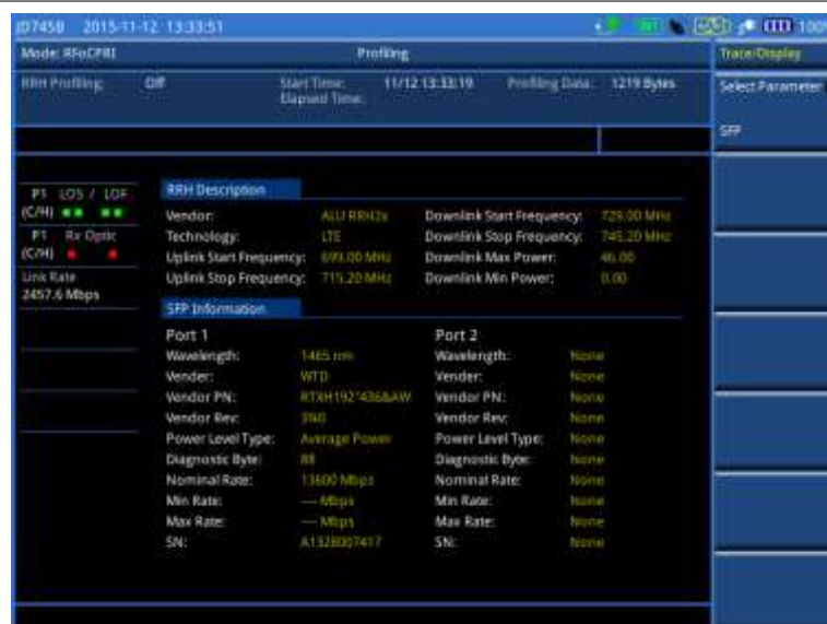
Figure 388 Example of RRH profiling results with SFP information
