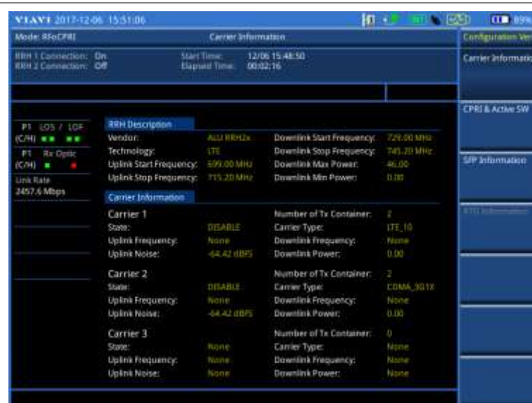
Figure 390 Example of verification of carrier configuration
