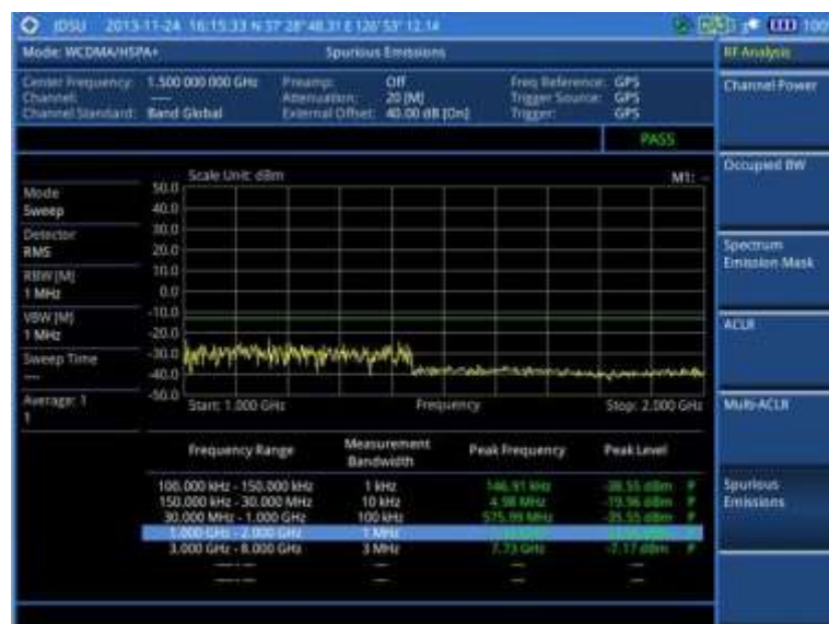
Figure 93 Spurious emissions measurement with WCDMA/HSPA+ signal analyzer
