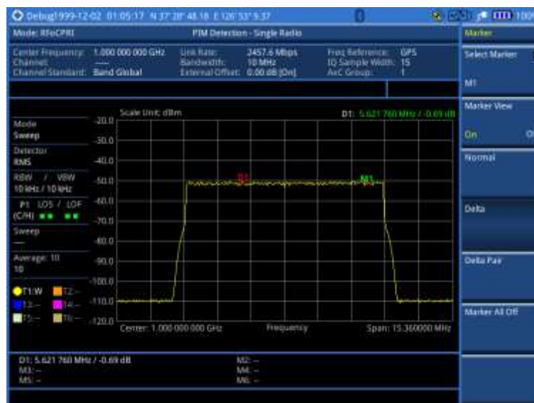
Figure 357 PIM detection of single radio
