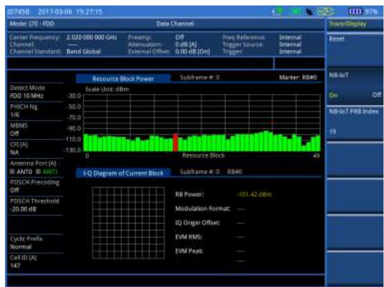
Figure 125 Data channel measurement with LTE-FDD signal analyzer (NB-IoT On)
