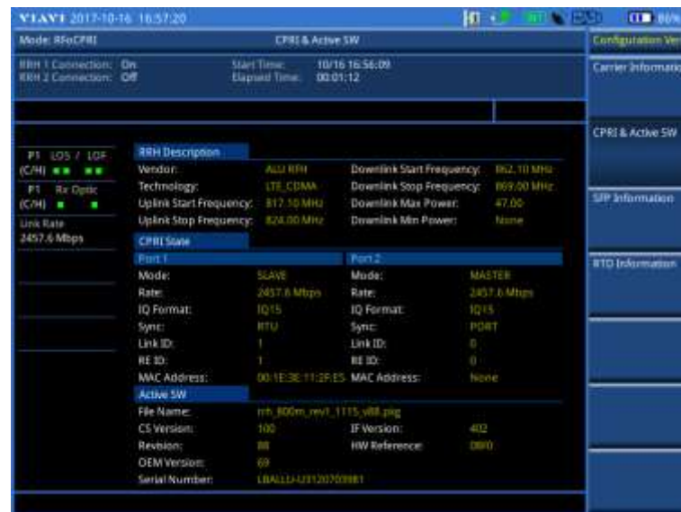
Figure 391 Example of verification of CPRI state and active software
