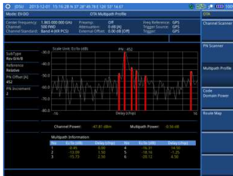
Figure 247 Multipath profile measurement with EV-DO OTA signal analyzer
