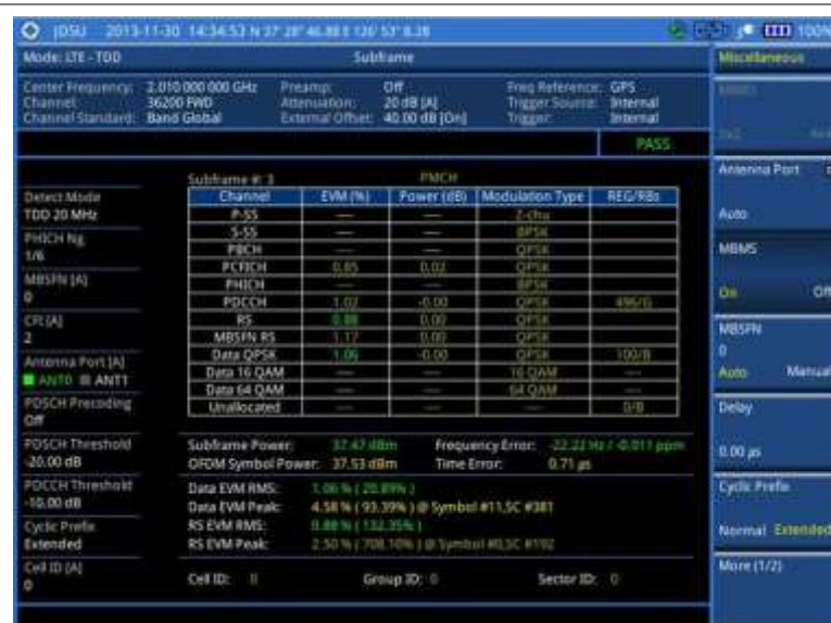
Figure 179 Subframe measurement with LTE-TDD signal analyzer (MBMS On)
