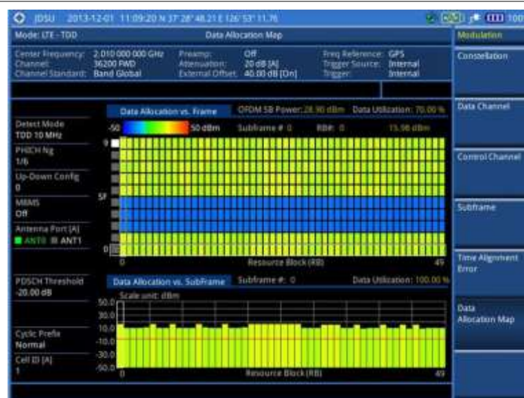
Figure 181 Data allocation map measurement with LTE-TDD signal analyzer
