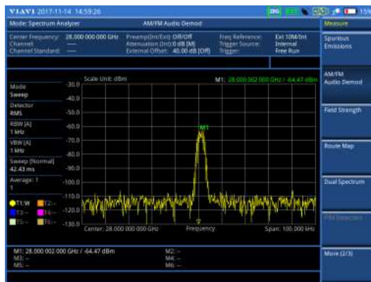
Figure 35 AM/FM audio demodulation with spectrum analyzer (on 28 GHz downconverter)
