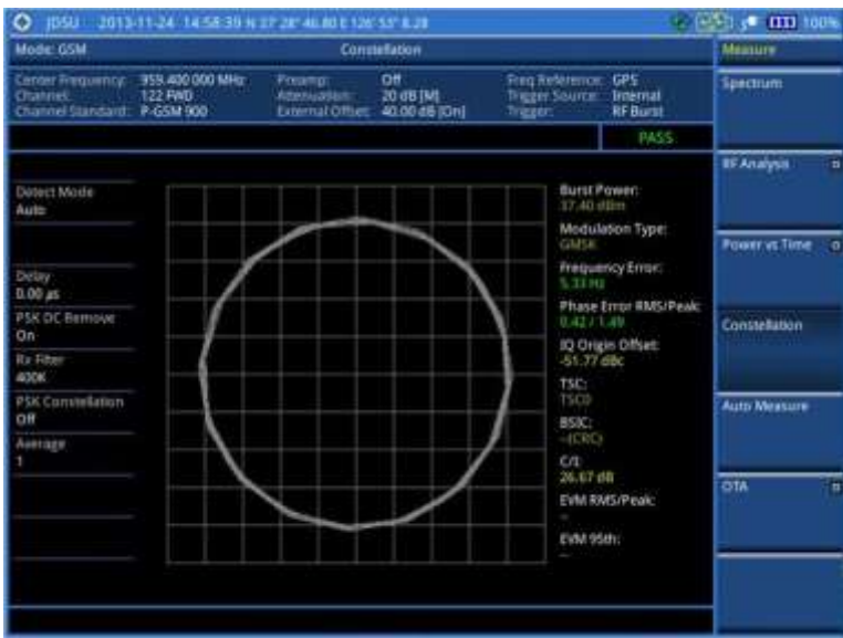
Figure 77 Constellation measurement (PSK on) with GSM signal analyzer
