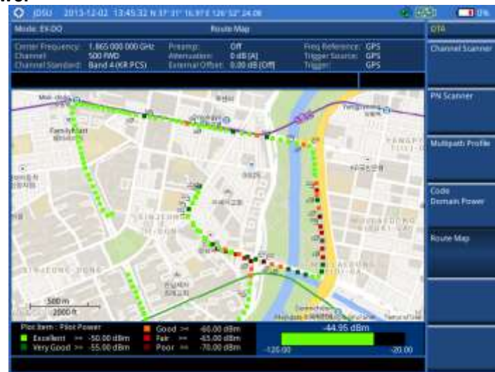
Figure 249 Route map measurement with EV-DO OTA signal analyzer
