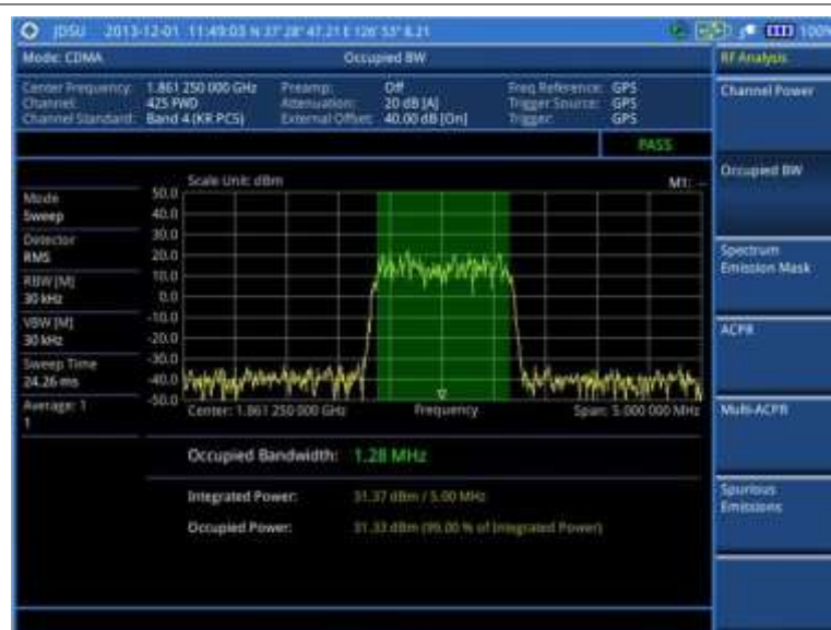
Figure 209 Occupied bandwidth measurement with CDMA signal analyzer
