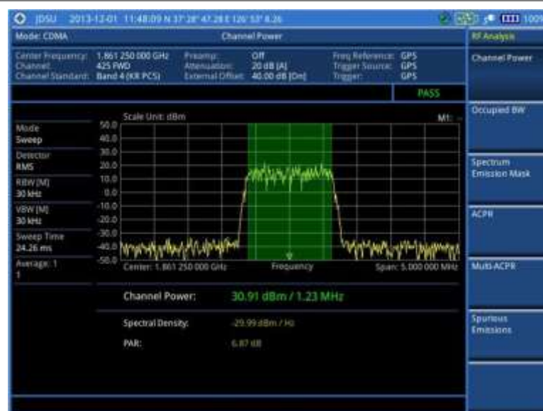
Figure 208 Channel power measurement with CDMA signal analyzer
