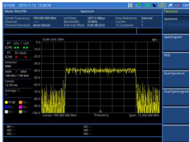
Figure 396 Example of spectrum measurement in BBU emulation
