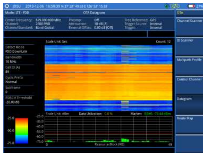
Figure 147 Datagram measurement with LTE-FDD signal analyzer
