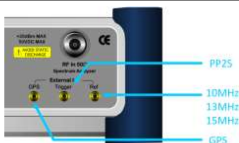
Figure 86 Connection ports for external reference clock
