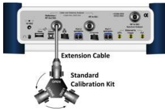
Figure 312 1-port calibration connection with mechanical Y-Cal kit
