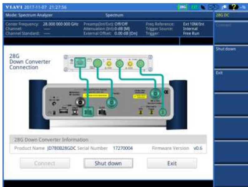
Figure 7 28 GHz Downconverter Connection Manager window
