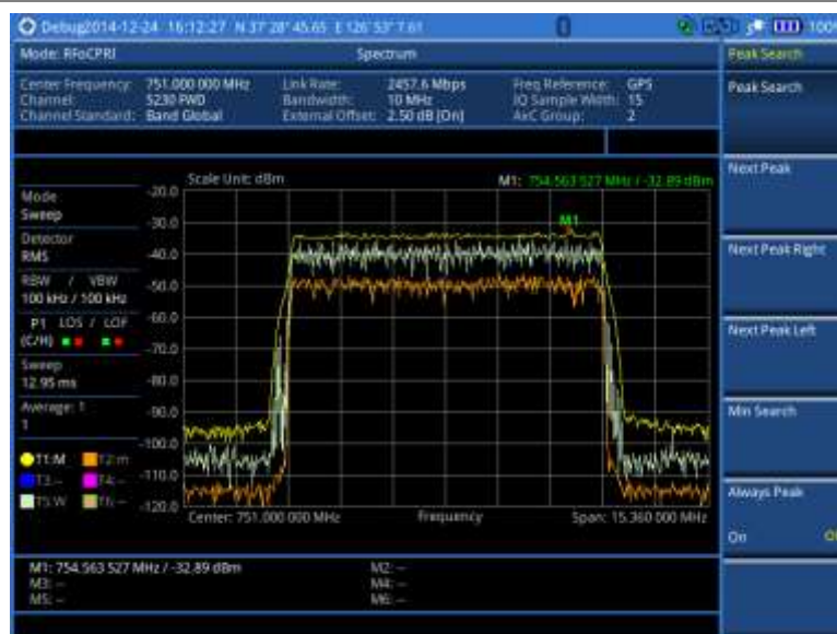
Figure 345 RFoCPRI spectrum analysis on LTE Uplink 10 MHz, antenna 2
