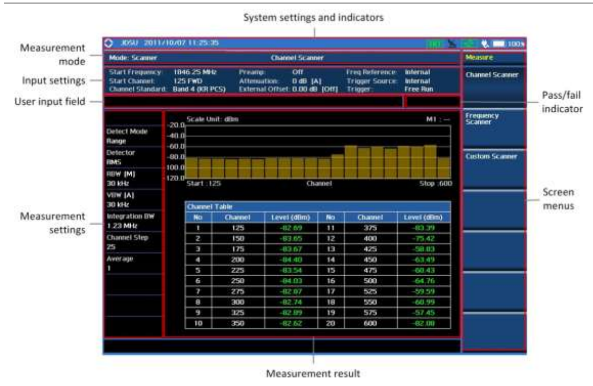
Figure 435 Channel scanner screen
