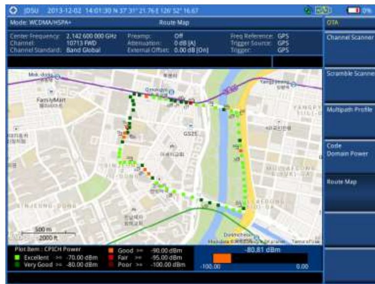
Figure 106 Route map measurement (CPICH Ec/Io) with WCDMA/HSPA+ OTA signal analyzer
