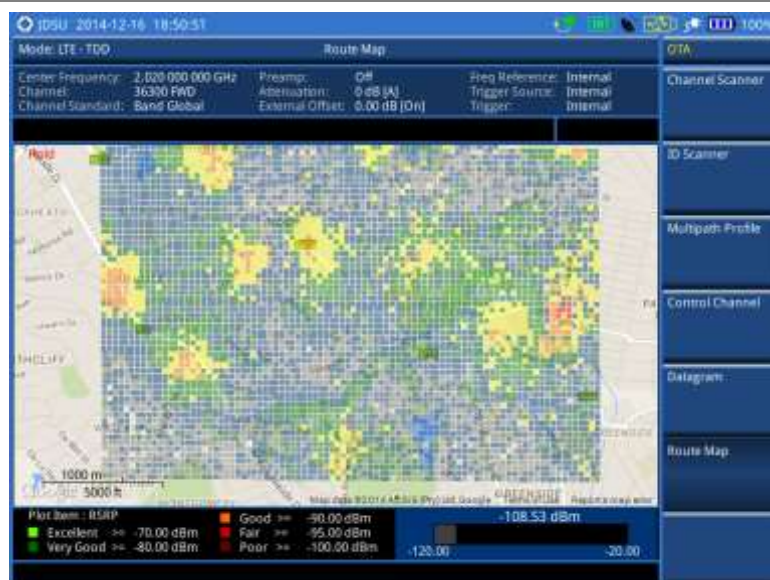
Figure 200 Raster image overlaid on the base map with LTE-TDD OTA signal analyzer
