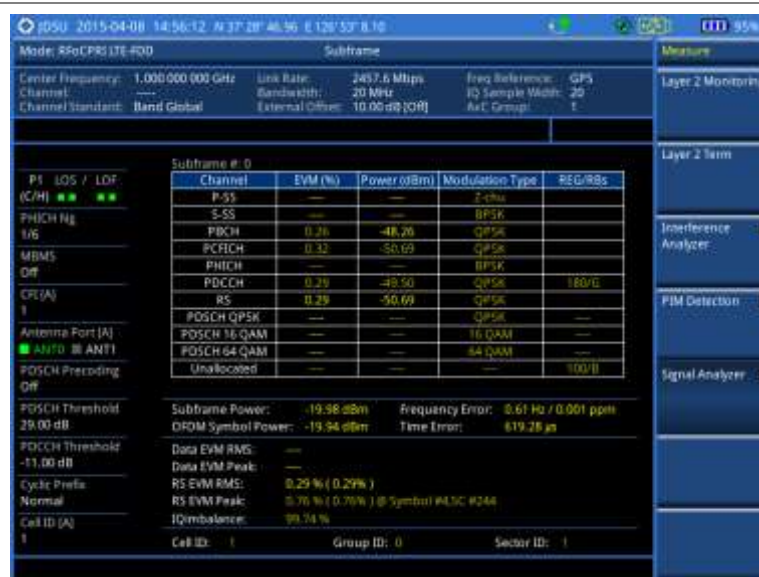
Figure 367 Subframe measurement (regular view) with RFoCPRI LTE-FDD signal analyzer
