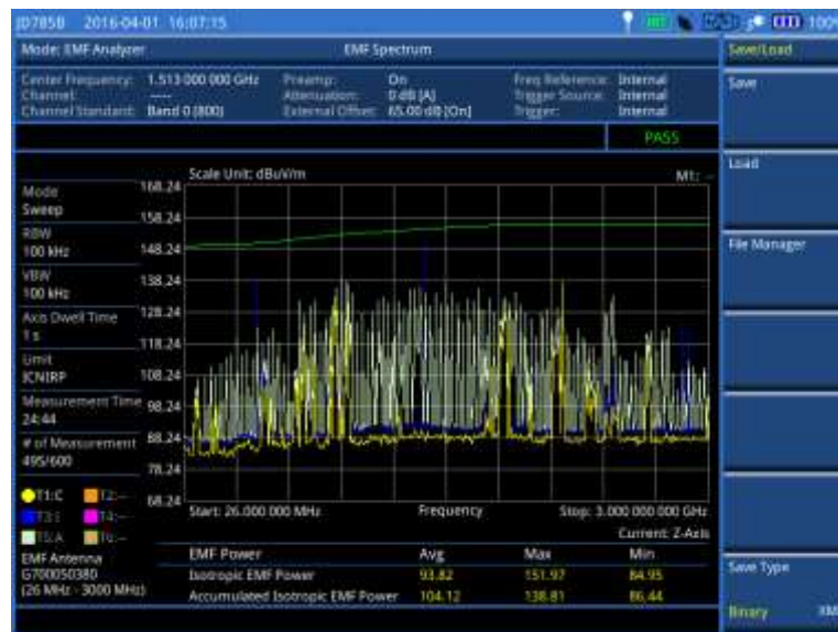
Figure 456 EMF spectrum measurement with EMF analyzer
