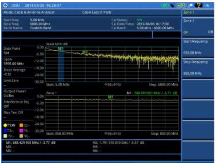
Figure 326 Cable loss (1 port) measurement with the zone enabled
