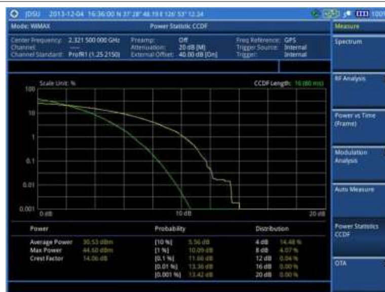
Figure 290 CCDF measurement with Mobile WiMAX signal analyzer
