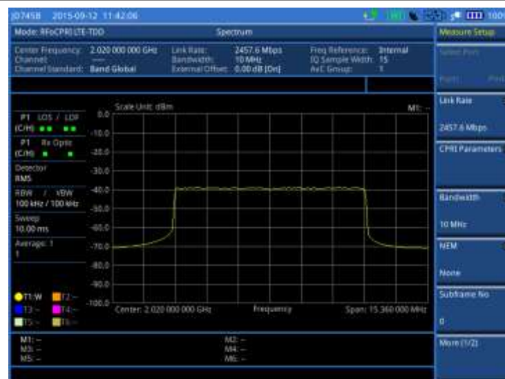
Figure 373 Spectrum measurement with RFoCPRI LTE-TDD signal analyzer
