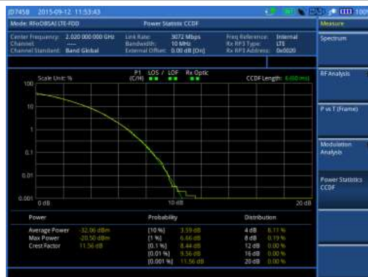
Figure 434 CCDF measurement with RFoBSAI LTE-FDD signal analyzer
