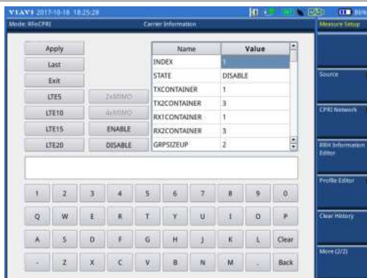
Figure 395 Example of RRH profile editor
