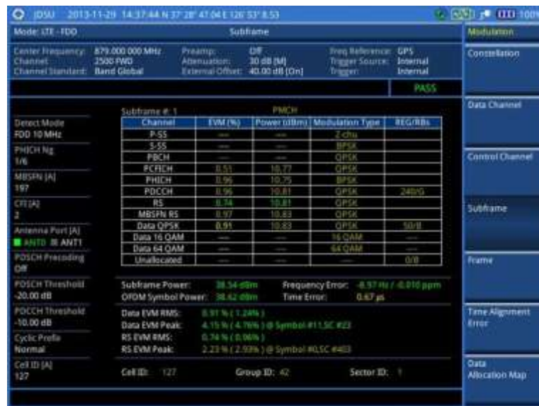
Figure 130 Subframe measurement with LTE-FDD signal analyzer (MBMS On)
