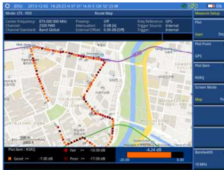
Figure 149 Route map measurement (RSRQ) with LTE-FDD OTA signal analyzer
