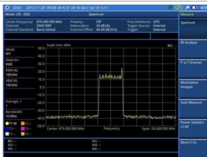
Figure 113 Spectrum measurement screen with LTE-FDD signal analyzer
