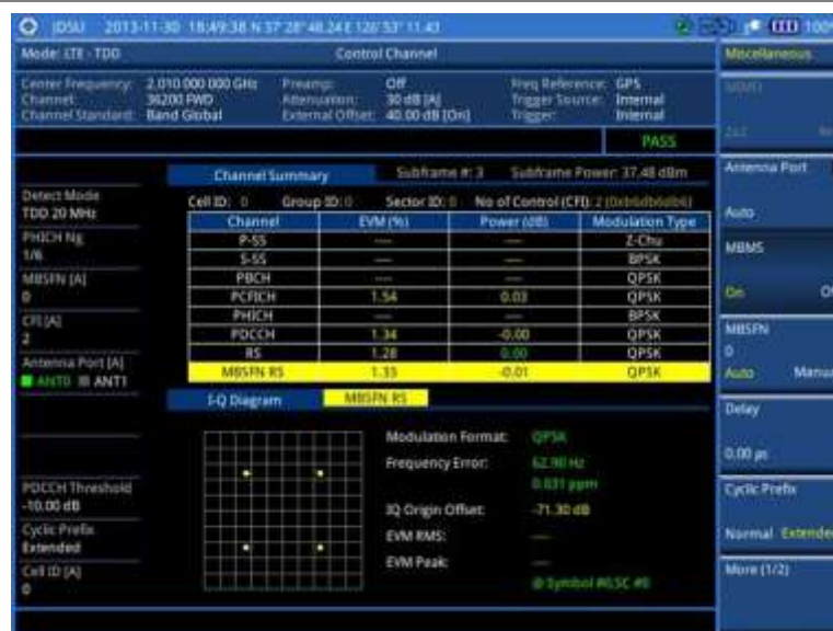
Figure 176 Control channel measurement with LTE-TDD signal analyzer (MBMS On)
