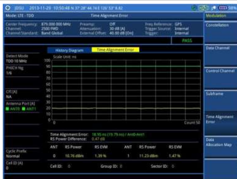
Figure 180 Time alignment error measurement with LTE-TDD signal analyzer
