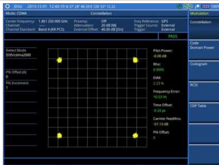
Figure 214 Constellation measurement with CDMA signal analyzer
