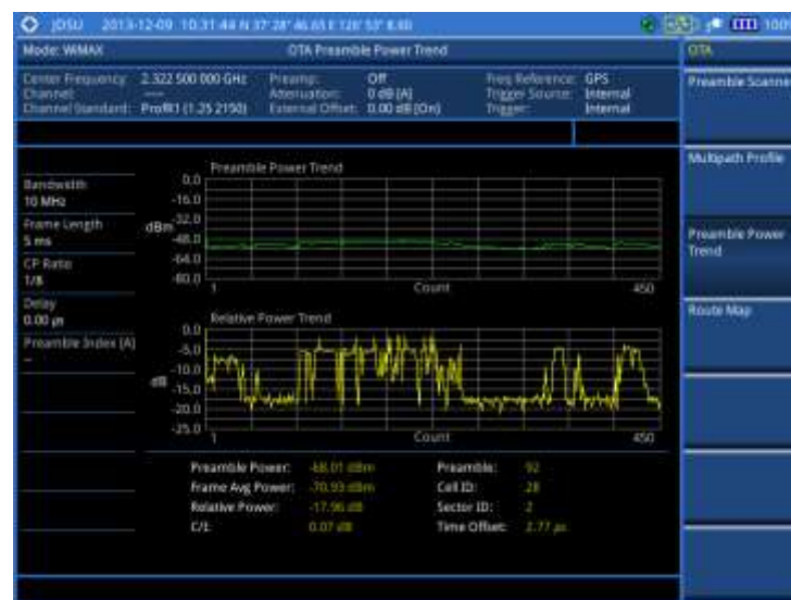
Figure 293 Preamble power trend with Mobile WiMAX OTA signal analyzer
