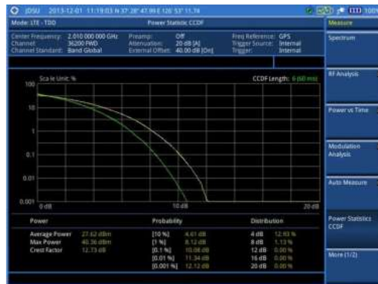
Figure 184 CCDF measurement with LTE-TDD signal analyzer
