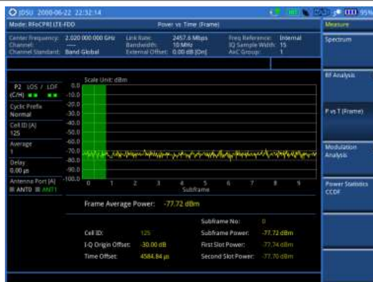
Figure 362 Power vs. time (frame) measurement with RFoCPRI LTE-FDD signal analyzer
