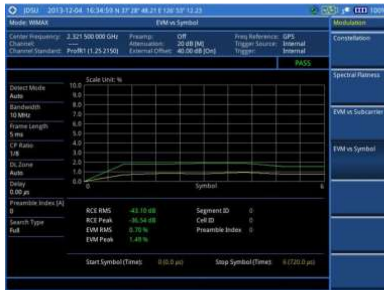
Figure 289 EVM vs. symbol measurement with Mobile WiMAX signal analyzer
