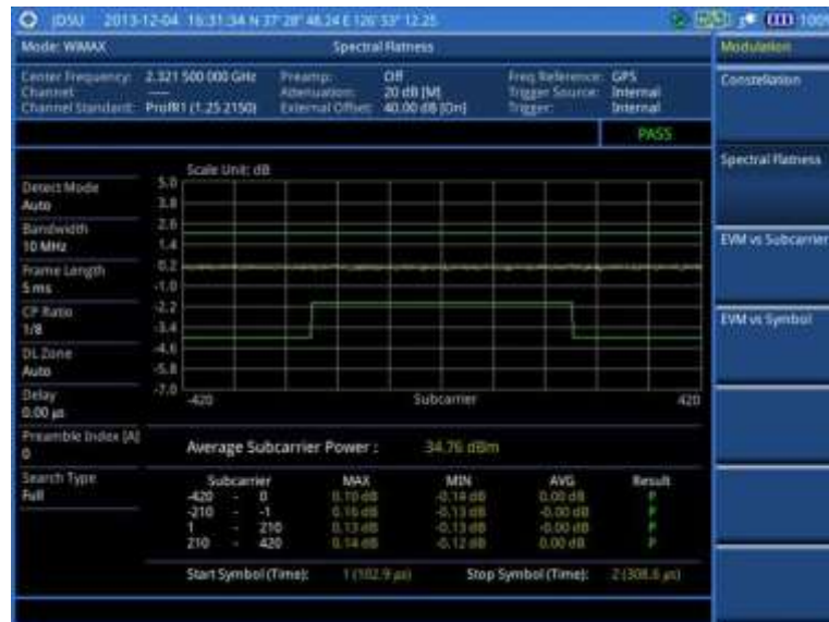
Figure 287 Spectral flatness measurement with Mobile WiMAX signal analyzer
