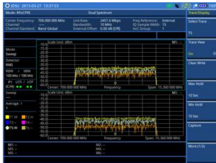
Figure 346 RFoCPRI dual spectrum analysis
