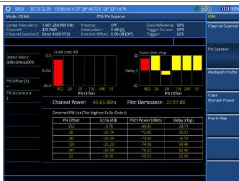
Figure 221 PN scanner measurement with CDMA OTA signal analyzer
