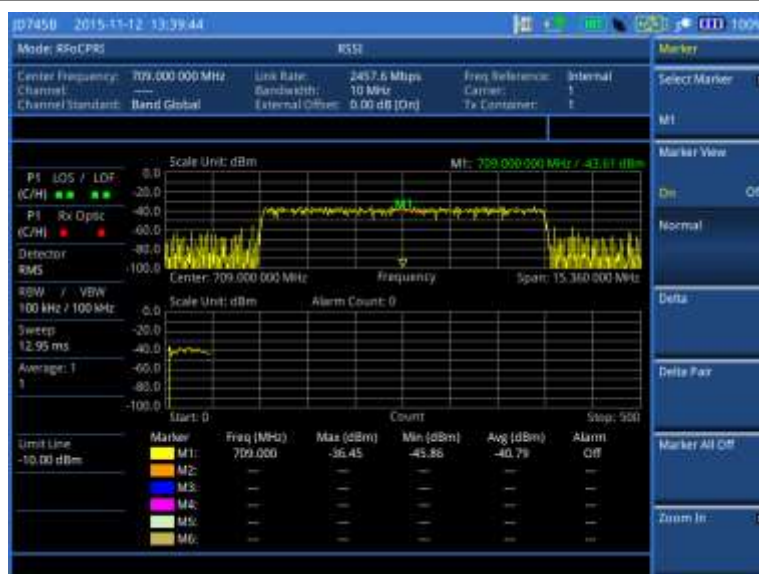
Figure 400 Example of RSSI in BBU emulation
