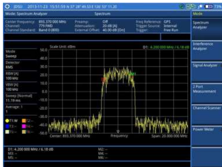
Figure 16 Spectrum measurement with spectrum analyzer
