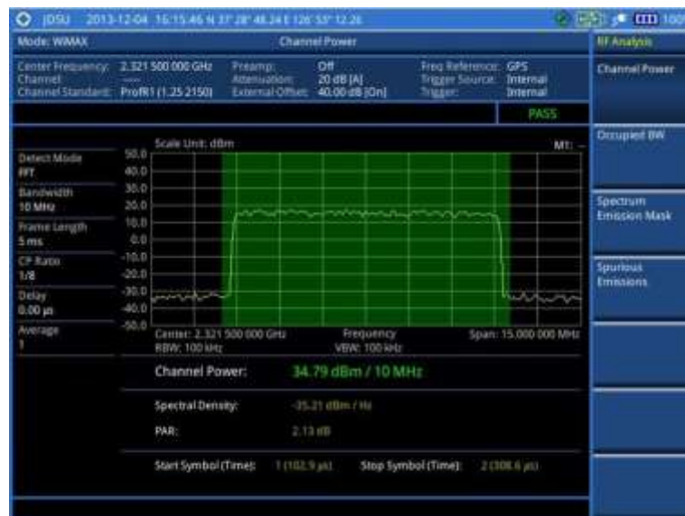
Figure 281 Channel power measurement with Mobile WiMAX signal analyzer
