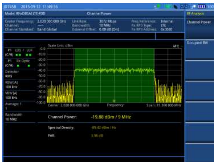
Figure 424 Channel power measurement with RFoBSAI LTE-FDD signal analyzer
