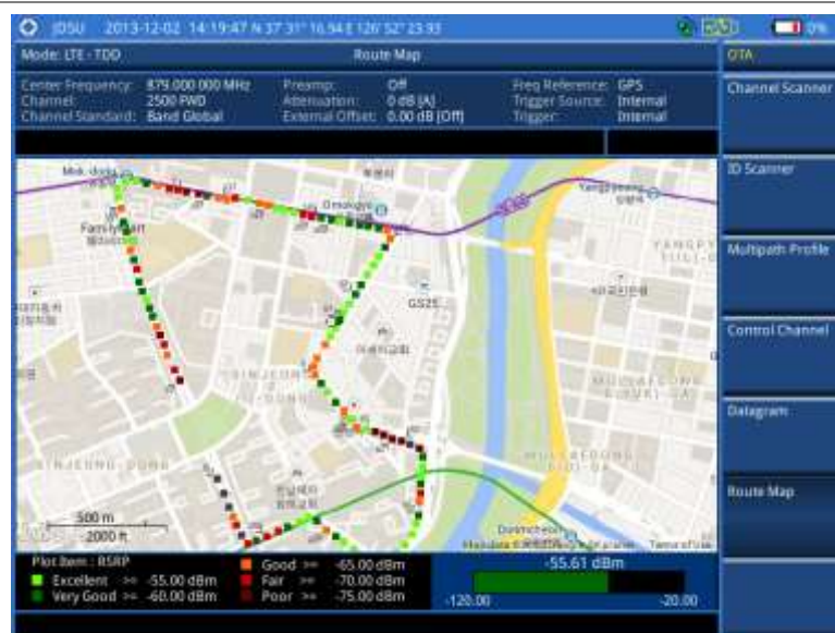
Figure 193 Route map measurement (RSRP) with LTE-TDD OTA signal analyzer
