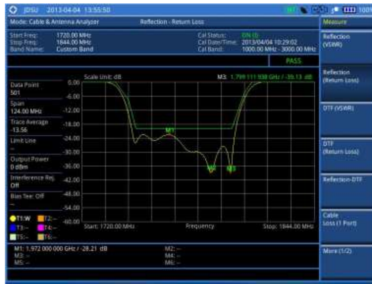
Figure 321 Reflection measurement in return loss scale
