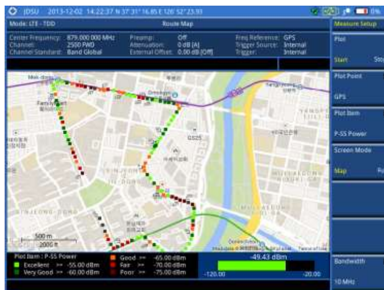
Figure 197 Route map measurement (P-SS Power) with LTE-TDD OTA signal analyzer
