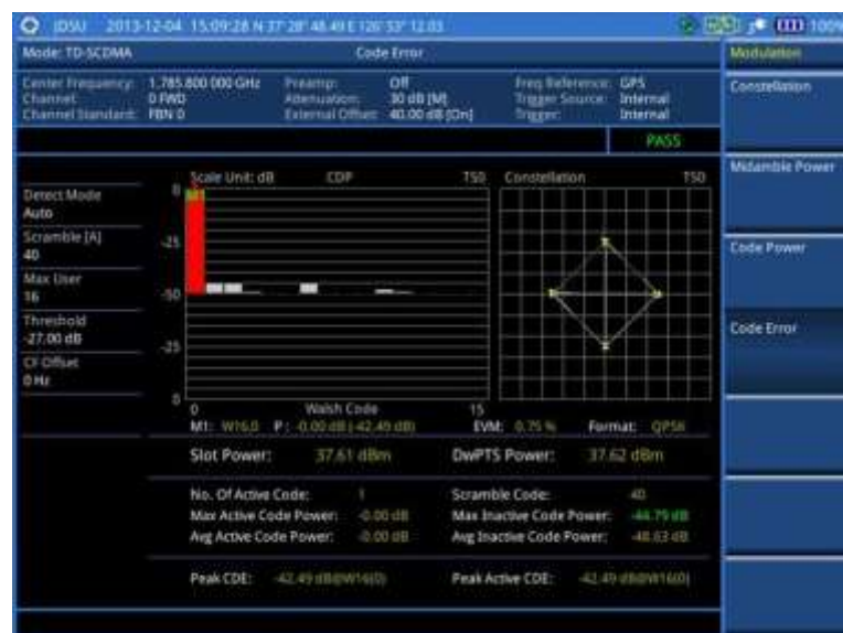
Figure 269 Code error measurement with TD-SCDMA signal analyzer
