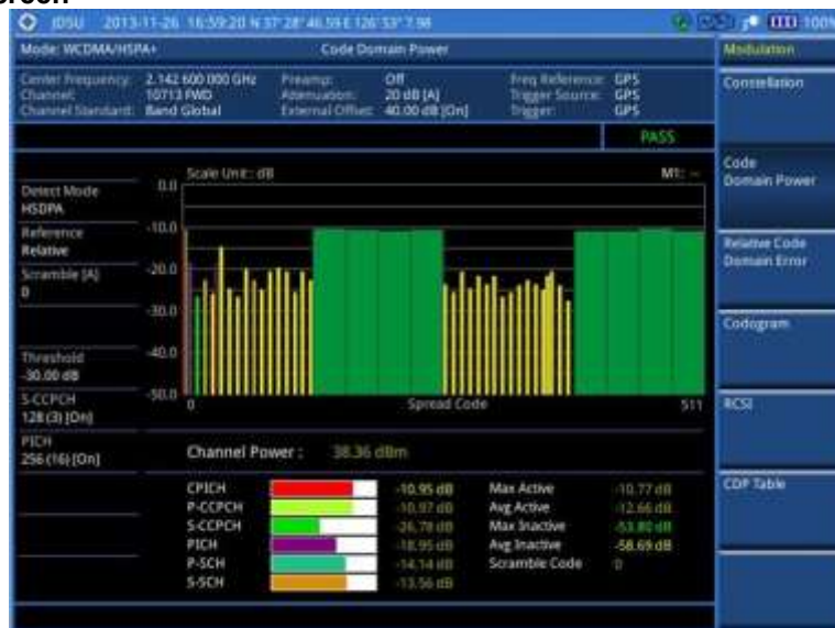
Figure 95 Code domain power measurement with WCDMA/HSPA+ signal analyzer
