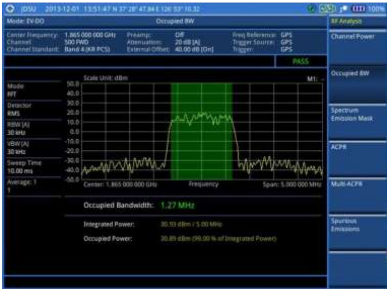
Figure 232 Occupied bandwidth measurement with EV-DO signal analyzer
