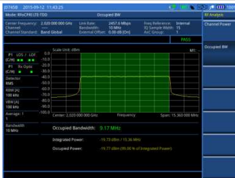
Figure 375 Occupied bandwidth measurement with RFoCPRI LTE-TDD signal analyzer
