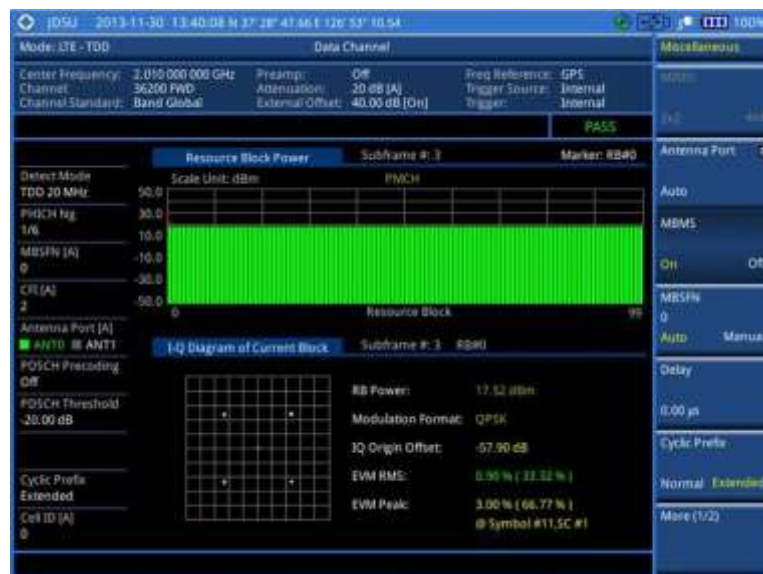
Figure 174 Data channel measurement with LTE-TDD signal analyzer (MBMS On)
