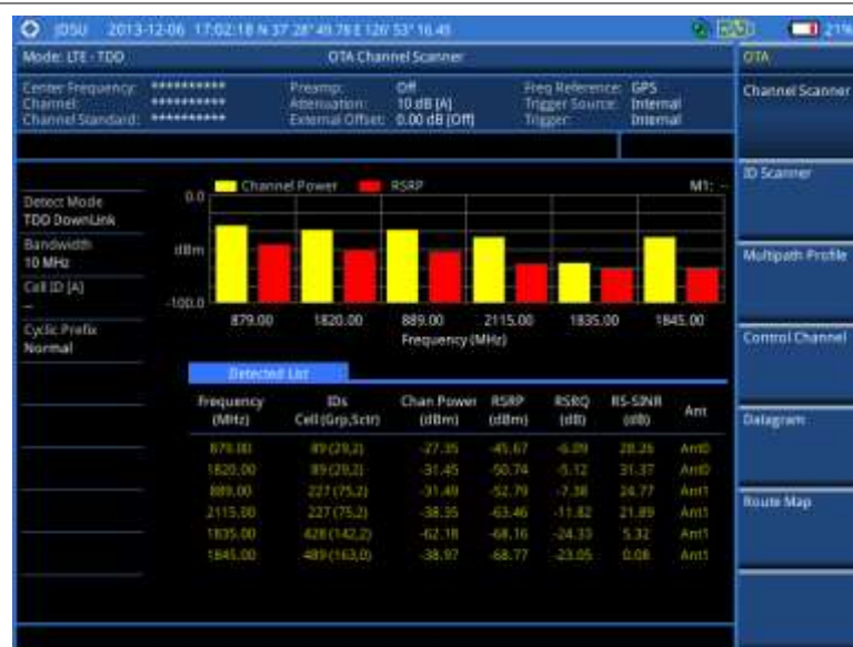
Figure 188 Channel scanner measurement with LTE-TDD OTA signal analyzer
