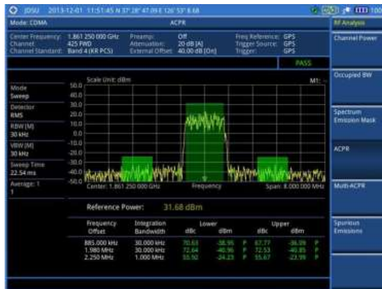
Figure 211 ACPR measurement with CDMA signal analyzer
