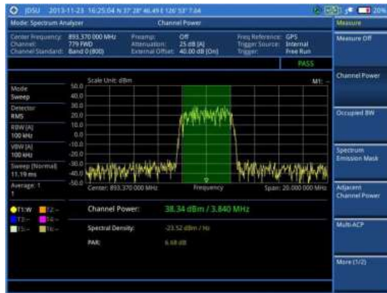
Figure 21 Channel power measurement with spectrum analyzer
