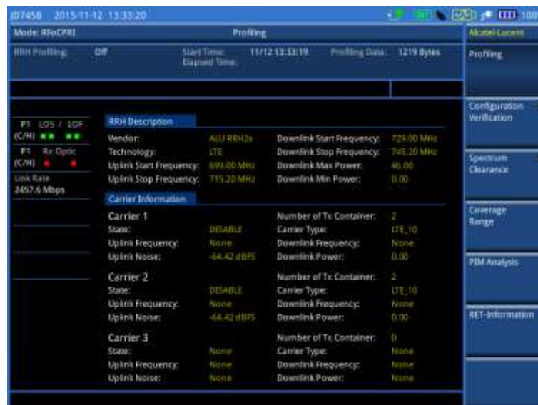
Figure 386 Example of RRH profiling results with carrier information
