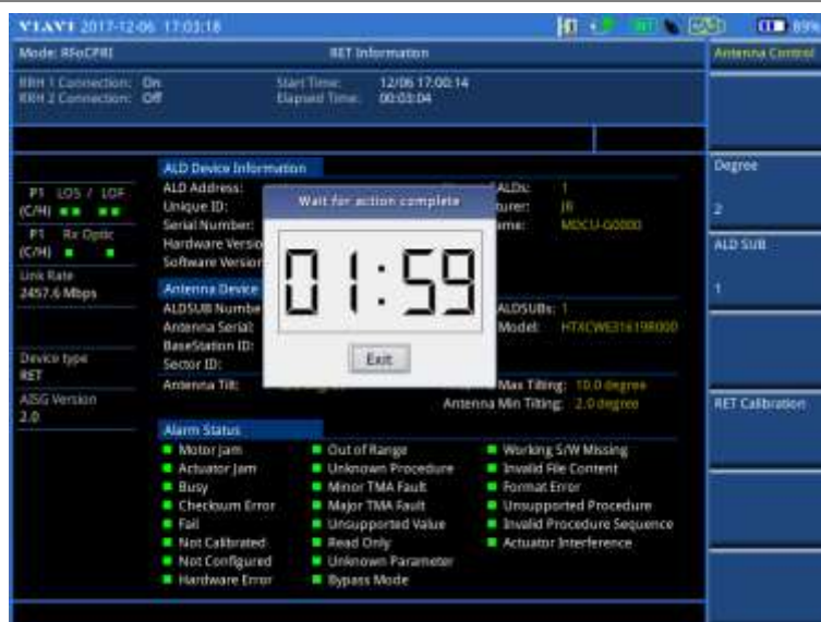
Figure 408 Example of antenna tilting in RET information
