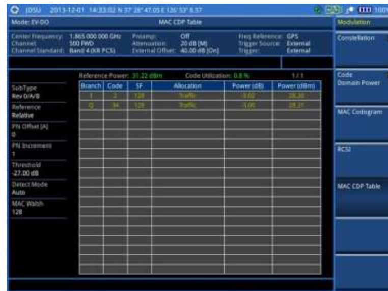
Figure 243 MAC CDP Table measurement with EV-DO signal analyzer
