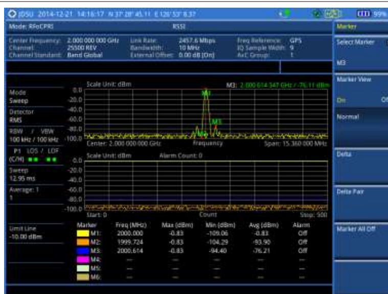
Figure 353 RFoCPRI interference measurement in RSSI
