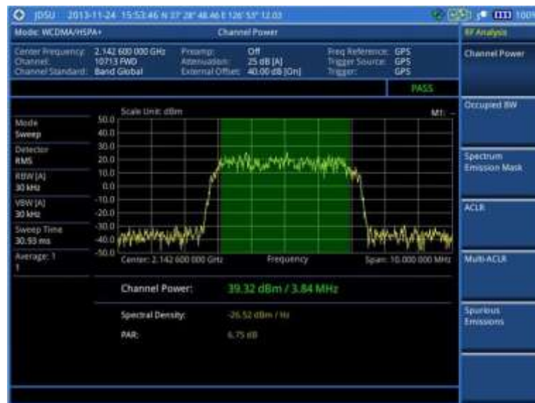
Figure 88 Channel power measurement with WCDMA/HSPA+ signal analyzer
