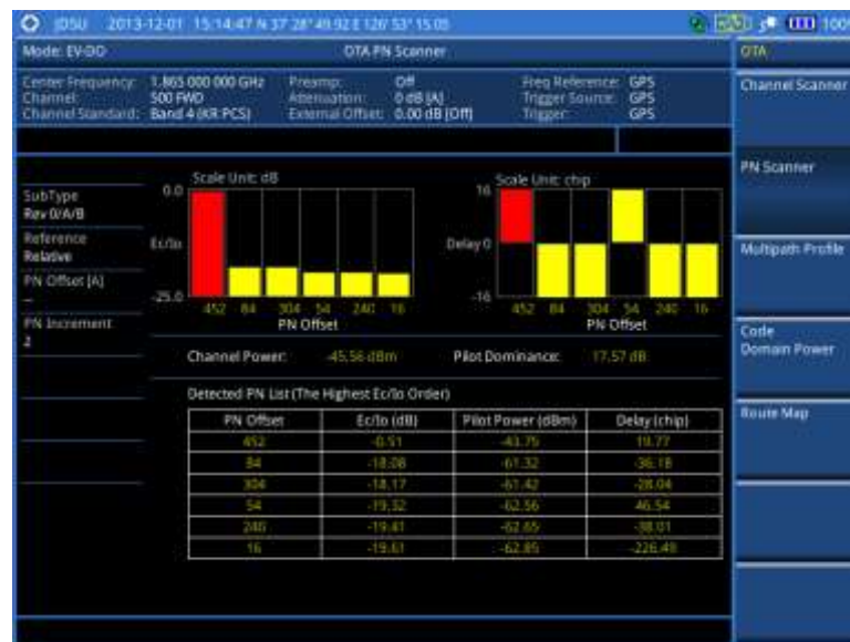
Figure 246 PN scanner measurement with EV-DO OTA signal analyzer
