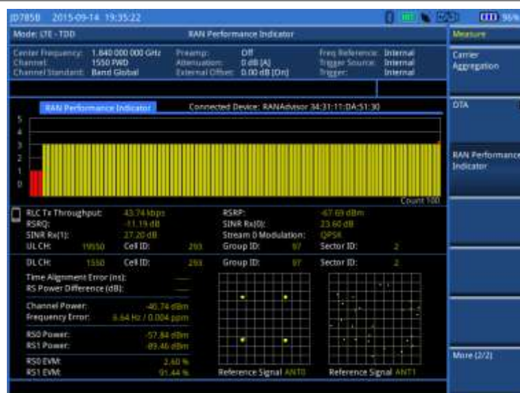
Figure 201 RAN performance indicator with LTE-TDD signal analyzer
