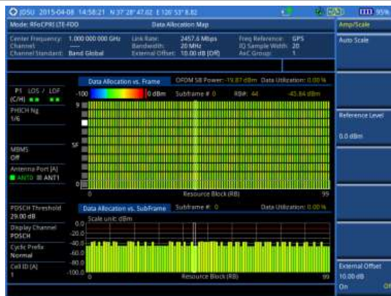
Figure 370 Data allocation map measurement with RFoCPRI LTE-FDD signal analyzer
