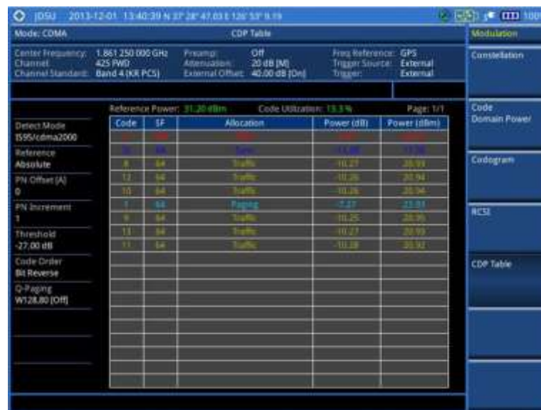
Figure 218 CDP Table measurement with CDMA signal analyzer
