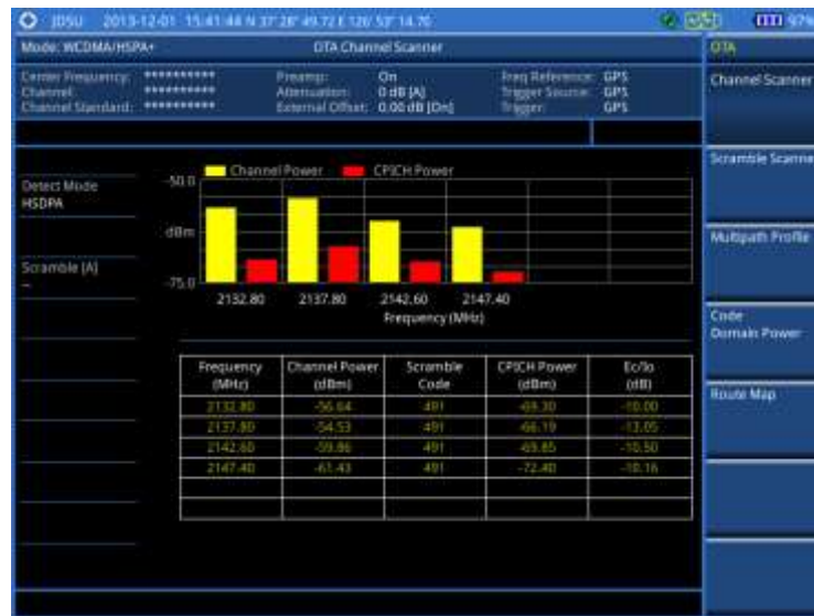
Figure 101 Channel scanner measurement with WCDMA/HSPA+ OTA signal analyzer
