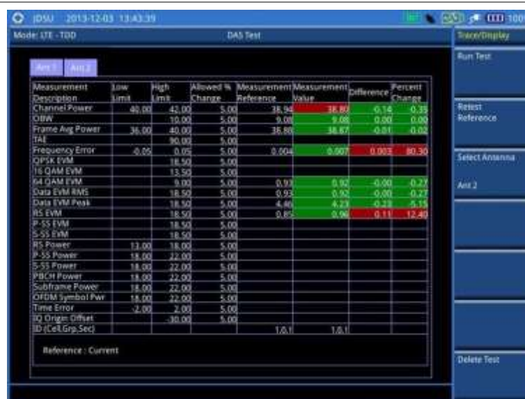
Figure 183 DAS measurement with LTE-TDD signal analyzer
