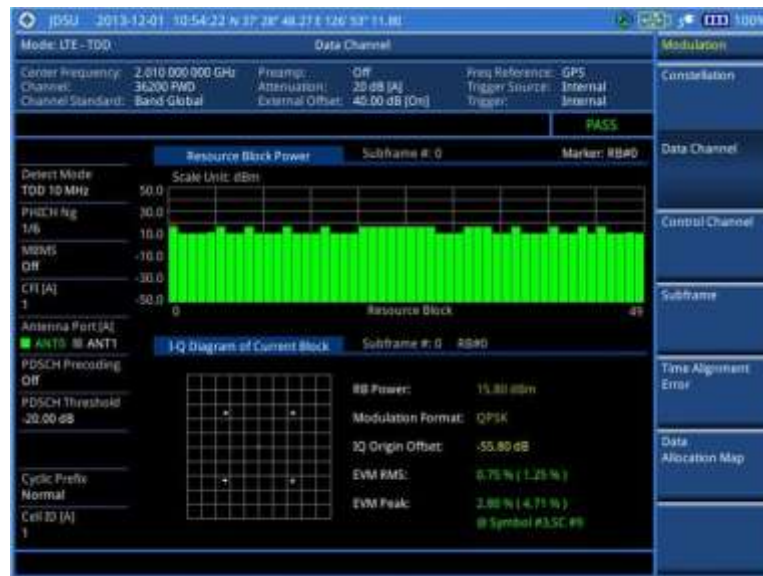
Figure 174 Data channel measurement with LTE-TDD signal analyzer (MBMS On)
