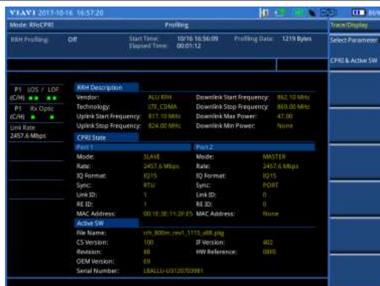
Figure 387 Example of RRH profiling results with CPRI state and activated SW
