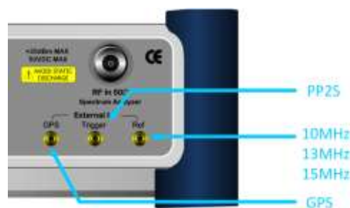
Figure 229 Connection ports for external reference clock
