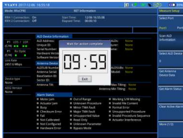
Figure 405 Example of ALD scanning in RET information
