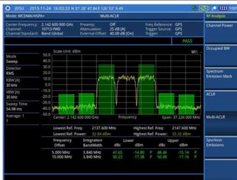
Figure 92 Multi-ACLR measurement with WCDMA/HSPA+ signal analyzer
