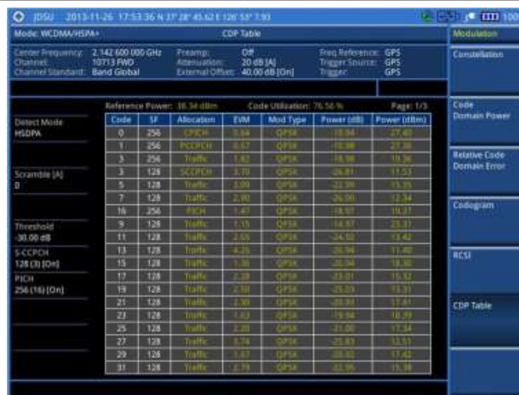
Figure 99 CDP Table measurement with WCDMA/HSPA+ signal analyzer
