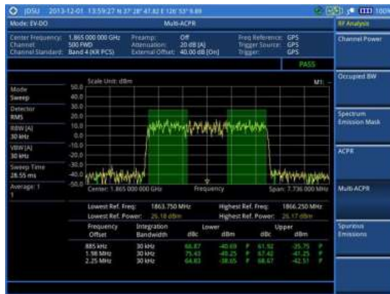
Figure 235 Multi-ACPR measurement with EV-DO signal analyzer
