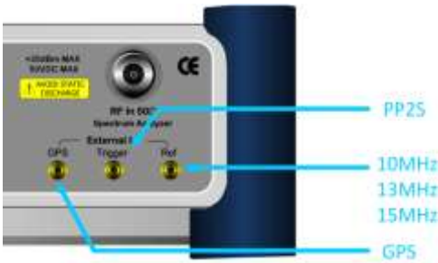
Figure 206 Connection ports for external reference clock
