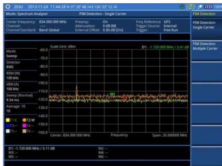
Figure 41 PIM detection for single carrier
