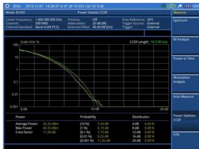
Figure 244 CCDF measurement with EV-DO signal analyzer
