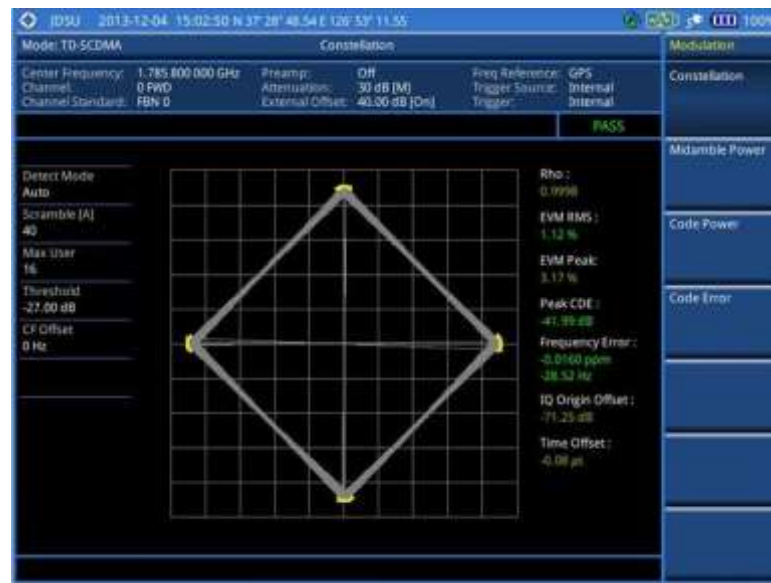
Figure 266 Constellation measurement with TD-SCDMA signal analyzer
