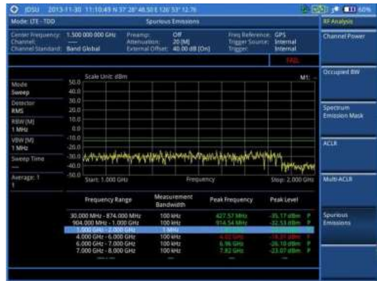
Figure 168 Spurious emissions measurement with LTE-TDD signal analyzer
