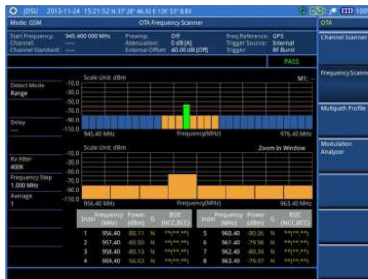
Figure 79 Frequency scanner measurement with GSM OTA signal analyzer
