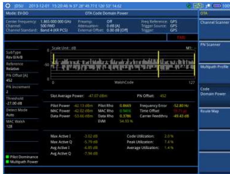
Figure 248 Code domain power measurement with EV-DO OTA signal analyzer
