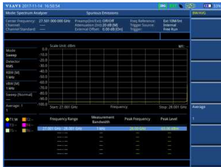
Figure 33 Spurious emissions measurement with spectrum analyzer (on 28 GHz downconverter)
