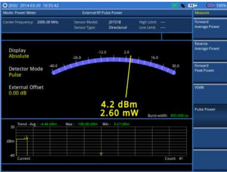
Figure 452 External power measurement of pulse power
