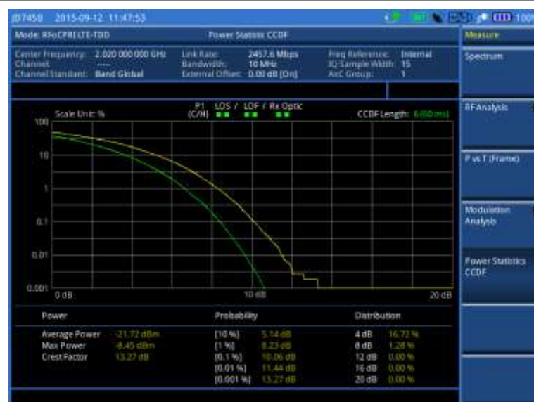
Figure 385 CCDF measurement with RFoCPRI LTE-TDD signal analyzer
