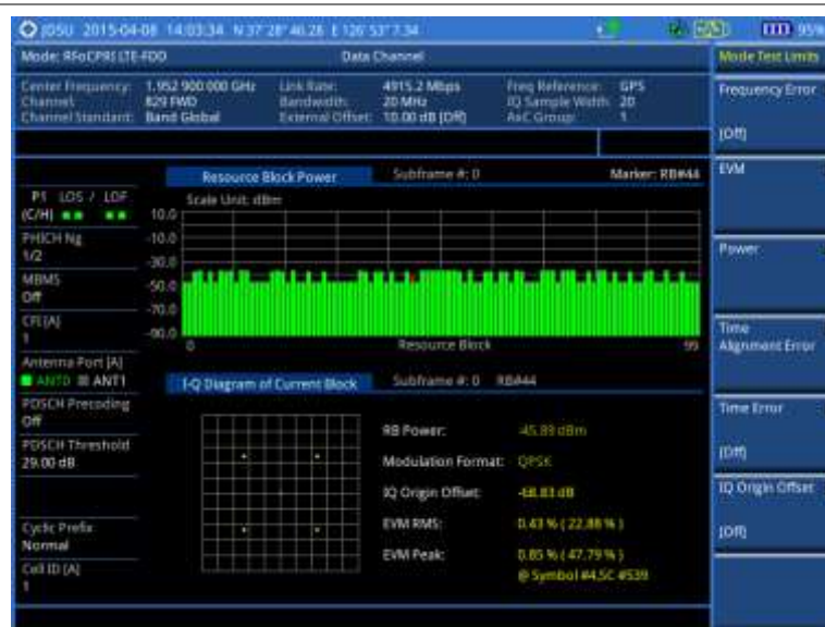
Figure 366 Data channel measurement with RFoCPRI LTE-FDD signal analyzer
