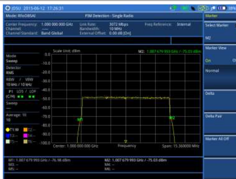
Figure 397 PIM detection of single radio
