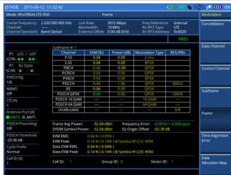
Figure 408 Frame measurement with RFoBSAI LTE-FDD signal analyzer
