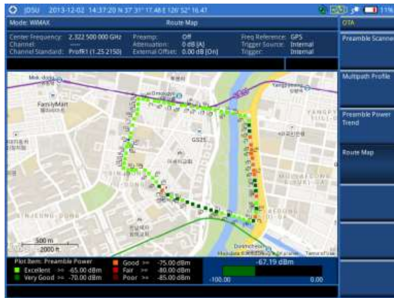
Figure 294 Route map measurement with Mobile WiMAX OTA signal analyzer
