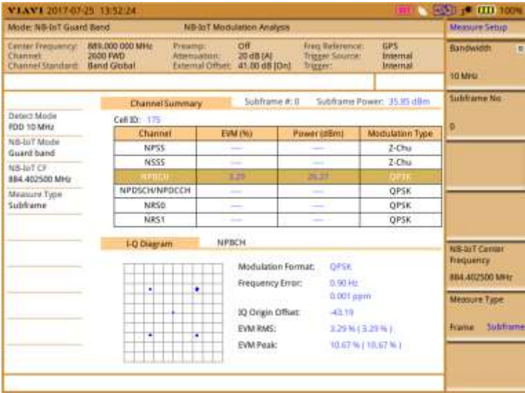
Figure 303 NB-IoT Guard Band Modualtion Analysis measurement screen (Subframe 0- NPBCH)
