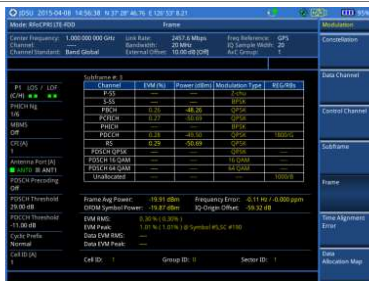
Figure 370 Frame measurement with RFoCPRI LTE-FDD signal analyzer
