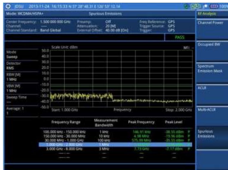
Figure 93 Spurious emissions measurement with WCDMA/HSPA+ signal analyzer
