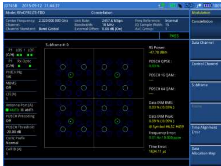
Figure 379 Constellation measurement with RFoCPRI LTE-TDD signal analyzer
