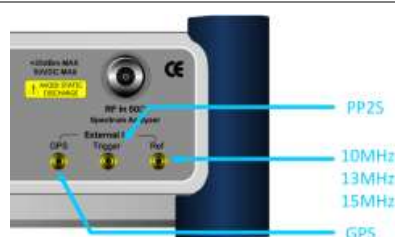
Figure 161 Connection ports for external reference clock
