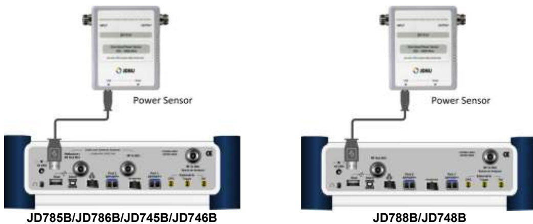
Figure 451 Directional power sensor connection
