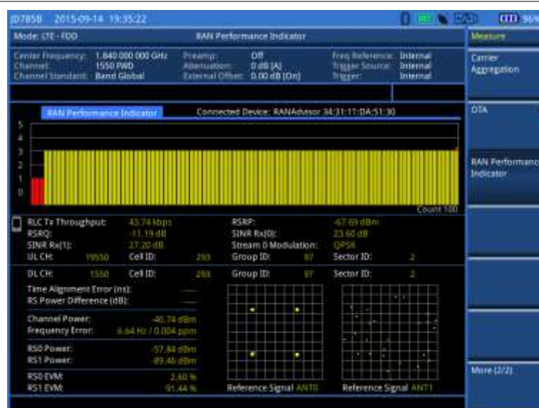
Figure 156 RAN performance indicator with LTE-FDD signal analyzer
