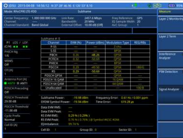
Figure 369 Subframe measurement (regular view) with RFoCPRI LTE-FDD signal analyzer
