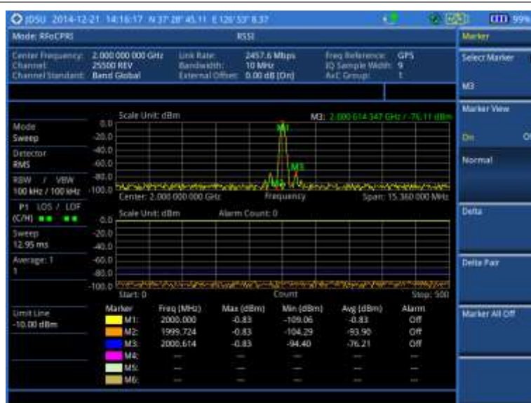
Figure 355 RFoCPRI interference measurement in RSSI
