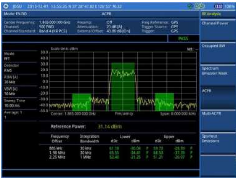
Figure 234 ACPR measurement with EV-DO signal analyzer
