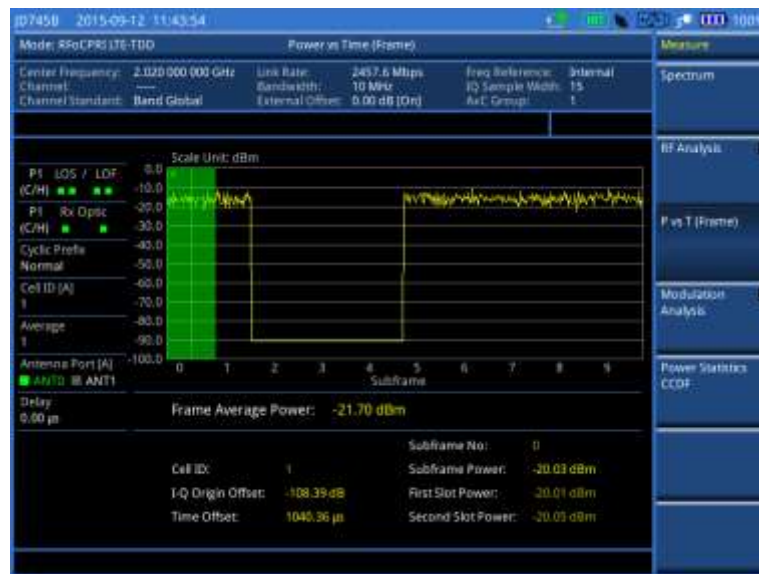
Figure 378 Power vs. time (frame) measurement with RFoCPRI LTE-TDD signal analyzer
