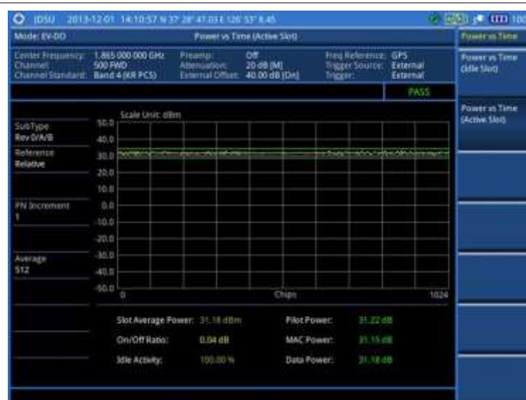
Figure 238 Power vs. time (active slot) measurement with EV-DO signal analyzer
