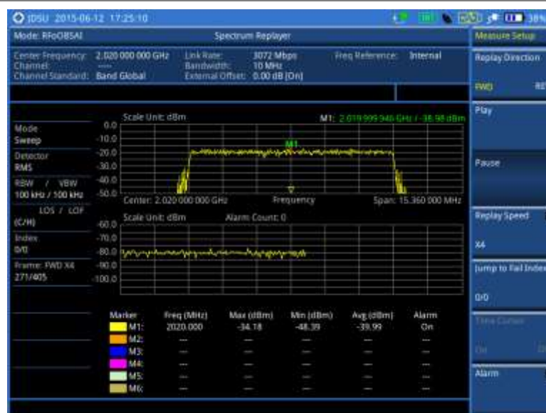
Figure 395 RFoBSAI spectrum replay
