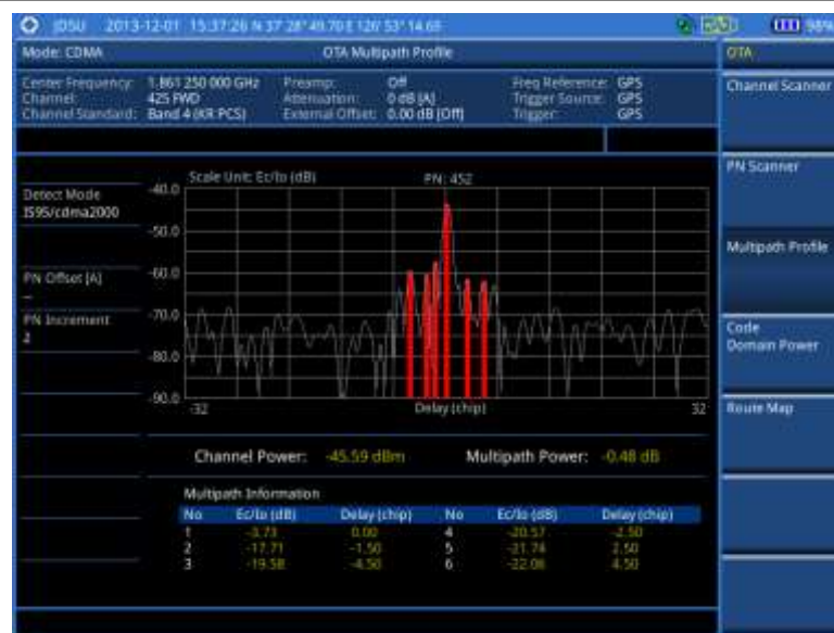
Figure 222 Multipath profile measurement with CDMA OTA signal analyzer
