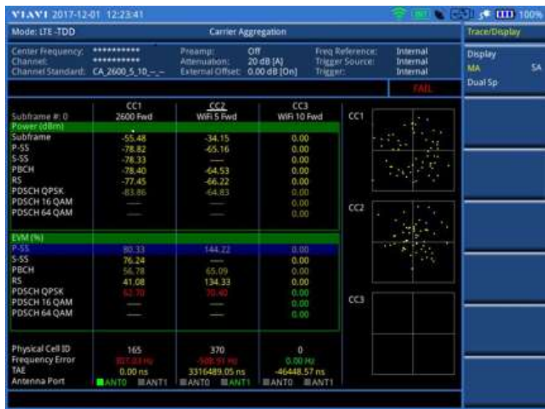
Figure 186 Carrier aggregation measurement with LTE-TDD signal analyzer (SA with Wi-Fi on)
