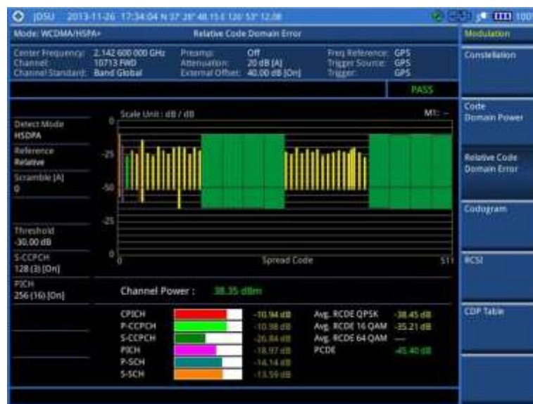
Figure 96 Relative code domain error with WCDMA/HSPA+ signal analyzer
