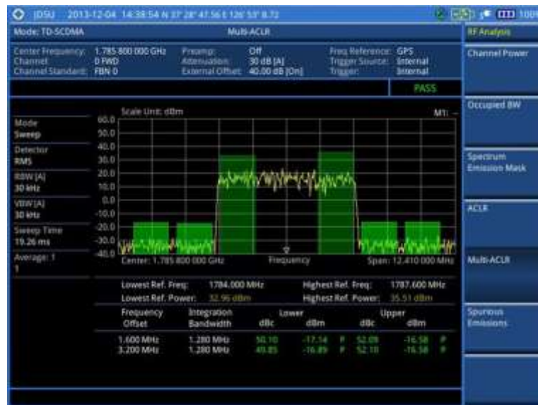
Figure 260 Multi-ACLR measurement with TD-SCDMA signal analyzer
