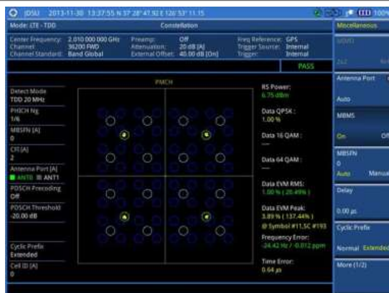
Figure 172 Constellation measurement with LTE-TDD signal analyzer (MBMS On)
