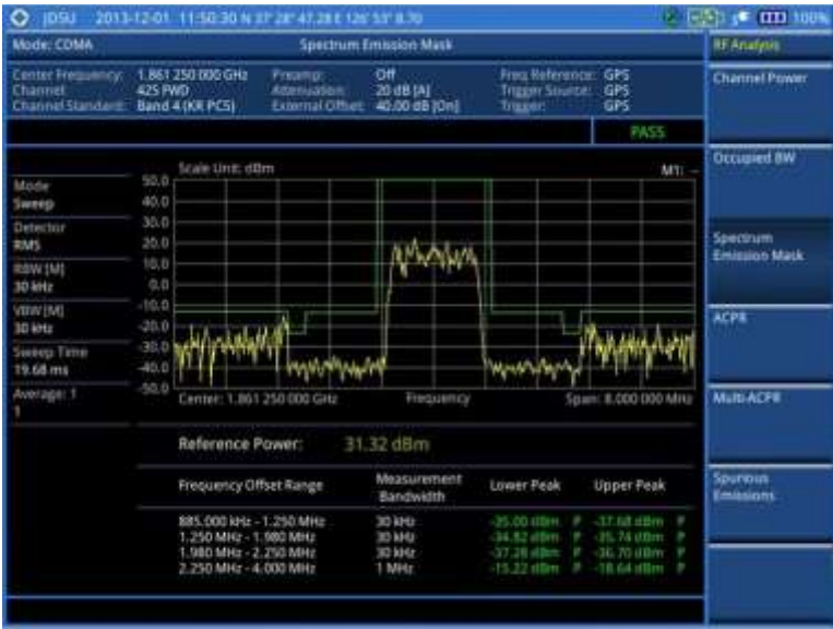
Figure 210 SEM measurement with CDMA signal analyzer
