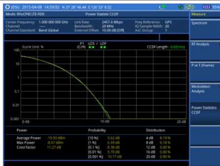
Figure 373 CCDF measurement with RFoCPRI LTE-FDD signal analyzer
