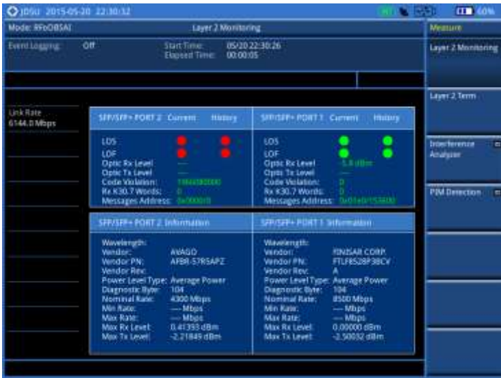
Figure 388 OBSAI RP3 layer 2 monitoring
