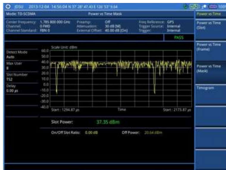
Figure 264 Power vs. time (mask) measurement with TD-SCDMA signal analyzer
