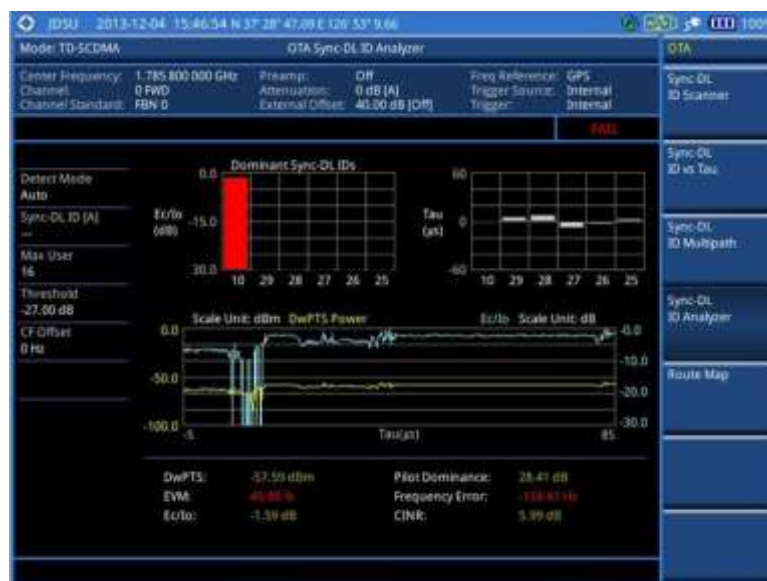
Figure 273 Sync-DL ID analyzer measurement with TD-SCDMA OTA signal analyzer
