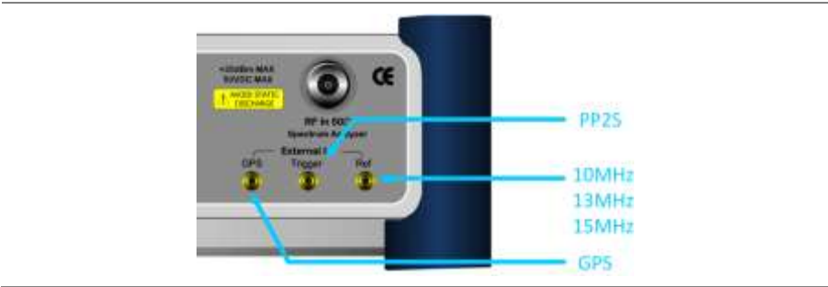
Figure 254 Connection ports for external reference clock
