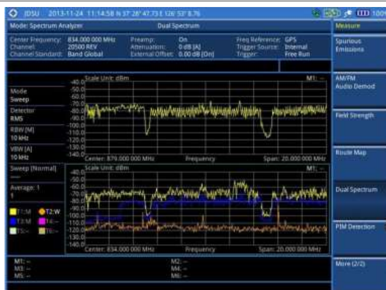
Figure 40 Dual spectrum measurement with spectrum analyzer
