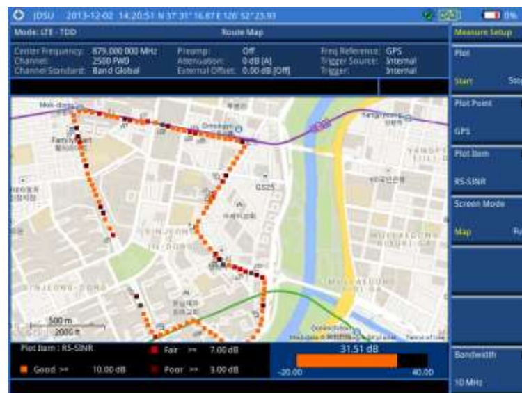
Figure 195 Route map measurement (RS-SINR) with LTE-TDD OTA signal analyzer
