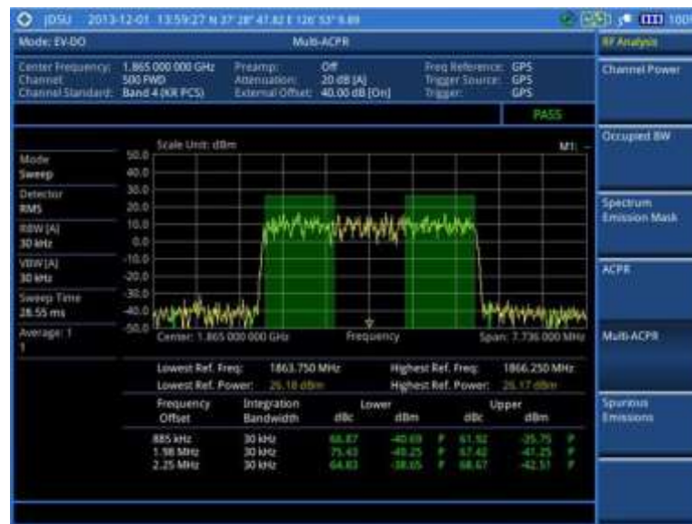
Figure 235 Multi-ACPR measurement with EV-DO signal analyzer
