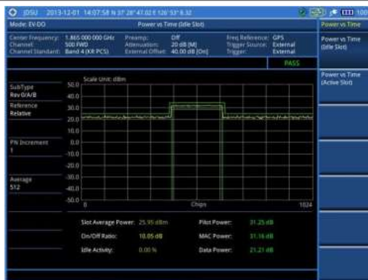
Figure 237 Power vs. time (idle slot) measurement with EV-DO signal analyzer
