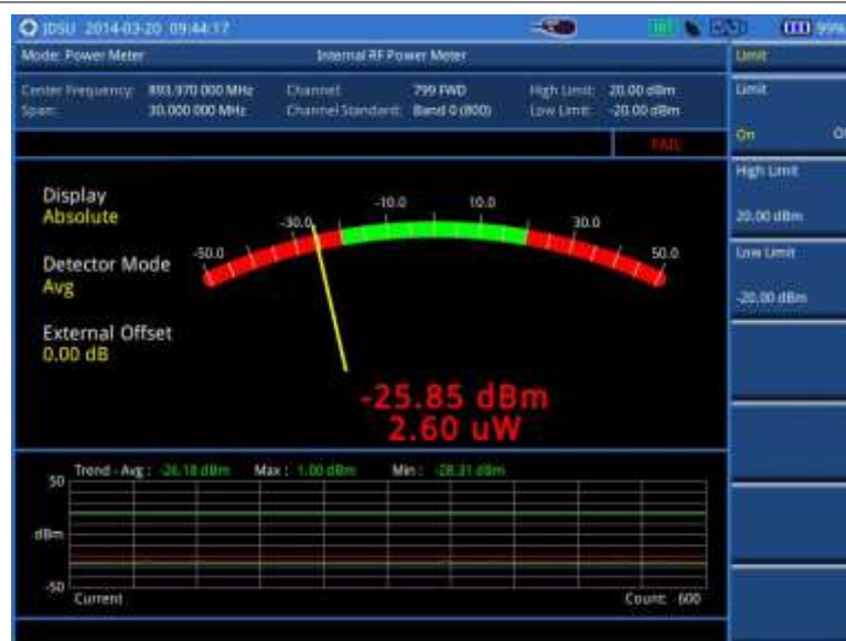
Figure 449 Internal power measurement
