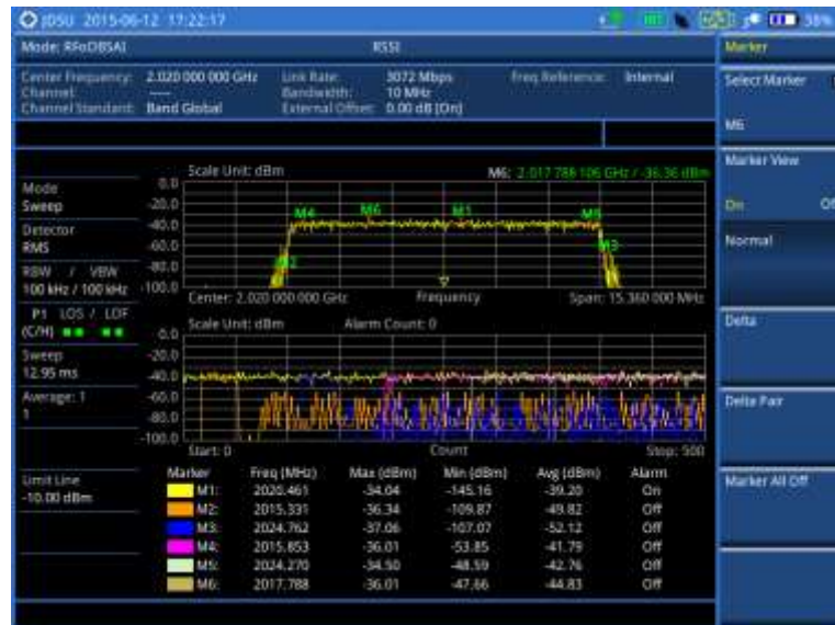
Figure 394 RFoBSAI interference measurement in RSSI
