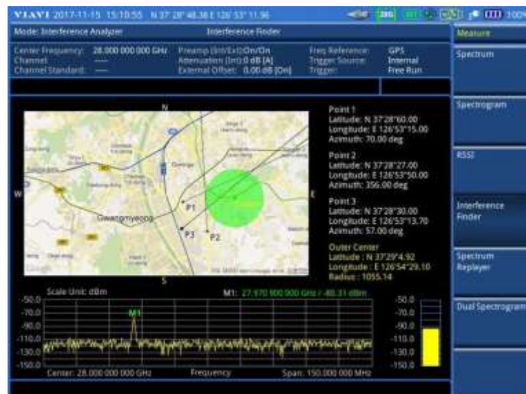
Figure 56 Interference finder measurement in map view (on 28 GHz downconverter)
