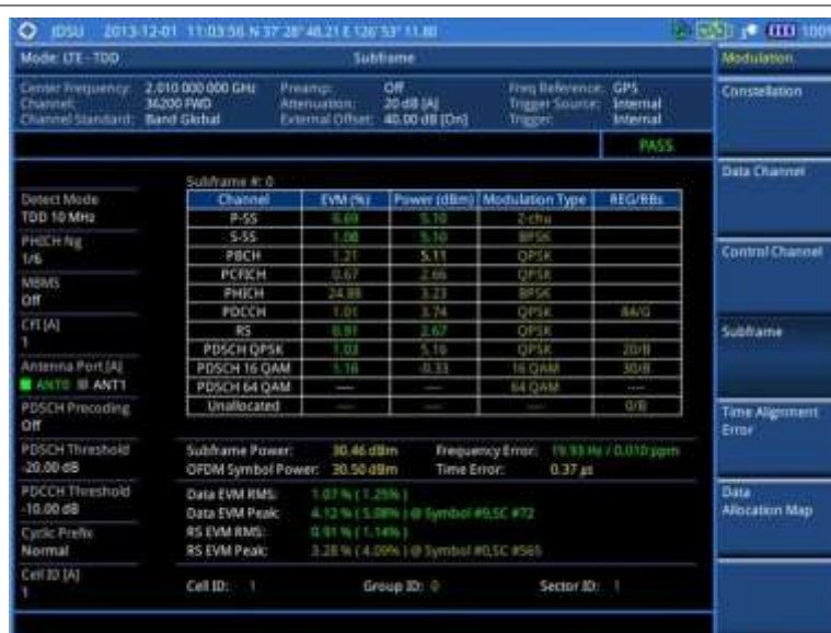
Figure 177 Subframe measurement with LTE-TDD signal analyzer
