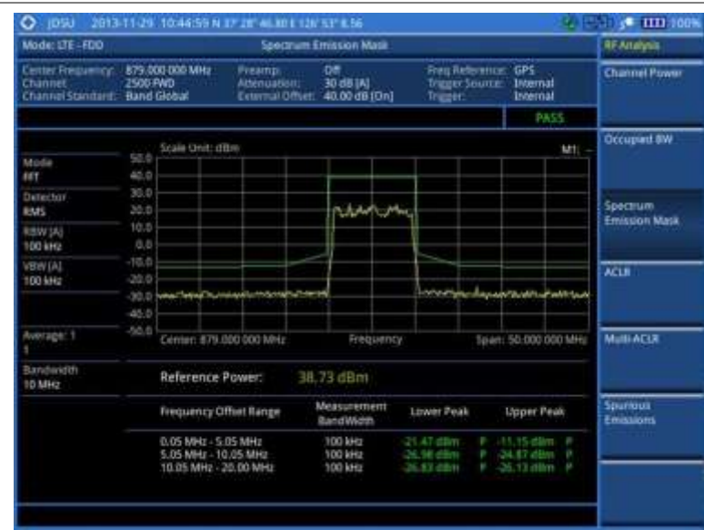
Figure 116 SEM measurement with LTE-FDD signal analyzer
