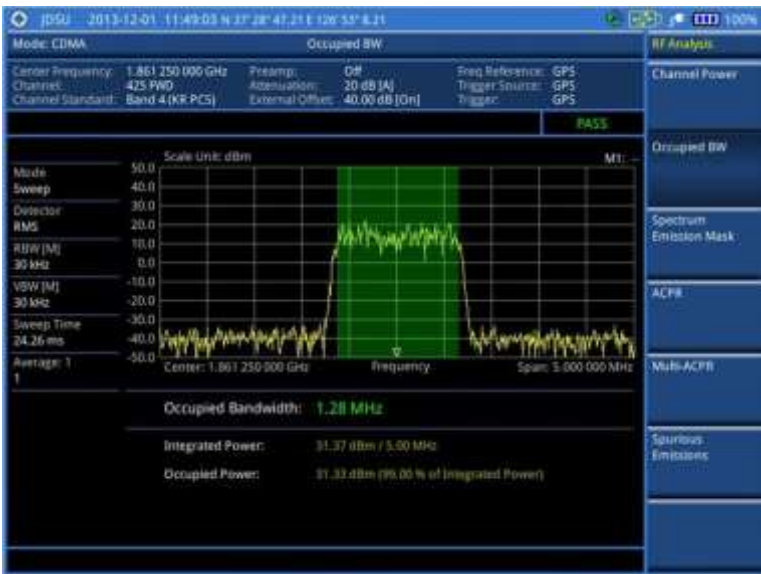
Figure 209 Occupied bandwidth measurement with CDMA signal analyzer
