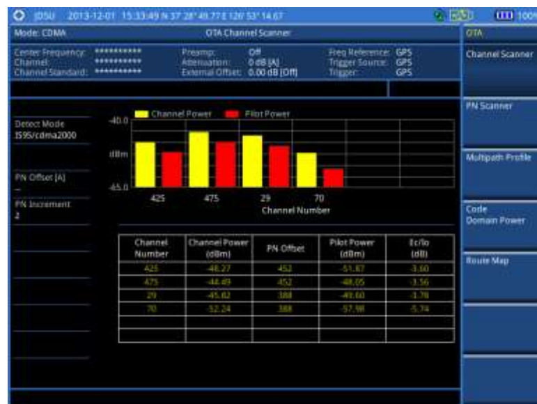
Figure 220 Channel scanner measurement with CDMA OTA signal analyzer
