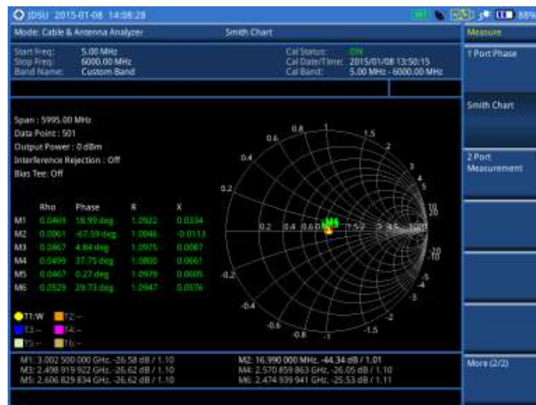
Figure 329 Smith chart measurement
