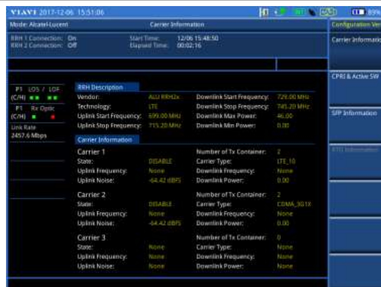
Figure 418 Example of verification of carrier configuration
