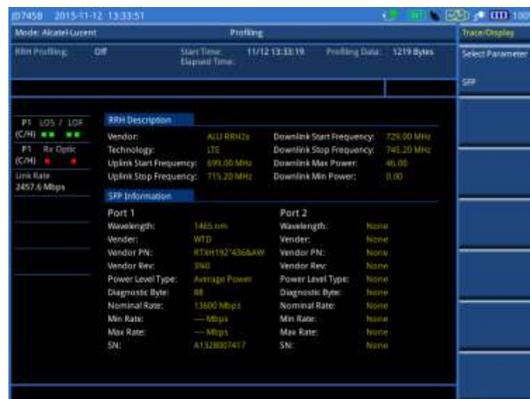
Figure 416 Example of RRH profiling results with SFP information
