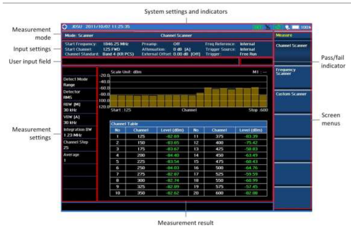
Figure 439 Channel scanner screen
