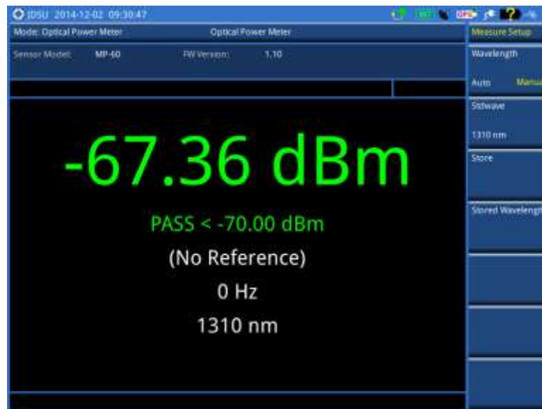
Figure 454 optical power measurement
