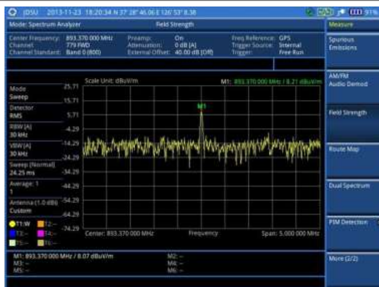
Figure 37 Field strength measurement with spectrum analyzer (on 28 GHz downconverter)
