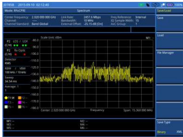
Figure 345 RFoCPRI spectrum measurement
