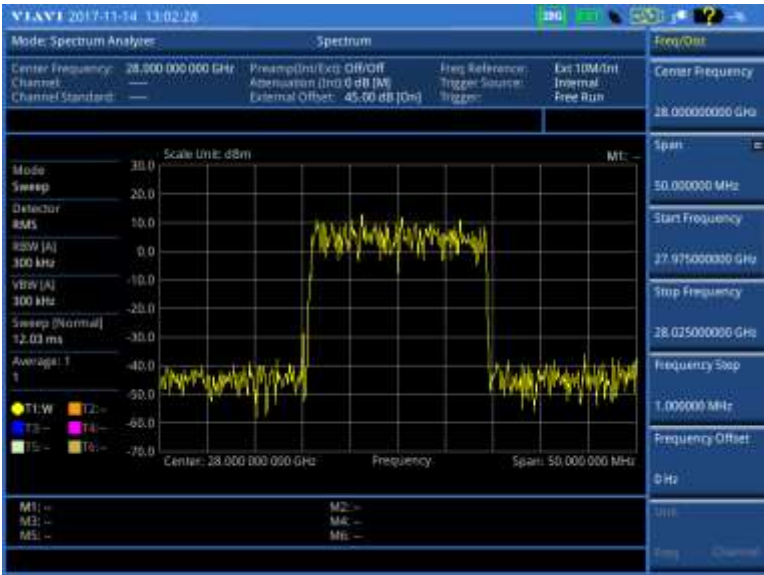
Figure 18 Gated sweep measurement with spectrum analyzer
