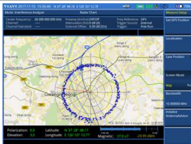
Figure 60 RSSI data plotted on the radar chart (on 28 GHz downconverter)
