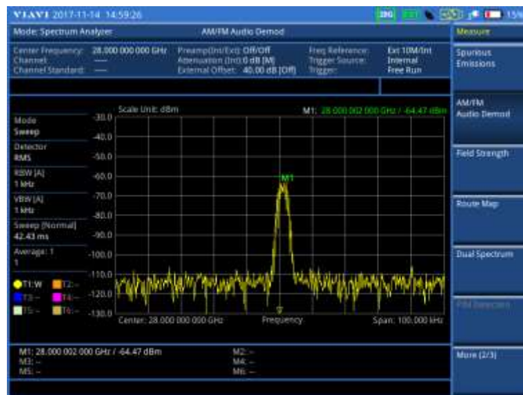
Figure 35 AM/FM audio demodulation with spectrum analyzer (on 28 GHz downconverter)
