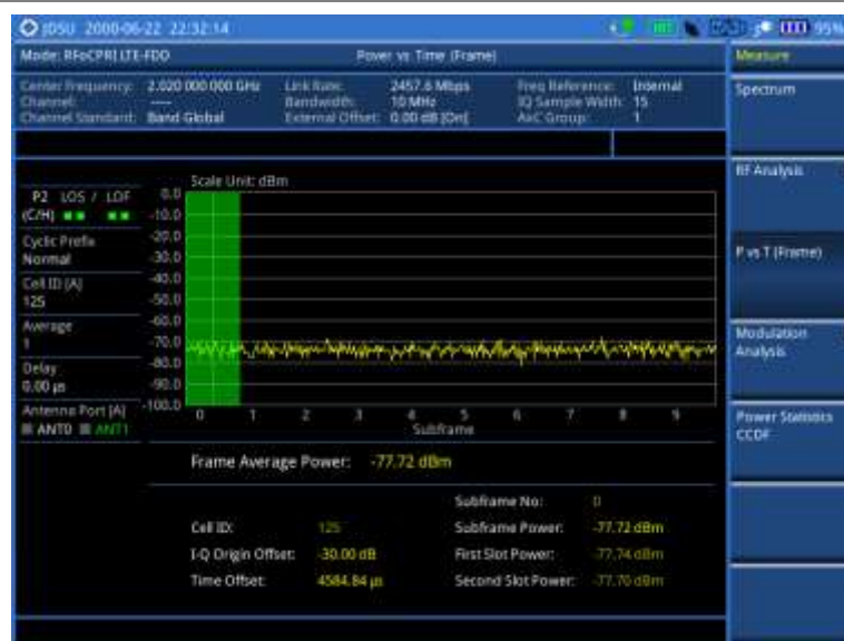
Figure 364 Power vs. time (frame) measurement with RFoCPRI LTE-FDD signal analyzer
