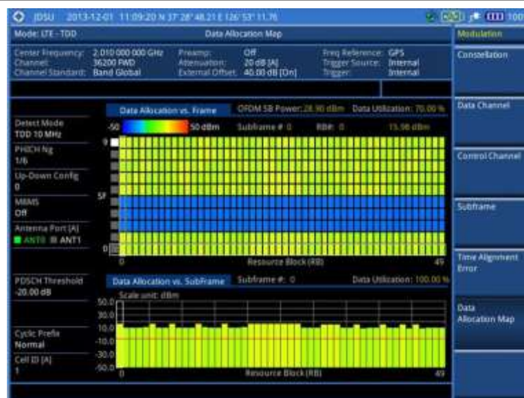
Figure 181 Data allocation map measurement with LTE-TDD signal analyzer
