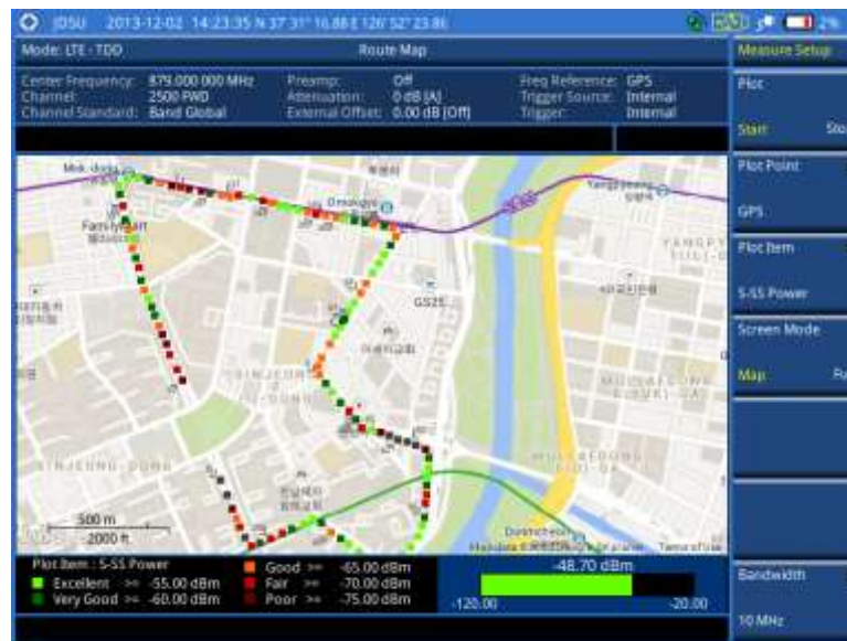
Figure 198 Route map measurement (S-SS Power) with LTE-TDD OTA signal analyzer
