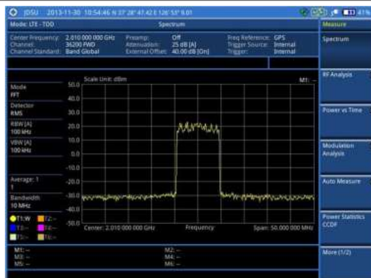
Figure 162 Spectrum measurement screen with LTE-TDD signal analyzer
