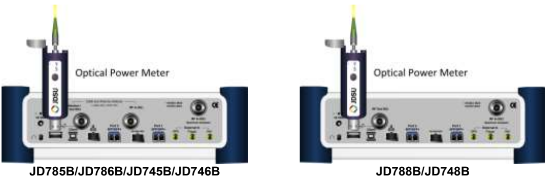
Figure 453 Optical power sensor connection
