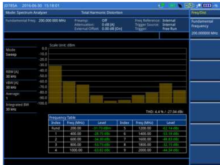
Figure 43 Total harmonic distortion screen
