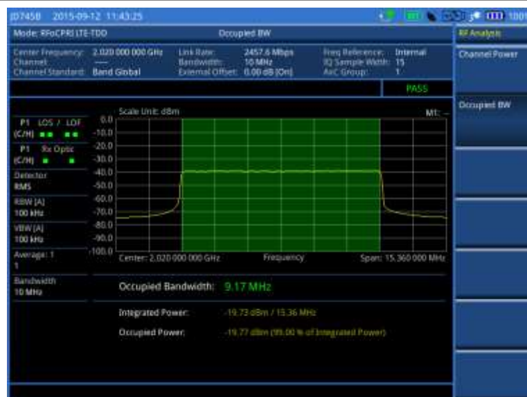
Figure 377 Occupied bandwidth measurement with RFoCPRI LTE-TDD signal analyzer
