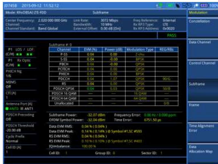
Figure 407 Subframe measurement with RFoBSAI LTE-FDD signal analyzer
