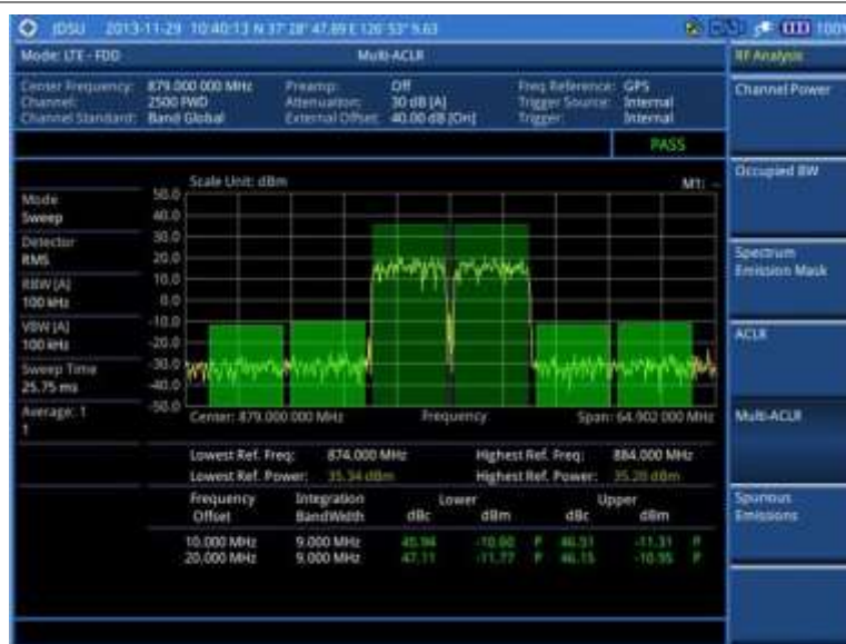
Figure 118 Multi-ACLR measurement with LTE-FDD signal analyzer
