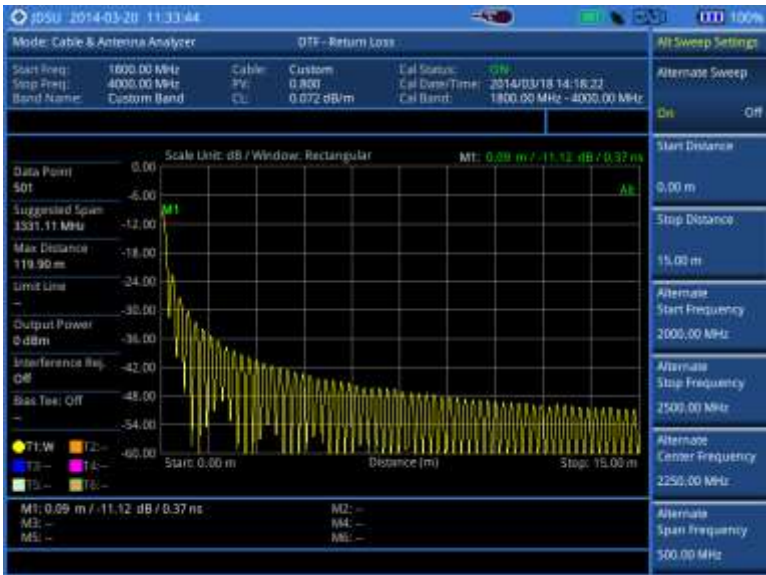
Figure 323 DTF measurement with the alternate sweep on
