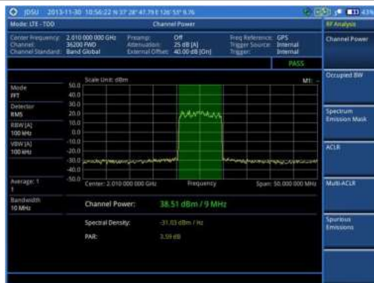
Figure 163 Channel power measurement with LTE-TDD signal analyzer
