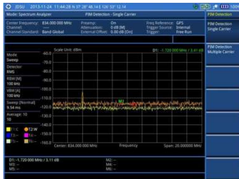
Figure 41 PIM detection for single carrier
