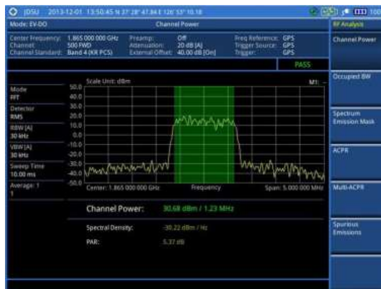
Figure 231 Channel power measurement with EV-DO signal analyzer
