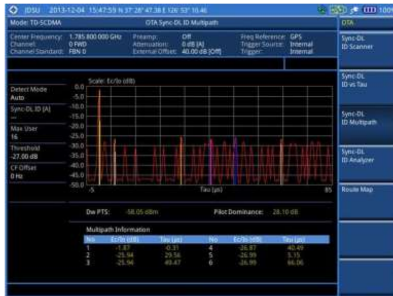
Figure 272 Sync-DL ID multipath measurement with TD-SCDMA OTA signal analyzer
