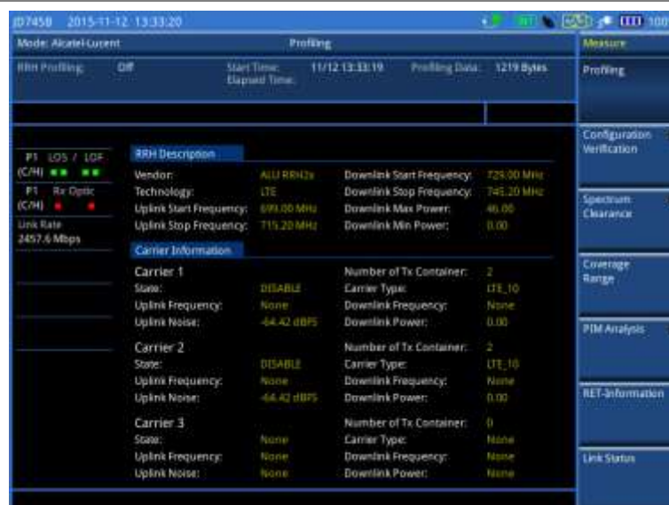
Figure 414 Example of RRH profiling results with carrier information
