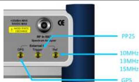
Figure 279 Connection ports for external reference clock
