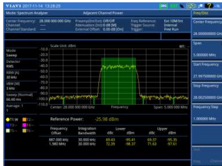
Figure 29 Adjacent channel power measurement with spectrum analyzer (on 28 GHz downconverter)
