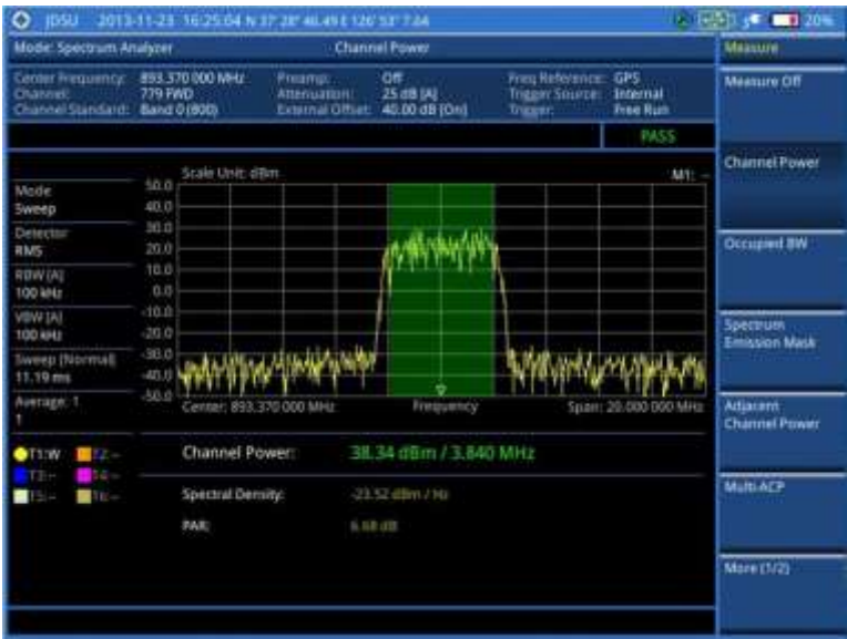
Figure 21 Channel power measurement with spectrum analyzer
