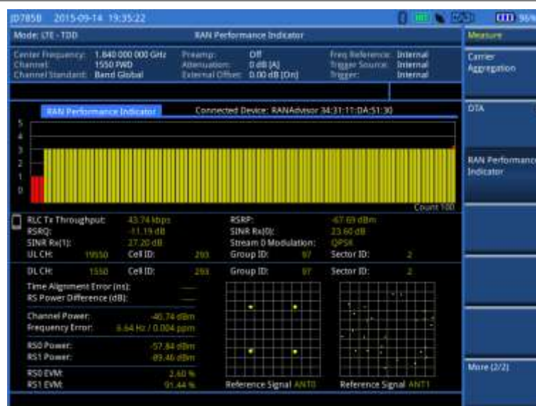
Figure 201 RAN performance indicator with LTE-TDD signal analyzer
