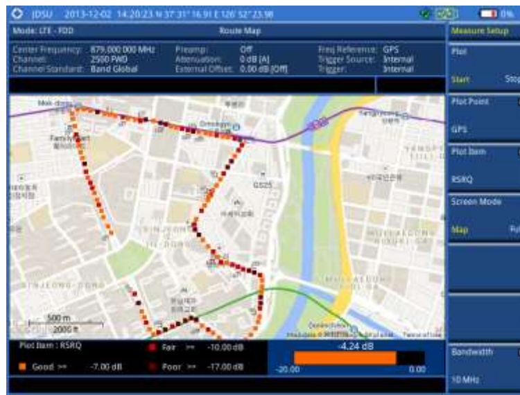
Figure 149 Route map measurement (RSRQ) with LTE-FDD OTA signal analyzer
