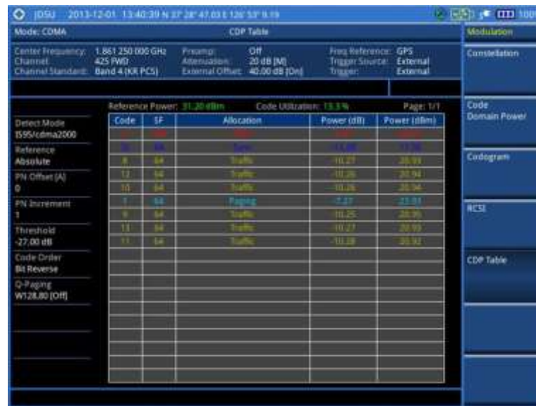
Figure 218 CDP Table measurement with CDMA signal analyzer
