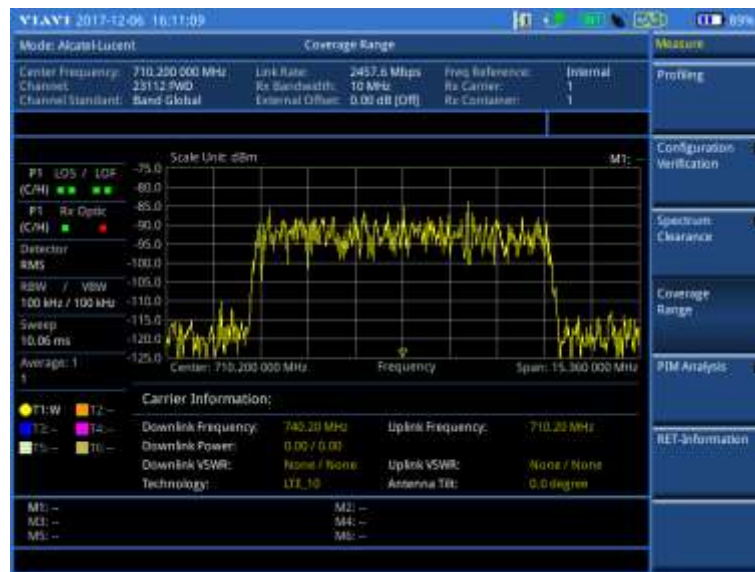
Figure 429 Example of coverage range in Alcatel-Lucent BBU emulation
