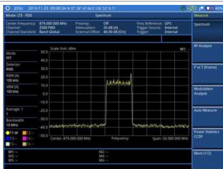
Figure 113 Spectrum measurement screen with LTE-FDD signal analyzer
