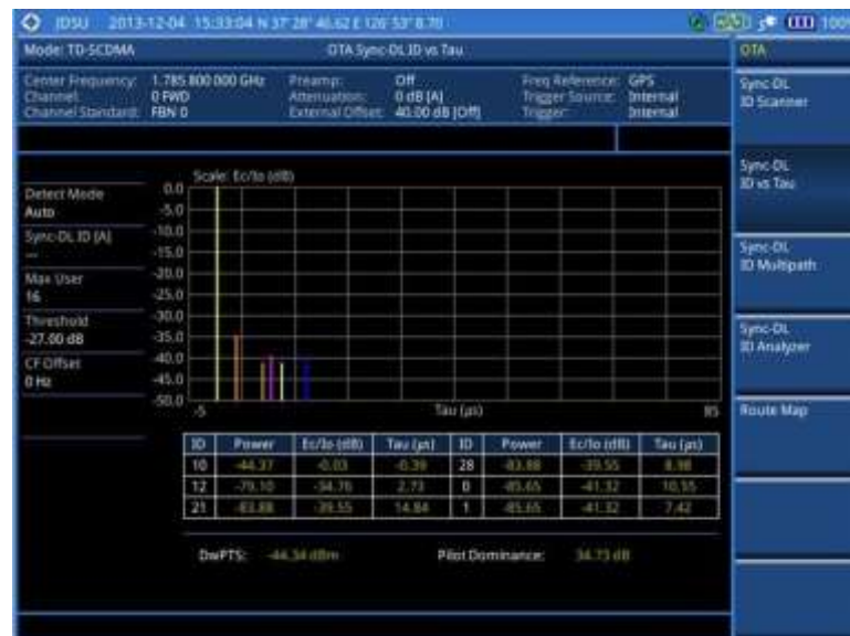
Figure 271 Sync-DL ID vs. Tau measurement with TD-SCDMA OTA signal analyzer
