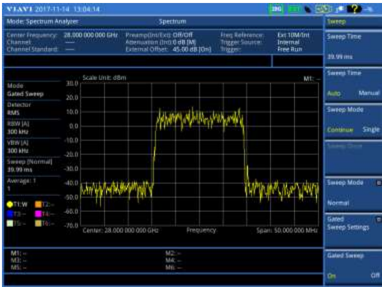
Figure 21 Gated sweep measurement with spectrum analyzer (on 28 GHz downconverter)
