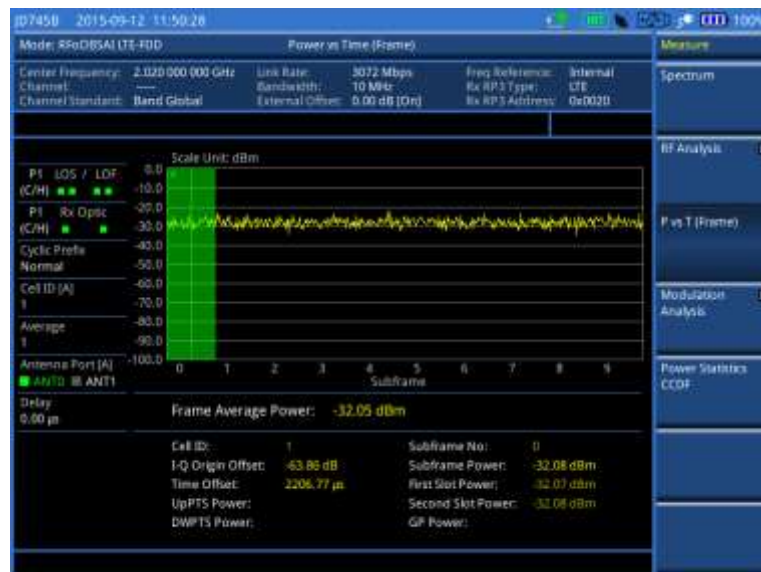
Figure 404 Power vs. time (frame) measurement with RFoOBSAI LTE-FDD signal analyzer
