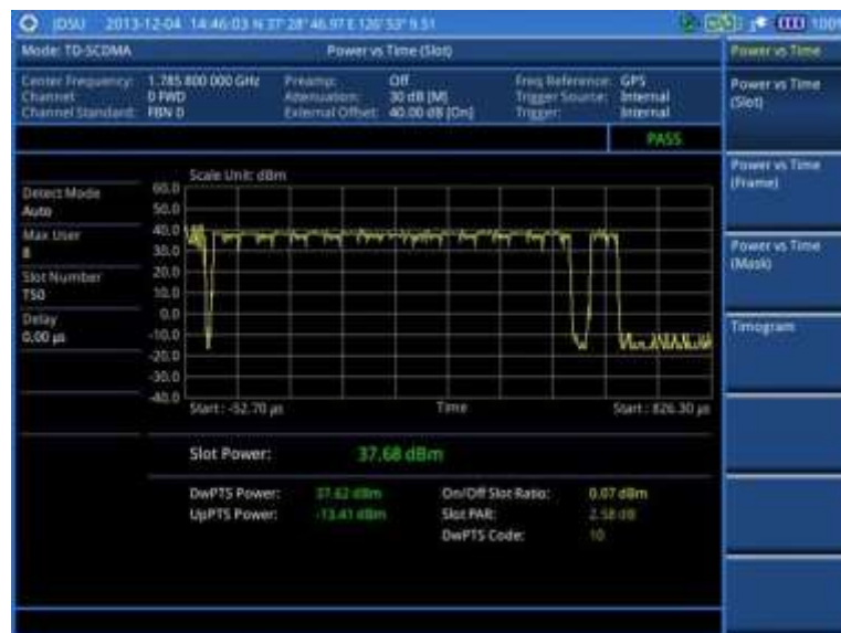
Figure 264 Power vs. time (slot) measurement with TD-SCDMA signal analyzer
