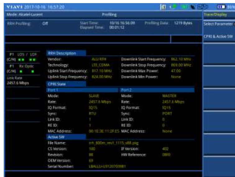
Figure 419 Example of RRH profiling results with SFP information
