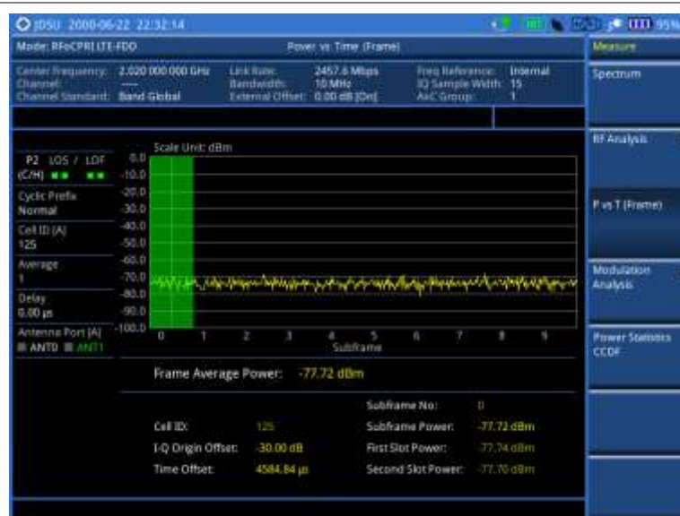
Figure 366 Power vs. time (frame) measurement with RFoCPRI LTE-FDD signal analyzer
