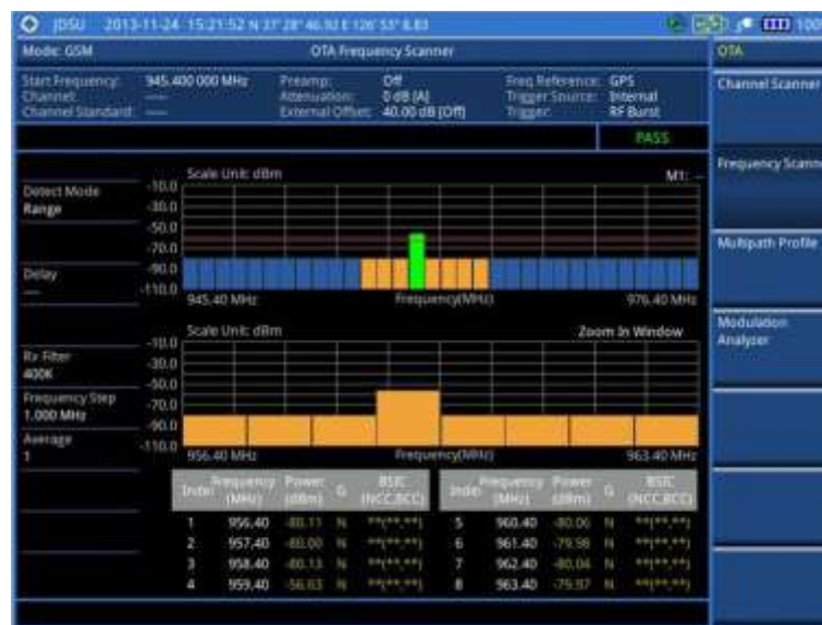
Figure 81 Frequency scanner measurement with GSM OTA signal analyzer
