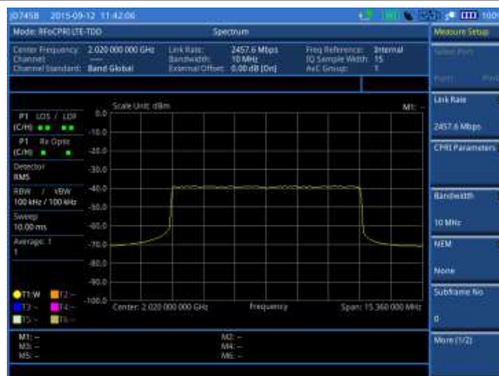
Figure 377 Spectrum measurement with RFoCPRI LTE-TDD signal analyzer
