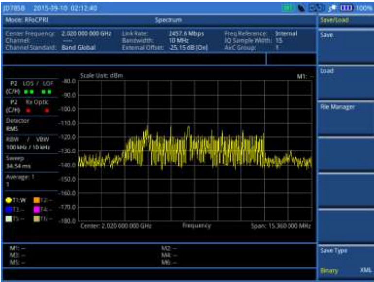
Figure 348 RFoCPRI spectrum analysis on LTE Uplink 10 MHz, antenna 1
