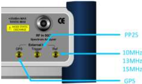
Figure 300 Connection ports for external reference clock
