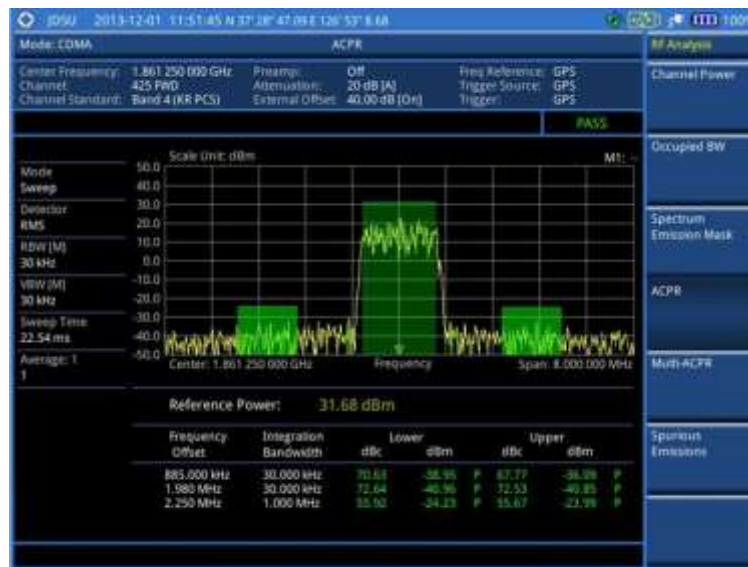
Figure 213 ACPR measurement with CDMA signal analyzer
