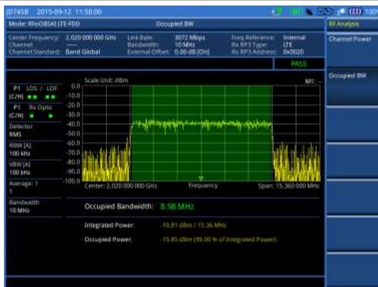
Figure 403 Occupied bandwidth measurement with RFoBSAI LTE-FDD signal analyzer
