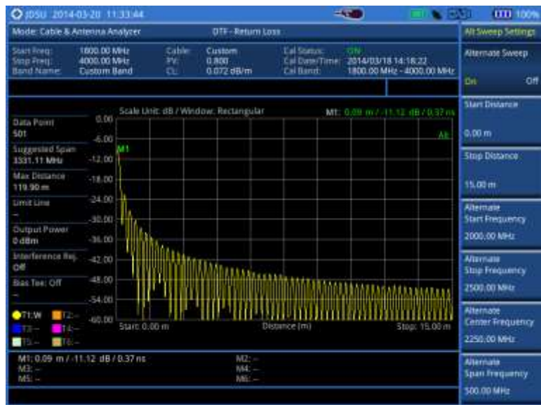
Figure 325 DTF measurement with the alternate sweep on
