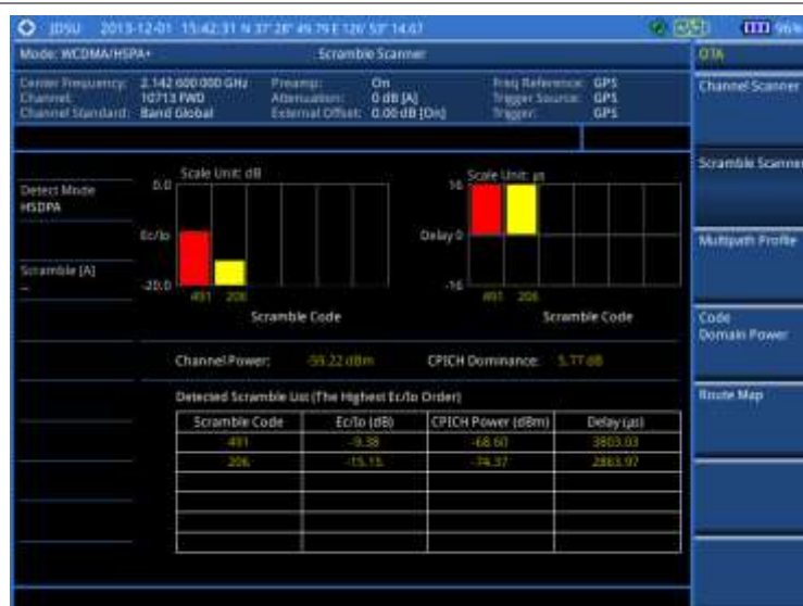
Figure 104 Scramble scanner measurement with WCDMA/HSPA+ OTA signal analyzer
