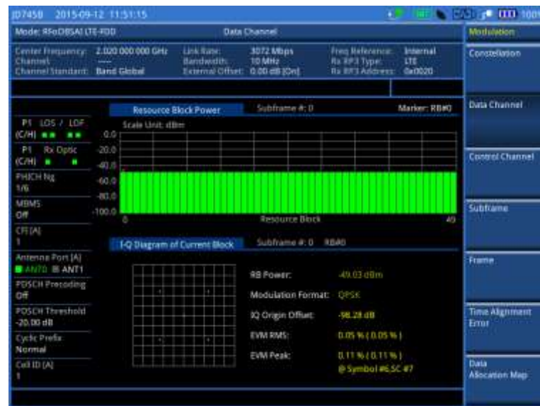
Figure 406 Data channel measurement with RFoOBSAI LTE-FDD signal analyzer
