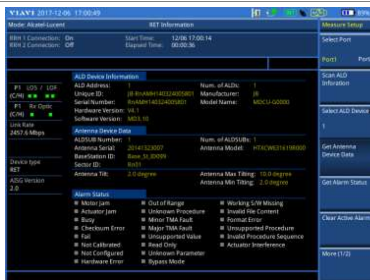
Figure 437 Example of antenna device data in Alcatel-Lucent RET information
