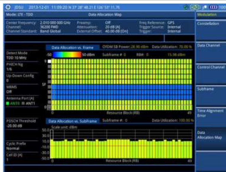
Figure 183 Data allocation map measurement with LTE-TDD signal analyzer
