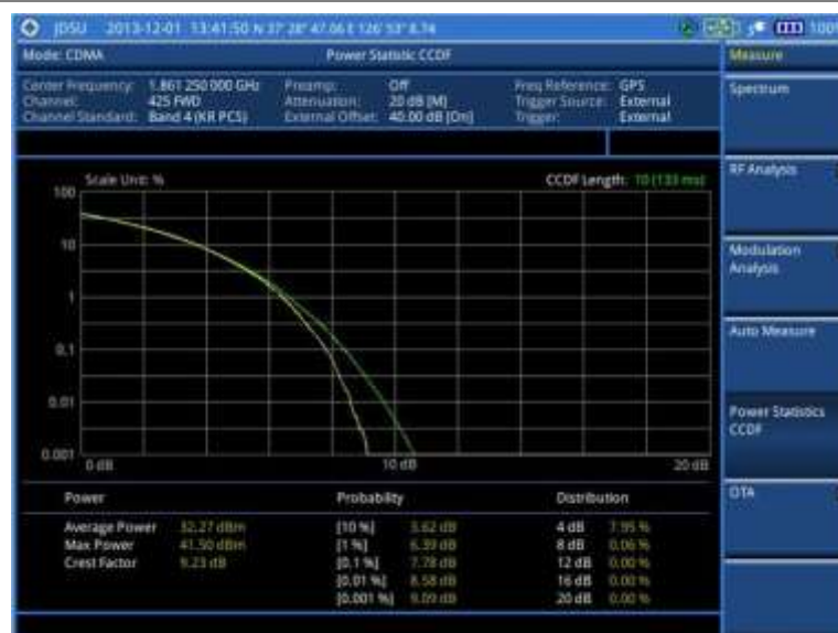
Figure 221 CCDF measurement with CDMA signal analyzer
