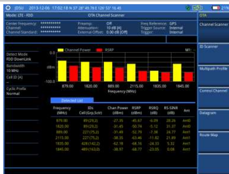
Figure 145 Channel scanner measurement with LTE-FDD OTA signal analyzer
