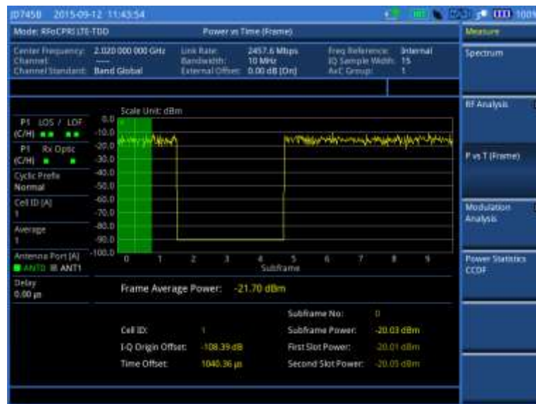
Figure 380 Power vs. time (frame) measurement with RFoCPRI LTE-TDD signal analyzer
