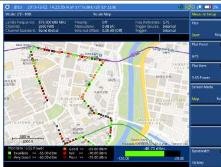
Figure 155 Route map measurement (S-SS Power) with LTE-FDD OTA signal analyzer
