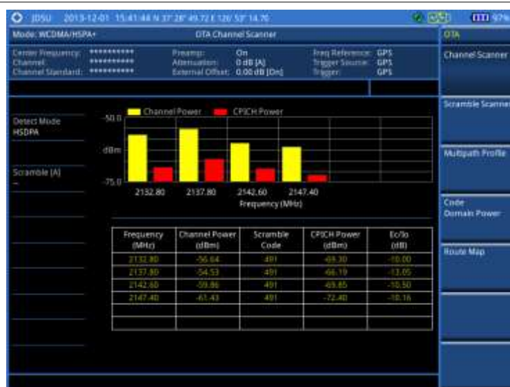
Figure 103 Channel scanner measurement with WCDMA/HSPA+ OTA signal analyzer
