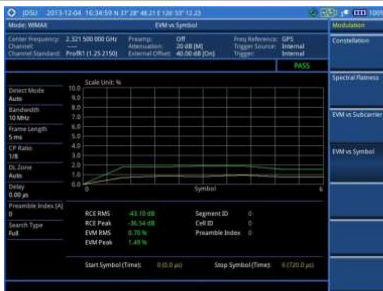
Figure 291 EVM vs. symbol measurement with Mobile WiMAX signal analyzer
