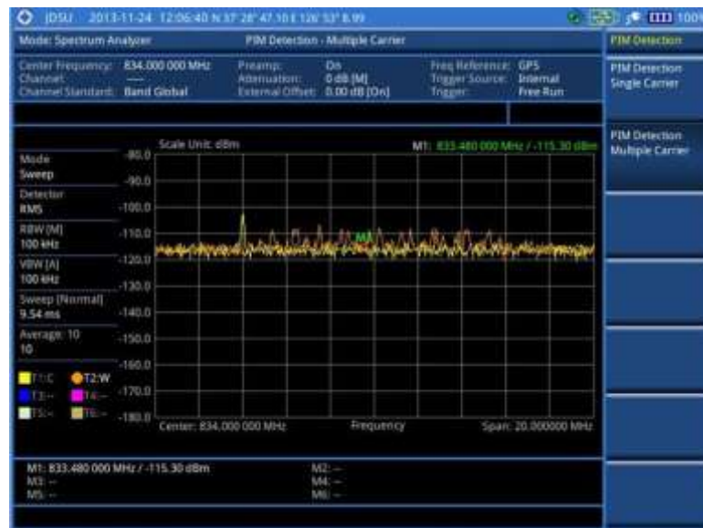
Figure 44 PIM detection for multiple carriers
