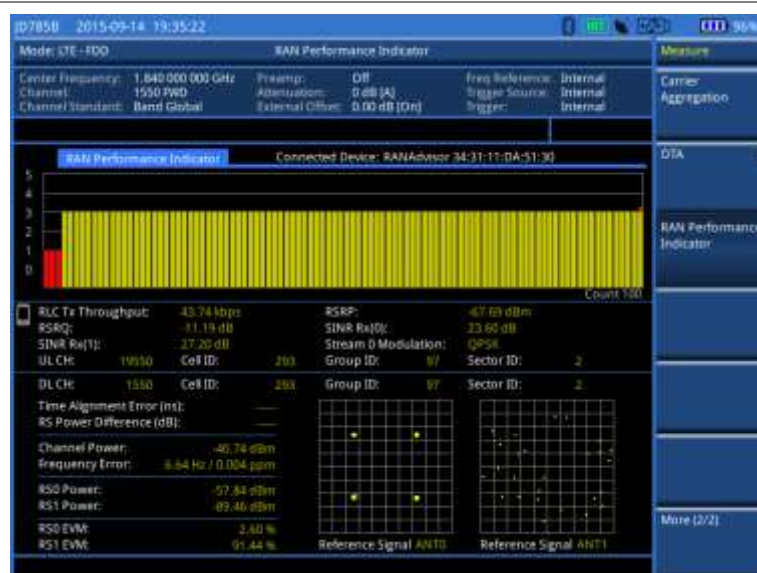
Figure 158 RAN performance indicator with LTE-FDD signal analyzer
