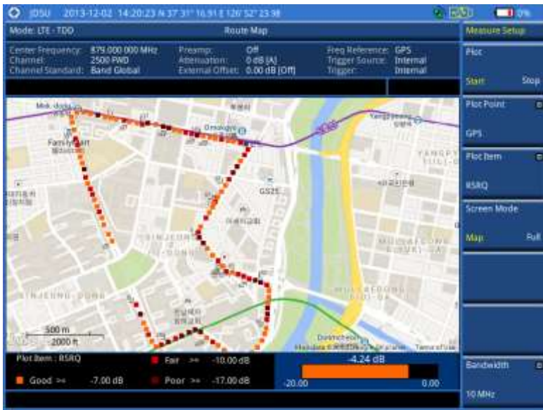
Figure 197 Route map measurement (RS-SINR) with LTE-TDD OTA signal analyzer
