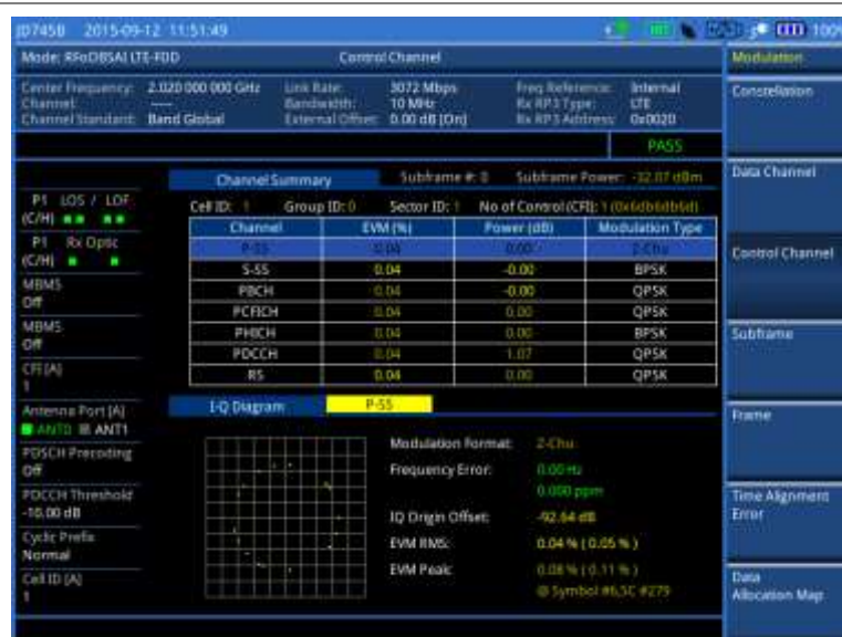
Figure 407 Control channel measurement with RFoBSAI LTE-FDD signal analyzer
