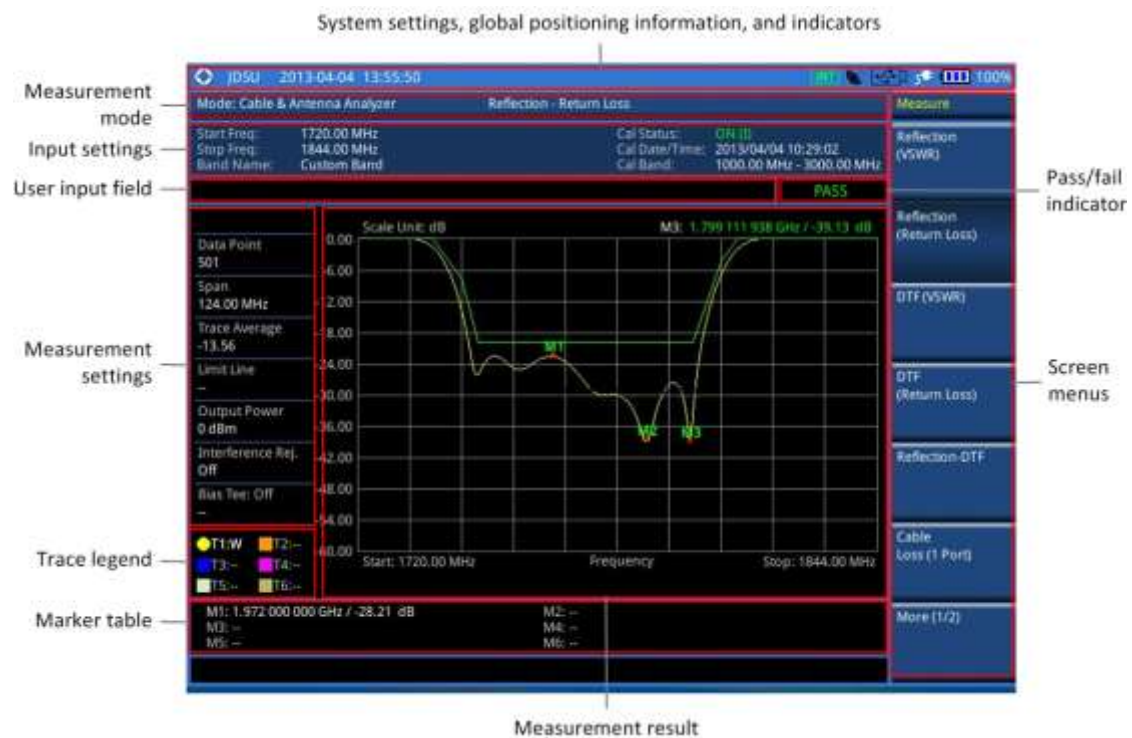
Figure 313 Reflection measurement screen
