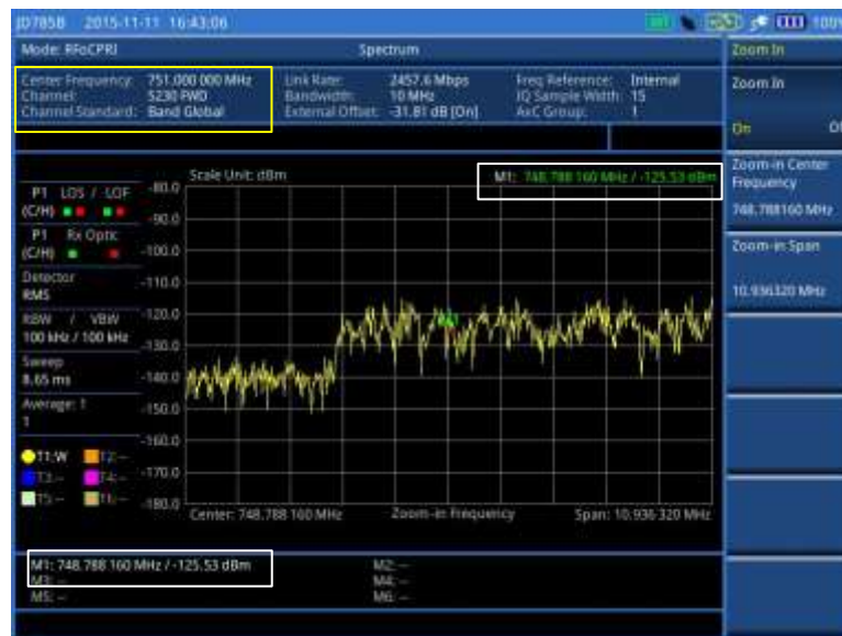
Figure 358 Zoomed-in spectrum view in RFoCPRI interference analyzer
