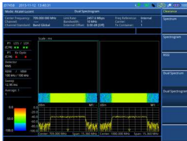
Figure 430 Example of dual spectrogram analysis in Alcatel-Lucent BBU emulation
