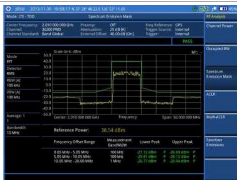
Figure 167 SEM measurement with LTE-TDD signal analyzer
