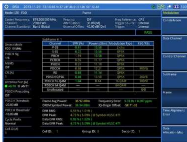
Figure 133 Frame measurement with LTE-FDD signal analyzer
