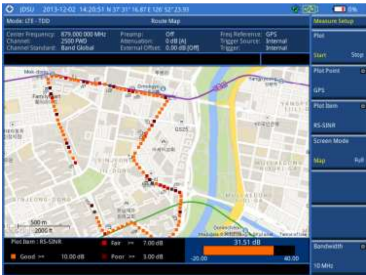
Figure 197 Route map measurement (RS-SINR) with LTE-TDD OTA signal analyzer
