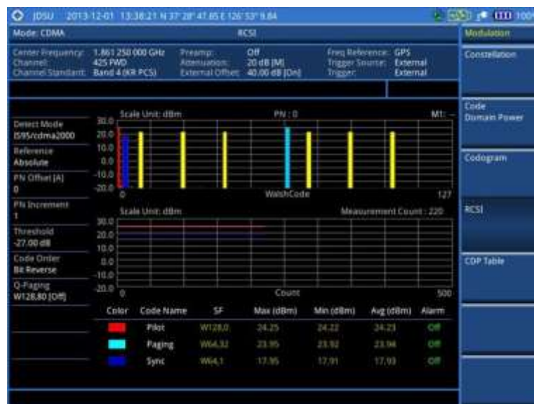
Figure 219 RCSI measurement with CDMA signal analyzer
