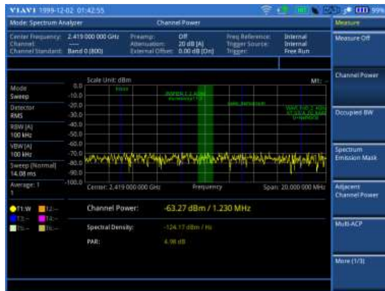
Figure 25 Wi-Fi SSID display in channel power measurement with spectrum analyzer
