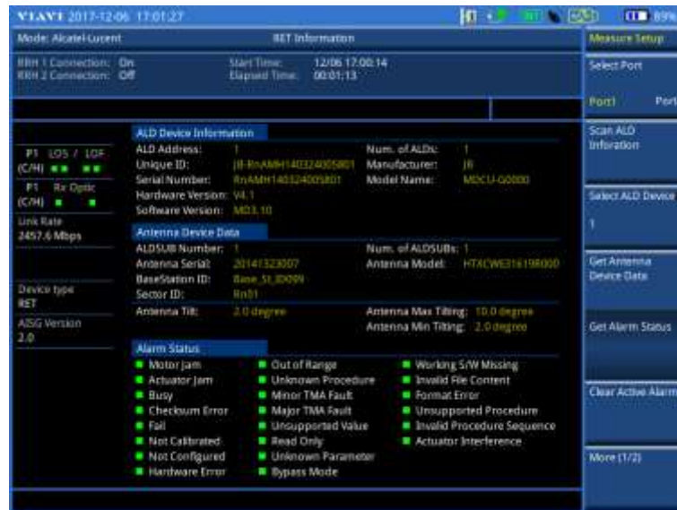
Figure 438 Example of getting alarm status in Alcatel-Lucent RET information
