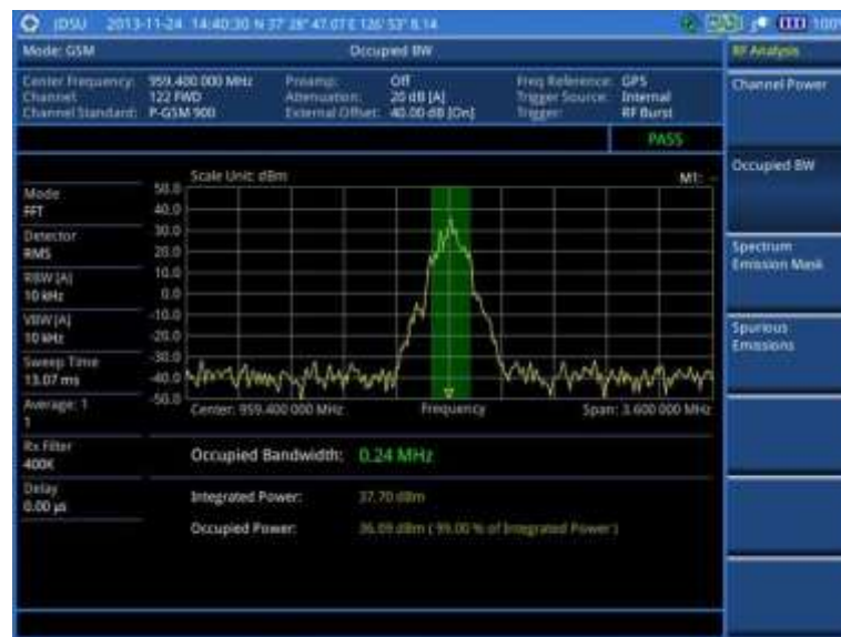
Figure 71 Occupied bandwidth measurement with GSM signal analyzer
