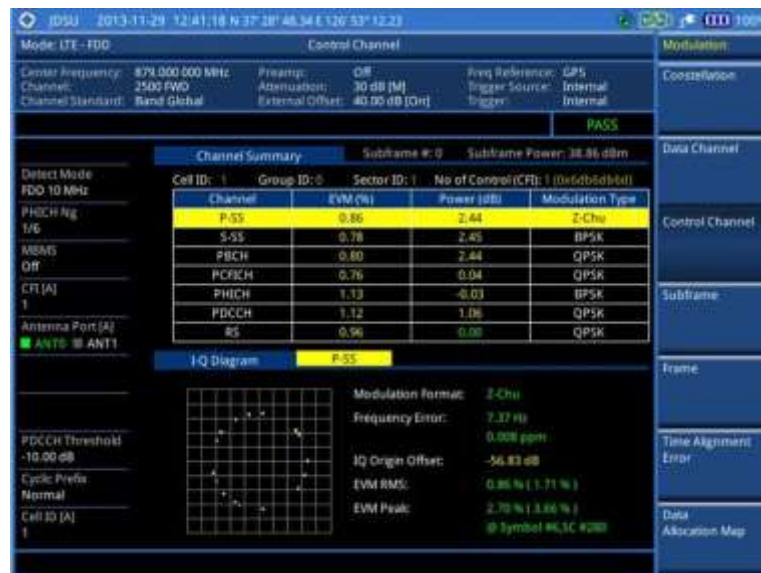
Figure 128 Control channel measurement with LTE-FDD signal analyzer
