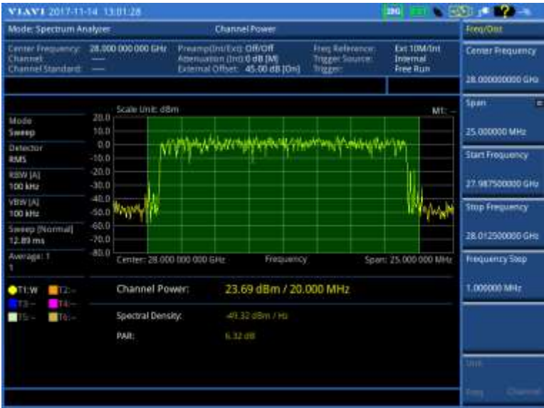
Figure 24 Channel power measurement with spectrum analyzer (on 28 GHz downconverter)
