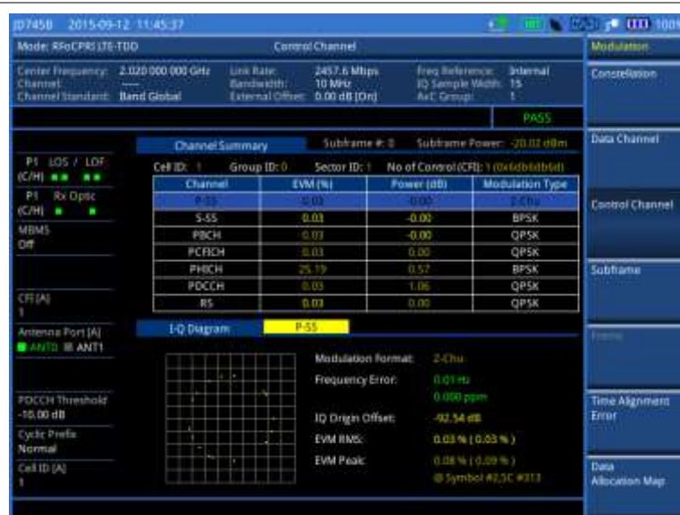
Figure 383 Control channel measurement with RFoCPRI LTE-TDD signal analyzer
