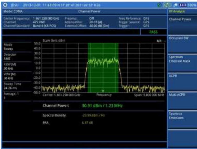
Figure 210 Channel power measurement with CDMA signal analyzer
