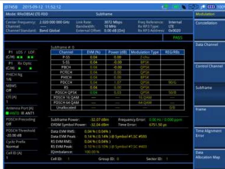
Figure 409 Subframe measurement with RFoBSAI LTE-FDD signal analyzer
