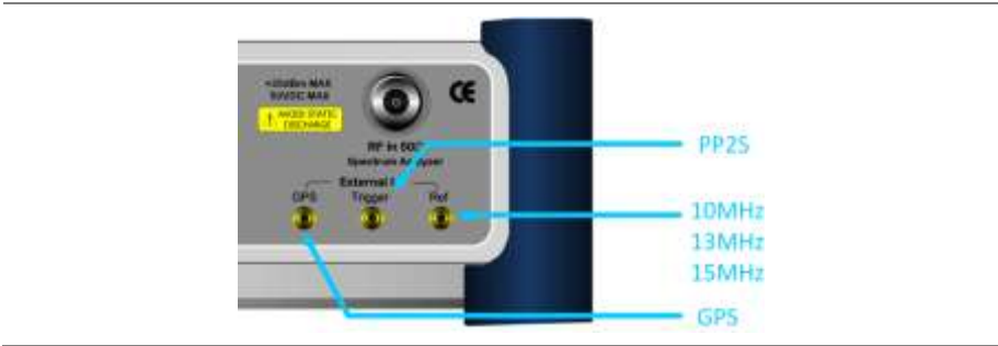
Figure 256 Connection ports for external reference clock
