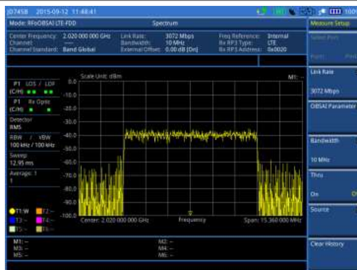
Figure 401 Spectrum measurement with RFoBSAI LTE-FDD signal analyzer
