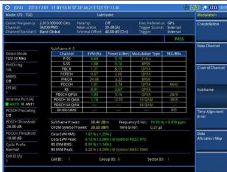
Figure 179 Subframe measurement with LTE-TDD signal analyzer
