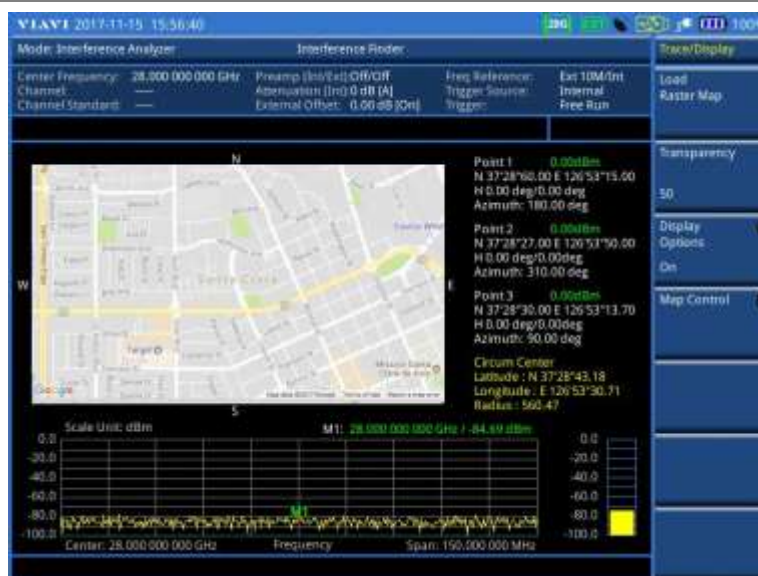
Figure 60 Raster image overlaid on the map in interference finder (on 28 GHz downconverter)
