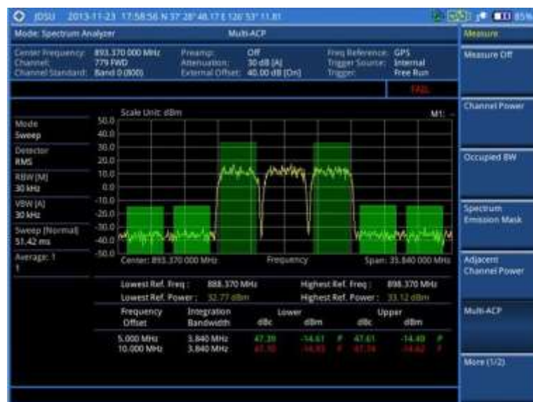
Figure 32 Multi-ACP measurement with spectrum analyzer
