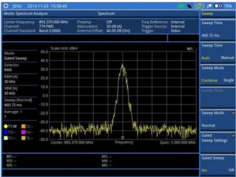
Figure 20 Gated sweep measurement with spectrum analyzer
