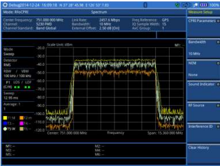
Figure 348 RFoCPRI spectrum analysis on LTE Uplink 10 MHz, antenna 1
