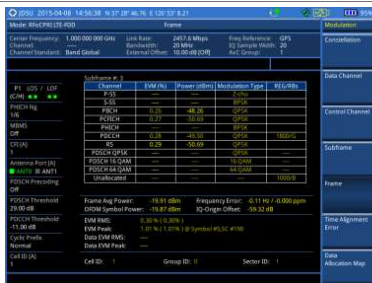
Figure 372 Frame measurement with RFoCPRI LTE-FDD signal analyzer
