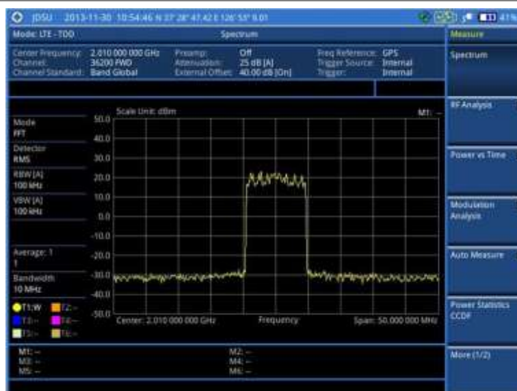
Figure 164 Spectrum measurement screen with LTE-TDD signal analyzer
