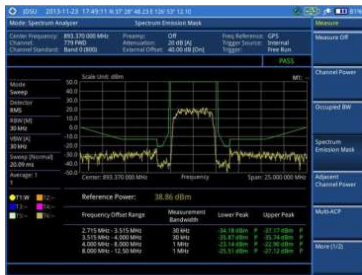
Figure 29 Spectrum emission mask measurement with spectrum analyzer (on 28 GHz downconverter)
