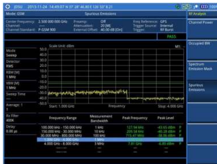
Figure 74 Spurious emissions measurement with GSM signal analyzer
