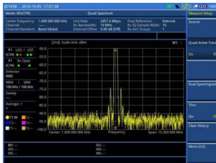
Figure 353 RFoCPRI quad spectrum with quad active trace off
