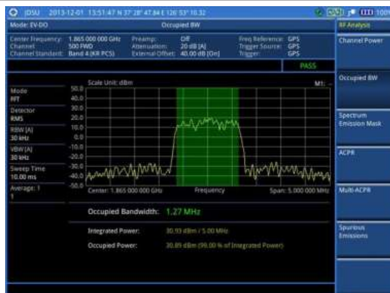
Figure 234 Occupied bandwidth measurement with EV-DO signal analyzer
