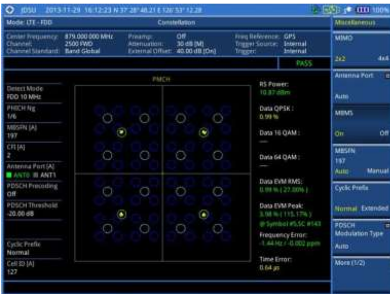
Figure 124 Constellation measurement with LTE-FDD signal analyzer (MBMS On)
