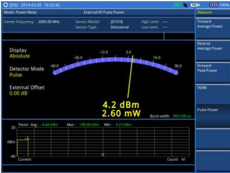
Figure 455 External power measurement of pulse power
