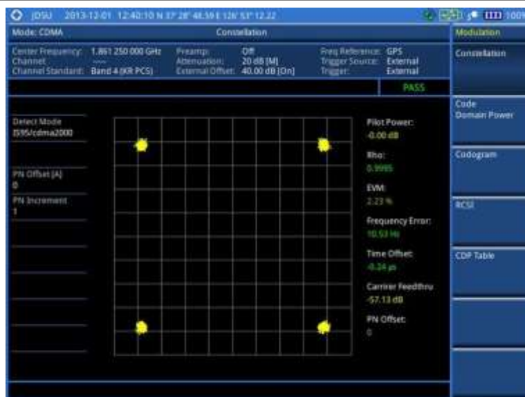
Figure 216 Constellation measurement with CDMA signal analyzer
