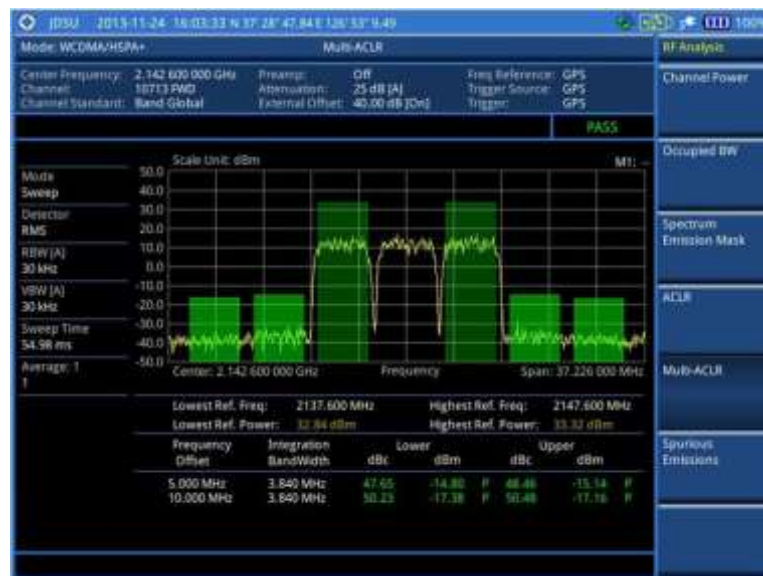
Figure 94 Multi-ACLR measurement with WCDMA/HSPA+ signal analyzer
