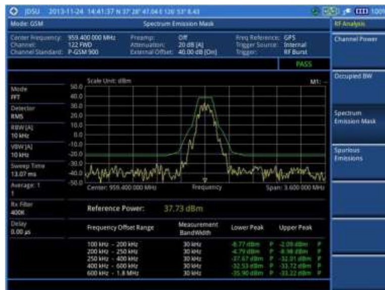
Figure 72 SEM measurement with GSM signal analyzer
