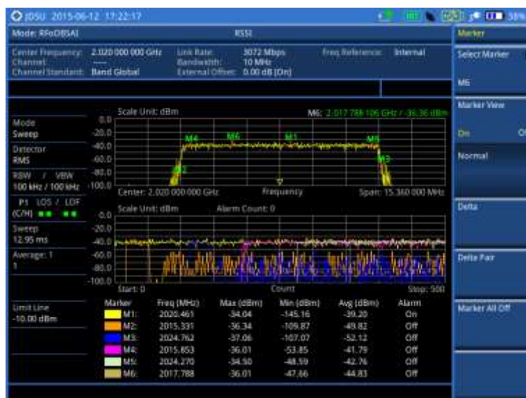
Figure 396 RFoBSAI interference measurement in RSSI
