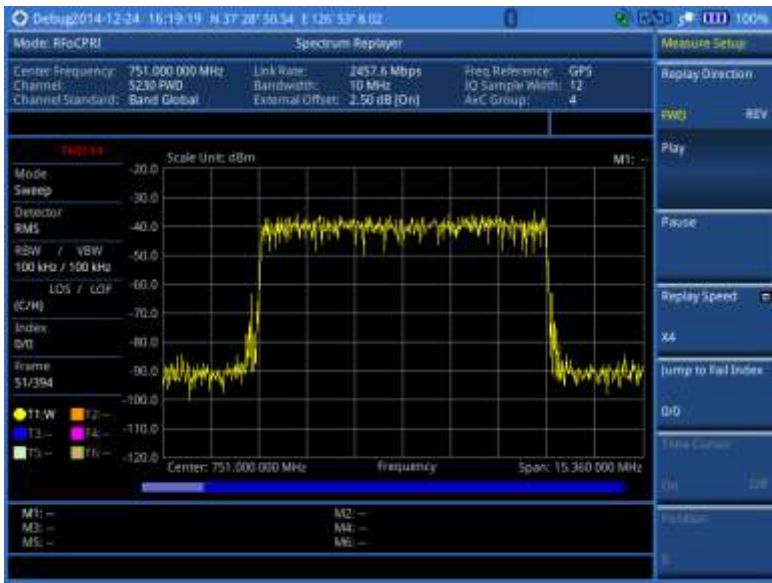
Figure 359 RFoCPRI spectrum replay
