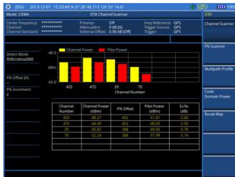
Figure 222 Channel scanner measurement with CDMA OTA signal analyzer
