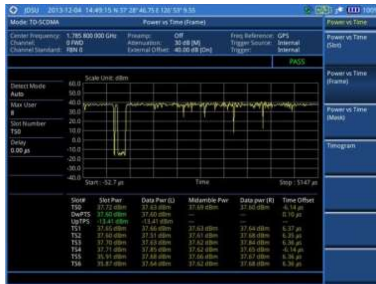
Figure 265 Power vs. time (frame) measurement with TD-SCDMA signal analyzer
