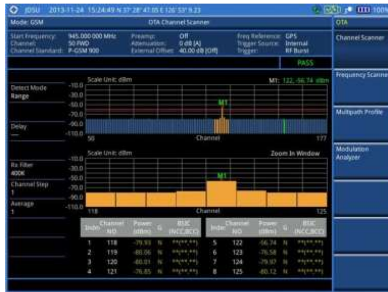
Figure 80 Channel scanner measurement with GSM OTA signal analyzer
