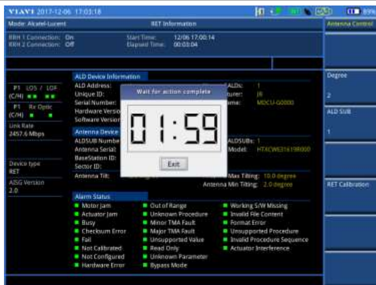
Figure 439 Example of antenna tilting in Alcatel-Lucent RET information
