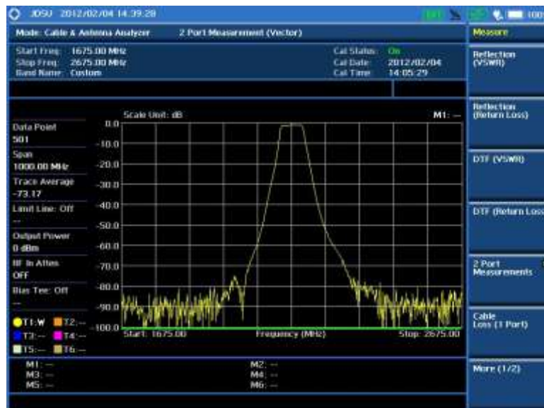
Figure 332 2-port vector measurement
