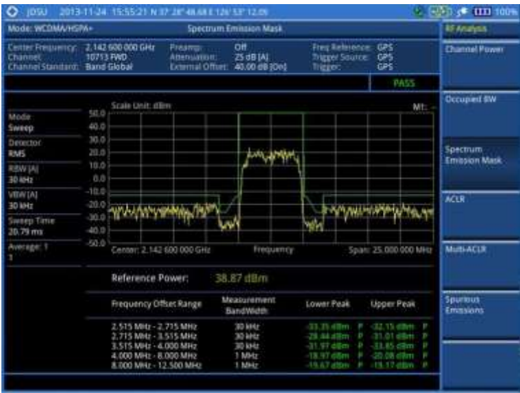
Figure 92 SEM measurement with WCDMA/HSPA+ signal analyzer
