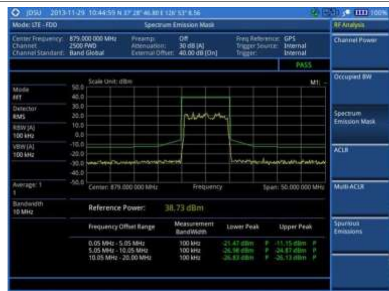
Figure 118 SEM measurement with LTE-FDD signal analyzer
