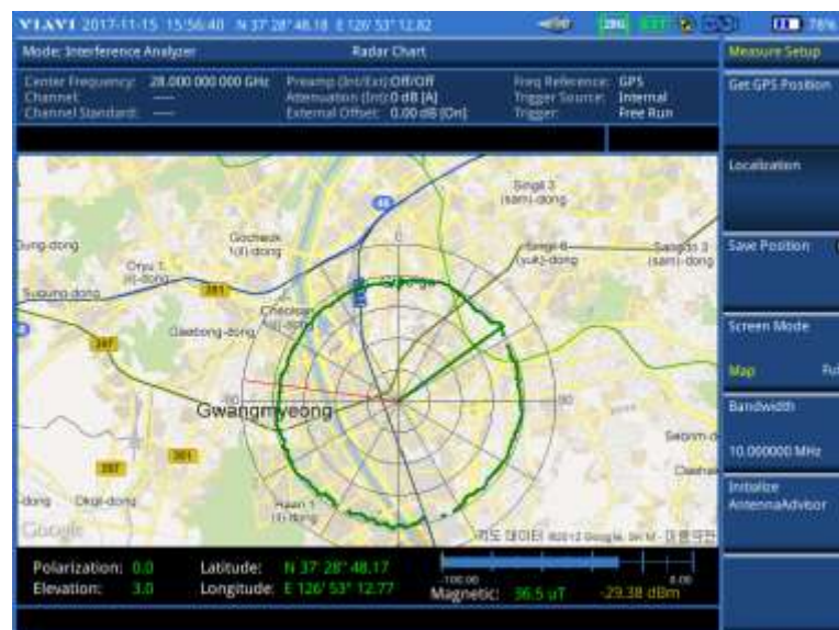
Figure 64 Localized RSSI data on the radar chart (on 28 GHz downconverter)
