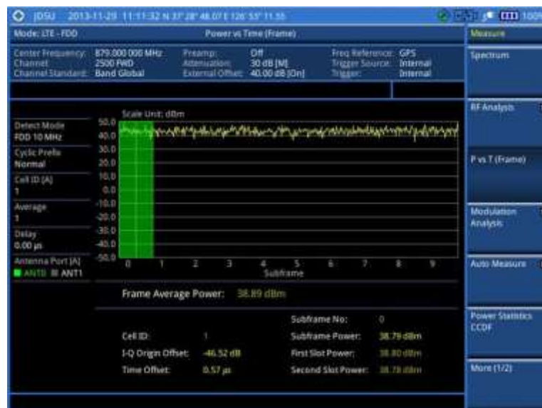
Figure 122 Power vs. time (frame) measurement with LTE – FDD signal analyzer
