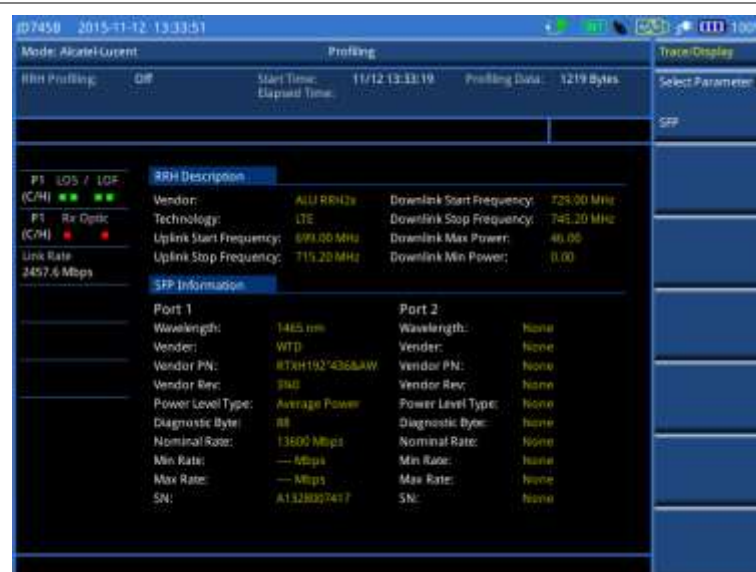
Figure 419 Example of RRH profiling results with SFP information
