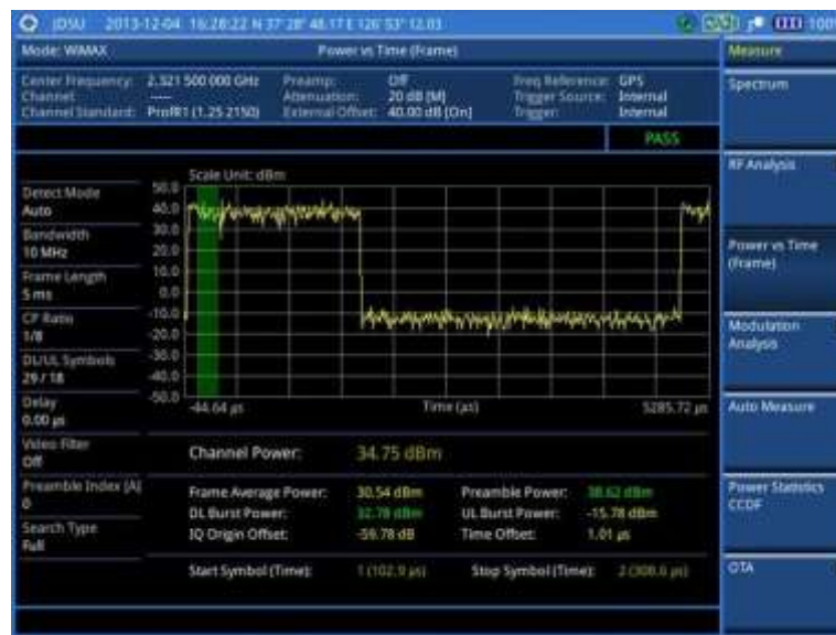
Figure 287 Power vs. time (frame) measurement with Mobile WiMAX signal analyzer
