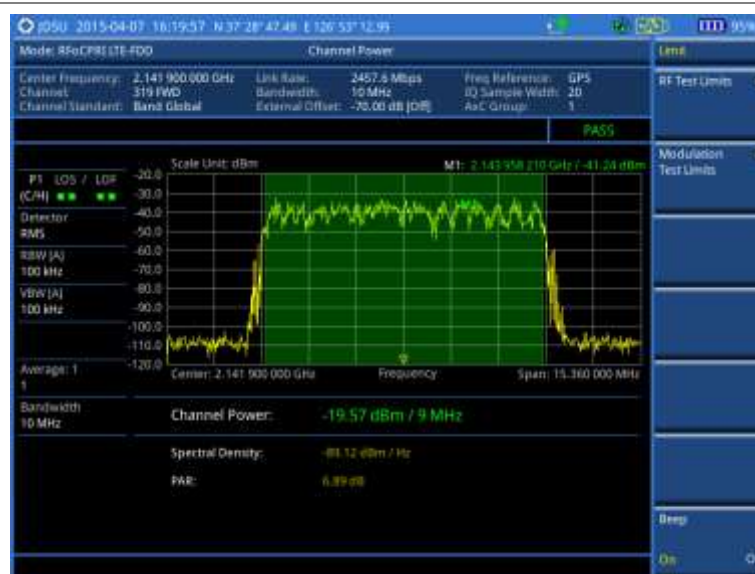
Figure 364 Channel power measurement with RFoCPRI LTE-FDD signal analyzer
