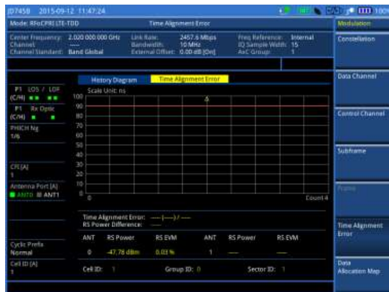
Figure 385 Time alignment error measurement with RFoCPRI LTE-TDD signal analyzer
