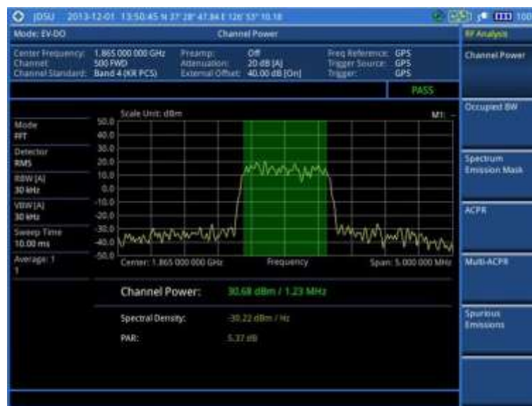
Figure 233 Channel power measurement with EV-DO signal analyzer
