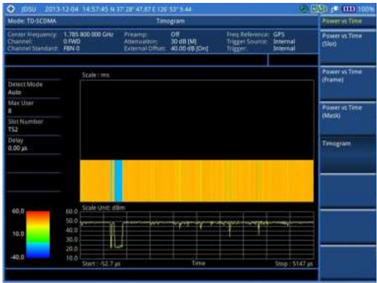
Figure 267 Timogram with TD-SCDMA signal analyzer
