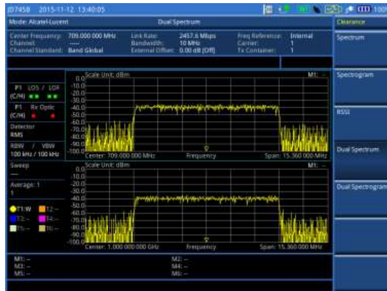
Figure 428 Example of dual spectrum analysis in Alcatel-Lucent BBU emulation
