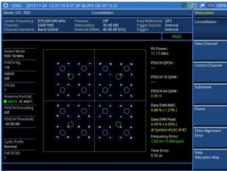
Figure 124 Constellation measurement with LTE-FDD signal analyzer (MBMS On)
