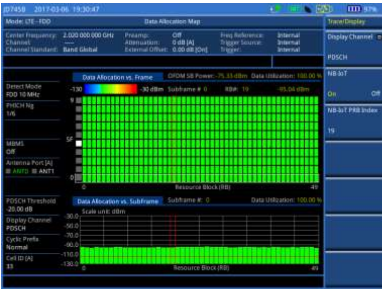
Figure 138 Data allocation map measurement with LTE-FDD signal analyzer (NB-IoT On)
