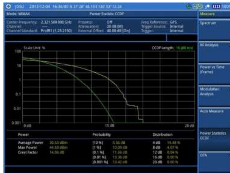
Figure 292 CCDF measurement with Mobile WiMAX signal analyzer
