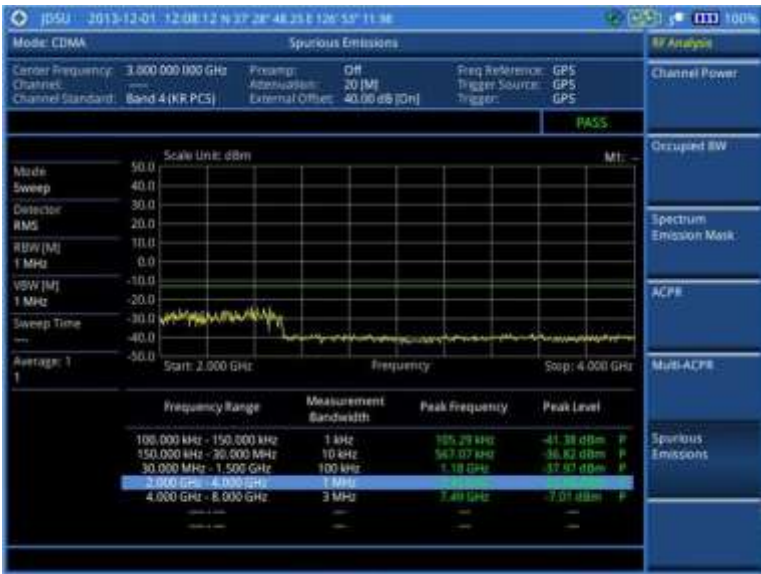
Figure 215 Spurious emissions measurement with CDMA signal analyzer
