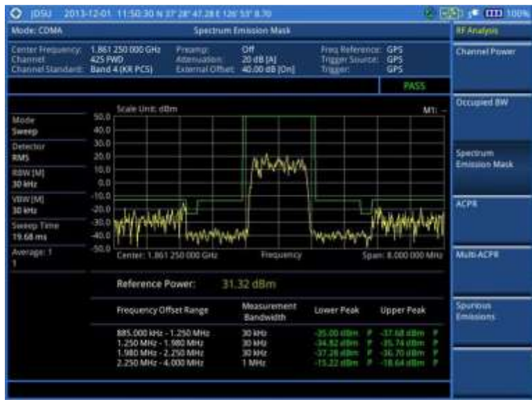
Figure 212 SEM measurement with CDMA signal analyzer
