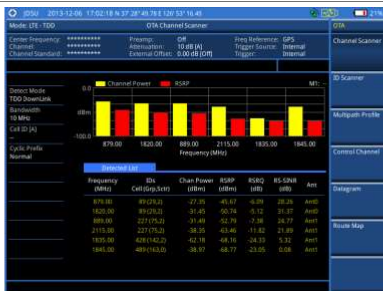
Figure 190 Channel scanner measurement with LTE-TDD OTA signal analyzer
