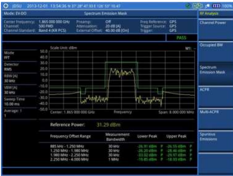
Figure 235 SEM measurement with EV-DO signal analyzer
