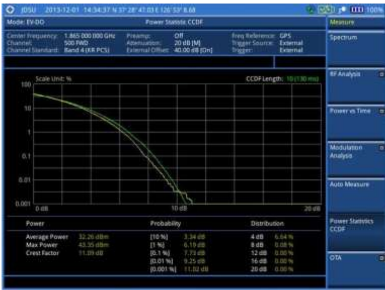
Figure 246 CCDF measurement with EV-DO signal analyzer
