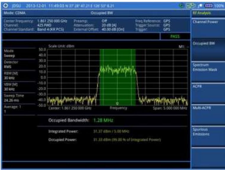
Figure 211 Occupied bandwidth measurement with CDMA signal analyzer
