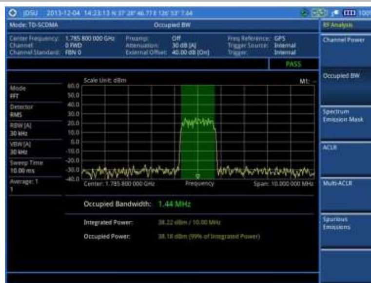
Figure 259 Occupied bandwidth measurement with TD-SCDMA signal analyzer
