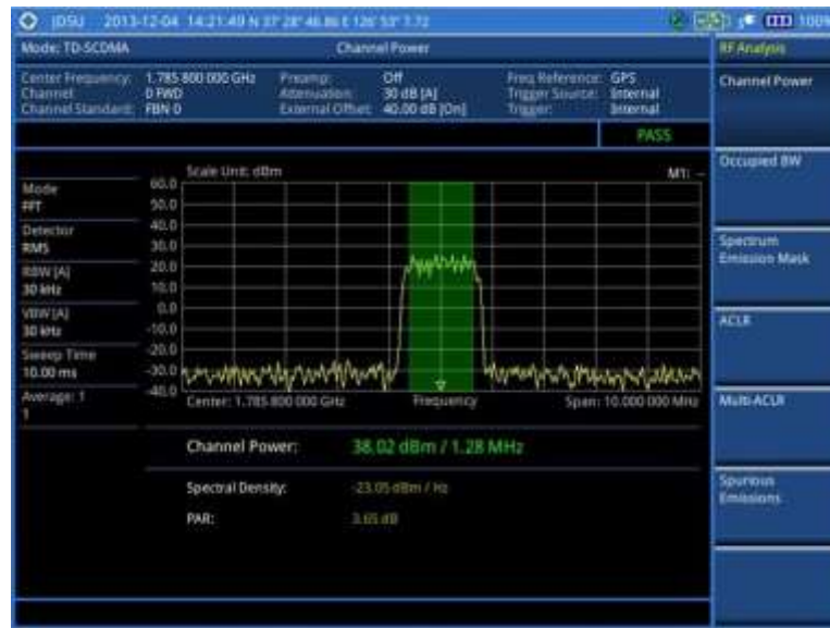
Figure 258 Channel power measurement with TD-SCDMA signal analyzer
