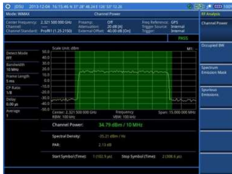
Figure 283 Channel power measurement with Mobile WiMAX signal analyzer
