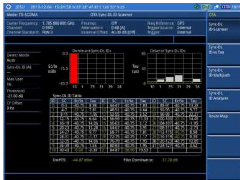
Figure 272 Sync-DL ID scanner measurement with TD-SCDMA OTA signal analyzer
