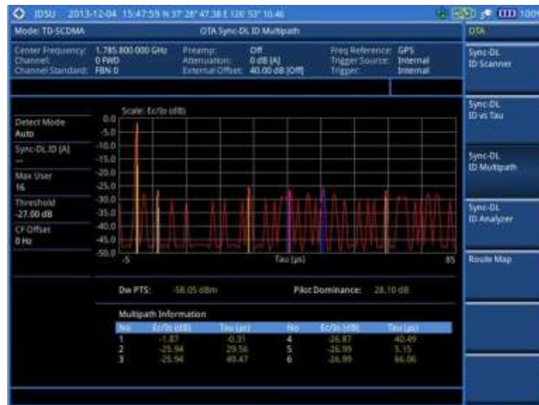
Figure 274 Sync-DL ID multipath measurement with TD-SCDMA OTA signal analyzer
