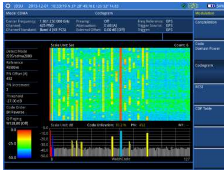
Figure 168 Codogram in full view with CDMA signal analyzer
