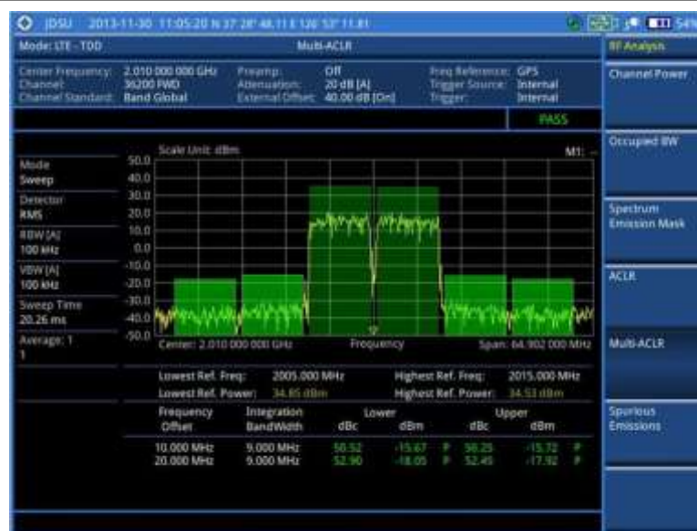
Figure 127 Multi-ACLR measurement with LTE - TDD signal analyzer
