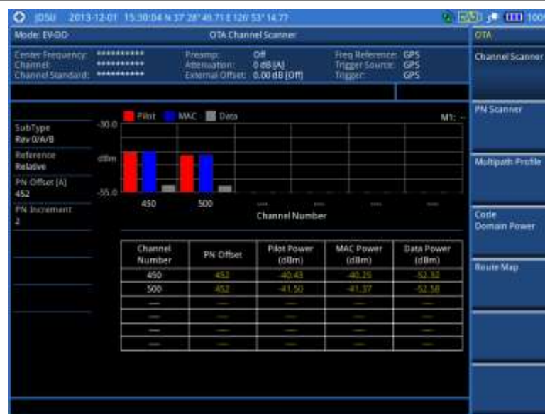
Figure 197 Channel scanner measurement with EV-DO OTA signal analyzer
