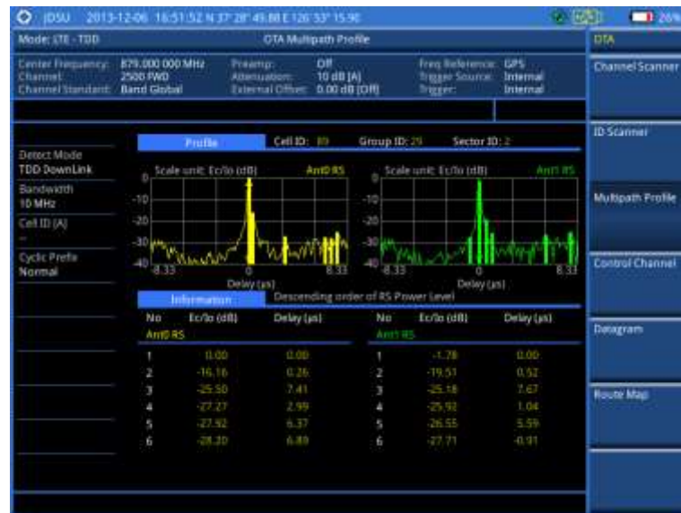
Figure 148 Multipath profile measurement with LTE - TDD OTA signal analyzer
