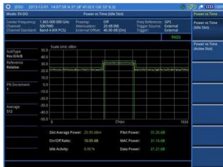
Figure 189 Power vs. time (idle slot) measurement with EV-DO signal analyzer
