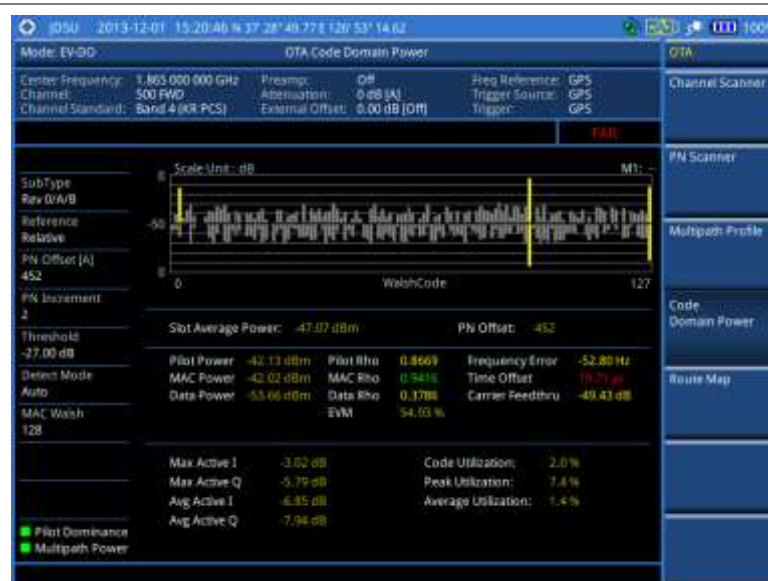
Figure 200 Code domain power measurement with EV-DO OTA signal analyzer
