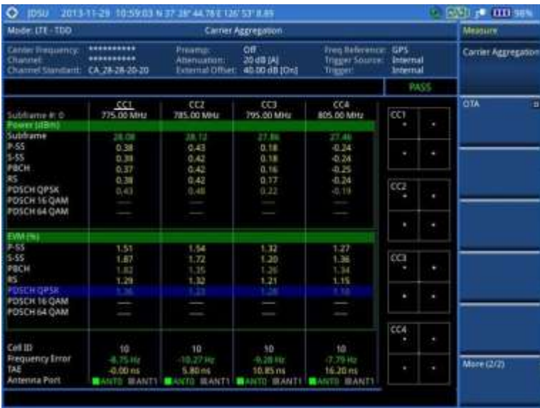
Figure 145 Carrier aggregation measurement with LTE - TDD signal analyzer (SA)
