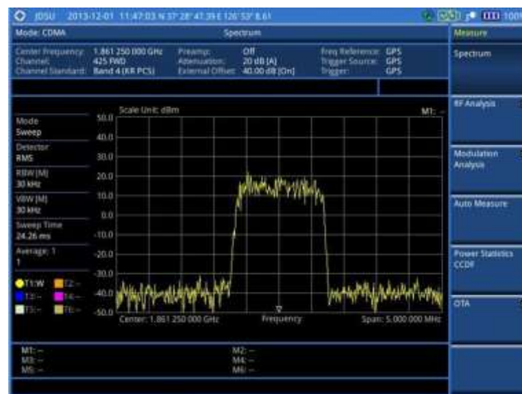
Figure 159 Spectrum measurement screen with CDMA signal analyzer
