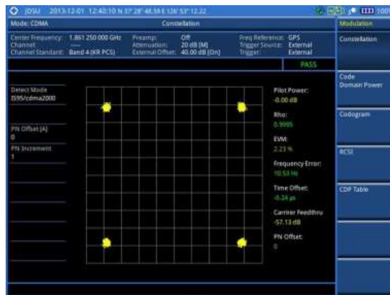
Figure 166 Constellation measurement with CDMA signal analyzer
