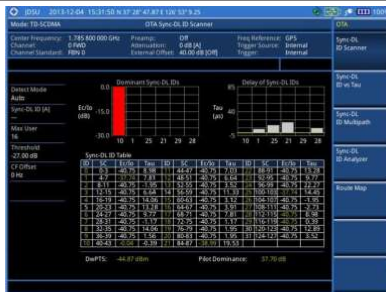
Figure 222 Sync-DL ID scanner measurement with TD-SCDMA OTA signal analyzer
