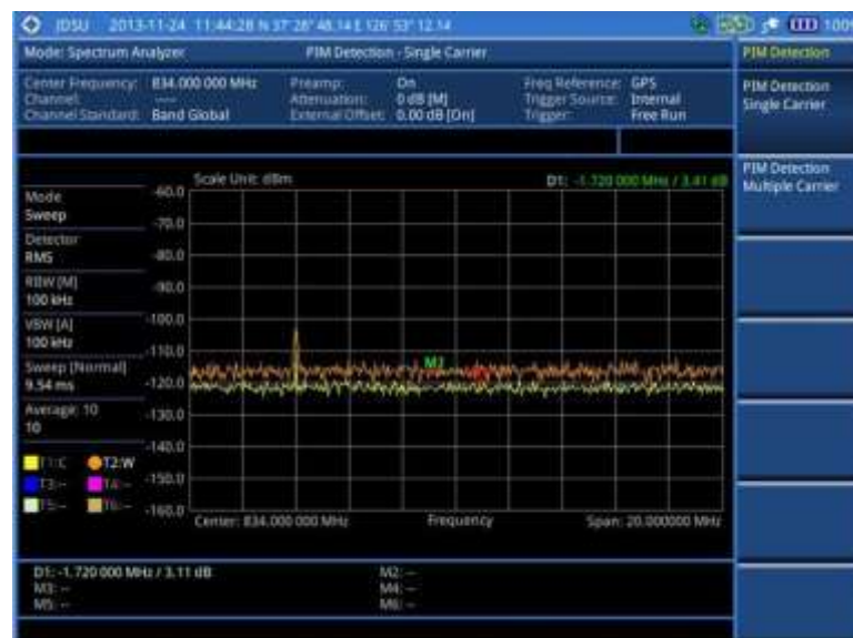
Figure 23 PIM detection for single carrier
