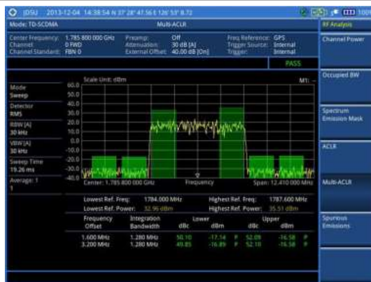
Figure 212 Multi-ACLR measurement with TD-SCDMA signal analyzer
