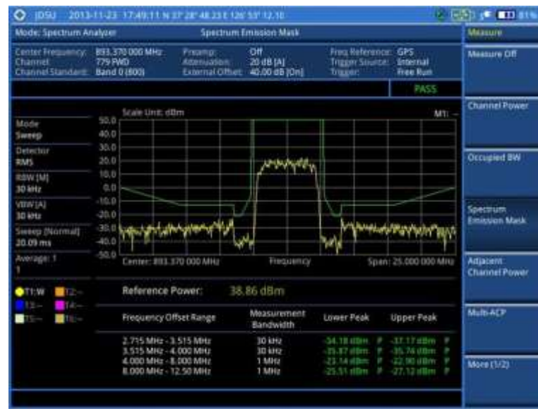
Figure 14 Spectrum emission mask measurement with spectrum analyzer
