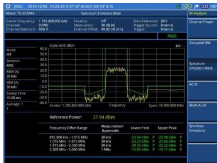
Figure 210 SEM measurement with TD-SCDMA signal analyzer
