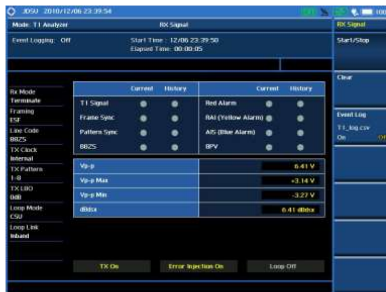
Figure 282 T1 RX signal testing
