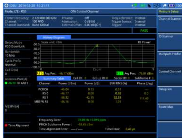
Figure 112 Control channel measurement with LTE - FDD OTA signal analyzer
