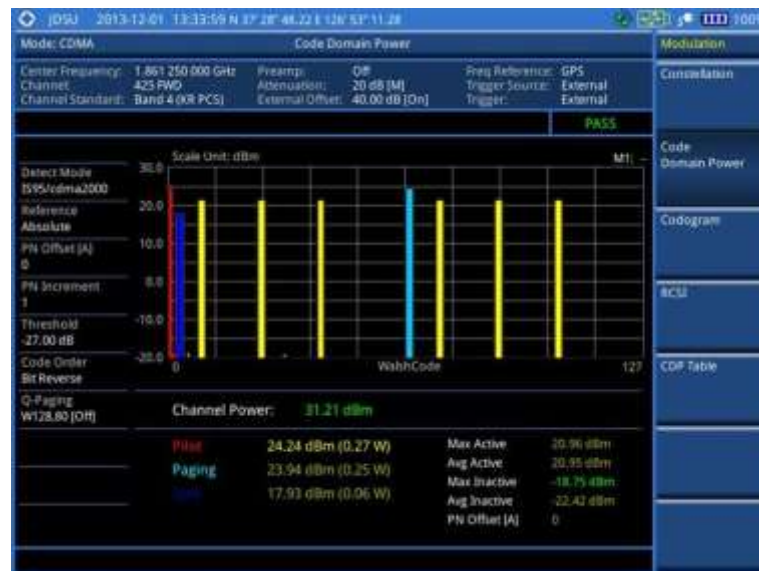
Figure 167 Code domain power measurement with CDMA signal analyzer
