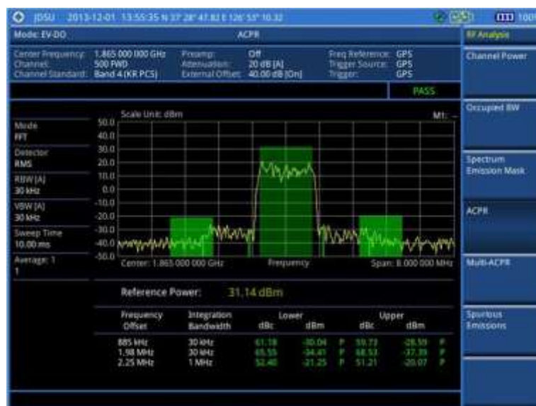
Figure 186 ACPR measurement with EV-DO signal analyzer
