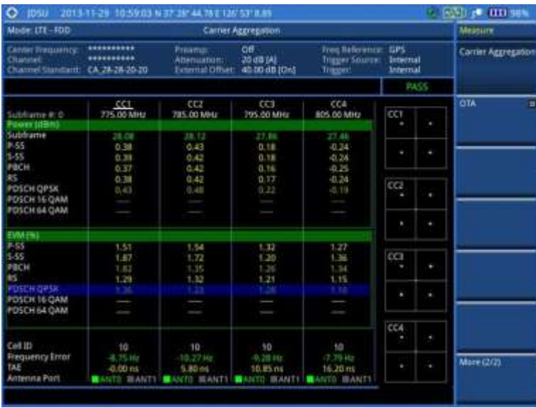
Figure 108 Carrier aggregation measurement with LTE - FDD signal analyzer (SA)
