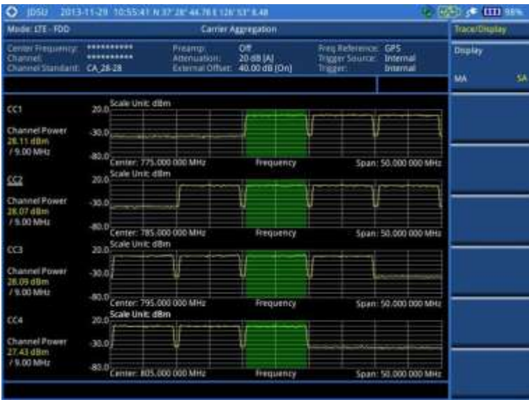
Figure 108 Carrier aggregation measurement with LTE - FDD signal analyzer (SA)
