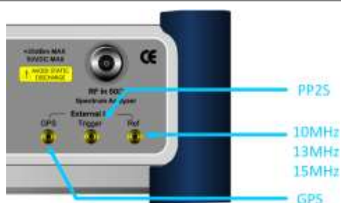
Figure 181 Connection ports for external reference clock
