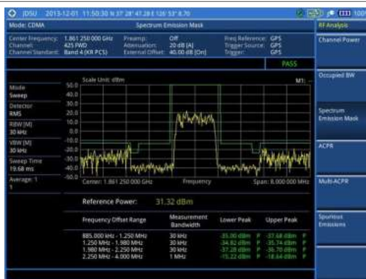
Figure 162 SEM measurement with CDMA signal analyzer
