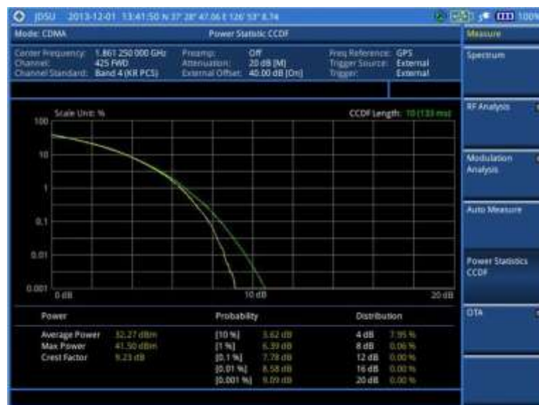
Figure 171 CCDF measurement with CDMA signal analyzer
