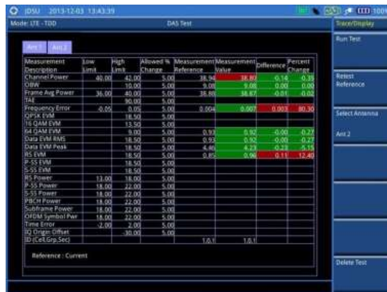
Figure 142 DAS measurement with LTE - TDD signal analyzer
