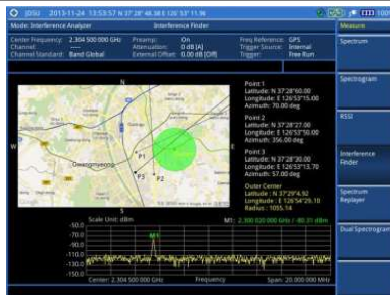
Figure 33 Interference finder measurement in map view
