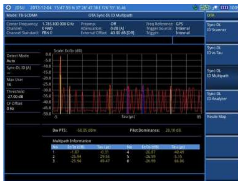
Figure 224 Sync-DL ID multipath measurement with TD-SCDMA OTA signal analyzer
