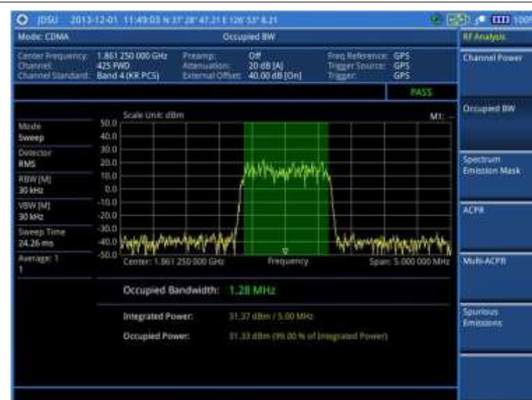
Figure 161 Occupied bandwidth measurement with CDMA signal analyzer
