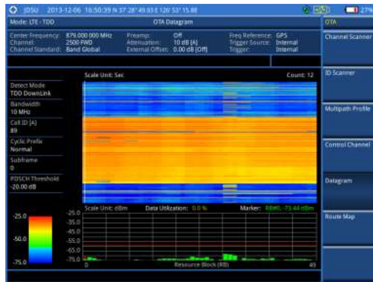
Figure 150 Datagram measurement with LTE - TDD signal analyzer
