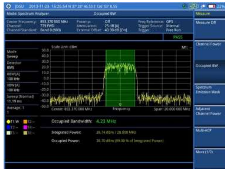
Figure 13 Occupied bandwidth measurement with spectrum analyzer
