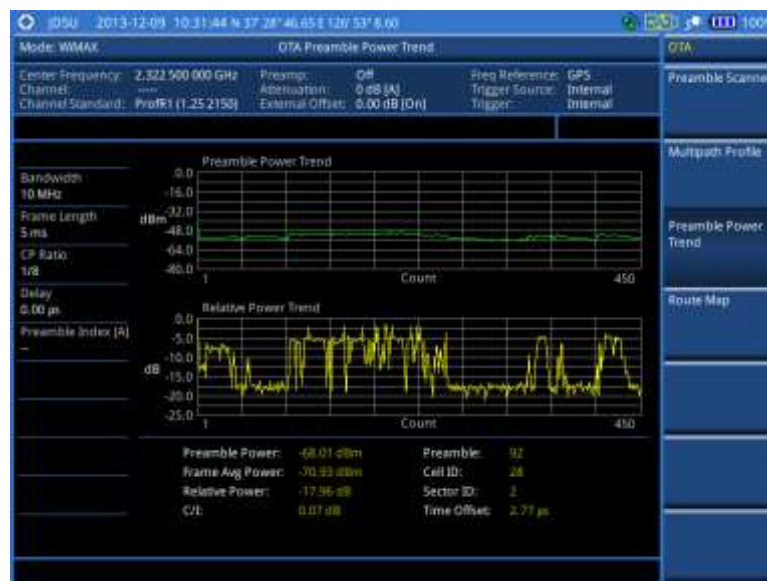
Figure 245 Preamble power trend with Mobile WiMAX OTA signal analyzer
