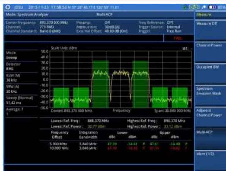
Figure 16 Multi-ACP measurement with spectrum analyzer
