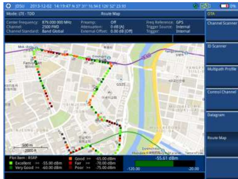
Figure 151 Route map measurement with LTE - TDD OTA signal analyzer
