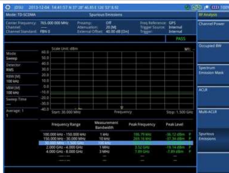
Figure 213 Spurious emissions measurement with TD-SCDMA signal analyzer
