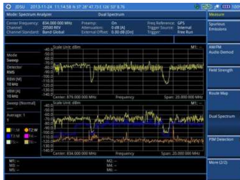
Figure 22 Dual spectrum measurement with spectrum analyzer
