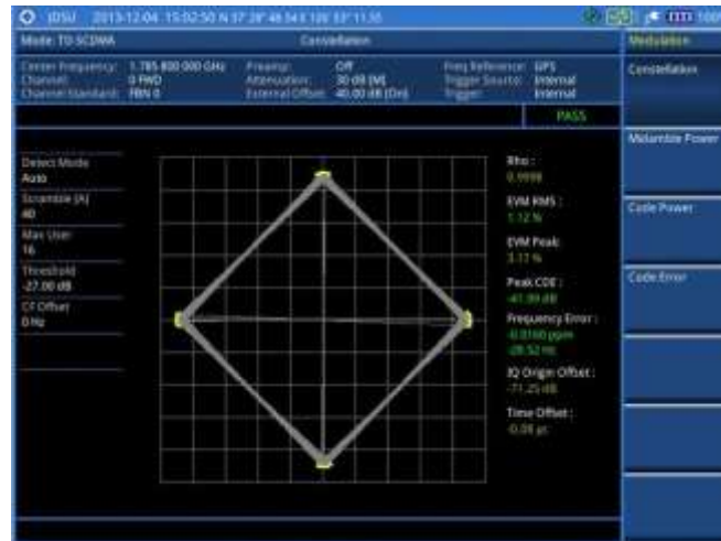
Figure 218 Constellation measurement with TD-SCDMA signal analyzer
