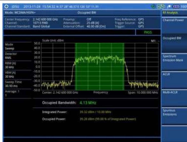
Figure 61 Occupied bandwidth measurement with WCDMA/HSPA+ signal analyzer
