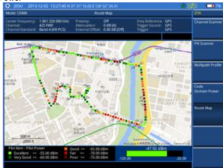
Figure 176 Route map measurement with CDMA OTA signal analyzer
