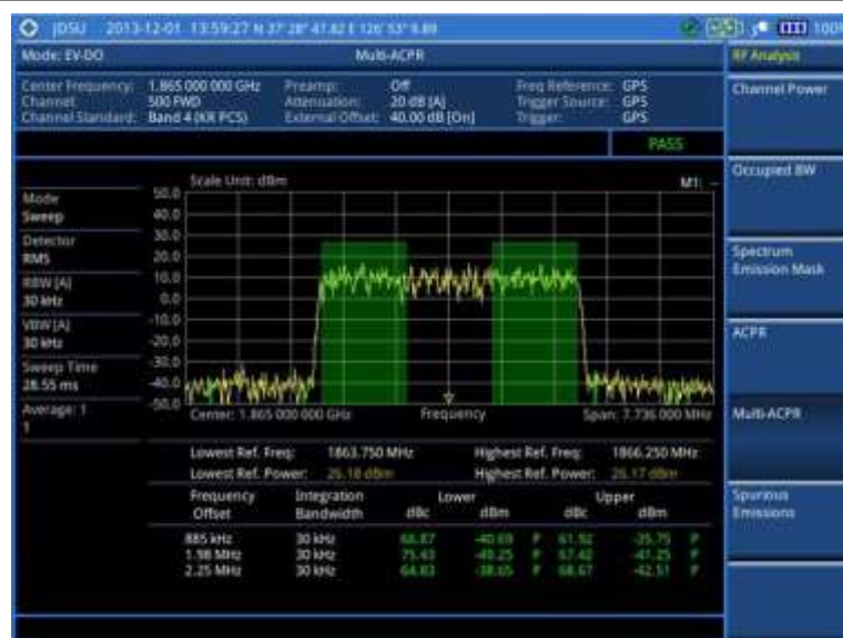
Figure 187 Multi-ACPR measurement with EV-DO signal analyzer
