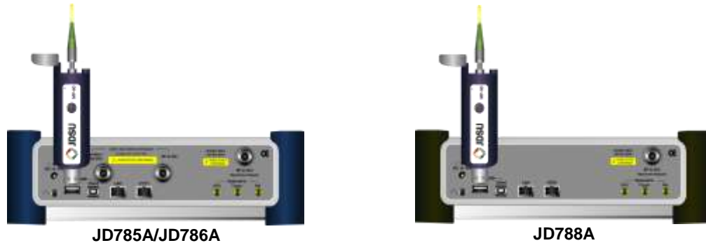
Figure 297 Optical power sensor connection
