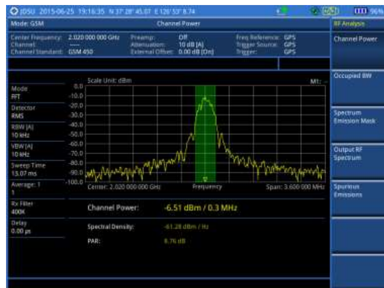
Figure 42 Channel power measurement with GSM signal analyzer
