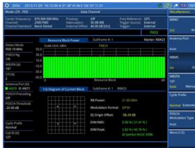
Figure 95 Data channel measurement with LTE - FDD signal analyzer (MBMS On)
