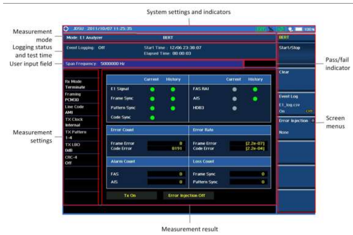
Figure 268 E1 analyzer screen
