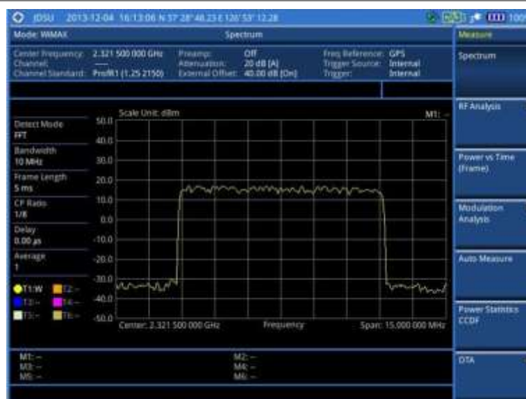
Figure 232 Spectrum measurement screen with Mobile WiMAX signal analyzer
