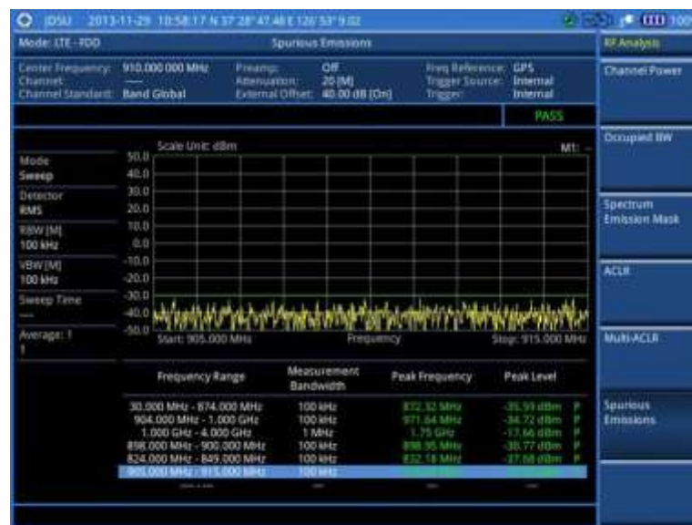
Figure 90 Spurious emissions measurement with LTE - FDD signal analyzer
