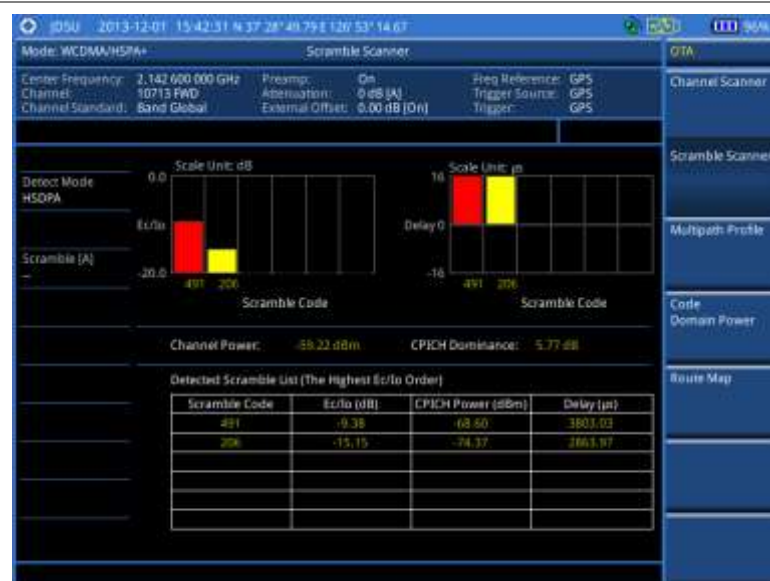
Figure 74 Scramble scanner measurement with WCDMA/HSPA+ OTA signal analyzer
