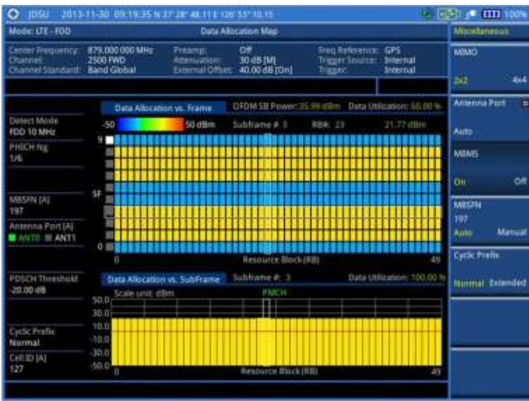
Figure 104 Data allocation map measurement with LTE - FDD signal analyzer (MBMS On)
