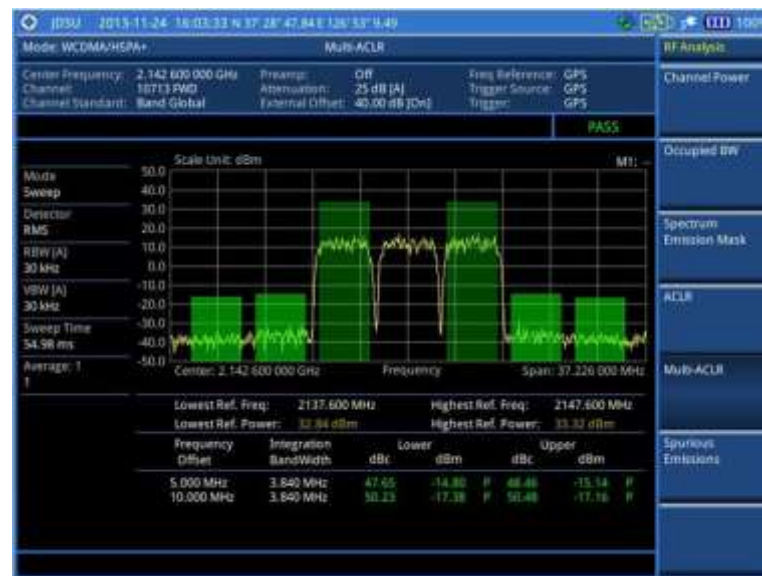
Figure 64 Multi-ACLR measurement with WCDMA/HSPA+ signal analyzer
