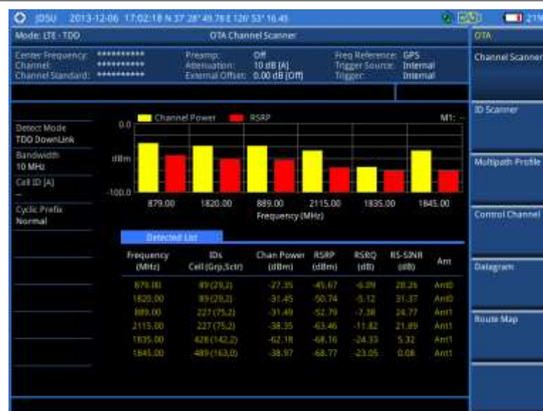
Figure 146 Channel scanner measurement with LTE - TDD OTA signal analyzer
