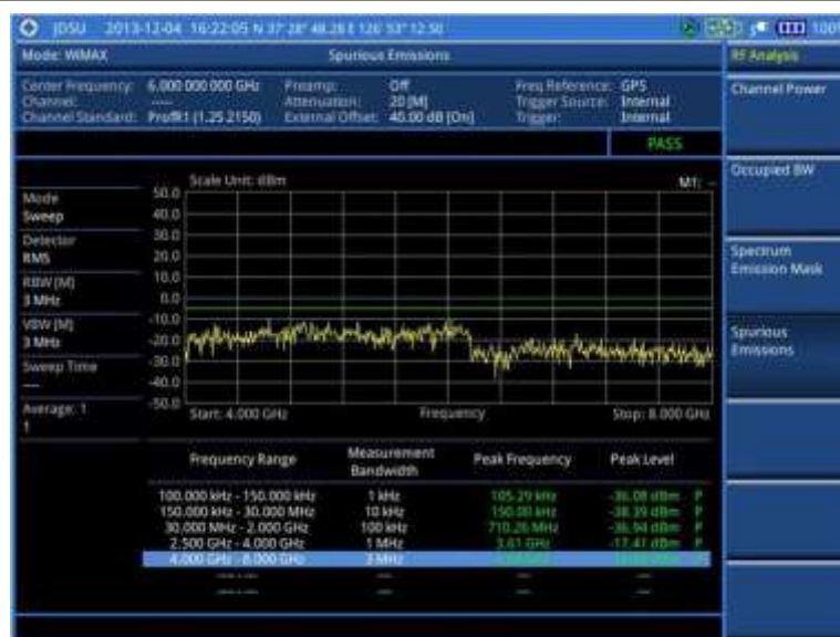
Figure 236 Spurious emissions measurement with Mobile WiMAX signal analyzer
