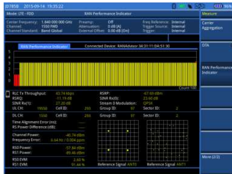
Figure 116 RAN performance indicator in LTE-FDD signal analyzer
