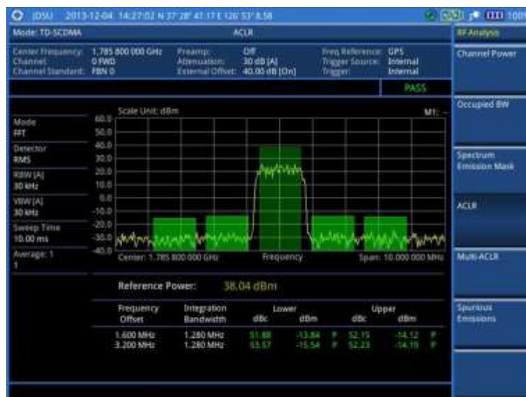
Figure 211 ACLR measurement with TD-SCDMA signal analyzer
