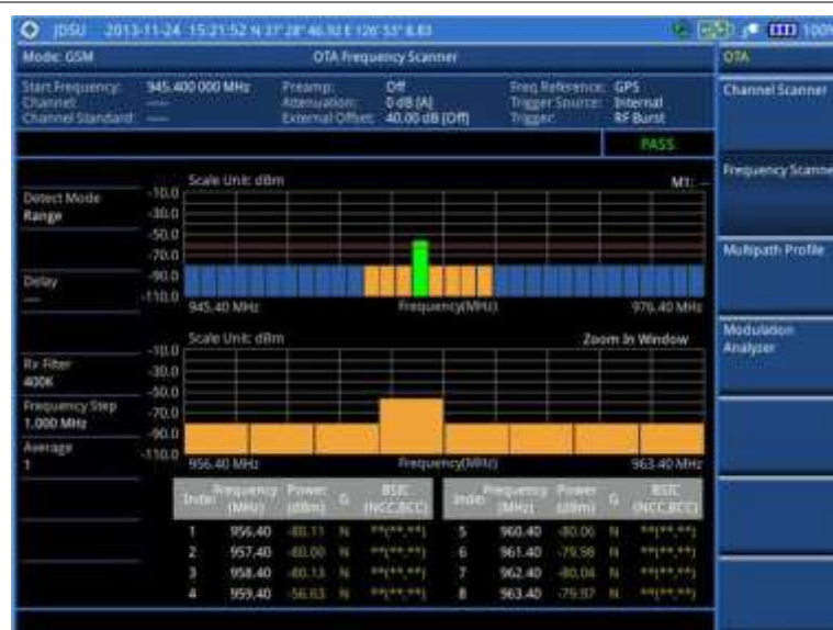
Figure 51 Frequency scanner measurement with GSM OTA signal analyzer
