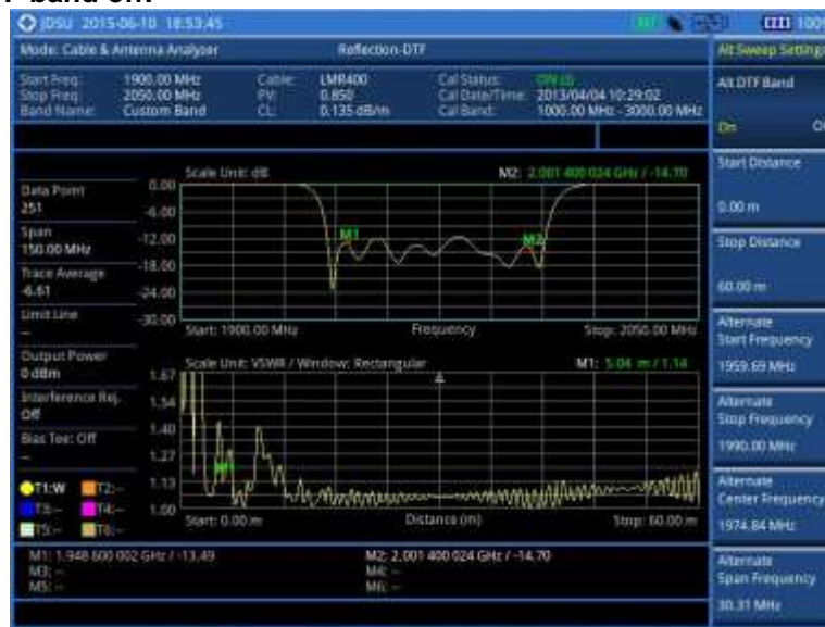
Figure 260 Reflection-DTF dual measurement
