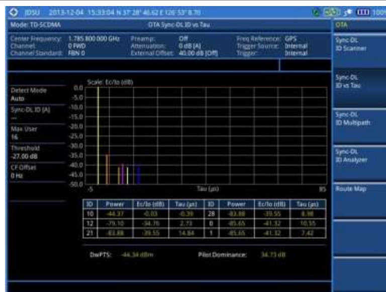
Figure 223 Sync-DL ID vs. Tau measurement with TD-SCDMA OTA signal analyzer
