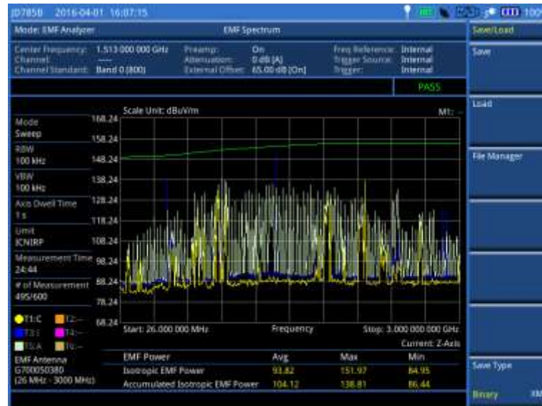
Figure 305 EMF spectrum measurement with EMF analyzer
