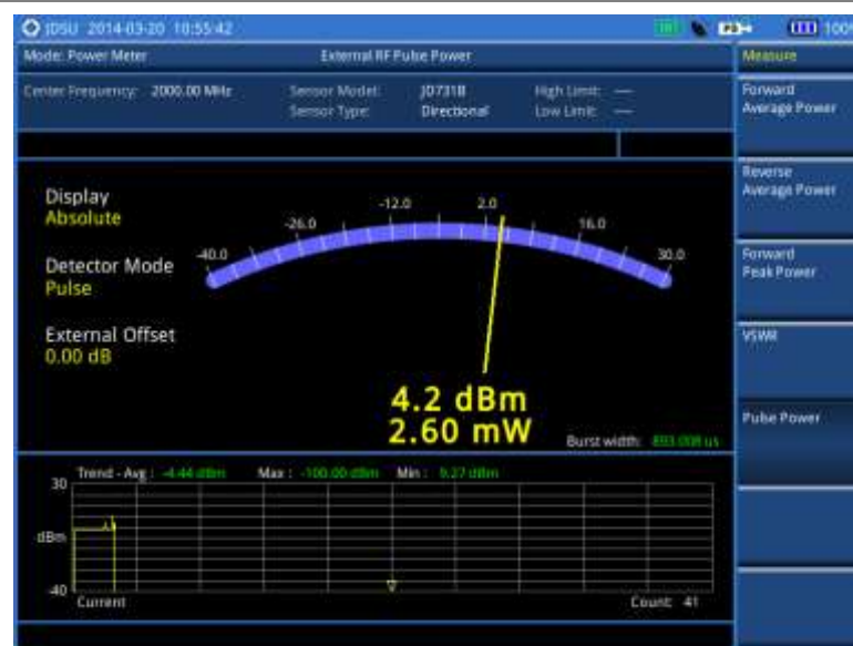
Figure 296 External power measurement of pulse power
