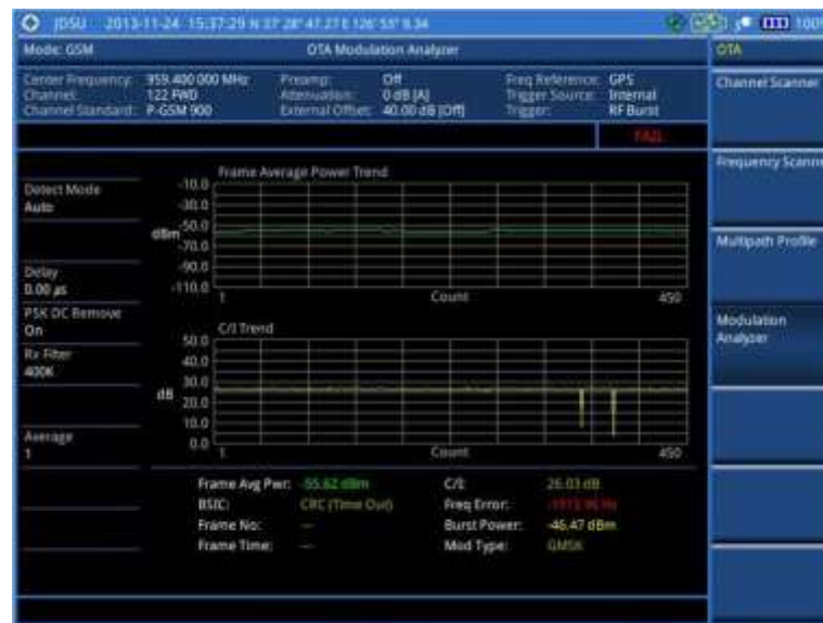
Figure 53 Modulation analyzer measurement with GSM OTA signal analyzer
