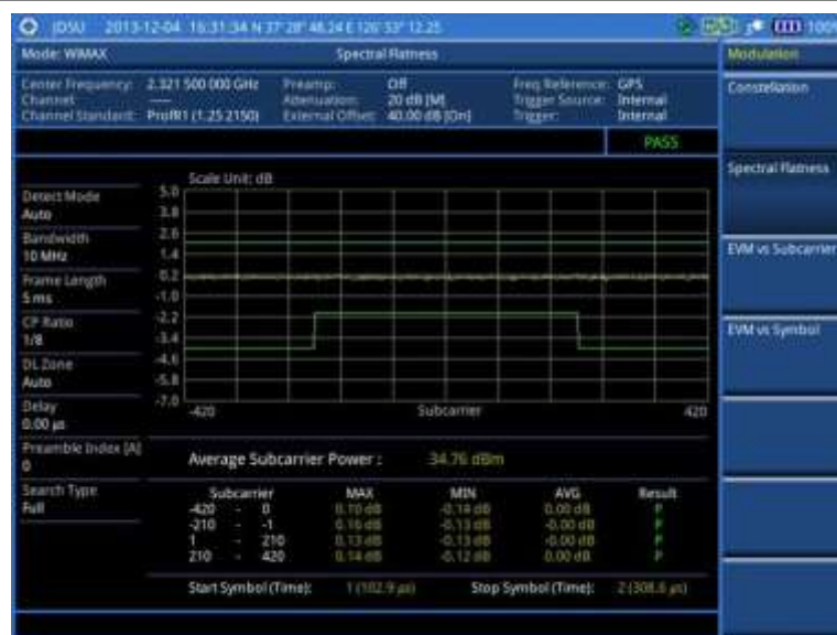
Figure 239 Spectral flatness measurement with Mobile WiMAX signal analyzer
