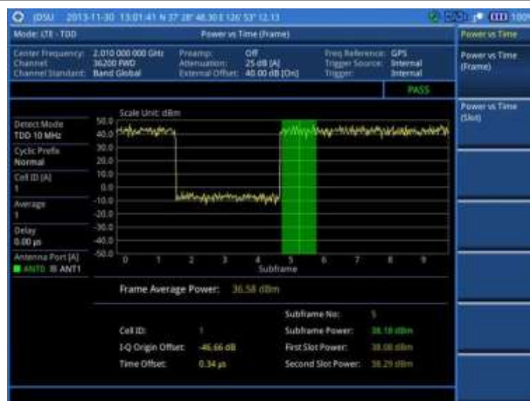
Figure 130 Power vs. time (frame) measurement with LTE – TDD signal analyzer
