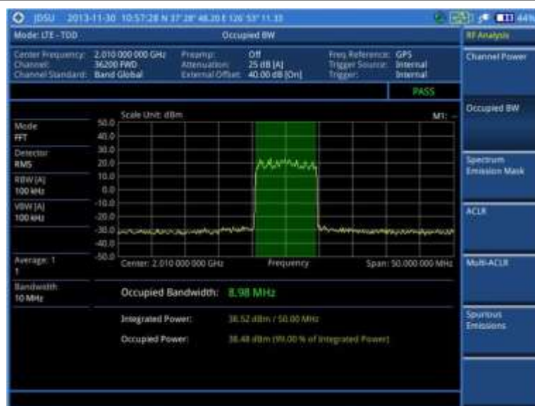
Figure 124 Occupied bandwidth measurement with LTE - TDD signal analyzer
