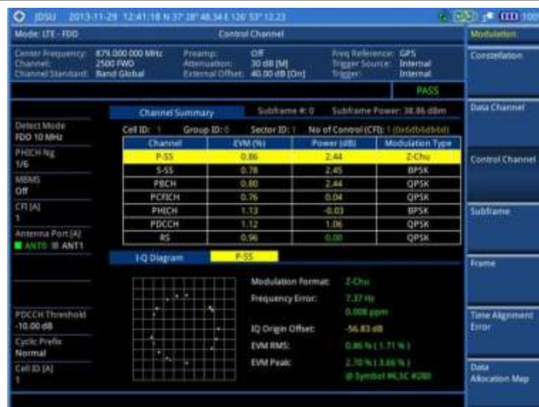
Figure 97 Control channel measurement with LTE - FDD signal analyzer (MBMS On)
