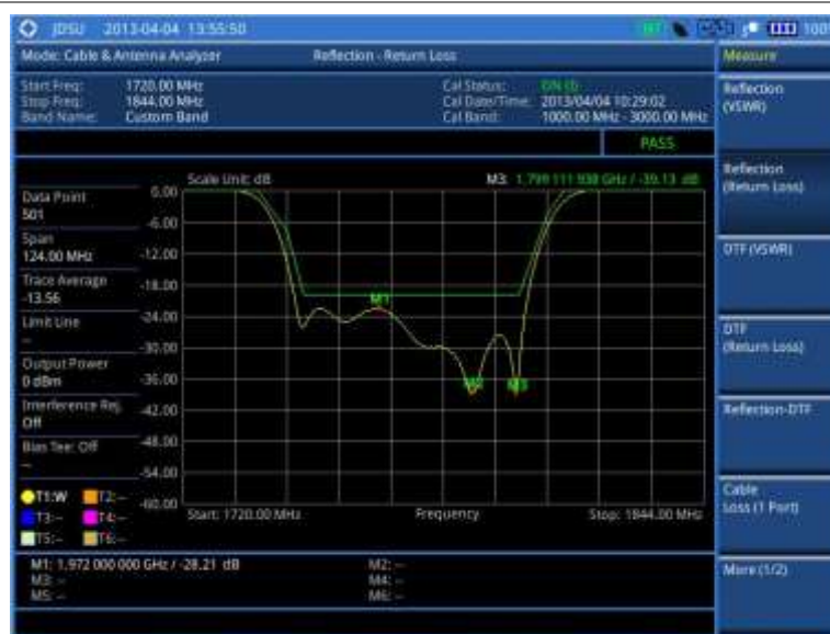
Figure 257 Reflection measurement in return loss scale
