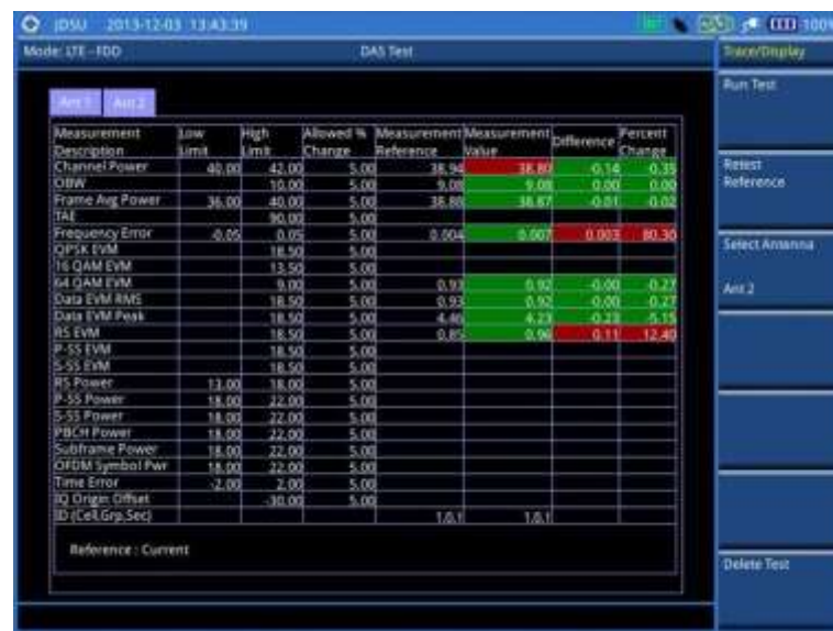
Figure 105 DAS measurement with LTE - FDD signal analyzer
