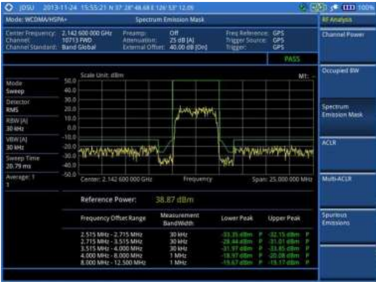
Figure 62 SEM measurement with WCDMA/HSPA+ signal analyzer
