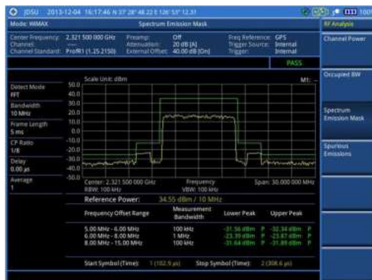
Figure 235 SEM measurement with Mobile WiMAX signal analyzer
