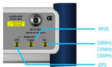
Figure 121 Connection ports for external reference clock
