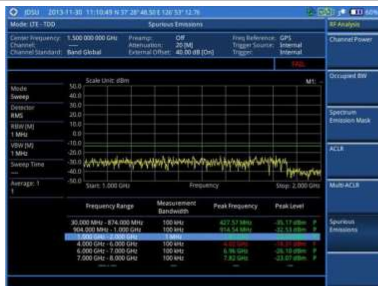
Figure 128 Spurious emissions measurement with LTE - TDD signal analyzer
