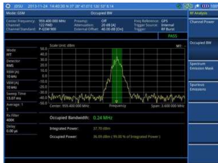
Figure 43 Occupied bandwidth measurement with GSM signal analyzer
