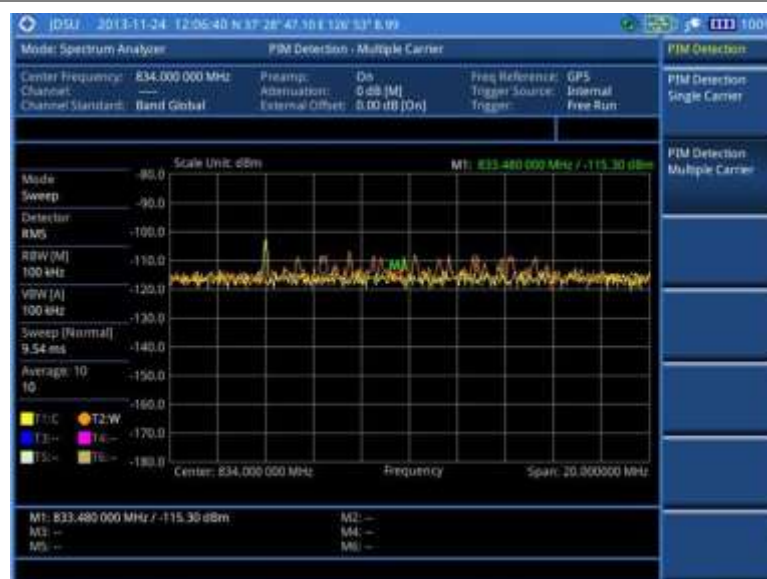
Figure 24 PIM detection for multiple carriers
