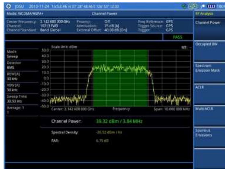
Figure 60 Channel power measurement with WCDMA/HSPA+ signal analyzer
