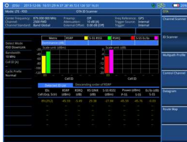
Figure 110 ID scanner measurement with LTE - FDD OTA signal analyzer
