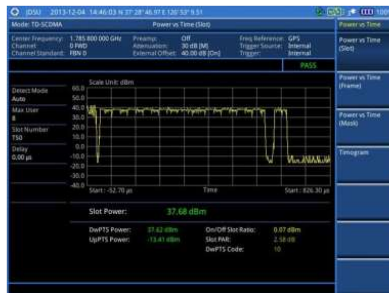
Figure 214 Power vs. time (slot) measurement with TD-SCDMA signal analyzer
