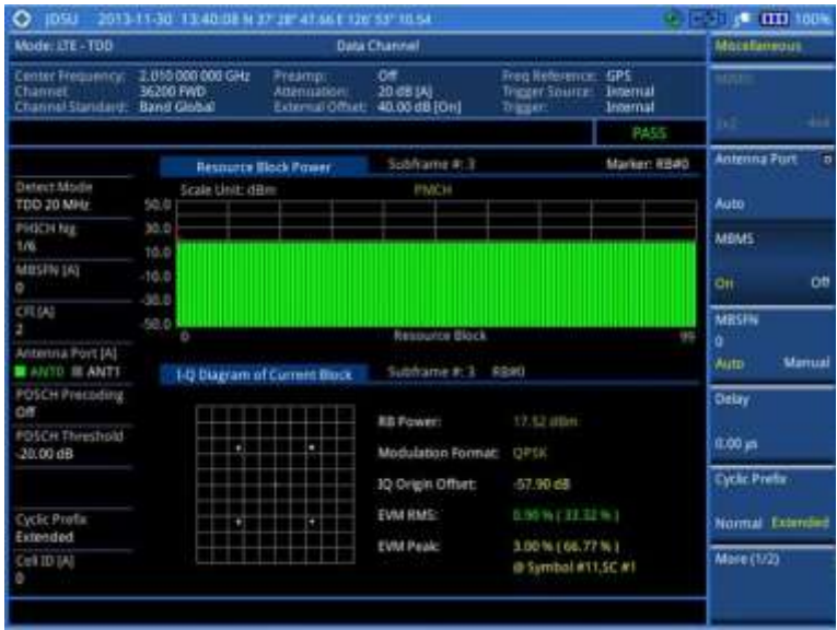
Figure 134 Data channel measurement with LTE - TDD signal analyzer (MBMS On)
