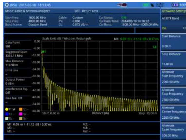
Figure 259 DTF measurement with the alternate DTF band on
