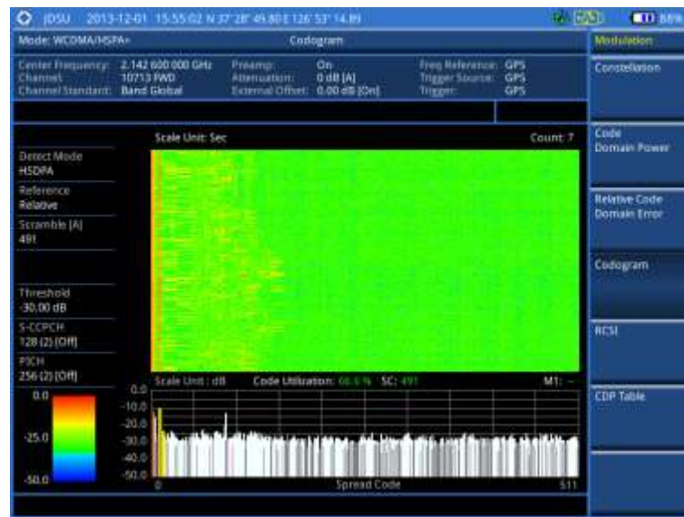
Figure 69 Codogram in full view with WCDMA/HSPA+ signal analyzer
