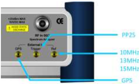
Figure 158 Connection ports for external reference clock
