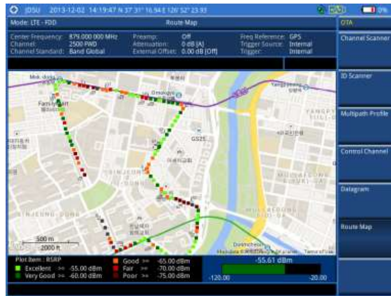
Figure 114 Route map measurement with LTE - FDD OTA signal analyzer
