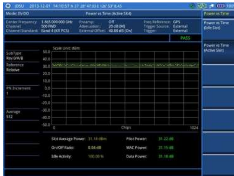
Figure 190 Power vs. time (active slot) measurement with EV-DO signal analyzer
