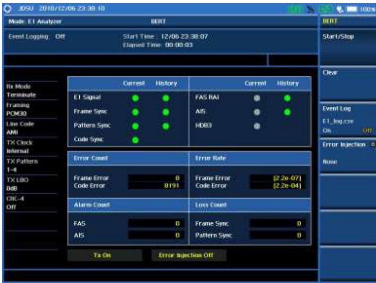
Figure 274 E1 BERT testing for framing PCM30
