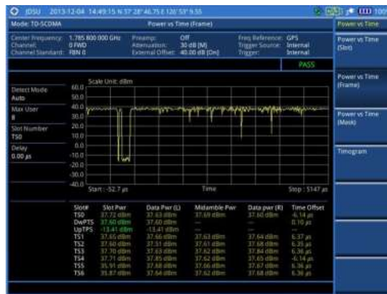
Figure 215 Power vs. time (frame) measurement with TD-SCDMA signal analyzer
