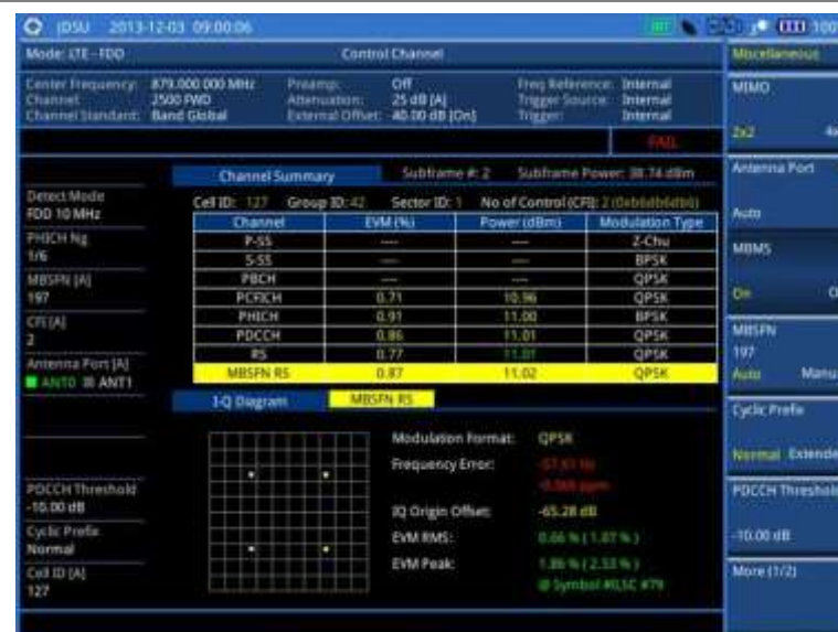
Figure 97 Control channel measurement with LTE - FDD signal analyzer (MBMS On)
