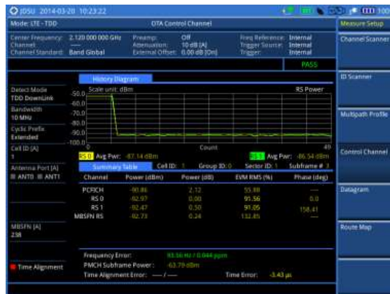
Figure 149 Control channel measurement with LTE - TDD OTA signal analyzer
