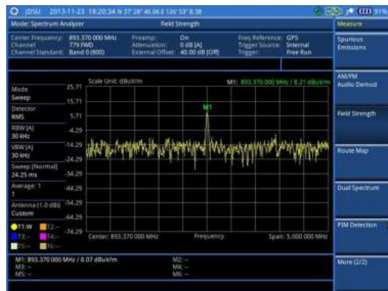
Figure 19 Field strength measurement with spectrum analyzer
