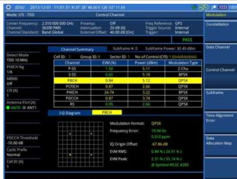
Figure 136 Control channel measurement with LTE - TDD signal analyzer (MBMS On)
