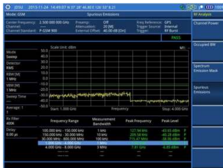
Figure 46 Spurious emissions measurement with GSM signal analyzer
