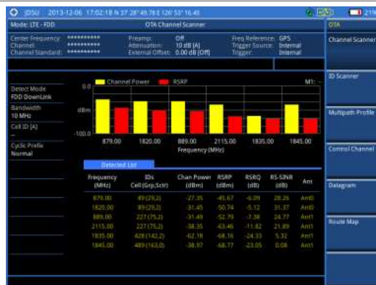
Figure 109 Channel scanner measurement with LTE - FDD OTA signal analyzer
