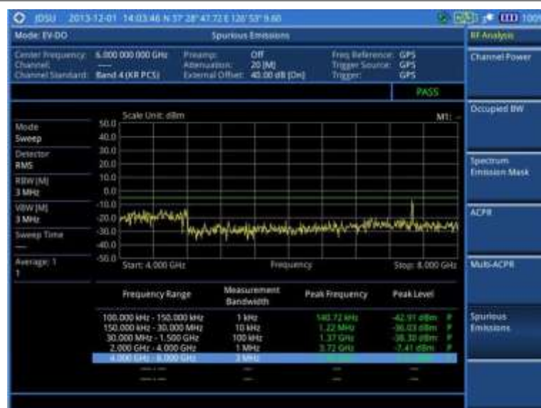
Figure 188 Spurious emissions measurement with EV-DO signal analyzer
