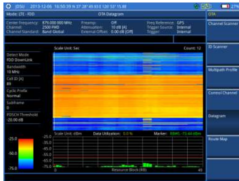
Figure 113 Datagram measurement with LTE - FDD signal analyzer
