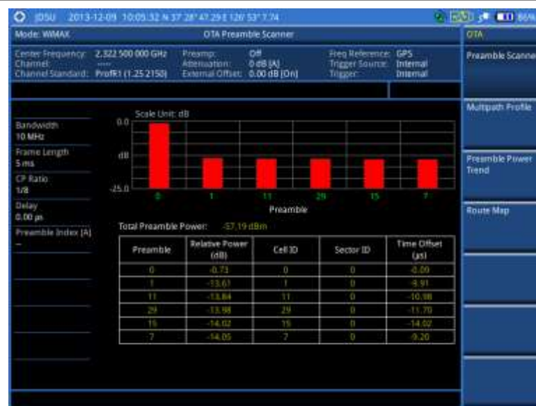
Figure 243 Preamble scanner measurement with Mobile WiMAX OTA signal analyzer
