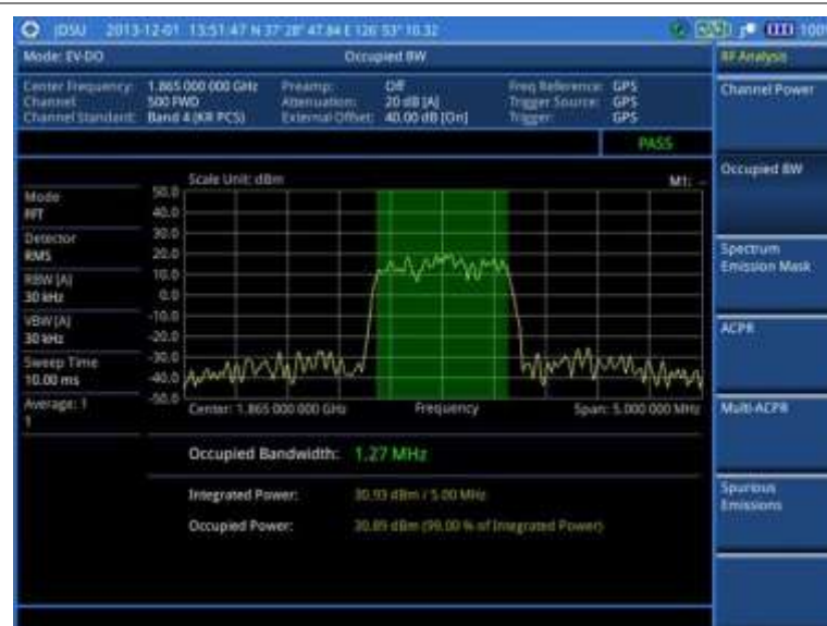
Figure 184 Occupied bandwidth measurement with EV-DO signal analyzer
