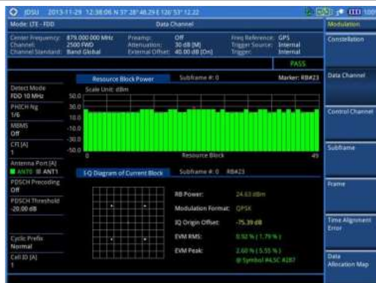
Figure 94 Data channel measurement with LTE - FDD signal analyzer
