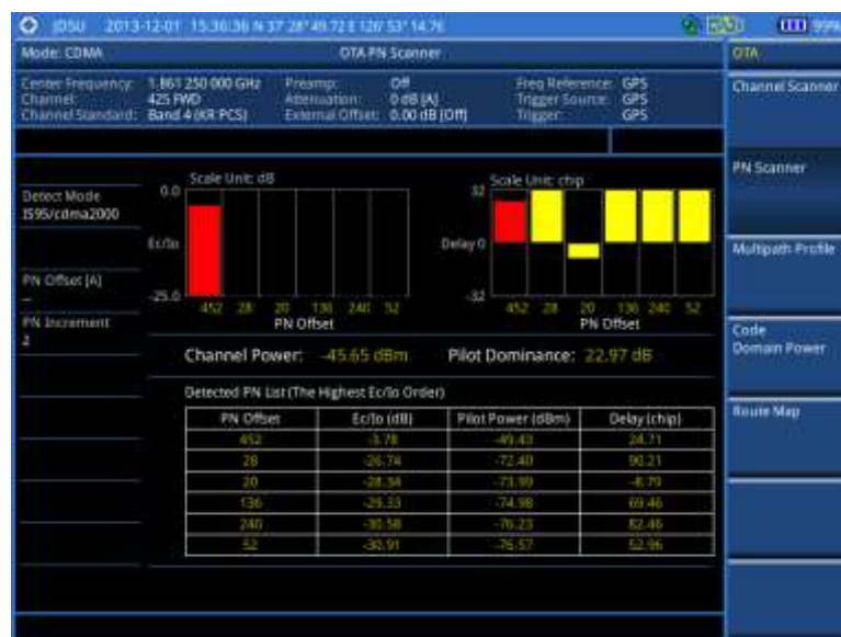
Figure 173 PN scanner measurement with CDMA OTA signal analyzer
