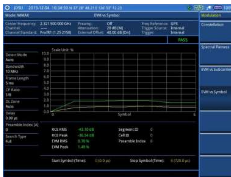
Figure 241 EVM vs. symbol measurement with Mobile WiMAX signal analyzer
