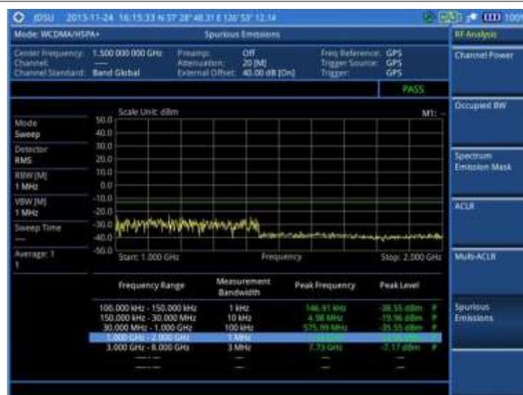
Figure 65 Spurious emissions measurement with WCDMA/HSPA+ signal analyzer
