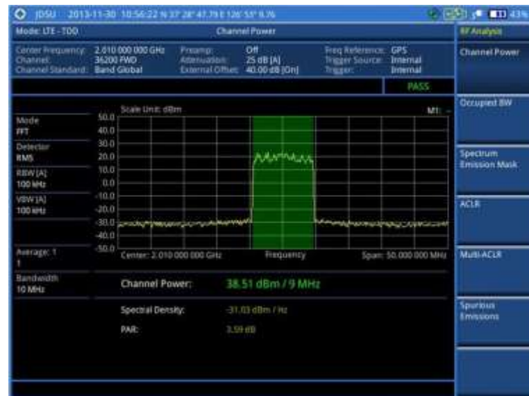
Figure 123 Channel power measurement with LTE - TDD signal analyzer
