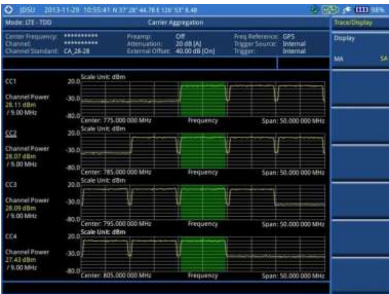
Figure 145 Carrier aggregation measurement with LTE - TDD signal analyzer (SA)
