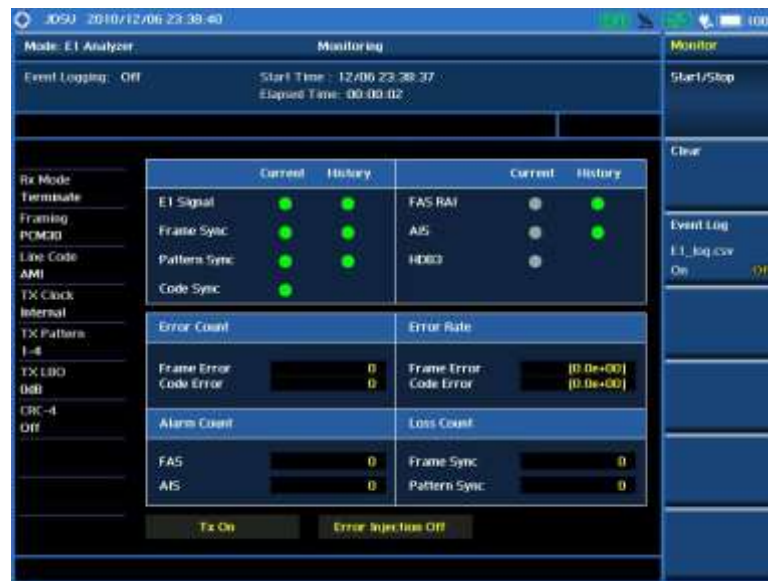
Figure 273 E1 transmission monitoring for framing PCM30
