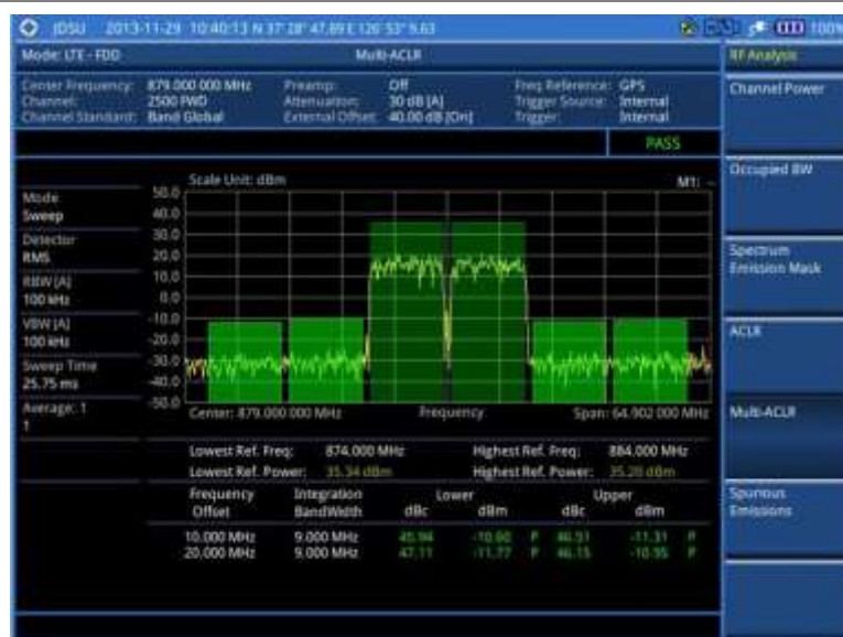
Figure 89 Multi-ACLR measurement with LTE - FDD signal analyzer
