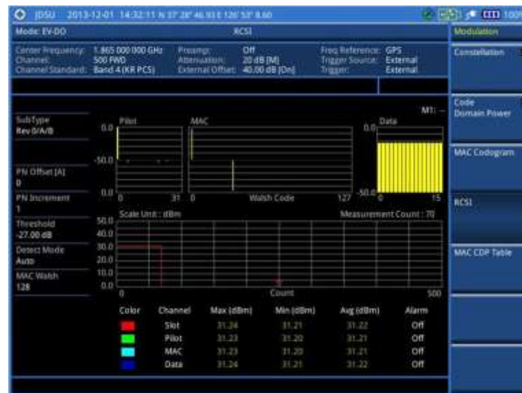
Figure 194 RCSI measurement with EV-DO signal analyzer
