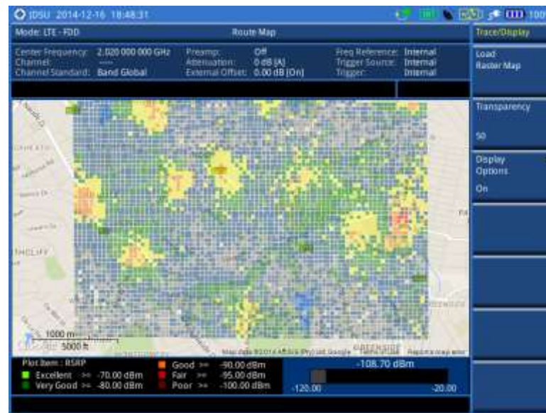
Figure 115 Raster image overlaid on the route map in LTE-FDD OTA signal analyzer
