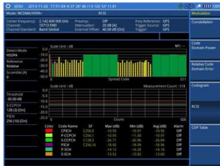
Figure 70 RCSI measurement with WCDMA/HSPA+ signal analyzer
