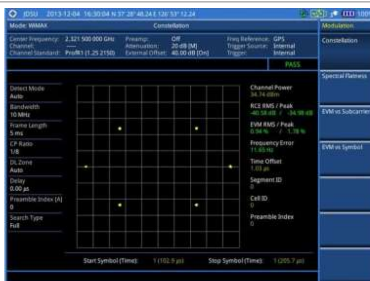
Figure 238 Constellation measurement with Mobile WiMAX signal analyzer
