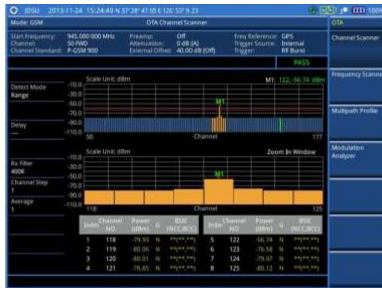
Figure 50 Channel scanner measurement with GSM OTA signal analyzer
