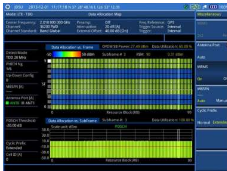
Figure 141 Data allocation map measurement with LTE - TDD signal analyzer (MBMS On)
