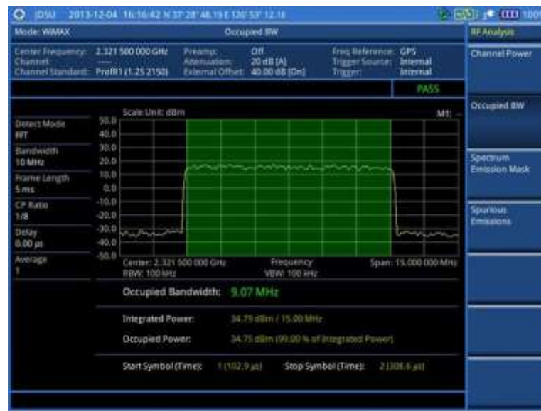
Figure 234 Occupied bandwidth measurement with Mobile WiMAX signal analyzer
