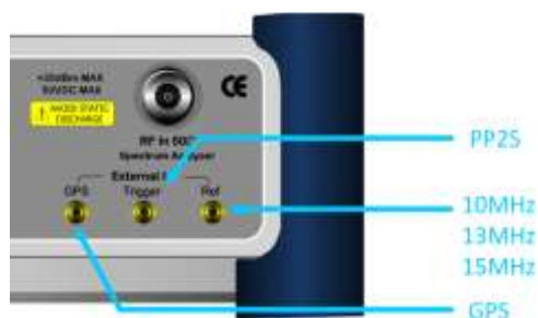
Figure 58 Connection ports for external reference clock
