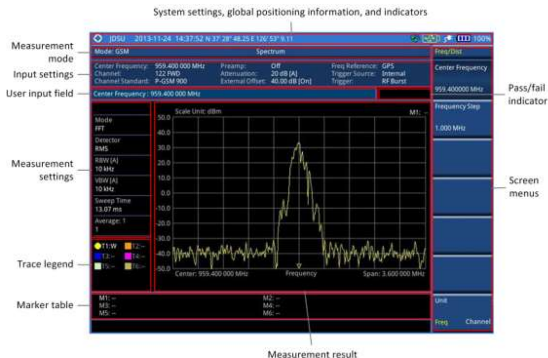
Figure 37 GSM signal analyzer measurement screen
