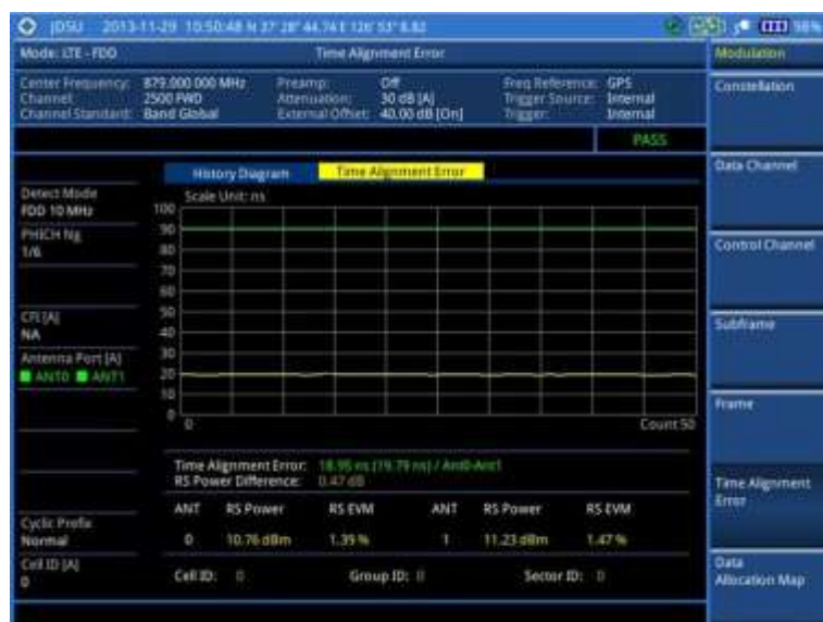
Figure 102 Time alignment error measurement with LTE - FDD signal analyzer
