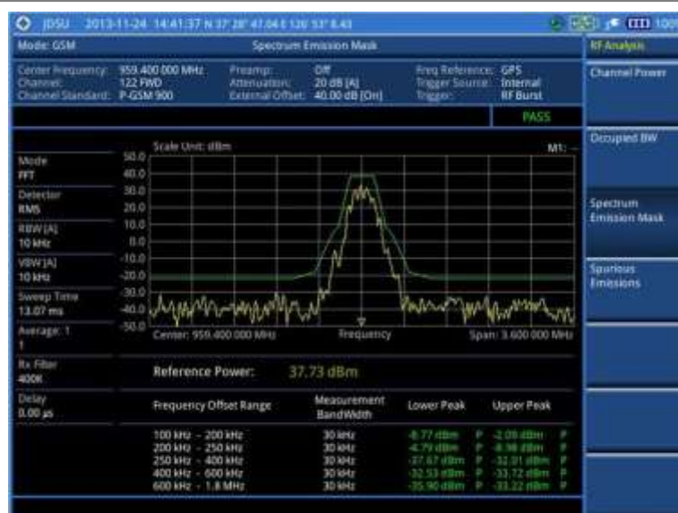
Figure 44 SEM measurement with GSM signal analyzer
