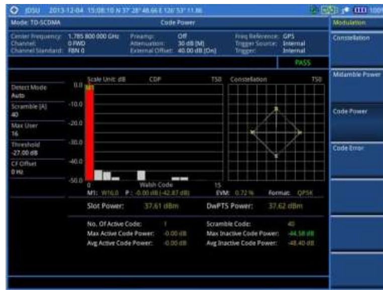
Figure 220 Code power measurement with TD-SCDMA signal analyzer
