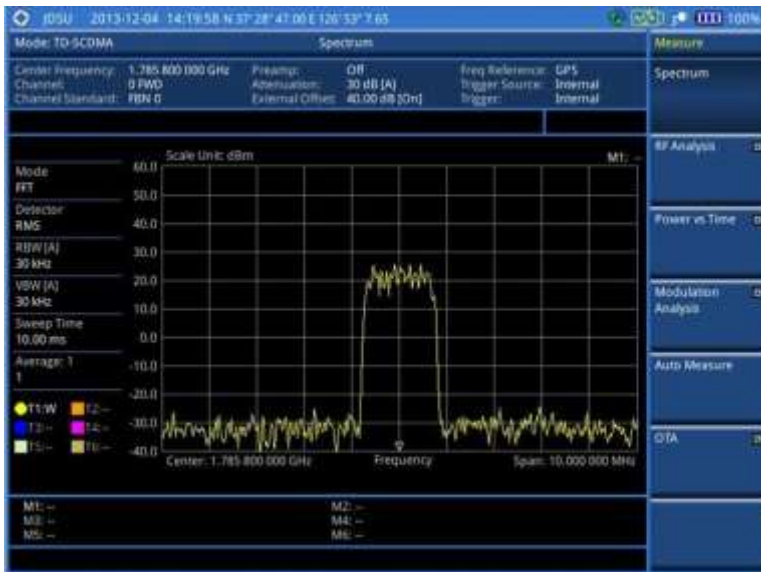
Figure 207 Spectrum measurement screen with TD-SCDMA signal analyzer
