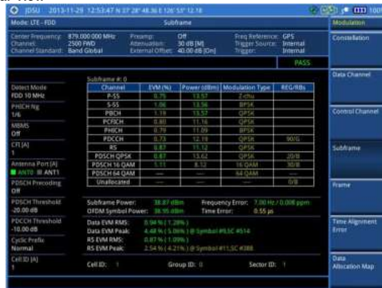
Figure 98 Subframe measurement with LTE - FDD signal analyzer
