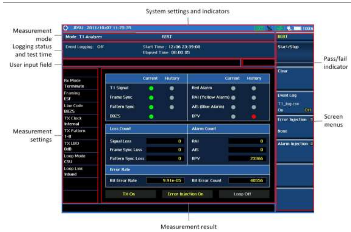
Figure 275 T1 analyzer screen
