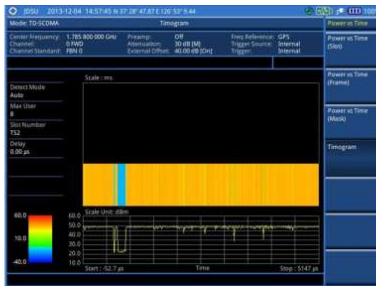
Figure 217 Timogram with TD-SCDMA signal analyzer
