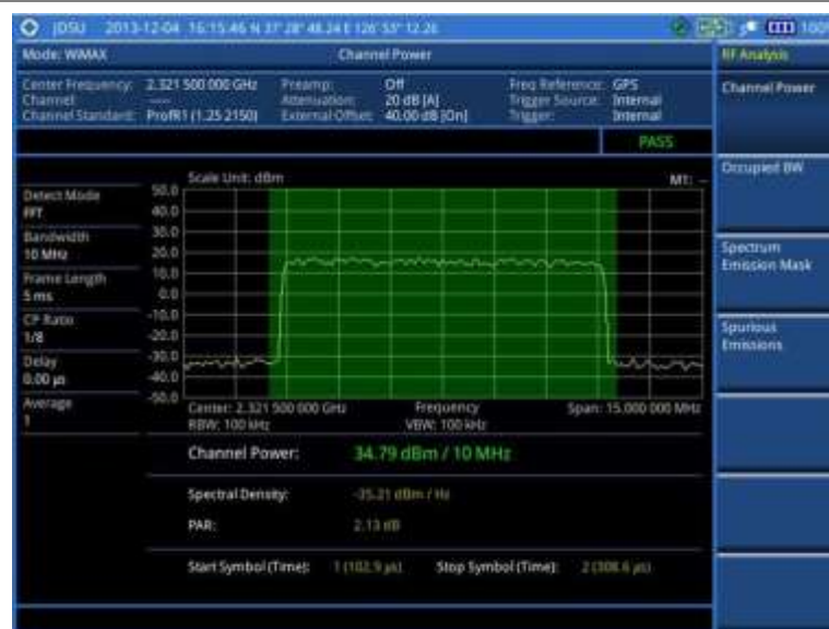
Figure 233 Channel power measurement with Mobile WiMAX signal analyzer
