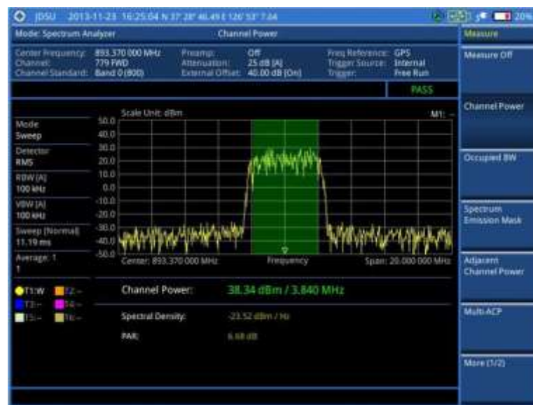
Figure 12 Channel power measurement with spectrum analyzer
