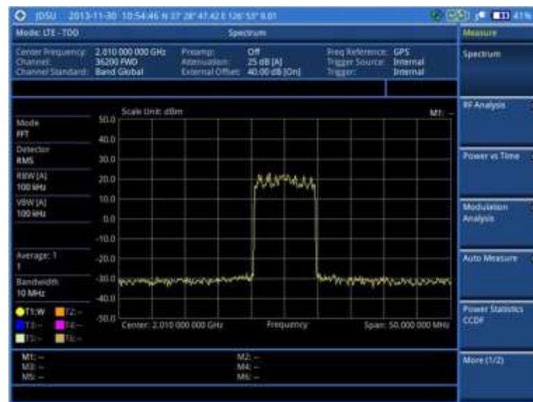
Figure 122 Spectrum measurement screen with LTE - TDD signal analyzer
