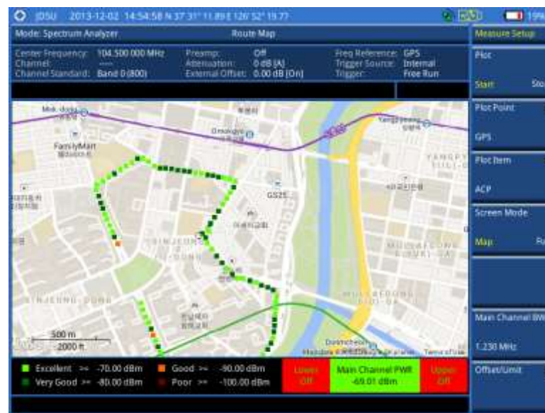
Figure 20 Route map measurement screen with GPS
