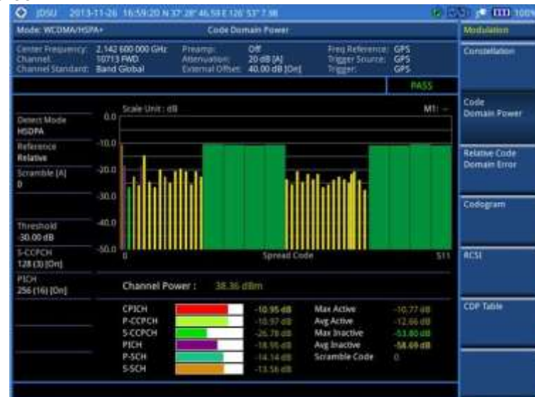
Figure 67 Code domain power measurement with WCDMA/HSPA+ signal analyzer
