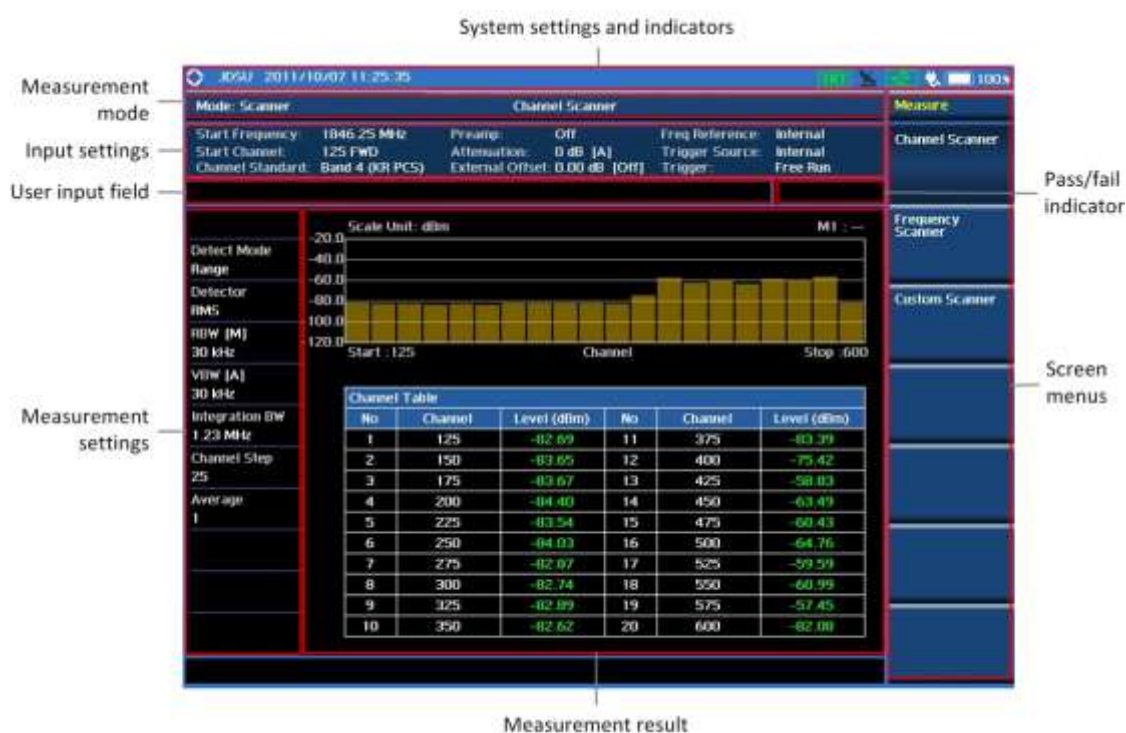
Figure 284 Channel scanner screen
