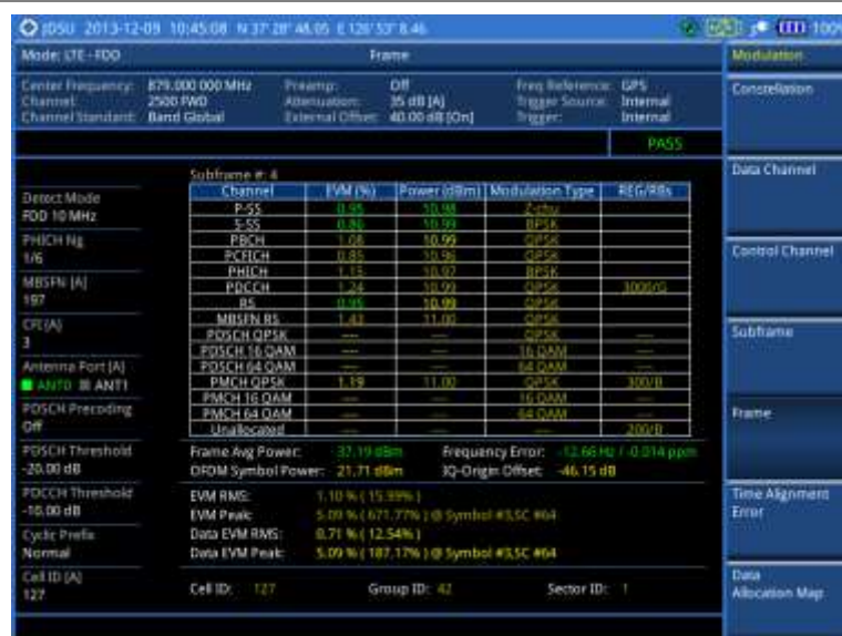
Figure 101 Frame measurement with LTE - FDD signal analyzer (MBMS On)
