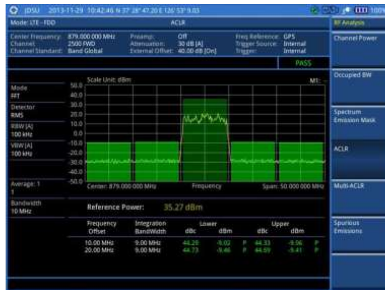
Figure 88 ACLR measurement with LTE - FDD signal analyzer
