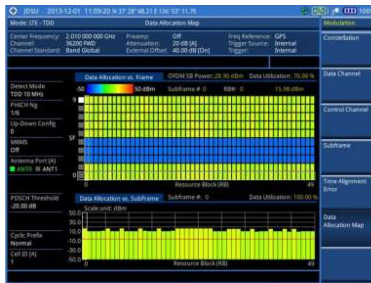
Figure 141 Data allocation map measurement with LTE - TDD signal analyzer (MBMS On)
