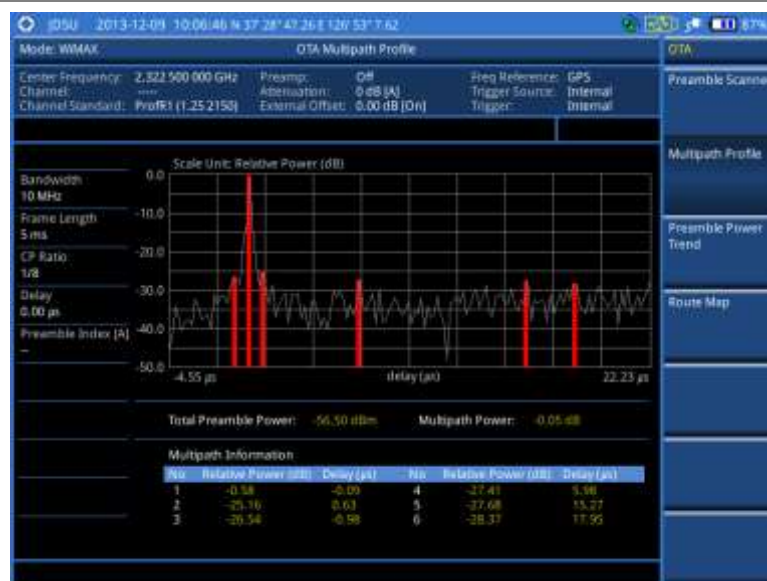
Figure 244 Multipath profile measurement with Mobile WiMAX OTA signal analyzer
