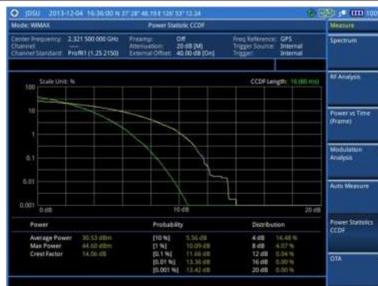
Figure 242 CCDF measurement with Mobile WiMAX signal analyzer
