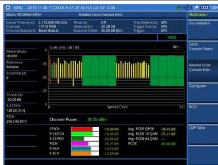
Figure 68 Relative code domain error with WCDMA/HSPA+ signal analyzer
