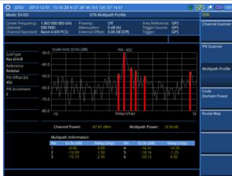
Figure 199 Multipath profile measurement with EV-DO OTA signal analyzer
