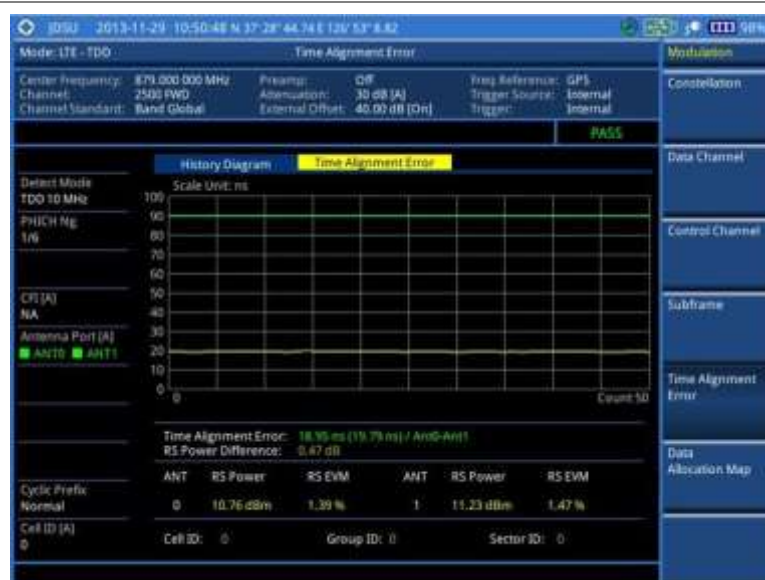
Figure 139 Time alignment error measurement with LTE - TDD signal analyzer
