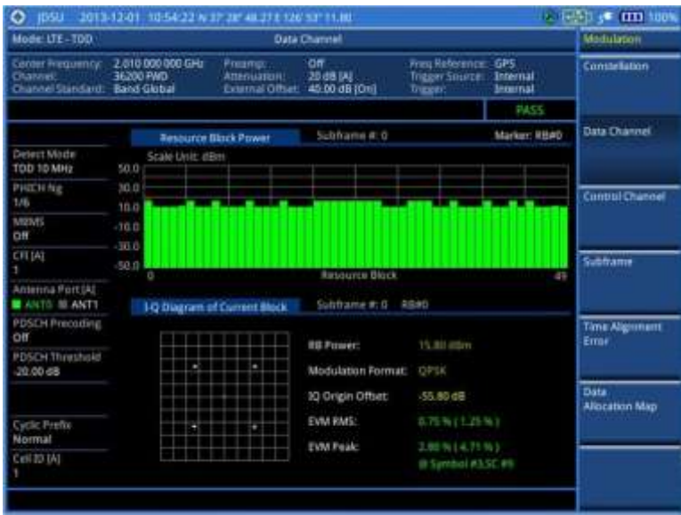
Figure 134 Data channel measurement with LTE - TDD signal analyzer (MBMS On)
