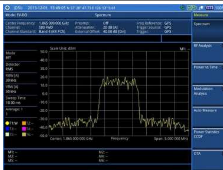
Figure 182 Spectrum measurement screen with EV-DO signal analyzer
