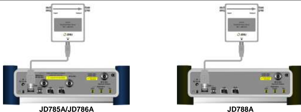
Figure 295 Directional power sensor connection
