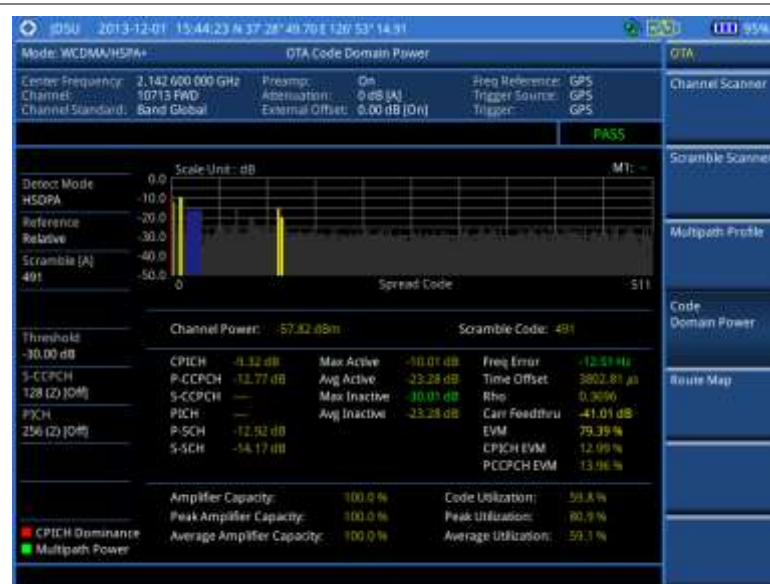
Figure 76 Code domain power measurement with WCDMA/HSPA+ OTA signal analyzer
