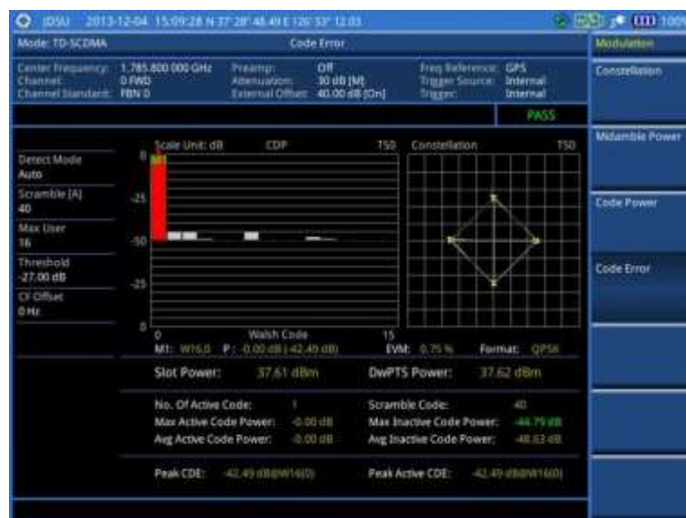
Figure 221 Code error measurement with TD-SCDMA signal analyzer
