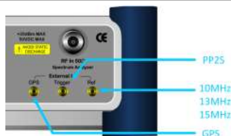
Figure 231 Connection ports for external reference clock
