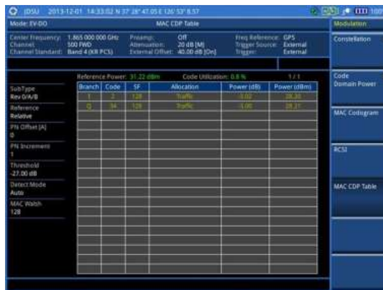
Figure 195 MAC CDP Table measurement with EV-DO signal analyzer
