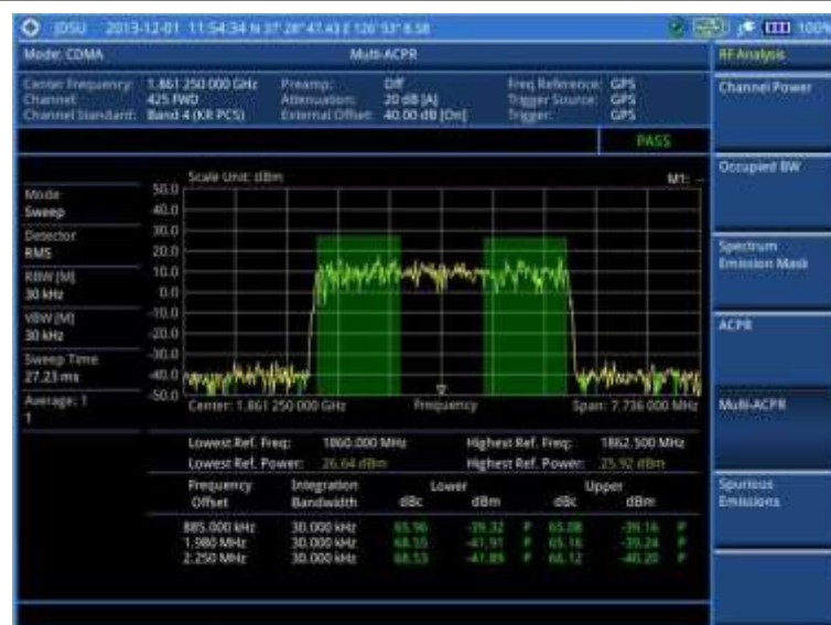
Figure 164 Multi-ACPR measurement with CDMA signal analyzer
