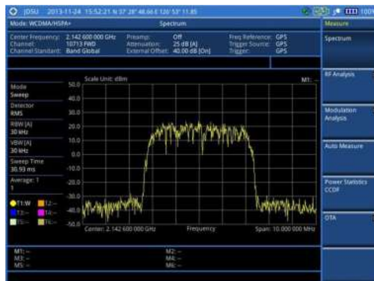
Figure 59 Spectrum measurement screen with WCDMA signal analyzer
