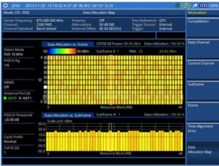
Figure 104 Data allocation map measurement with LTE - FDD signal analyzer (MBMS On)
