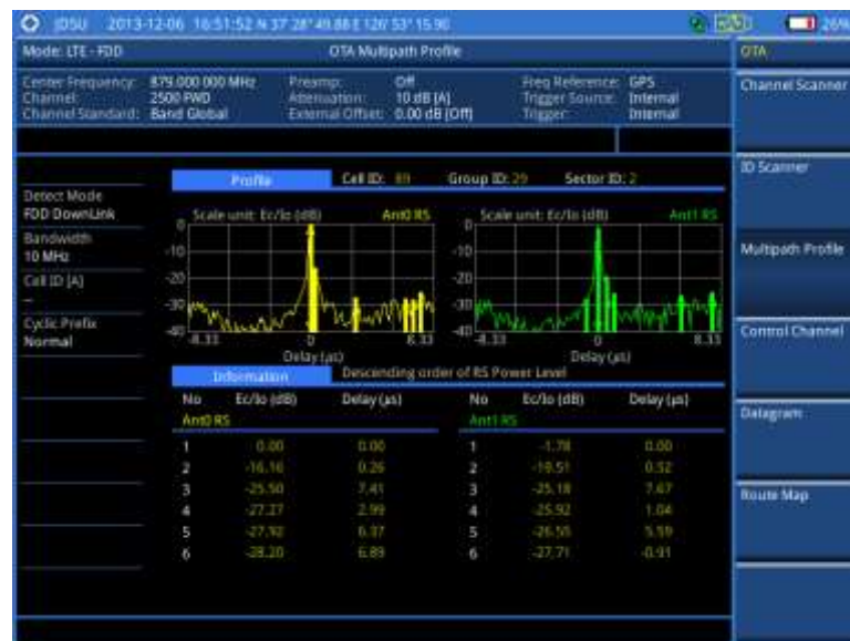
Figure 111 Multipath profile measurement with LTE - FDD OTA signal analyzer
