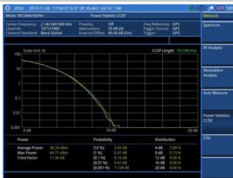
Figure 72 CCDF measurement with WCDMA/HSPA+ signal analyzer
