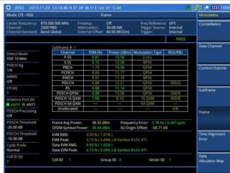
Figure 100 Frame measurement with LTE - FDD signal analyzer
