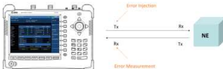
Figure 271 Error injection and measurement connection
