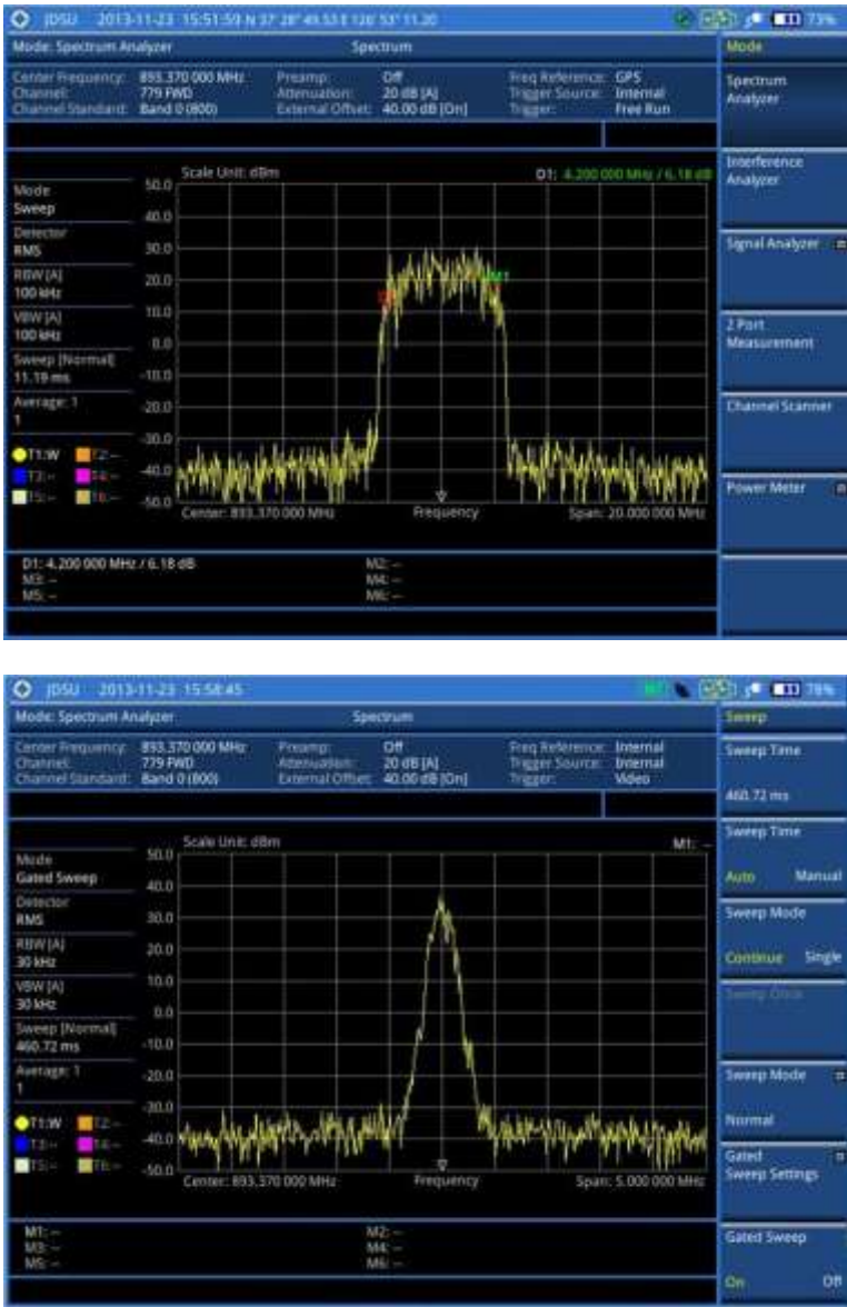
Figure 11 Spectrum measurement with spectrum analyzer
