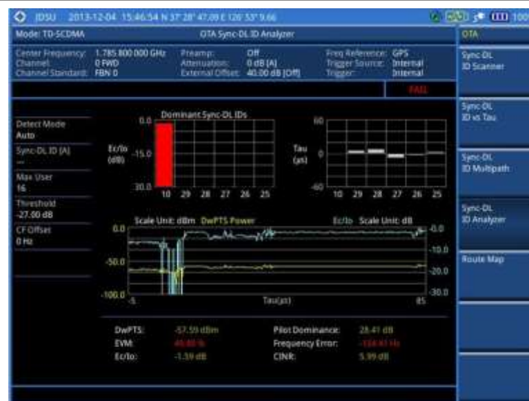
Figure 225 Sync-DL ID analyzer measurement with TD-SCDMA OTA signal analyzer
