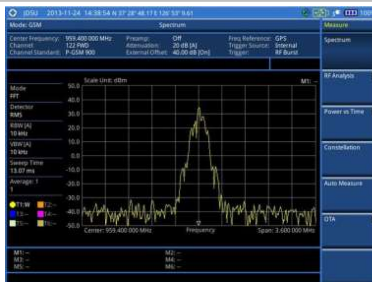
Figure 41 Spectrum measurement screen with GSM signal analyzer
