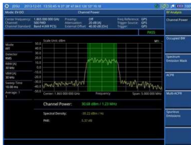
Figure 183 Channel power measurement with EV-DO signal analyzer
