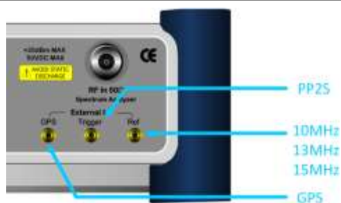
Figure 206 Connection ports for external reference clock
