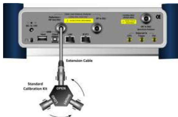
Figure 248 1-port calibration connection with mechanical Y-Cal kit
