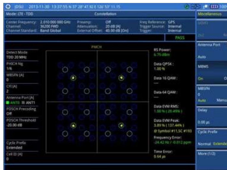
Figure 132 Constellation measurement with LTE - TDD signal analyzer (MBMS On)
