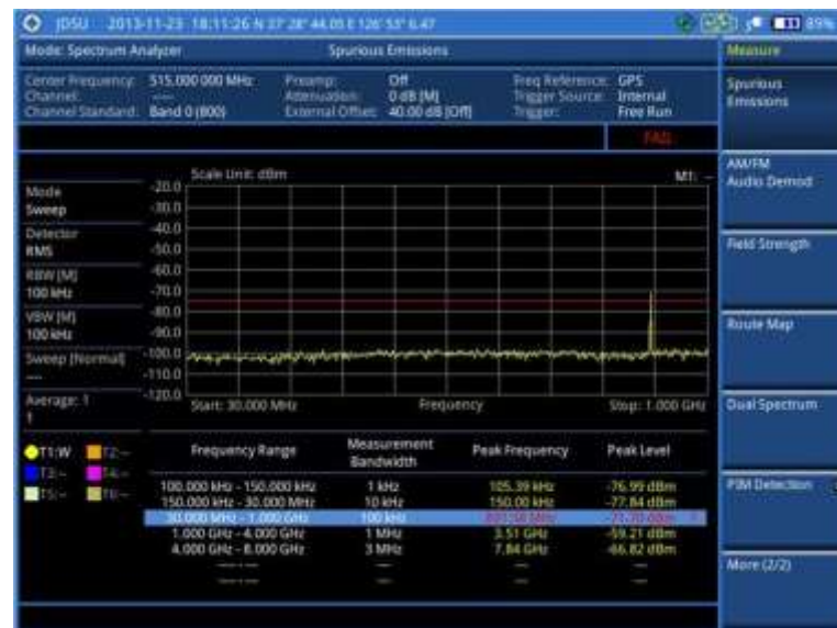
Figure 17 Spurious emissions measurement with spectrum analyzer
