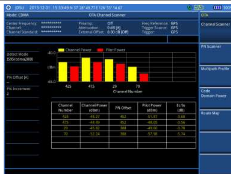
Figure 172 Channel scanner measurement with CDMA OTA signal analyzer
