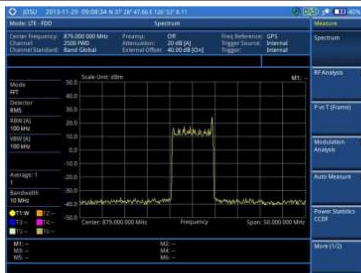
Figure 84 Spectrum measurement screen with LTE - FDD signal analyzer
