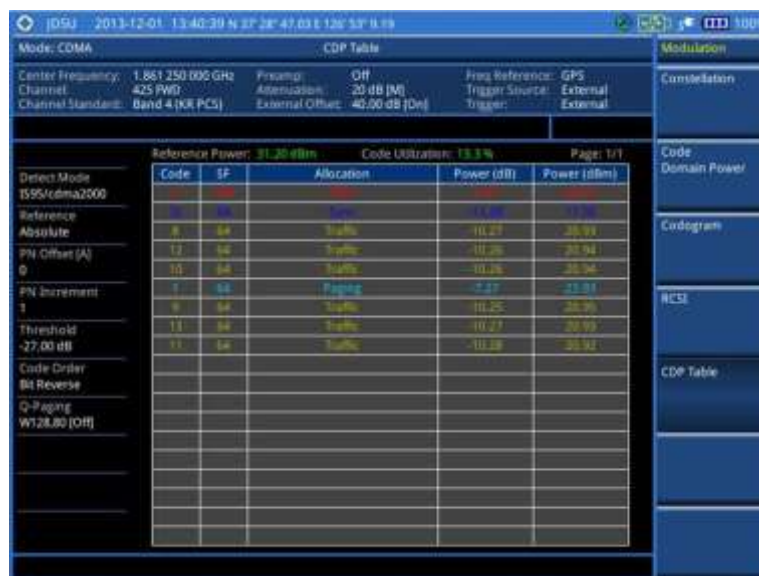
Figure 170 CDP Table measurement with CDMA signal analyzer
