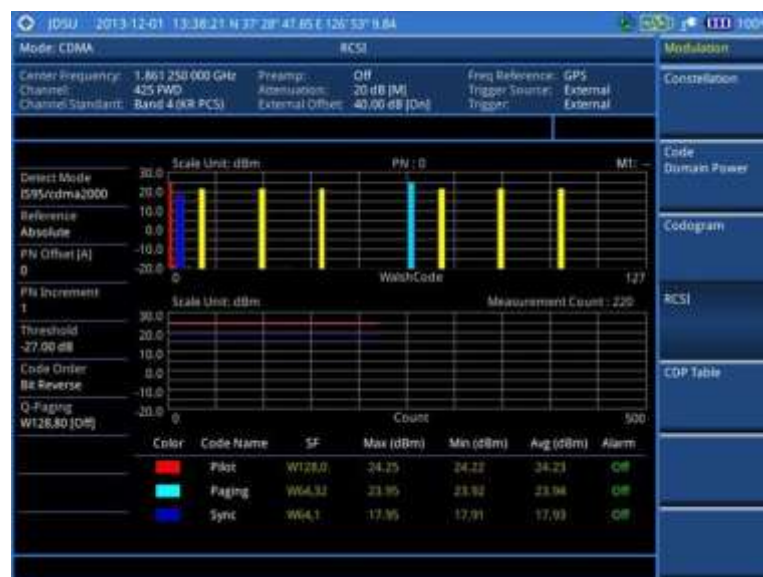
Figure 169 RCSI measurement with CDMA signal analyzer
