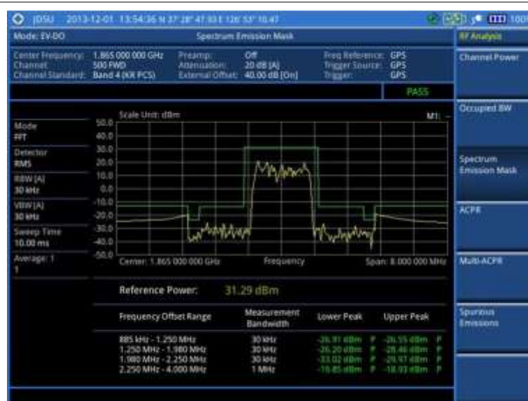
Figure 185 SEM measurement with EV-DO signal analyzer
