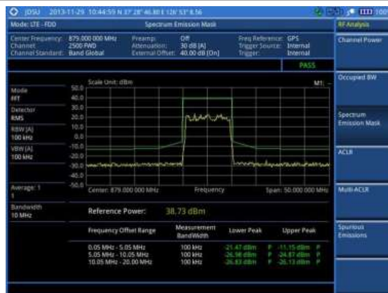
Figure 87 SEM measurement with LTE - FDD signal analyzer
