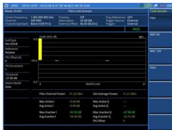
Figure 192 Code domain power measurement with EV-DO signal analyzer
