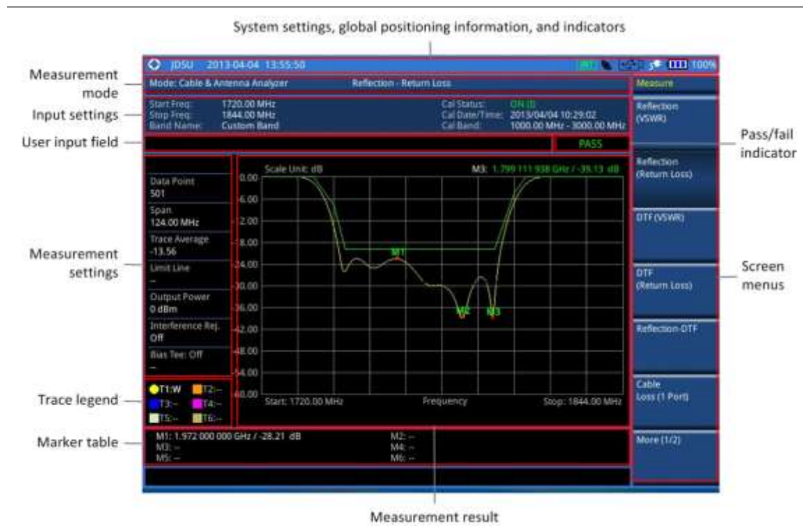
Figure 247 Reflection measurement screen
