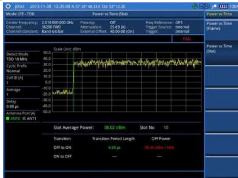
Figure 129 Power vs. time (slot) measurement with LTE – TDD signal analyzer
