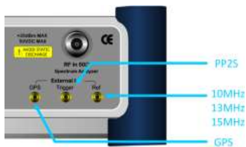
Figure 83 Connection ports for external reference clock
