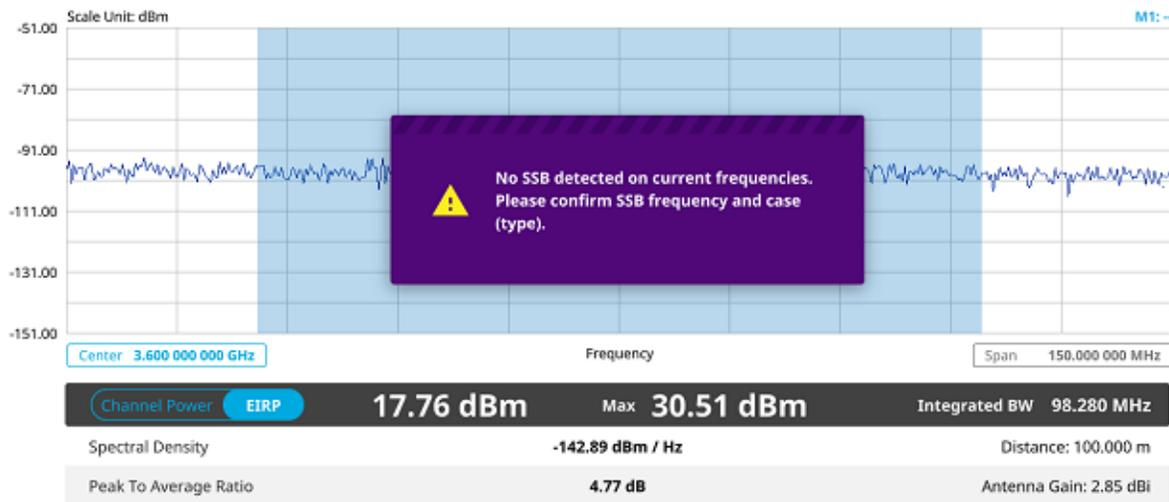
Channel power measurement result shows channel power and spectrum density in a user specified channel bandwidth. The peak to average ratio (PAR) is shown at the bottom of the screen as well. The shaded area on the display indicates the channel bandwidth.
