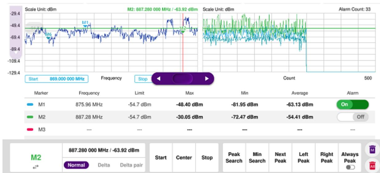
You can go to Menu > Limit to analyze your measurements with the display line, multi-segment line, and channel limit. See "[Setting limit](#)" for more details. Once you tap the vertical move bar and move it up and down, the reference line value changes.
